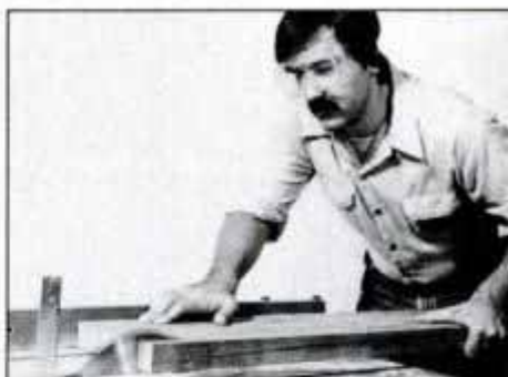
Eye protection, either goggles or face shield, is extremely important to block flying splinters and chips when using a table saw.
