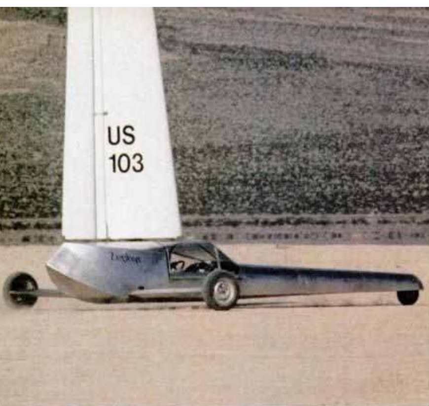
Recent breakthroughs include the wing/sail (above) on the hyper-speed Zephyr , and the aircraft-style cockpit (below) on Scudoo IV .
