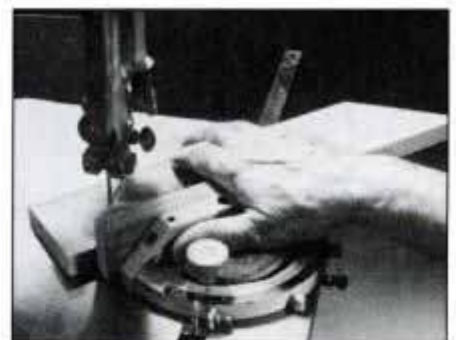
The miter gauge is also useful for sawing miters of various angles. Use a wide saw blade and slow feed rate to produce smooth cuts.
