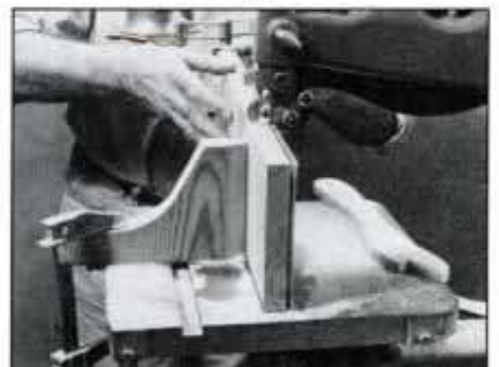
To make resawing easier, use a simple shopmade pivot block. Clamp the block to the worktable and guide the board against it.
