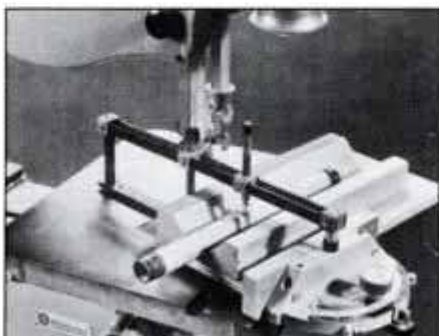
This setup shows how to employ a shopmade V-shaped cradle and a miter gauge to saw round stock, such as pipe and tubing, safely.
