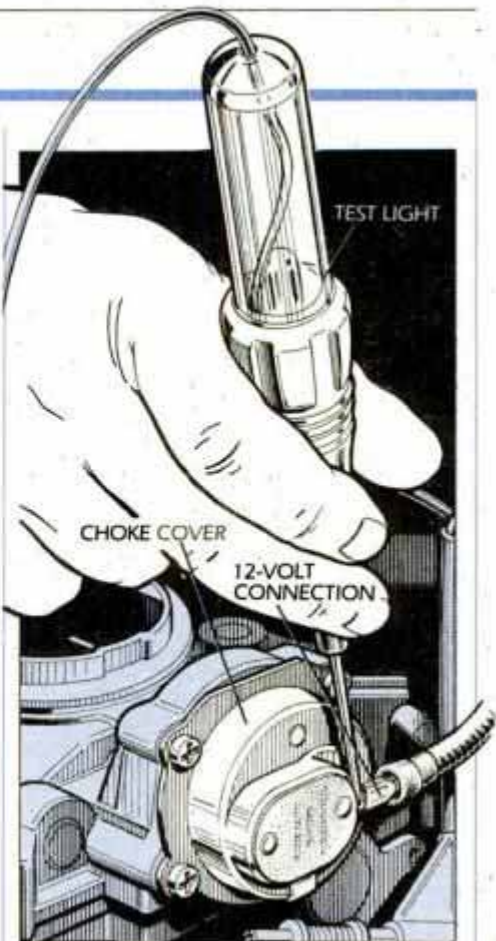
4 Test for 12 volts at choke cover with test light while engine idles. Light should glow.
