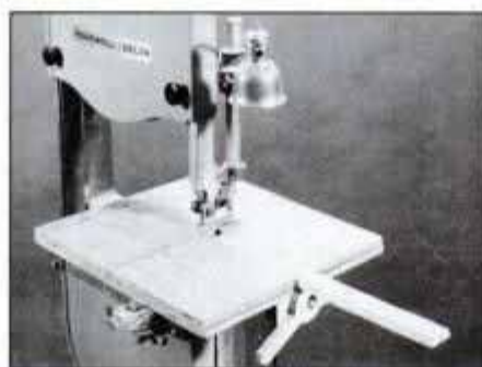
Easy-to-make circle-cutting jig fits over the saw's table. The bar extending from the jig to the right, adjusts for various size circles.
