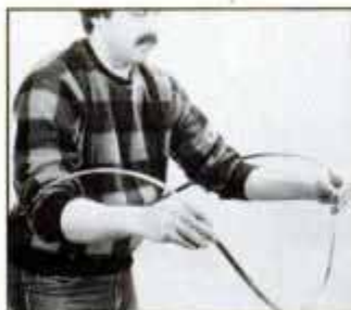
1 Grasp blade firmly, teeth facing up. Apply downward pressure to form first loop.
