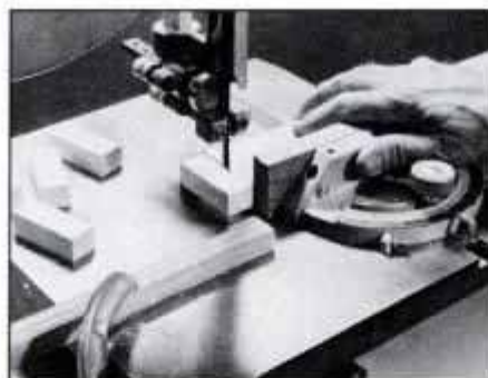
Use a miter gauge for accurate crosscuts. The wood bar clamped to the worktable acts as a stop. Butt stock to stop and make crosscut.
