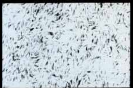
Compared to conventional videotape, Super VHS has finer particles, and more of them, to capture greater detail. These electron microscope photographs from Scotch/3M show (from left) standard VHS and Super-VHS particles magnified 42,000 times.
