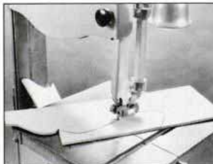
When two curves meet at a sharp, inside corner, first cut straight into the corner. Then, saw the two curved cuts to free the waste.
