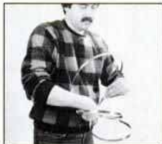
3 Slide out elbows, hold blade firmly in one hand as the other brings the loops together.
