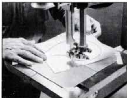
When sawing thin stock, such as sheetmetal, tape a 1/4-in. plywood panel to the saw's worktable to ensure smooth, burr-free cuts.
