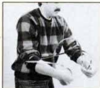
2 Turn wrists in and move your hands together. Bend blade up and keep elbows apart.
