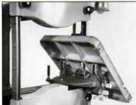
Underside of tilting worktable has a scale and pointer that indicates the degree of tilt. Note high-quality, cast-iron construction.
