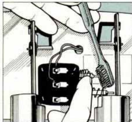
7 Use a toothbrush and lighter fluid to clean the parts of a bell, buzzer or chime. Don't lubricate to avoid collecting dust.
