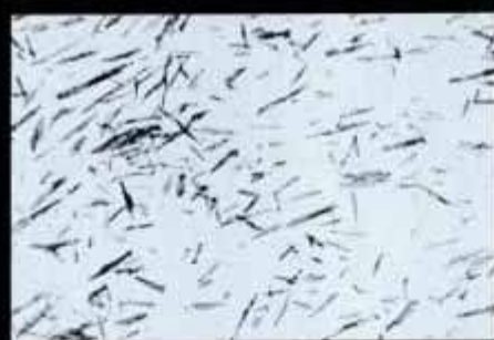
Compared to conventional videotape, Super VHS has finer particles, and more of them, to capture greater detail. These electron microscope photographs from Scotch/3M show (from left) standard VHS and Super-VHS particles magnified 42,000 times.
