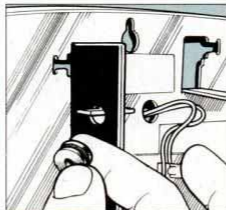
8 Rubber grommets in a chime unit isolate tone bar from its mounting. Get replacements if they're worn, hard or missing.
