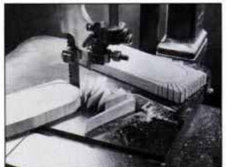
To cut curves with a wide blade, make tangential cuts or cut to the line several times, and then saw away waste (background).
