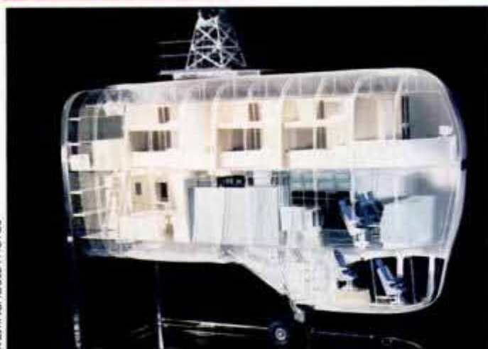
(Top right) Prototype Navy Airship. (Above) Airship's gondola: three decks include sleeping quarters for long-duration flight.
