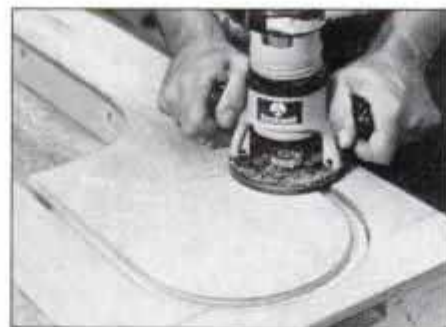
12 Use a straight bit and guide bushing to dress the edges. After one edge on each piece is done, disassemble and flip over.
