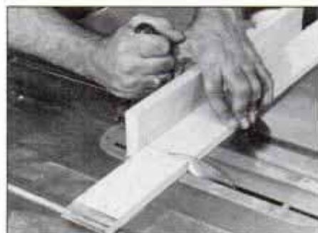
14 The straight ends of each lamination are cut individually on the table or radial-arm saw. Sand slats after trimming is done.
