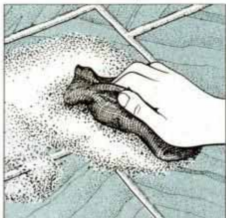
16 When grout is dry to touch, sprinkle sawdust on tile and rub with burlap cloth. This removes residue from grouting job.
