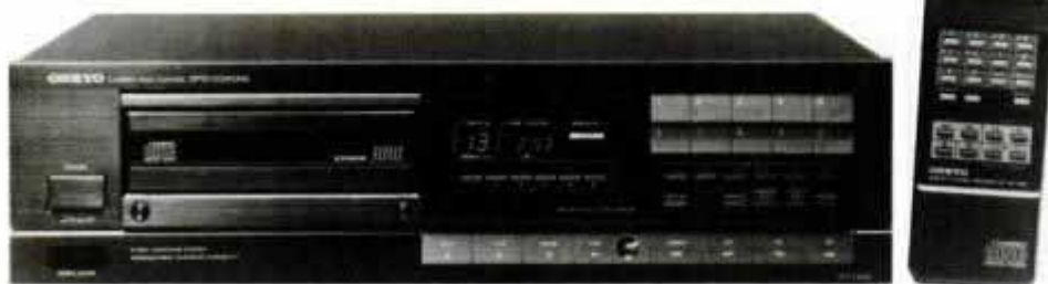
Onkyo's DX-C600 changer ($600) holds six compact discs, and has noise-free fiberoptic coupling between digital and analog stages. Remote control (right) is a bonus.
