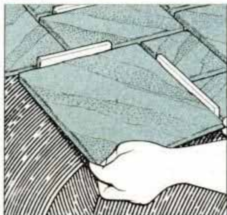
13 Set tile into mastic and press into place with slight twist. Use wood spacer blocks to maintain uniform grout spacing.
