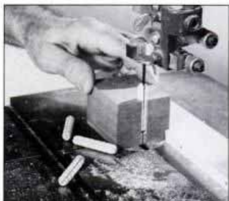
Using a shopmade jig, cut \frac{3}{4} of the way through a dowel. Use these dowels to dry-assemble parts—they won't stick in holes.
