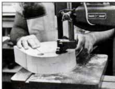
1 Glue up 2x4 stock to create the 3 \times 9 \frac{3}{4} -in.-sq. front form blank. Then, lay out the profile and saw to the line.
