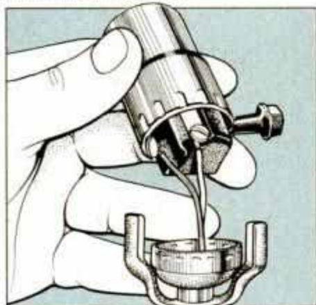
4 To expose the terminal screws, slide up the socket shell and insulating sleeve. Loosen terminal screws and pull off wires.
