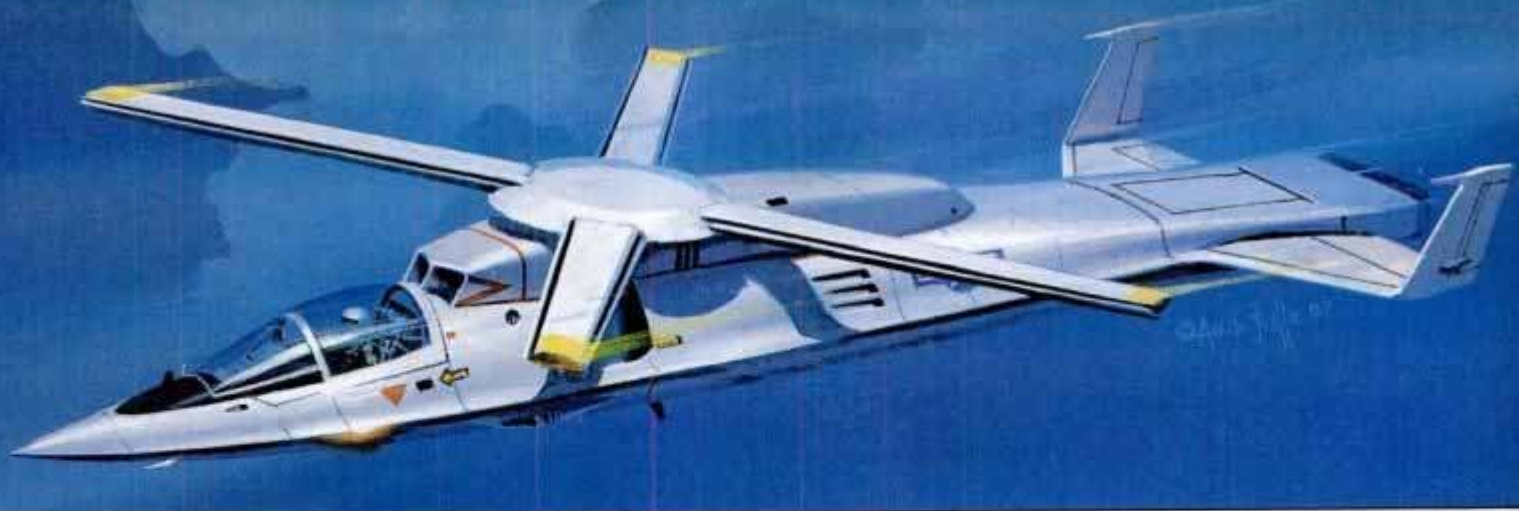
Slats in X-Wing's rotor will create lift in transition from vertical to horizontal flight. Plane will fly low-level attack, and engage fighters.
