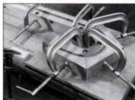
8 With the cauls in place, check that strips are even and fully tighten clamps starting at one end and working to the other.
