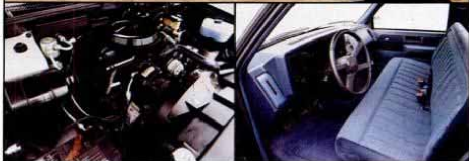
All-new Chevy combines good looks and performance with throttle-body fuel injection on its 5.7-liter V8. Interior is long on style, short on comfort and practicality.
