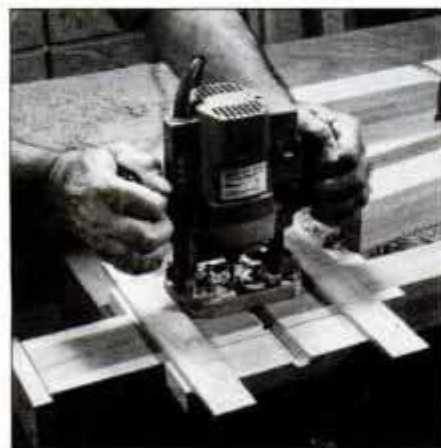
4 Horizontal coving jig guides the router squarely across each face of the leg. Use a \frac{3}{4} -in.-dia. corebox bit.
