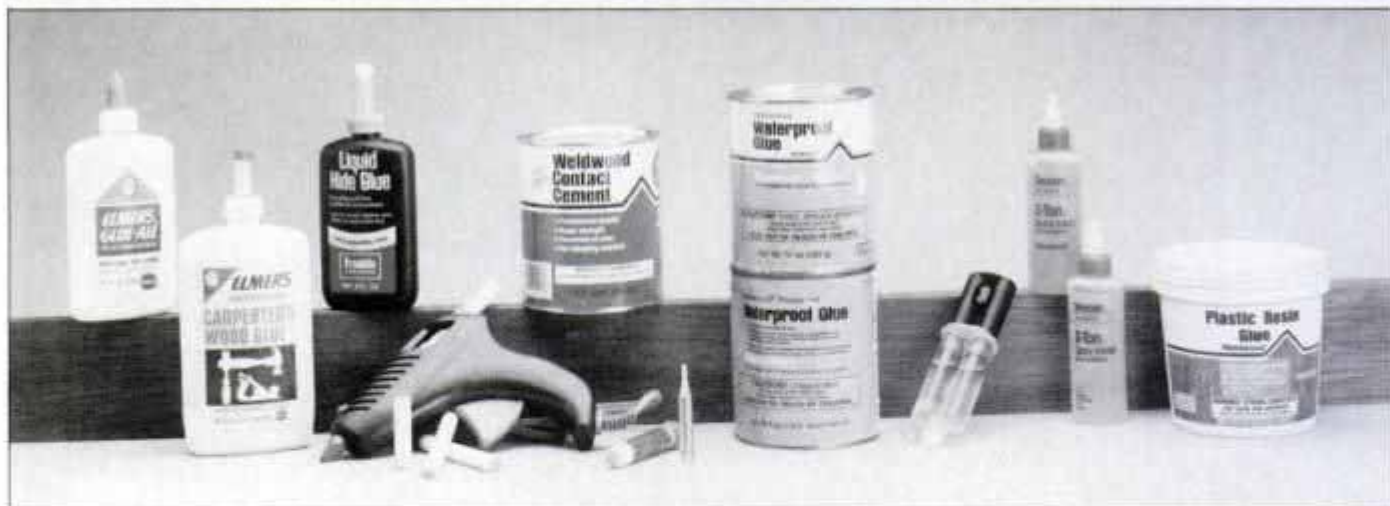
Here are the 10 most useful workshop adhesives (left to right): white glue, yellow glue, liquid hide glue, hot-melt glue sticks with glue gun, contact cement, instant-bond glue, resorcinol, 5-minute epoxy syringe, slow-set epoxy and plastic resin. See chart for uses.
