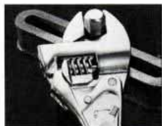
Close-up view shows that as the handle is swung to the right, the wrench's lower ratcheting jaw slides over the bolthead.
