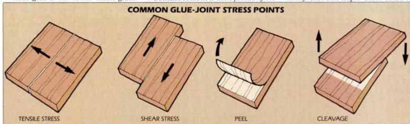
This illustration shows four of the many types of stress exerted on glue joints. Tensile stress pulls perpendicular to glue line. Shear stress
