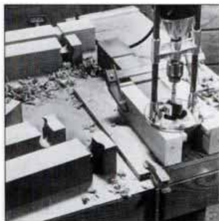
1 Two 1/2-in. holes create the inside curve on the front legs. Use a jig and drill guide for accurate positioning.
