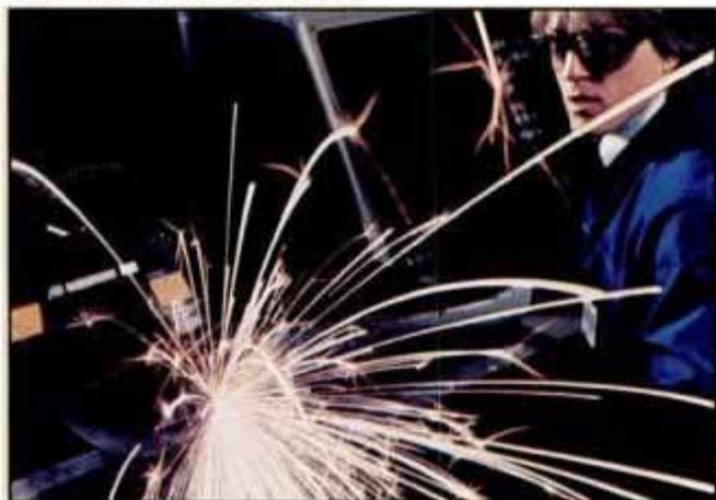
Northrop's 5-axis titanium cutting laser.
