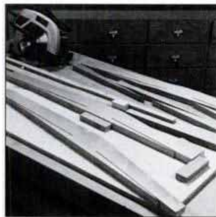
4 Rear leg cuts are guided with this jig. The stop keeps the circular saw from cutting too far. Finish with sabre saw.
