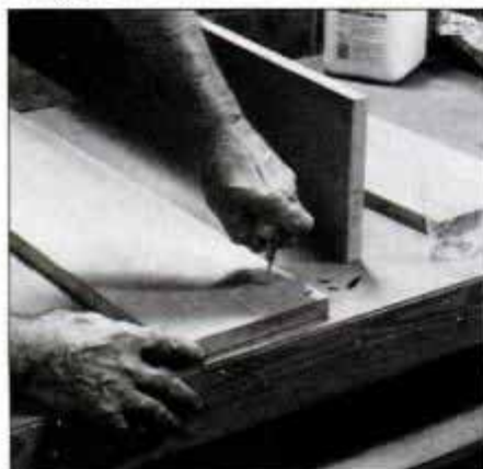
1 Select leg stock for color and grain orientation and insert headless brads to keep boards aligned during assembly.
