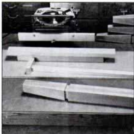
2 After cutting the horizontal coves, bolt a fence to the saw base and set up the tapering jig to shape the leg bottoms.
