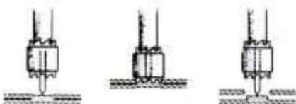
Line up Drill Cuts top layer only
