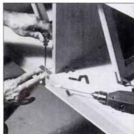
17 Hinge screw hole template ensures accurate positioning of doors. Use an awl to mark for the screw pilot holes.
