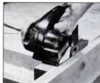
Cut a rabbet with a tungsten-carbide sleeve. Extend the sleeve beyond the tool's housing to equal the rabbet width.
