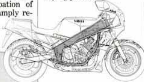
FZR1000's Deltabox framework is seen in the technical illustration above. The frame spars (left) snugly envelop the engine.
