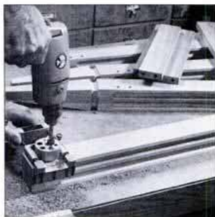
7 After marking the side rail hole positions in the legs, use a doweling jig to cut \frac{1}{8} -in.-dia. x 1\frac{5}{16} -in.-deep holes.
