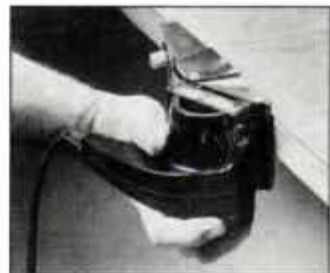
When fitted with an aluminum-oxide sleeve, the plane trims a door bottom quickly and neatly. Note the 1-handed operation.
