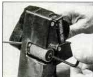
To change the abrasive sleeve, first insert a locking pin to secure the arbor. Then remove the screw with a hex-key wrench.
