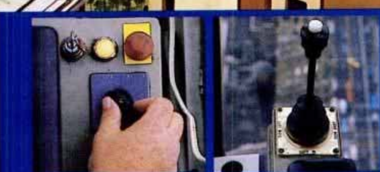
Photos L-R: Worker stands high above New York City on tip of American Pecco luffing boom crane; crews visit the end of the boom to grease the hoist cable sheave. Operator's-eye view of building site. Start key, condition lamp and master-stop button over gear selector. Joy stick controls left/right "slewing" action and boom angle.
