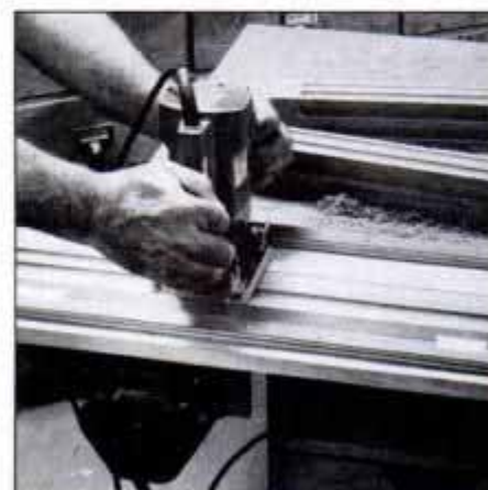
6 Tape spacer to side rail to provide support on both sides of the router. Shift spacer to the other side for second flute.
