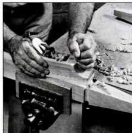
4 Use a sharp, finely set smoothing plane to dress the rough sawn surfaces of each of the legs before routing the flutes.
