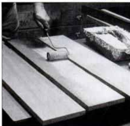
2 Use a roller to spread the glue fast and evenly. Make sure the brads are placed in waste area of stock. Clamp until dry.
