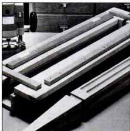
5 The flute routing jig guides router when making stopped flutes. Use a \frac{3}{8} -in.-rad. corebox bit set for \frac{5}{16} -in.-deep cuts.
