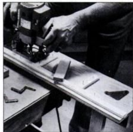
14 Hinge mortising jig guides router when making 3/16-in.-deep mortises in the doors. Space guides to suit your router.
