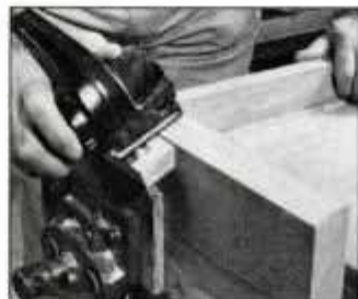
To plane a beveled edge, attach a shop-made wood fence to the tool's base. Cut the fence to match the desired bevel angle.
