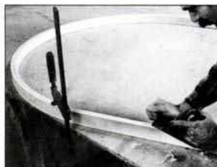
9 When the glued-up bow has completely dried, clamp it to the worktable and hand plane one edge square and flat.
