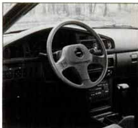
Steering wheel turns the front wheels, rears are turned automatically, 5" maximum.
