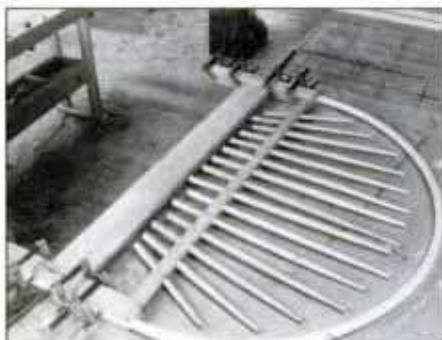
16 After gluing up headboard legs, rail and spindle rail, insert spindles. Glue and clamp the completed bow in place.
