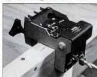
Then, without moving the jig, bore a mating hole in the other board. Shift the jig and bore the next pair of dowel holes.
