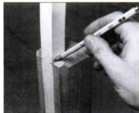
11 Insert the bow in the headboard-leg grooves and mark the starting points for the chamfers. Cut chamfers with a router.
