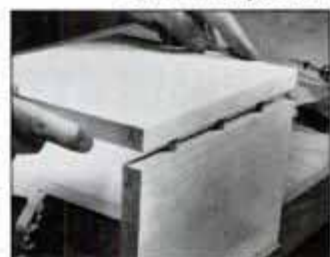
Assemble the joint with glue and fluted or spiral-grooved dowel pins. Don't use sections of plain dowel rod as dowel pins.
