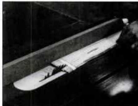
3 Cut the veneers to a uniform width by first stacking them and securing with tape. You'll need 17 12-ft. strips.
