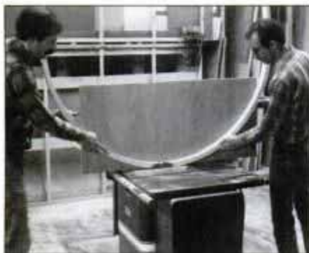
10 Install an oversize fence on the table saw. Rip and saw bow to width. Make sure the bow rests on table at the saw blade.
