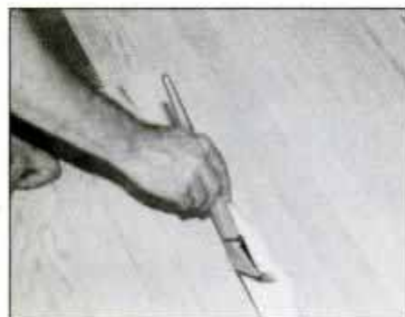
Tone down dark spots and any wild grain using additional paint. Work with a small brush and remove excess with a rag.
