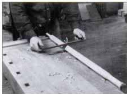
15 Turn short spindles completely on the lathe. Turn only long spindles, ends and shape with a drawknife and spokeshave.
