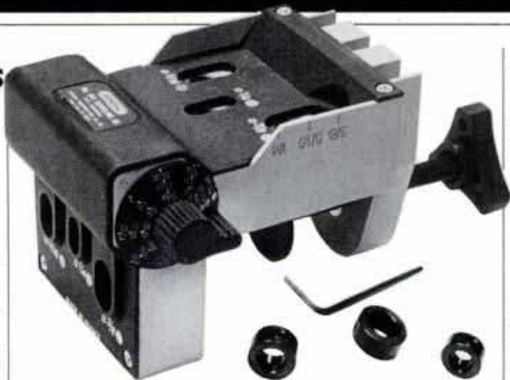
Doweling jig accepts stock from 1\frac{3}{32} in. to 1½ in. thick. Set calibrated dial to stock thickness and the dowel holes are centered automatically. The jig comes with three drill stops and hex-key wrench.
