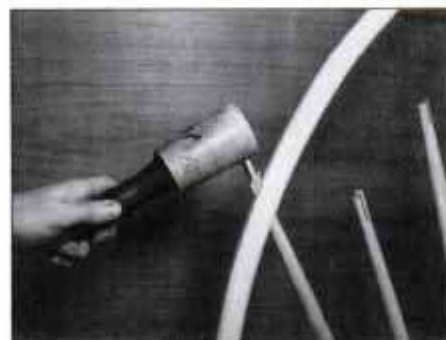
17 Pass the spindles through the bow-spindle holes and drive wedges in the slotted ends at bow and spindle rail.
