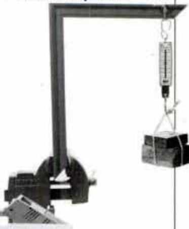
Hot-melt glue proved to be surprisingly strong. The partially assembled frame shown supported 13 pounds without falling.
