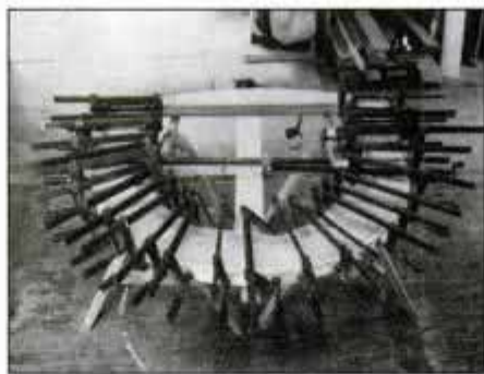
5 Start applying clamps at one end and work your way around the form. Use as many clamps as possible for a uniform joint.
