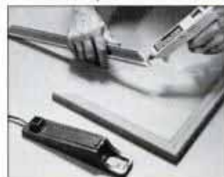
Hot-melt glue is excellent for assembling small workpieces. The glue bonds in just a few seconds. No clamping is required.
