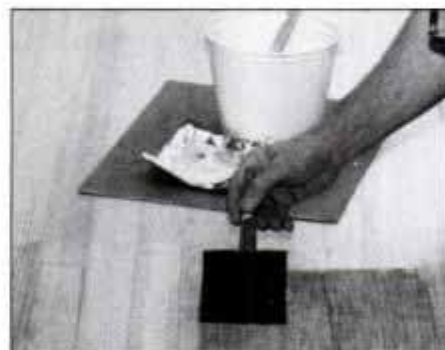
Apply polyurethane with a disposable foam brush. Do not over brush, and be sure to stir polyurethane frequently as you work.
