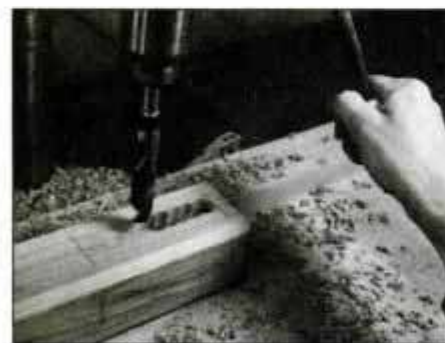
7 The mortises in the legs are started on the drill press by boring 3/4-in.-dia. holes. Use a sharp chisel to clean up waste.
