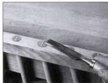
18 Cut the spindle ends nearly flush with a fine dovetail saw and use a sharp chisel to trim them flush with the surface.
