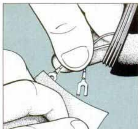
3 Use very fine emery cloth or sandpaper to clean Y-shaped terminals of receiver. Clean back surface of the receiver, too.
