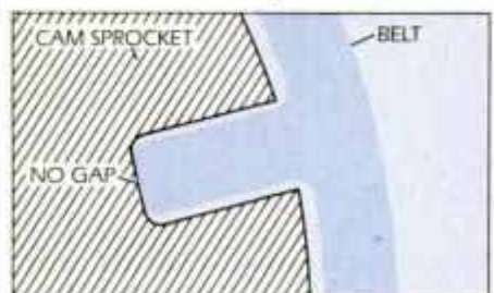
CHRYSLER: 2.2 and 2.5 cam timing belt teeth have been reprofiled to reduce noise.
