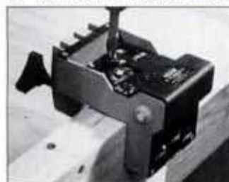
With the boards held securely in a vise, clamp the jig in place. First, bore the dowel-pin hole in edge of the board, as shown.
