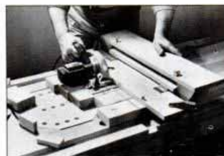
3 Crosscuts on long unwieldy stock are easy when the stock is held under the bridge fence and cut with a handheld saw.
