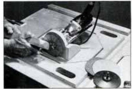
14 The top-mounted drill also powers a disc sander or disc rasp. Install a buffing wheel for polishing chores.
