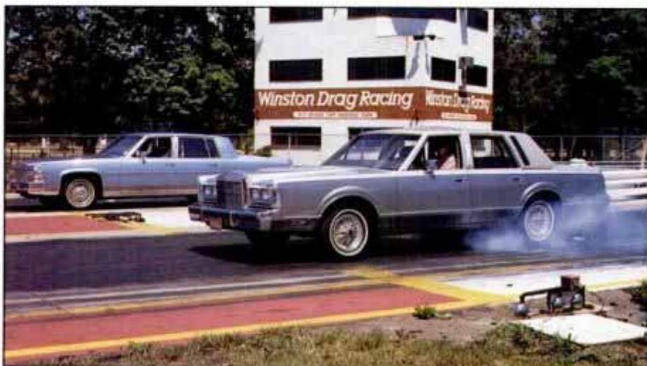
Injected Lincoln was much faster than 4-barrel Caddy at the drag strip despite only a 10-hp difference in their official horsepower ratings.
