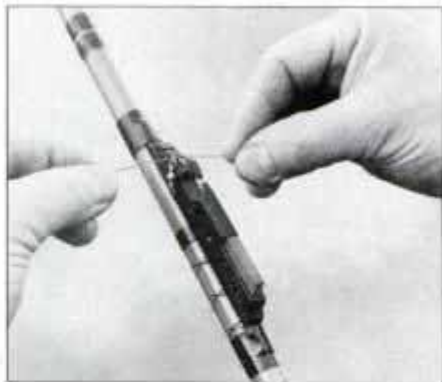
A blade and sharpening stone are combined in this cleverly mounted fishing tool.
