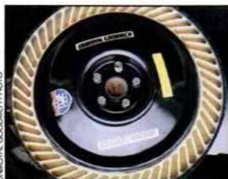
Steel wheel drilled for standard bolt holes is surrounded by spare's polyurethane vanes.
