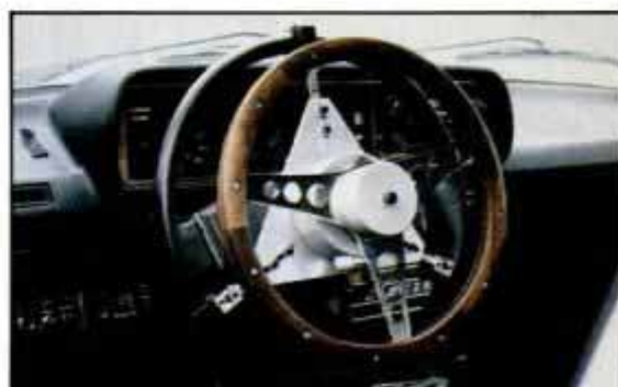
The clamp-on transducer tells engineers how much force it takes to turn front-wheel-drive steering wheel.
