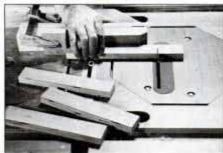
5 Clamp a stop block to the miter gauge for repetitive cutting. For longer pieces, clamp the block to the table surface.
