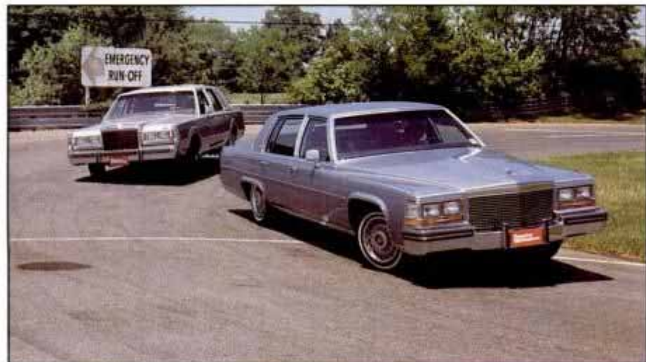
Handling of the two cars was flaccid with lots of body roll and plowing. The numbers generated on the test track were about the worst we've ever recorded.
