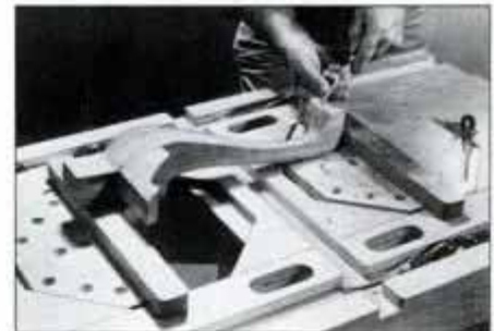
16 Auxiliary clamping blocks permit gripping work with small contact surfaces. Use them with a split clamping plate.
