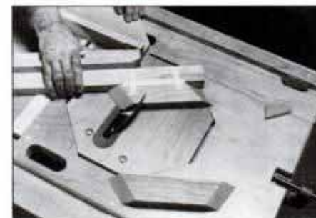
6 Cut compound angles by adjusting the miter gauge and bevel the angle on the saw. Use backup stock to cut small pieces.
