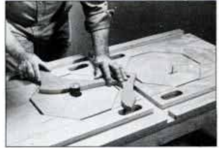
12 After cutting the profile, move to the drum sander. It's powered by the drill mounted in a drill guide under the plate.
