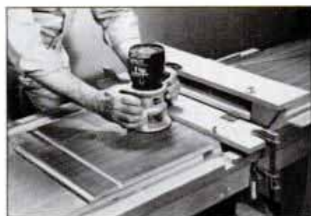
4 Use the bridge fence to guide your router when cutting dadoes square to the panel edge, as in shelf construction.
