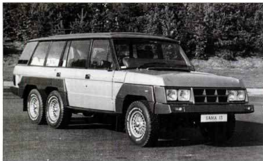
You, too, could be at home in a Range Rover that's been stretched nearly 4 ft. Extra axle at the rear supports added weight of luxury appointments that are literally fit for a king.
