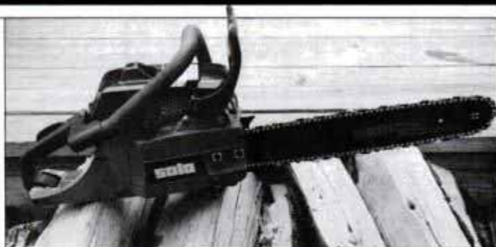
The saw's excellent power-to-weight ratio means higher torque at reduced weight. Model 647 accepts a 14-, 16- or 18-in.-long bar.
