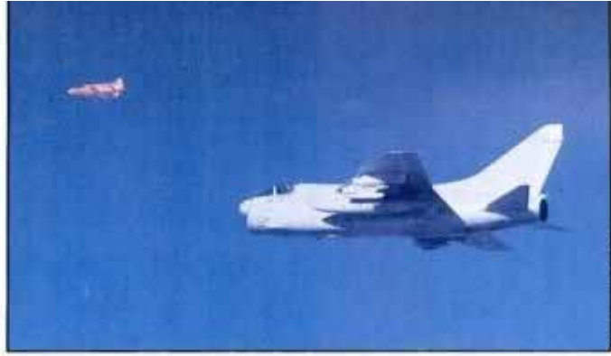
Tacit Rainbow antiradar missile being released by an A-7 Corsair. The new missile waits for enemy radar to activate.
