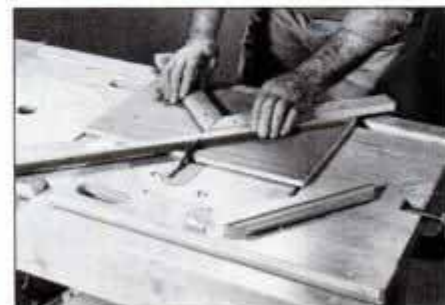
7 Picture frames require that stock be held molding side up for smooth cuts. Use this miter jig for accurate, clean corners.
