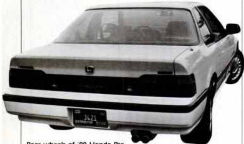
Rear wheels of '88 Honda Prelude countersteer 5.3°.
