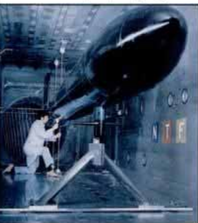
Technician checks inverted sub model in Langley wind tunnel.
