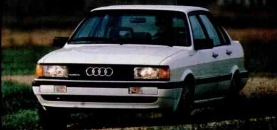
Audi Quattro 4wd system, meant for full-time use, also has 50-50 split.
