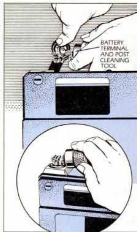
3 Use brush of battery post cleaning tool to scrub side mount terminals and connectors.
