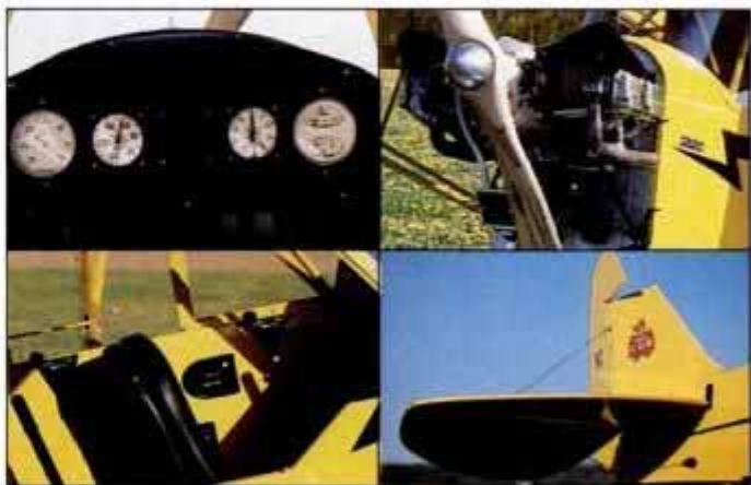
Details of the exquisitely restored Cub, from the top left and moving clockwise: Original instruments let you know the VFR basics, an engine meant for flying low and slow, elemental cockpit controls, and the lower right, fabric and dope tail section.
