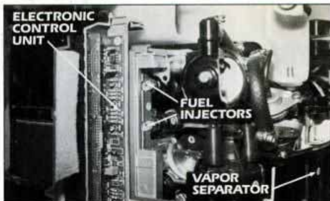
Mercury XRI: Power and efficiency from a production EFI outboard.
