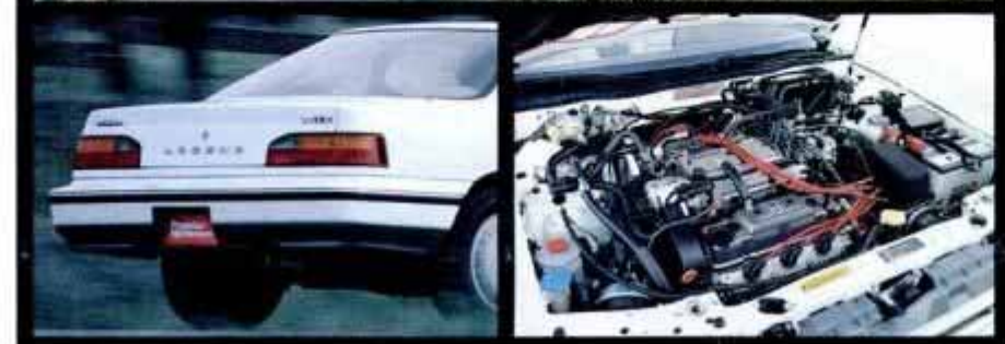
Enlarged 2.7-liter version of the Honda V6 gives new Legend Coupe more power. Coupe roofline styling suggests that of several BMWs, the new Acura's target audience.
