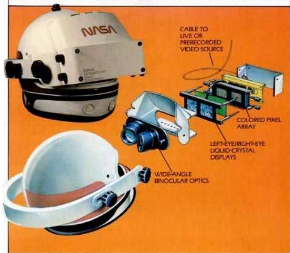
What's the opposite of tunnel-vision? It's NASA's Virtual Environment Workstation, a 3-D theater in a helmet that uses wide-angle LCD goggles to send the correct perspective to each eye. Images can come from dual video cameras or from prerecorded 3-D sources.
