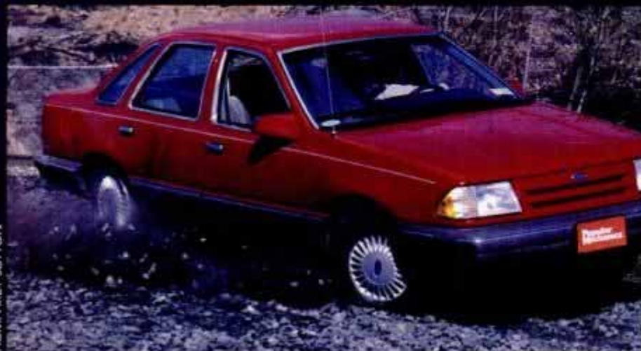
New 4wd entry, Ford Tempo, has part-time system with 50-50 torque split.
