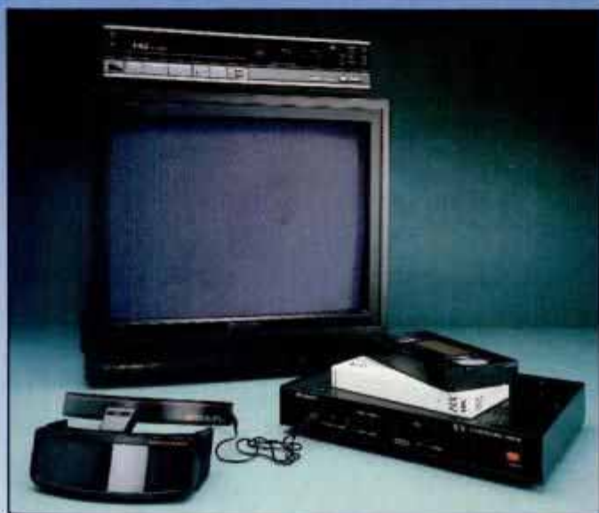
Sharp's prototype 3-D home video system uses a conventional TV and VCR. An adapter (right) connects to these and to LCD glasses (left) to synchronize left/right views on 3-D videotape.
