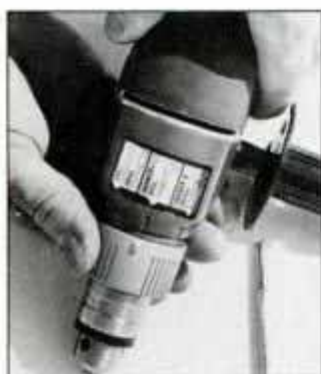
To switch operating modes, push control collar forward and rotate it to desired position.
