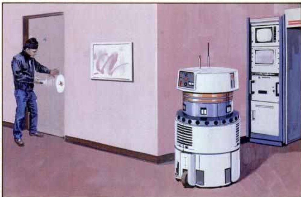
Sentry I senses movement and heat from intruders, and reports to security personnel. Unit stores in control panel alcove, which contains a socket to recharge Sentry I 's 12-volt batteries.
