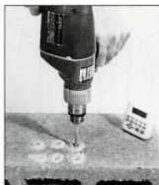
It took just 6 seconds to hammer-drill through block. Regular drill mode took 55 seconds.
