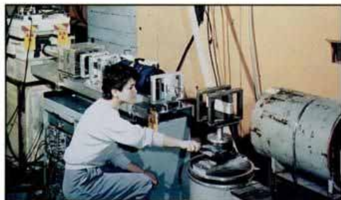
A scientist measures magnetic fields on the surface of materials using a new device called a polarized neutron reflectometer.
