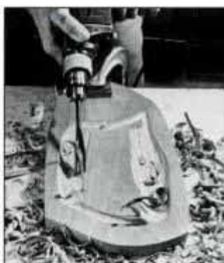
Power chisel, with V-shaped gouge, removes stock quickly. Flat chisels are also available.
