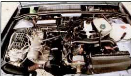
Familiar 1.8-liter VW engine sits front-to-back under the Fox hood, rather than transversely.
