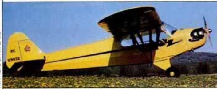
An early version of the Piper J-3 Cub restored: Fabric, dope, easy to maintain powerplant—and a liberating simplicity.
