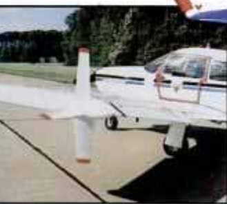
Wind turbine generators harness energy lost from a wing's tip vortex.
