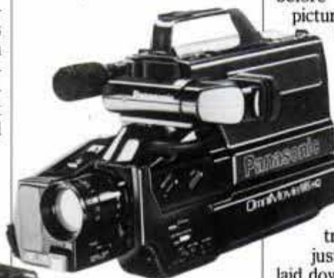
Panasonic's VHS-C format camcorder (above) and Sanyo's 8mm model share high-speed shutters for sharp slow-motion, flying erase heads for edits.
