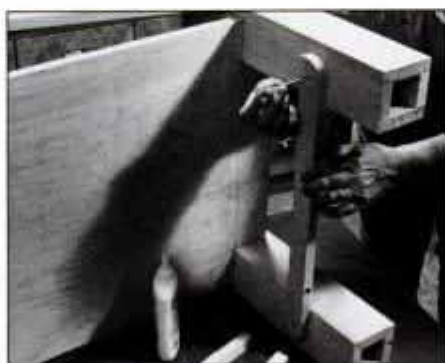
5 Slide in the top shelf before attaching the support cleats. Screw and glue the cleats and screw the shelf in from below.
