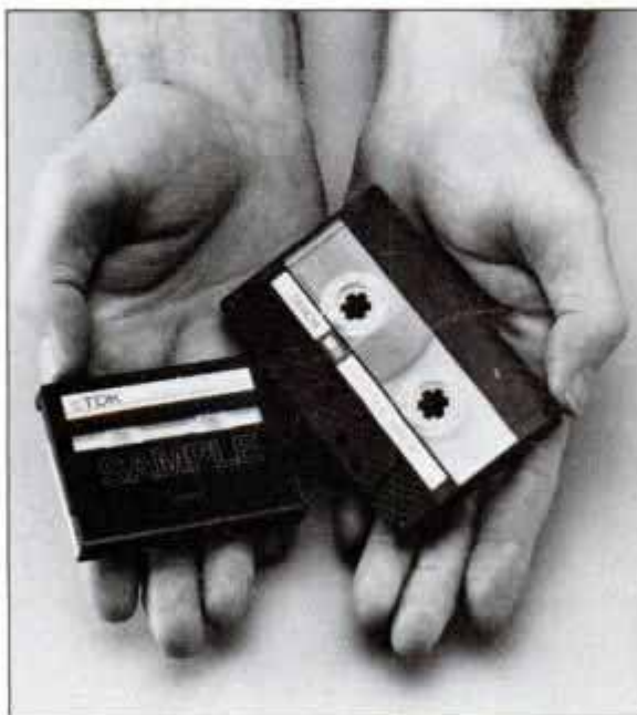
DAT cassette (left) is half the size of today's analog cassette, yet holds two hours of sound. Though tape is same 15/100 in. wide, it uses a high-density metal formula.
