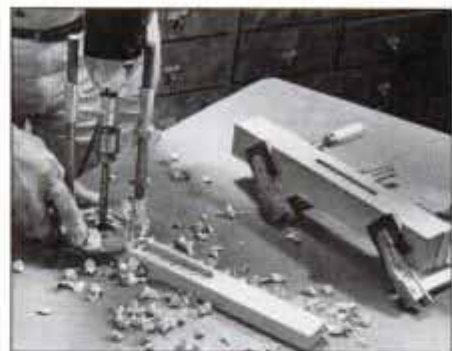
14 The miter-gauge rail is recessed underneath for the carriage bolt head. Laminate maple stock for the adjustable beam.
