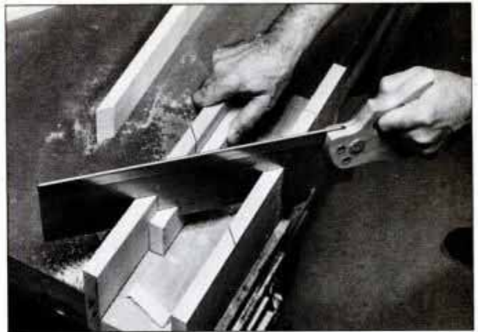
A miterbox guides a fine-tooth backsaw for cutting accurate 90° square and 45° miter cuts. The saw slides in guide-slots cut in the box sides. Hold work securely to prevent shifting.
