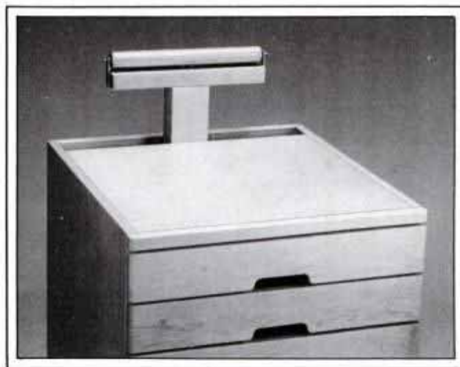
Cabinet features an adjustable-height outfeed roller that stores behind the drawers. Use roller to support long boards when working on the torsion-box workbench or power-tool table.
