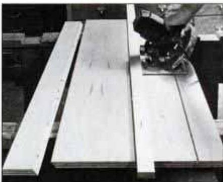
8 Rip the inner guides and the fixed and sliding plates. Be sure that the cuts are absolutely straight and parallel.
