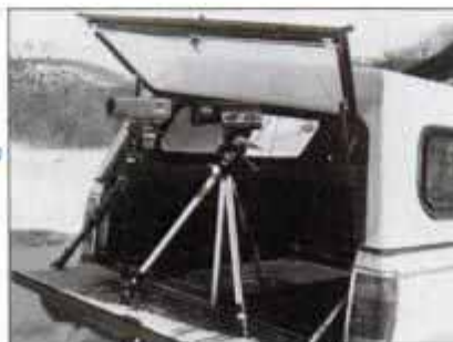
X- and K-band radar guns were clamped to tripods and used alternately in tests.
