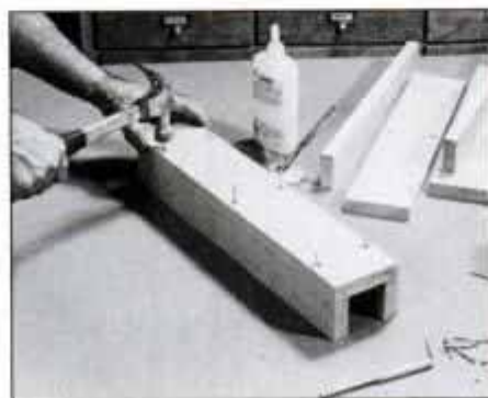
1 Assemble the legs with nails and glue. Bore ⅝-in. pilot holes and counterbore for plugs. Finish driving with a drift punch.
