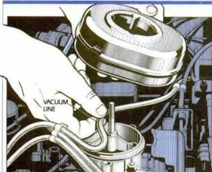
2 Damaged vacuum lines can disable an EGR system; be on the lookout constantly for kinked or cracked hoses.
