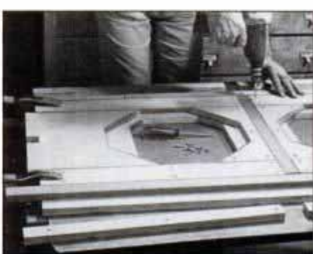
10 Bore pilot holes and counterbores for the guide mounting screws and plugs. Align outer guides with a 1 1/2-in. spacer.
