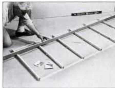
3 Check the assembly surface to be sure it's absolutely flat. If necessary, fine tune the cleat upper edges with a plane.
