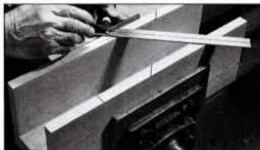
Glue and screw together the box. Then, use a combination square to mark cutting lines on the top edge of the sides. Mark 90° and 45° lines.
