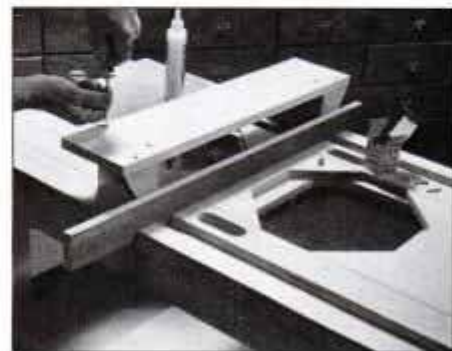
15 Assemble the fence with the rails in the tracks. Use a piece of straight stock in the cross track to insure square.
