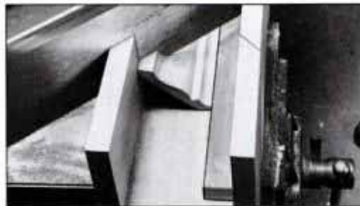
When cutting crown molding, insert a spacer strip to prop it up at the correct angle. Make a 45° cut to produce a compound-angle cut.
