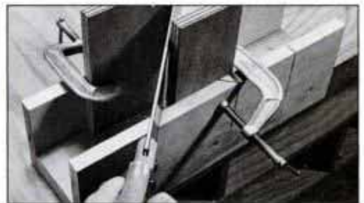
Clamp wood blocks to the box to guide the saw and hold it on the cutting lines. While sawing, the saw's spine should be against blocks.
