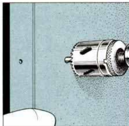
2 Bore lockset hole first using hole saw. Bore until pilot bit breaks through other side, then complete hole from other side.
