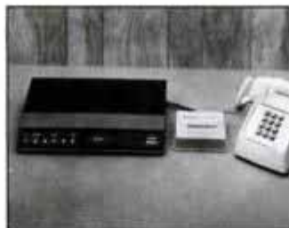
Two of the many accessories available include a glass-break detector (left) and an automatic phone dialer (above). In case of a break-in, dialer calls a central dispatch station that, in turn, calls emergency numbers.
