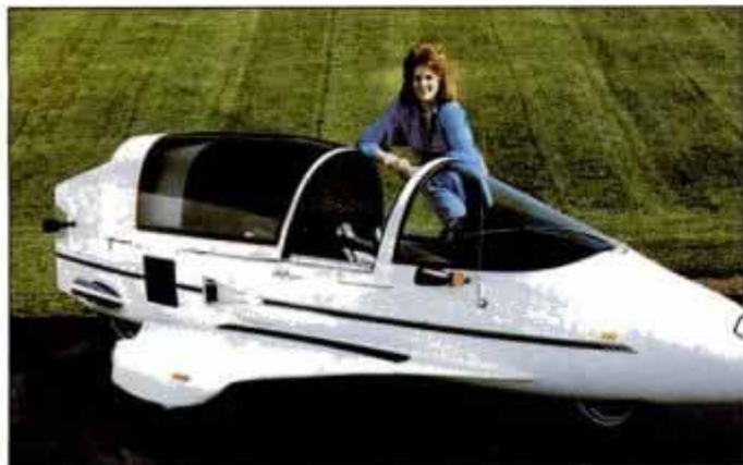
Aerodynamic Pulse GCRV has tandem seating for two, training wheels in the little winglets, and a Honda motorcycle drivetrain.
