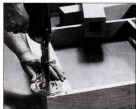
4 A drill guide ensures straight dowel holes. Bore 1½-in.-deep holes for 2-in. dowels to allow for excess glue.
