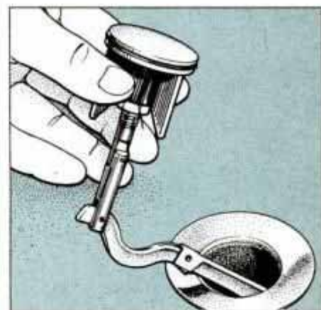
2 To clean plunger type, just remove screen. For pop-up (shown above) just pull mechanism from drain opening.
