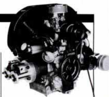
Beetle motor can be converted to an air compressor.
