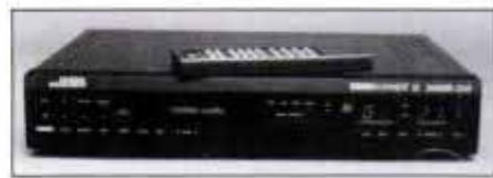
Scrambler-owner General Instruments also builds descrambler into its remote-control VideoCipher II 2400R satellite TV receiver.
