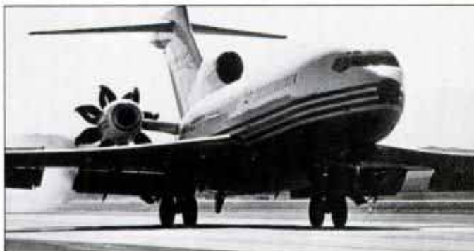
GE's unducted fan engine goes through R&D at Mojave.
