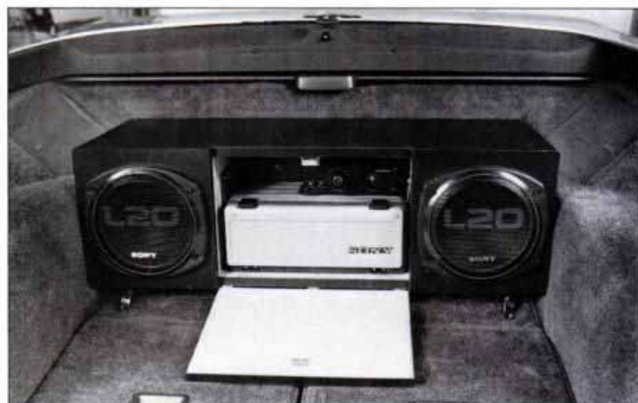
Hatchbacks, such as this Corvette, lack shelf and trunk for good bass. The built-in platform here (housing subwoofer, CD changer) serves same purpose and supports cargo.
