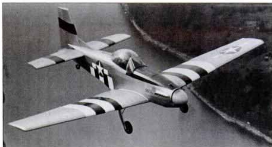
The "5151" repliplane, a 3/4-scale Mustang replica, passes its first 100-hour test.
