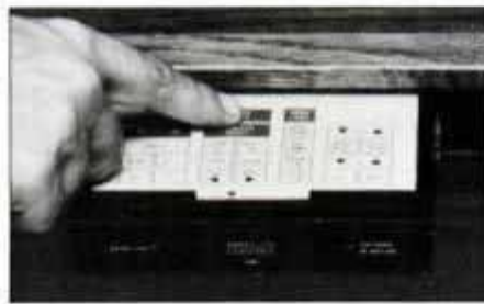
The latest satellite receivers have built-in descramblers. Experimental Zenith system packages receiver, descrambler and antenna-positioner into 27-in. stereo TV.
