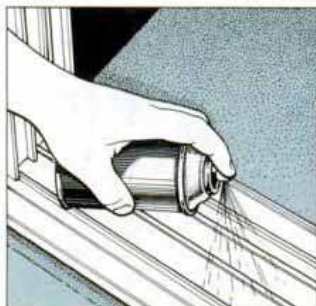
2 After cleaning, apply a light spray lubricant to discourage dirt buildup and help keep the rollers moving smoothly.
