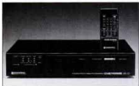
Cheyenne IR/D from Chaparral integrates satellite TV receiver with descrambler.
