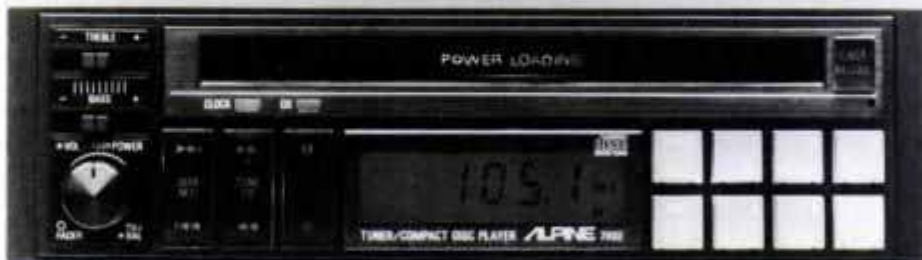
Most recent car CD players now include an AM/FM tuner, thanks to miniaturized components and improved internal shielding. Alpine's 7902 adds a cassette input, too.
