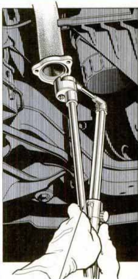
5 Stud removal tool and careful use of heat can save a corroded manifold.
