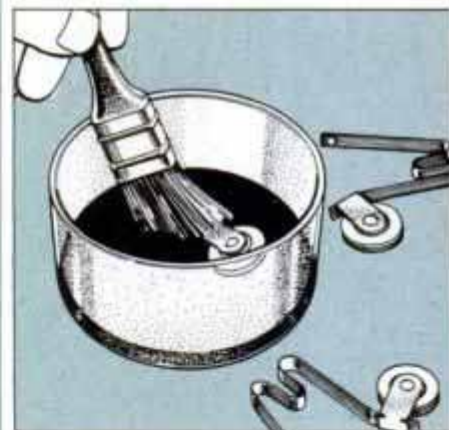
7 Thoroughly wash the rollers in mineral spirits. After wiping them dry, lubricate with a light oil for smooth running.
