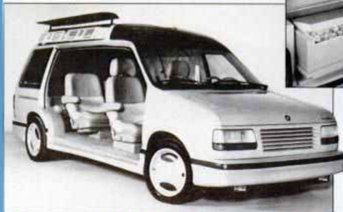
Sculpted front end, contour seating and integrated roof storage characterize the Plymouth dream machine. Party module, top, inserts in tailgate.
