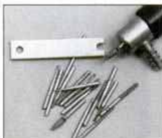
The handpiece and wrench are shown with just a few of the hundreds of burs available.
