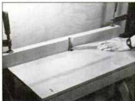
5 Cut a bullnose on the outside curved edge of the leaves with a \frac{3}{4} -in.-rad. rounding-over bit mounted in the router table.
