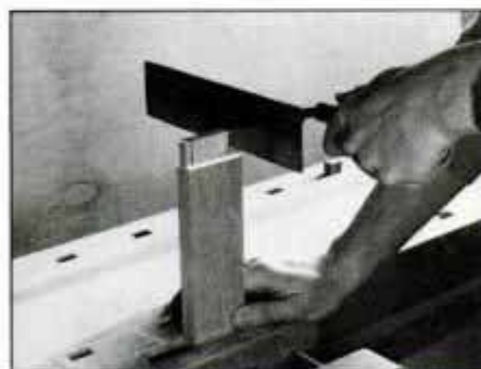
10 After cutting the apron tenon cheeks, mark and cut the shoulders using a dovetail saw. Check fit in leg mortises.
