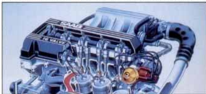
Saab's 16-valve is 2 liters, good for 160 hp with turbocharger.
