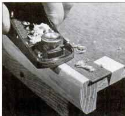
Here's an easy way to get the wood edge flush with the laminate. Place the laminate upside-down and plane the wood flush.
