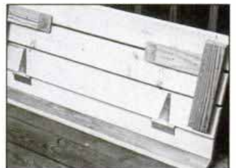
24 Nail boards for tabletop to end cleats. Then attach wedge-shaped stop blocks and galvanized T-hinges to bottom of table.
