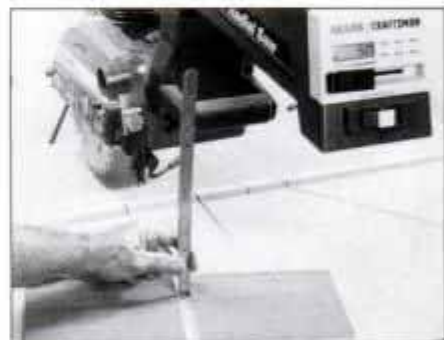
Rule is used to check \frac{1}{4} -in.-deep dado cut in \frac{3}{4} -in. stock. Elevation reading of .50 in. is distance from table to blade.
