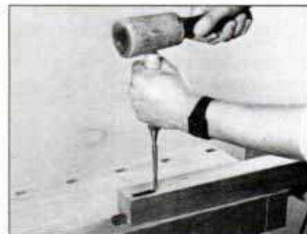
9 Clamp the table leg to the bench and use a sharp chisel to clean up the sides and square the ends of the mortise.
