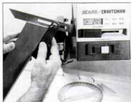
To test accuracy, I cut an odd-angle miter—20 \frac{1}{2} °—and then checked the cut with a bevel square. Cut was right on the mark.
