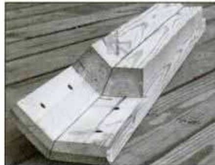
20 Join both sides of angled post together with 3\frac{1}{2} -in. No. 12 fh screws. Bore pilot holes, countersink and plug screwheads.
