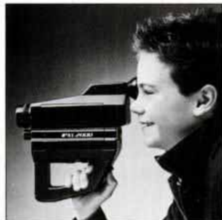
Fisher-Price PXL 2000 camcorder uses audio tapes to record b&w video movies.
