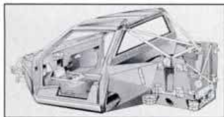
Composite chassis is light and strong.
