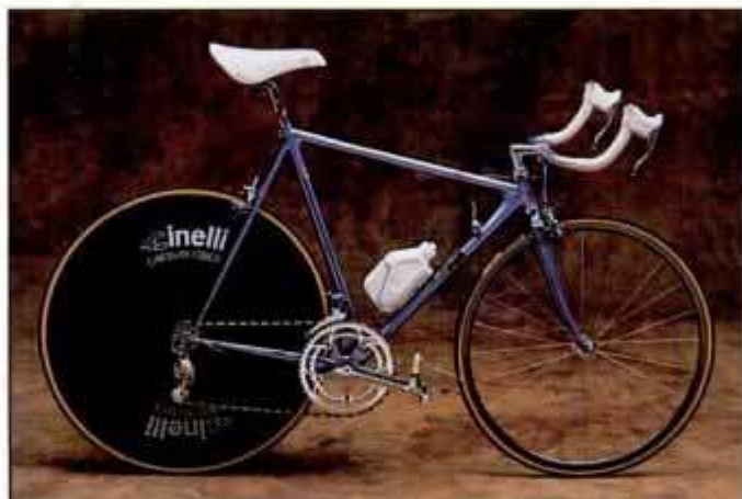
Cinelli Laser Kronos is a road-going time trial machine that displays racing posture with sloped top tube and competition wheels.
