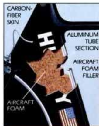
Outlawed! Now illegal for UCI events, the Huffey Olympic hopeful for 1988 gained an aero edge with a carbon-fiber and aircraft foam seat tube section. New design is already in the works.
