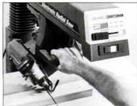
The saw will cut bevels between 0 and 90°. Here, a 30° bevel cut is made. Note the 30° reading visible in the LCD window.
