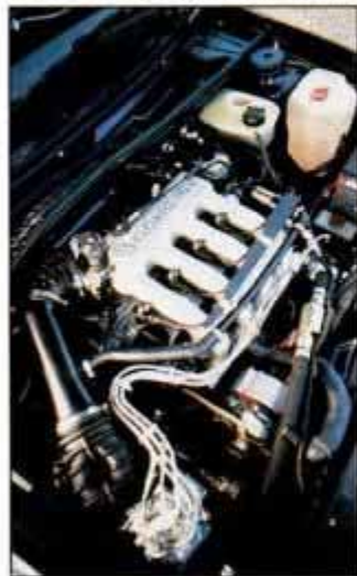
VW's 16V, seen mounted in the GTI, is a 1.8-liter handful.
