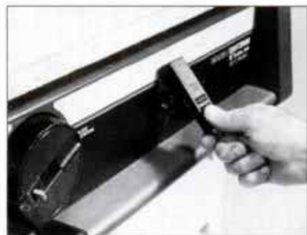
Quick-release clamps make it easy to change or reposition saw fence. Lift handles to release tension; push down to lock fence.
