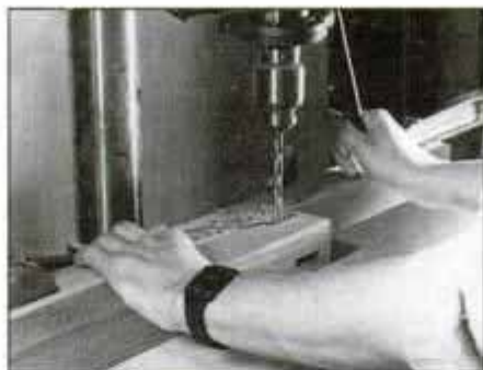
8 Clamp a fence to the drill press table and bore overlapping \frac{3}{8} -in.-dia. holes to rough out the mortises in each leg.
