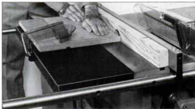
Router table bolts to saw table. Here, the saw fence is used to route a groove. Auxiliary wood fence comes with the router table.
