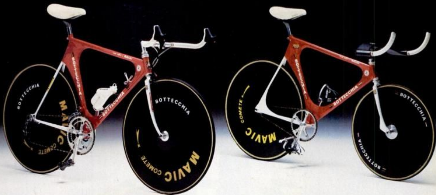
Bottecchia track bike (right) has fixed gearing, delta aero handlebar, webfoot frame gussets. Road racer (left) looks more familiar.
