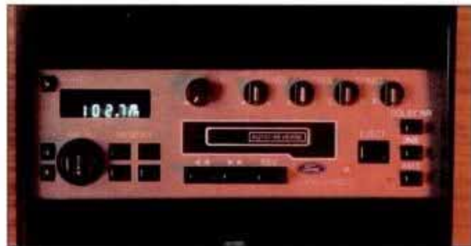
Ford radio/tape unit has electronic tuning, mechanical push-button tape controls, rotary bass, treble, balance, fader.
