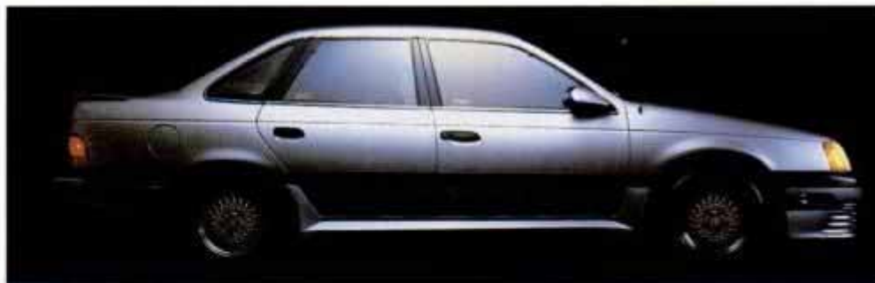
Kolb-Design Taurus features slick aero aids and uprated tires/wheels/suspension.
