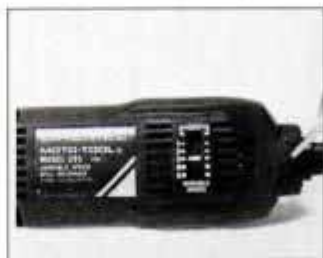
Conveniently located sliding switch allows speed selections between 5000 and 30,000 rpm.
