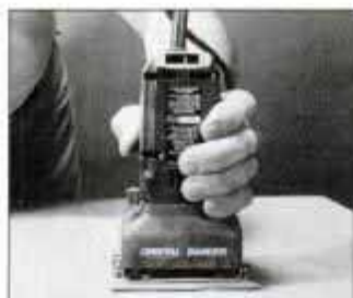
Palm-grip orbital sander uses 1/4 sheet of standard sandpaper. Orbit stroke is about 1/16-in. dia.
