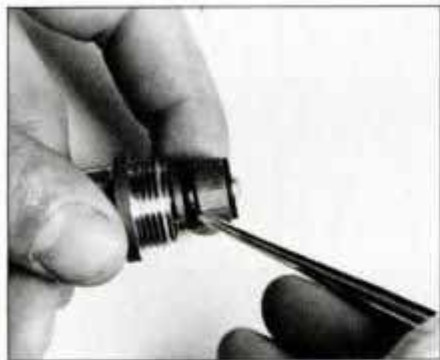
5 Carefully remove old O-ring from side of valve stem with awl or knife. Then replace with size recommended by manufacturer.
