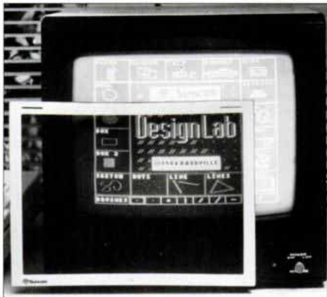
GlareDown mesh screen (foreground) protects your eyes from glare.
