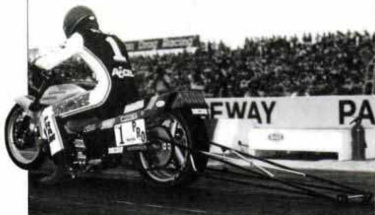
Wheelie bar keeps front wheel on pavement for 162-mph sprints.
