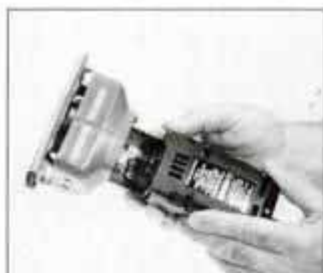
Slide motor onto tool and engage locking lever. The 1.6-lb. motor pack has a 6-ft. cord.
