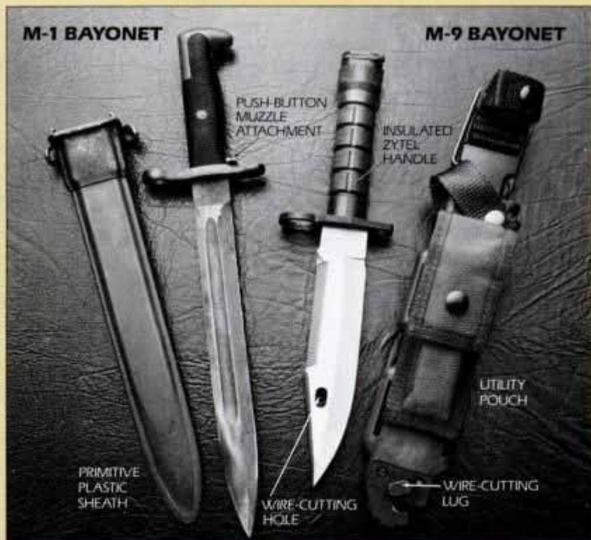
The M-1, developed in 1942 (left), is forebear to the Army's M-9 field tool (right).
