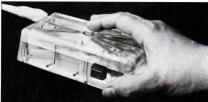
IBM's Braille computer card on control device can be read by feel.
