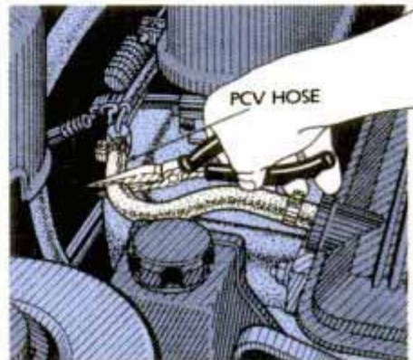
2 Squeezing off vacuum lines with pliers can isolate a suspect component. Use smooth-jawed pliers or cover with rag.
