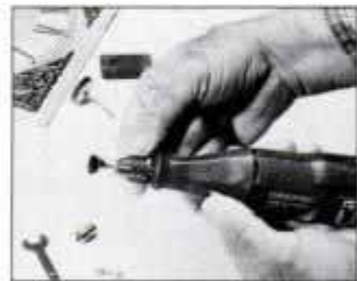
Keyless chuck makes bit changes quick. Chuck is available in kit or as an accessory.
