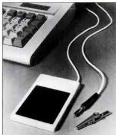
Touchpad drains away static charges.
