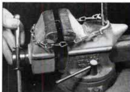
To form the handle, or bale, insert pipe in hole drilled in vise, hook chain on ends of bale, open vise jaws slowly to bend bale.
