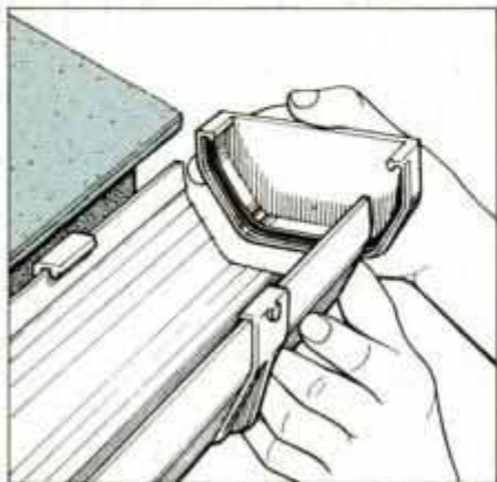
9 The high end of a gutter run doesn't require a drop outlet. In such a case, install an end cap with gasket over gutter.
