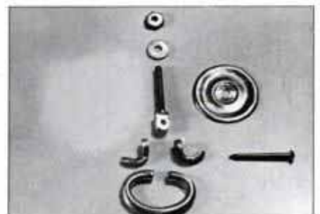
Here's the drop-ring pull prior to assembly. Solder the two comma-shaped parts to the ring. Attach ring to post with brass pin.
