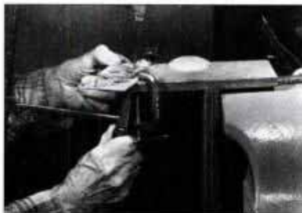
Glue a full-size template of the backplate to a brass piece. Cut out the plate using a jeweler's saw. File the edges smooth.
