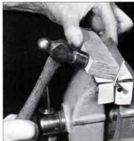
Clamp the tongue in vise with pin in position. Use a ball-peen hammer and wood block to bend the tongues around pin.
