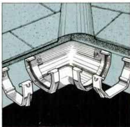
5 Attach a gutter bracket about 2 in. from each side of the inside corner to provide additional support of the gutter ends.
