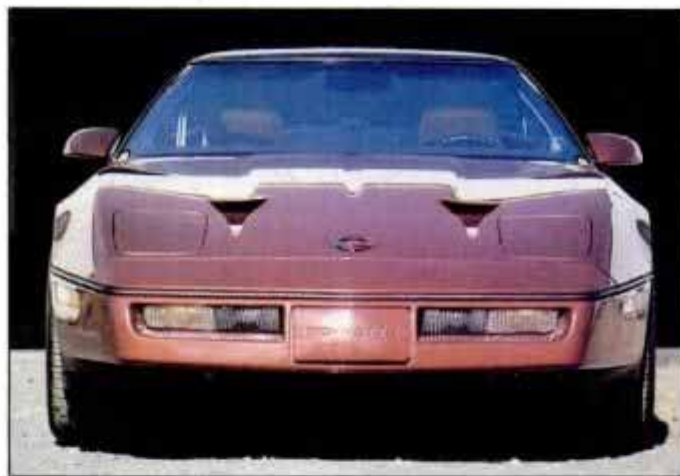
Twin NACA ducts feed directly to twin intercoolers.
