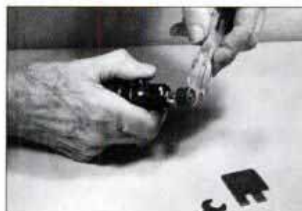
Smooth the rough-cut edges of the hasp with a Dremel tool fitted with a sanding drum. Wear safety goggles while sanding.
