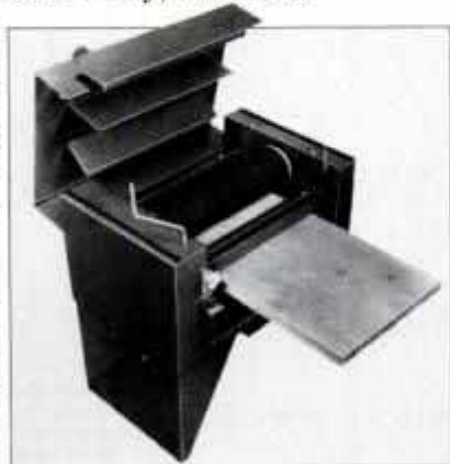
This automatic-feed 6-in.-dia. drum sander can surface boards up to 26 in. wide at a rate of about 11 feet per minute.
