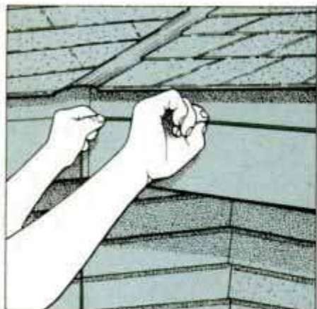
1 Snap a chalk line on the fascia. Be sure line slopes toward a downspout. Highest point of line is \frac{1}{4} in. below roof shingles.
