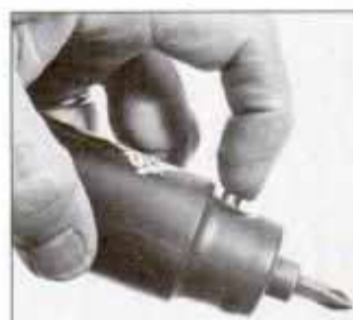
Engage the collet lock by pushing in the steel bar, as shown. Don't use the rocker switch while collet lock is engaged.
