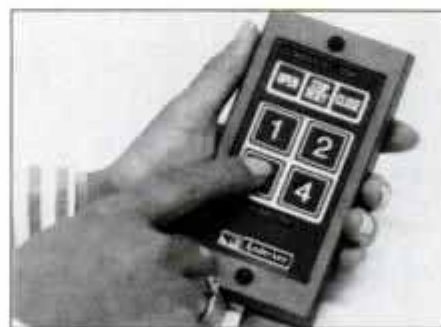
The command module allows windows to be opened or closed from anywhere in the room. It operates up to four windows.
