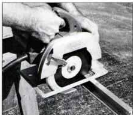
Cut all ferrous and nonferrous metals with an aluminum-oxide metal blade. Avoid side pressure that may shatter blade.
