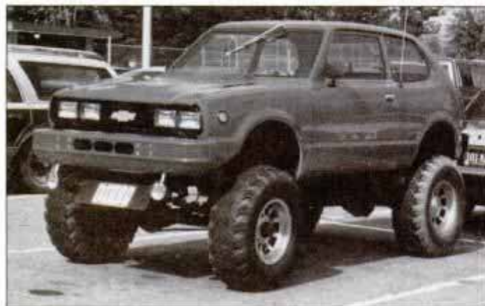
Honda 4x4 spotted in parking lot at GM Proving Grounds has Blazer chassis. Swing-away wheel gives access to rear (only) seat.
