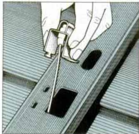
12 If an electrode wire assembly is faulty, and not the module, replace it. Begin by unscrewing the part and lifting it up.
