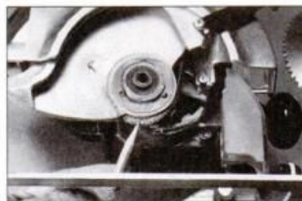
Remove blade and check spring on retractable guard for a buildup of resinous sawdust. Inspect and clean the spring periodically.
