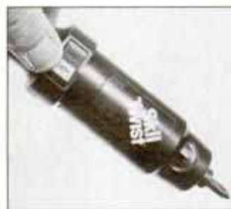
Rocker switch is reached easily by your thumb. Arrows on the switch indicate tool's forward and reverse rotation.
