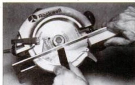
If your saw doesn't have an arbor lock, jam a wood block in the blade to keep the arbor from turning as you loosen arbor nut.
