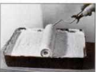
The tray is designed to accommodate a 9-in. roller. Use a high-quality, short-nap paint roller.
