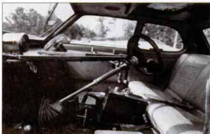
Honda 4x4 spotted in parking lot at GM Proving Grounds has Blazer chassis. Swing-away wheel gives access to rear (only) seat.
