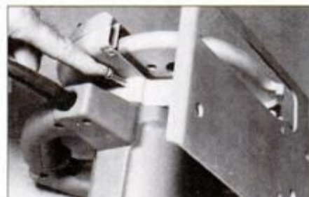
An arbor lock makes blade changing easy. Simply push in lock to keep arbor from spinning when removing arbor nut.
