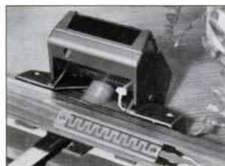
The rain sensor strip screws to the window-sill on the outside of the screen. It shuts a window if damped by rain.
