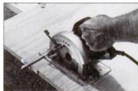
Most circular saws come with an accessory rip fence. Attach the T-shaped fence to the saw's shoe for making narrow rip cuts.
