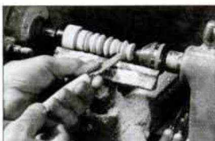
Narrow tool-steel cutting edge permits turning intricately shaped workpieces.
