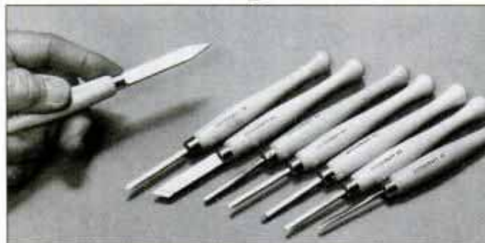
Turn small, highly detailed projects easily with this 8-piece miniature turning tools set. The tools are 7- and 7½-in long.
