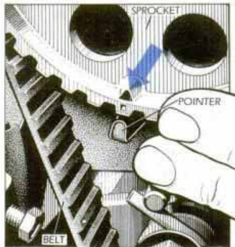
1 Turn the crank in the direction of normal rotation to align the timing marks.
