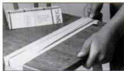
Try reusable stretch clamps to hold chairs (top) and other hard-to-clamp objects. Stretch and wrap for maximum pressure (above) then tuck underneath to hold.
