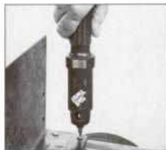
With the collet locked, use the Twist as a manual screwdriver to loosen a stubborn screw. Note hand position above switch.
