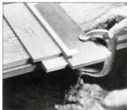
Use an offset block to position the guide. Flip back the hinged strip and align edge of the offset block with the cutting line.
