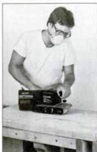
Automatic belt-tracking keeps the sanding belt aligned and reduces constant adjustments.
