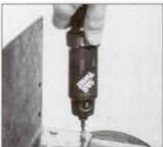
Once screw has loosened slightly, disengage the collet lock and press down the rocker switch to remove the screw.
