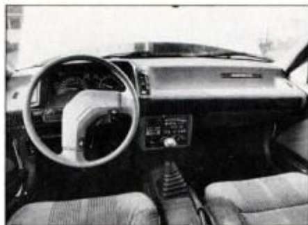
Derived from Cavalier drivetrain and suspension, car is noticeably wider inside.
