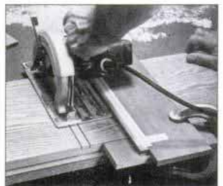
Make first cut with strip hinged back. Flip strip down and make next cut. Remove waste between kerfs with repeat-cuts.
