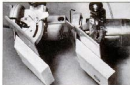
Often saw design, not size, dictates depth-of-cut capacity. When set at 45^\circ , this 7\frac{1}{4} -in. saw (left) cuts no deeper than 6\frac{1}{2} -in. saw.
