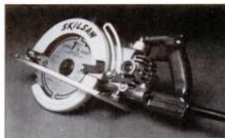
A worm-drive saw, distinguished by a long motor housing and rear-mounted handle, is the pro's choice for power and durability.
