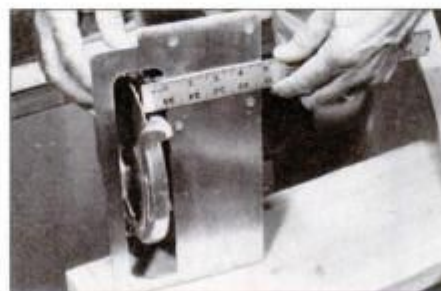
To determine where to clamp a straight-edge guide, first measure from an inward-facing tooth to the edge of the saw's shoe.
