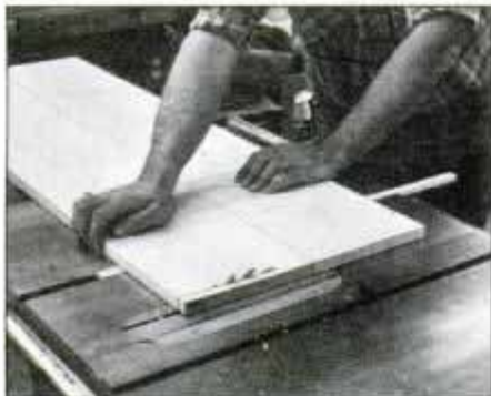
4 Crosscut panels on table saw. Tacknail a wood strip to bottom of panel. Strip rides in miter gauge slot in saw table to control cut.
