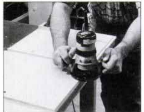
6 Rabbet rear inside edge of cabinet sides to accept plywood back. Rout rabbets with \frac{3}{8} -in. rabbeting bit with ball-bearing pilot.
