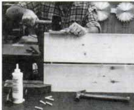
2 Spread glue in holes and on board edge. Insert dowel pins, tap two boards together using rubber mallet and wood block.
