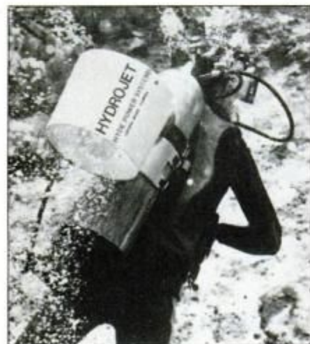
Underwater power from compressed air.
