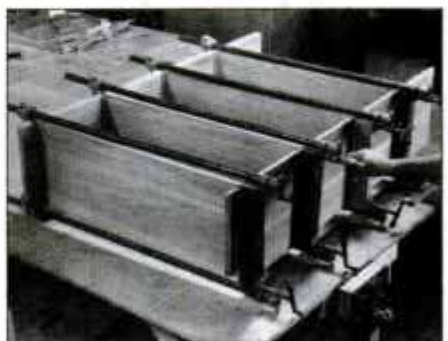
9 Assemble the cabinet with eight pipe clamps, as shown. Place cauls under clamp jaws to distribute even clamping pressure.
