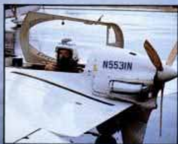
Test craft has a small, air-cooled Kawasaki 2-stroke engine. The next version will have a more powerful Rotax 532 engine.
