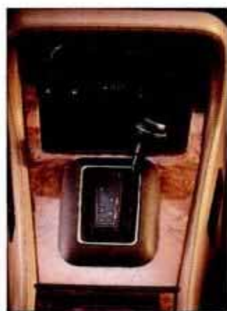
Jag's J-gate (on rh-drive car) lets you shift auto like manual.
