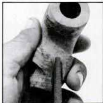
Fine-hone with a rattail file to remove machine markings.
