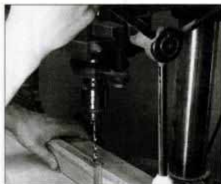
11 Bore overlapping \frac{1}{4} -in.-dia. holes in door rail to form mortise. Clamp auxiliary fence to drill press table to position work.
