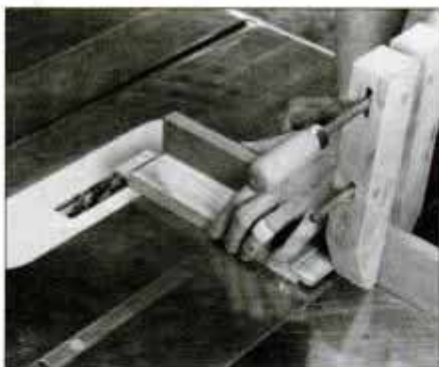
10 Cut tenon cheeks on table saw with a dado blade. Handscrew clamped to the miter gauge fence acts as a stop.
