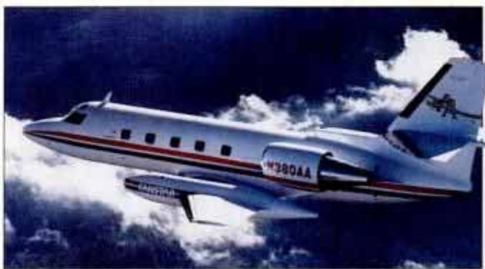
The FanStar was unveiled at the fall aviation show. It has gone to Mach .76 and has reached a 38,000-ft. ceiling in early testing.
