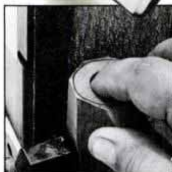
Use belt sander to trim the excess briar into rough contours.
