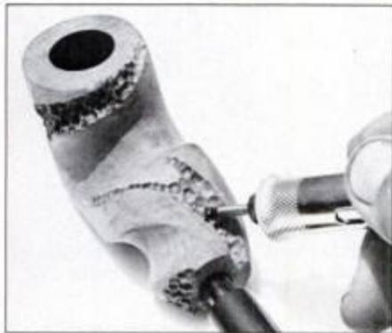
Carbide ball cutter bit makes decorative carving in grooves, masks flaws in briar.
