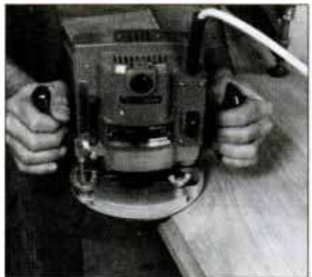
6 With cabinet top clamped upside-down, rout a decorative profile only in front and end edges with a \frac{1}{2} -in.-rad. cove bit.
