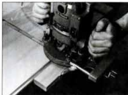
2 Rabbet the rear inside edge of cabinet sides and top to accept plywood back. Note edge-guide attachment on router.
