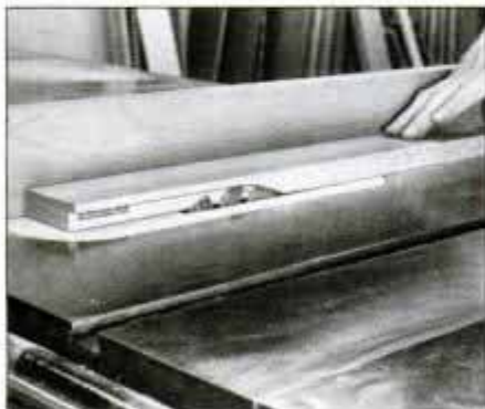
13 Use a dado blade and table saw to cut a \frac{1}{4} x \frac{1}{2} -in.-deep rabbet in each door rail and stile to accept the glass pane and stop.
