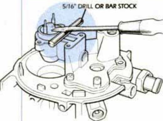
2 Use fulcrum for screwdriver to pry injector from GM throttle-body injector.
