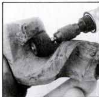
Cut contour grooves with the hand-gripping of the Dremel aids in heavy shaping.
