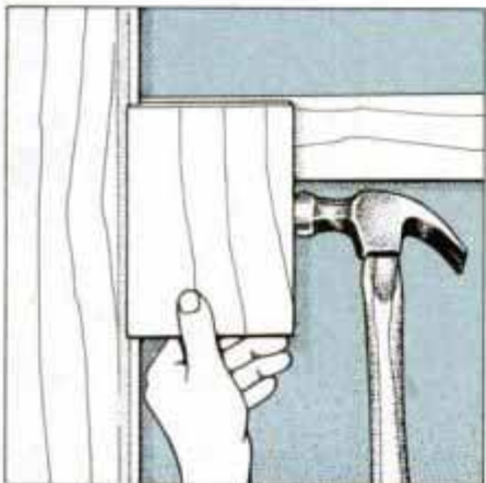
8 Hammer on a paneling scrap when you tap a board into place. Put the scrap's grooved edge over the board's tongue.
