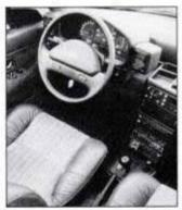
Instrument pod moves with the adjustable steering wheel.
