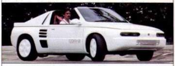
Isuzu COA-2 is mid-engine test bed with intercooled, dohc turbo.
