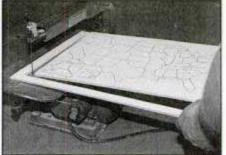
Bore a small-diameter hole in the corner of the map, insert the scroll saw blade and cut a 1/4-in.-wide border from the map.
