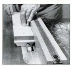
When a deep cut is made, workpiece can split easily. Avoid this dangerous situation by tack-nailing a backup board to the work.
