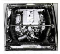
Four-valve heads, two knock sensors, intake runners tuned to two different torque peaks give 10 percent gain to 316 hp.
