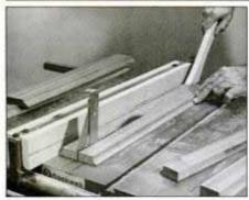
Cut a cove shape in both edges of two 4-in.wide boards. Then, rip the boards down the center to produce the rear frame members.
