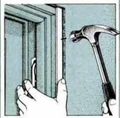
2 If jambs are recessed from the wall surface, glue and nall extension jambs in place. If jambs project, plane them flush.
