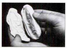
2 Mold (right) is shaped from undamaged area, then baked. Patch (left) is pressed into mold, removed, trimmed and baked.
