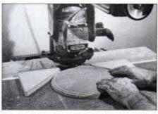
Use this 2-part jig to edge-shape circular workpieces. Triangular parts are nailed to strips that are clamped in fence channel.
