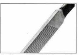
Many files are available with "safe" or uncut edges. This edge permits filing in tight spots without cutting into an adjoining surface.
