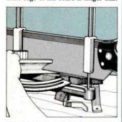
16 Outside corner on ceiling molding requires closed miters. Keep in mind that top of molding is held away from saw fence.
