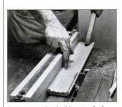
Replace cutterhead with a standard saw blade. Angle saw blade 45° and make rip cuts to produce finished crown molding.
