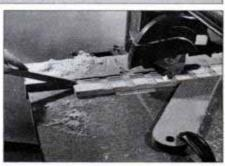
Molding cutterhead can also be used with radial-arm saw in the ripping position. Always feed work against knives' rotation.
