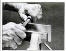
To draw file, use a single-cut bastard file. Hold it level and perpendicular to the surface. Push and pull the file along the workpiece.
