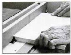
Execute an inboard cut when shaping only a portion of an edge. Guide the workpiece slowly against the auxiliary wood fence.
