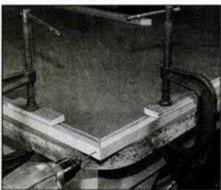
Clamp the frame parts together and bore pilot holes for 4d finishing nails. Locate the holes so the nails don't hit each other.
