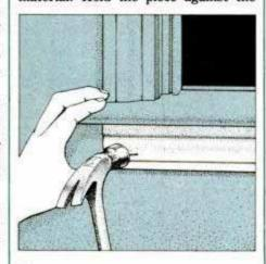
9 Nall the finished apron under the sill. Note that ends of apron should align with outside edge of both side casing boards.
