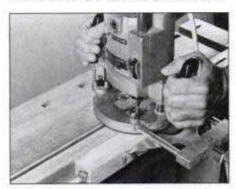
5 Cut legs to size, then using router and guide, cut stopped groove in each leg. Groove accepts side rails and panels.
