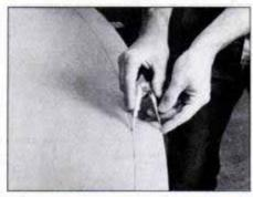
3 Using a scriber or compass, trace a line on the second panel 2 in. in from the perimeter. Cut out the interior waste.
