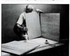
6 Apply glue to the dadoes in the front and end panels and to the edges of the base panel. Then, slide the base in place.
