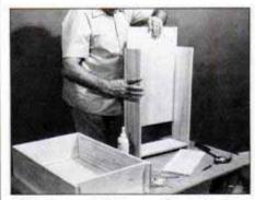
13 To assemble drawers, first join sides to back with glue and nails. Then, slide in bottom—without glue—and attach front.
