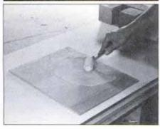
10 When veneer is ready, cut core panel to size. Then, roll glue over surface of panel. Do not apply glue to the veneer.
