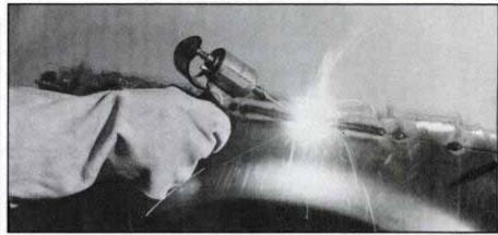
Most arc welders have been designed for joining ¼" metal; our stitch welder attachment controls welding heat to produce smooth, even welds on body panels — limits distortion and burn-through.
