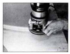
4 Glue and clamp the top and support band together. Using a router, cut a 3/16-in. chamfer around the top and bottom.
