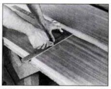
8 To cut veneer to length, score the sheet with a utility knife and straightedge guide. Lift sheet to separate.
