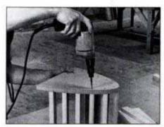
7 Counterbore screw clearance holes, then join both leg caps to the stave ends using glue and 2-in. No. 8 fh screws.
