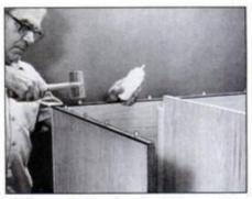
9 Glue and drive dowels before applying glue to entire edge. This yields more working time before glue dries.
