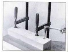
5 To join bottom panel to legs, first clamp parts together. Then, drive lagscrews through mating corner blocks.
