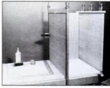
7 Glue and install the partition panel, then join the assembly with bar clamps. Be sure to check the assembly for square.
