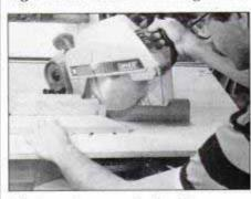
14 Cut miters on ends of top frame members using a miter box or table saw. Make precise cuts for tight joints.
