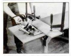
1 Cut the mitered ends of the top and leg panels using a circular saw and straightedge guide. Make a test cut in scrap first.
