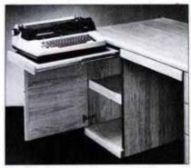
a manual machine. Additional storage space is available under the lower platform of the desk. The door of the typewriter compartment is made to resemble the right-hand drawer fronts and is hung with easy-to-install, self-closing, concealed hinges. Due to the moderate pressure required to operate the door and drawers, no pulls were needed. This preserved the desk's clean, contemporary lines.
