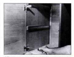
18 Attach mounting blocks to the side panel and hinges to the door. Then, slide hinges onto blocks and tighten screws.
