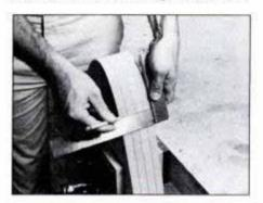
6 Sand all edges smooth. Then, using our drawing as a guide, lay out the position of pedestal staves on edges of leg caps.
