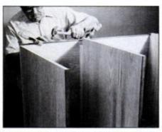
8 Once both pedestals are joined to the front, glue and nail the walnut strips to the top edge of the front and side panels.
