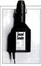
Sound Sender plugs into car lighter, sends sound to radio.
