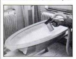
11 Spray paint onto table using smooth, even strokes. Hold gun 8 to 10 in. off surface and keep it moving at all times.
