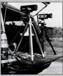
X- and K-band radar guns were clamped to tripods and used alternately to assure consistent performance during tests.
