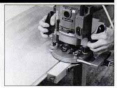
3 Using a router and edge guide, cut a ¼ × ½-in. rabbet—for the case back—along the back edge of the bottom panel.
