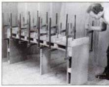
7 Support bottom panel with temporary brace, then glue and clamp top panel in place. Use cauls to distribute pressure.
