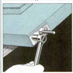
9 Attach hanger brackets to door with hanger bolt temporarily in place. Make sure the bolt is free to slide out.
