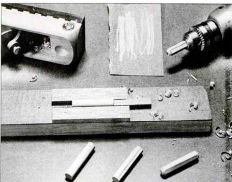
Here's how to make dowel pins from standard dowel rod. Plane two flat areas on each dowel to allow air and excess glue to escape as clamping pressure is applied. Make this simple jig to hold the dowel. Then, spin dowel in drill on sandpaper to form chamfer.
