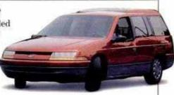
Removable panels convert TSX-6 into a pickup with side glass.
