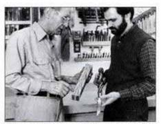
Glewwe (left) shows author the laminated blank he uses for turning chisel handles. Blank is comprised of several different wood species. Author examines a finished handle.
