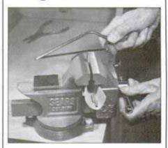
When working on small items in a vise. keep them from dropping to the benchtop or floor when the jaws are loosened. Install a catch-all trough-a strip of cardboard, springy sheetmetal or other pliable material—in the space beneath the jaws. Cut the strip somewhat wider than the space between the jaw arms when the jaws are nearly closed. Position the strip so that closing the jaws on a workpiece bends the strip into a trough.-Walter E. Burton
