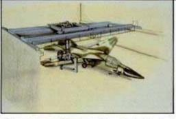
will sweep an airframe with X-rays and neutron radiography. As the plane sits under a rolling canopy, Xray and neutron beam "cameras" move along its surface, stopping at preprogrammed points to take an image. These are fed to a mainframe computer that assembles images of the subskin. It can even "zoom in" on areas just inches across for closeups of what is inside the honeycomb structure of composite airframe skin. The testing device will be operational by the early 1990s.
