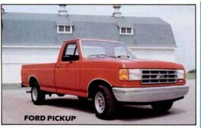
lines. Styling is new inside and out, but more important is the new braking system. Ford will have ABS brakes on the rear wheels of all its 1987 full-size pickups and Broncos, a first for lightduty trucks.
