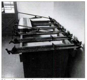
Salvaged from a casket factory's clamping machine, these clamps are used to edge-glue boards and to laminate turning blanks. Long bars have flat metal shoes that apply downward pressure.
