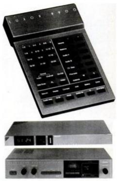
Remote control (top) operates Luxor 9900 CKu receiver/actuator (bottom). Blockdown-conversion allows use of Luxor 9500 (center) as slave receiver.
