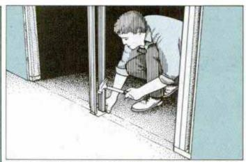
5 Snap chalkline between ends of bottom plates, then slide top of split Jamb onto the door track. Center bottom of split Jamb between lines. Check plumb with level and nail to floor.
