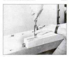
6 After the ¾-in.-deep holes have been bored, use a sharp chisel to cut the mortises square and to clean out remaining waste.
