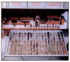
Turning tools storage rack is situated directly over lathe. Note custom-made handles.
