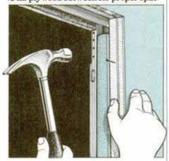
13 Nail door stop to both sides of split jamb and door track. Split jamb flange has slots so nails can reach wood strips behind.
