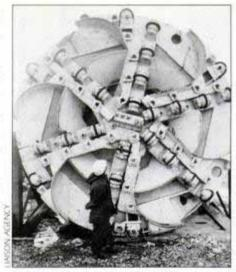
The cutter head on the Robbins machine features replaceable ceramic "teeth."
