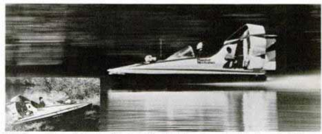
Tri-Flyer You grab the joystick, twist the throttle grip and suddenly you're flying at speeds over 75 mph on land or water. That's PM's latest high-tech hovercraft, propelled by a 65-hp snowmobile engine that powers a four-bladed fan. Lift comes from a 10-hp mower engine that carries you and two passengers over obstacles and up hills. Plans include six blueprint-size sheets and a 60-page instruction booklet with drawings, photos and building tips. (PL-1805-\$19.95)
