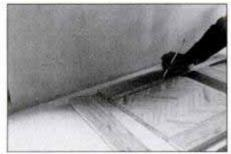
Lay out position of holes for the dowels that will be used to join the patterned inset to the top border pieces.
