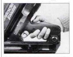
Closeup view shows fan switch on top of the handle and the trigger located underneath. Note how the nail load is clearly visible.
