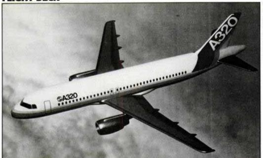
The A320 airliner of the 1990s will have servocontrols run in a fly-by-wire scheme. The cockpit will be able to fly the plane, with the pilot just keeping an eye on the video displays.
