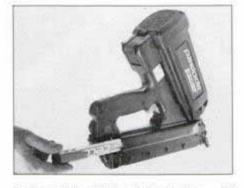
Rechargeable nickel-cadmium battery will drive about 4000 nails. Tool's red light warns when battery charge is getting low.
