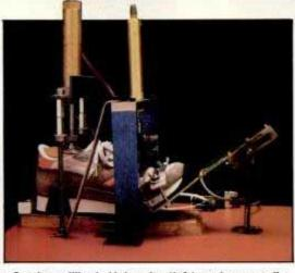
Testers from the Biomechanics Lab at Southern Illinois University (left) evaluate mediolateral control and shock absorption in one athletic shoe design. The science of designing athletic footwear is controlling, but not inhibiting, natural foot function as shown in diagrams on facing page. A Converse shoe (right) is mechanically tested for wear and flex.
