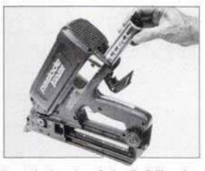
Insert hydrocarbon fuel cell. Cell's valve, acting like a carburetor, injects a precise amount of fuel at start of each cycle.
