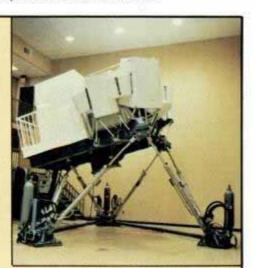
Flightsafety's Bell 222 helicopter simulator sits on top of a system of hydraulic jacks. The hydraulic system gives the cabin pitch, roll, yaw and lift that feels like flying to the student inside.
