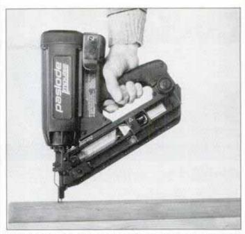
Cordless, airless nailer is powered by a patented linear combustion motor that operates off a disposable fuel cell and a battery.
