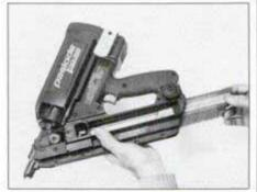
Loading nail strips into the magazine is quick and easy. A spring-tensioned follower bar advances the nails after each shot.
