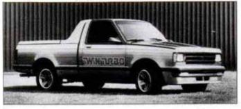
Chevy's Twin Turbo has a pair of blowers piped into V6 pienum.
