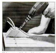
Make a wood-block guide to bore angled holes. Align centerlines on block with hole centers to position the bit accurately.
