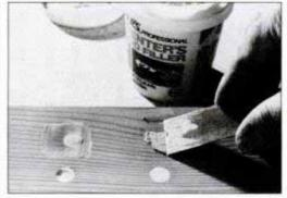
Slightly overfill holes and then sand or shape the filler flush, as at right, front and back. Otherwise filler will shrink as it dries, left front.
