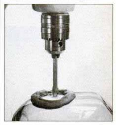
Drill glass with this carbide-tipped bit. Make a dam of putty or modeling clay to form a reservoir for the kerosene lubricant.
