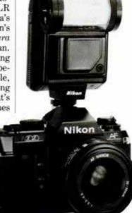
it with the optional TC-16A teleconverter to get autofocus operation from 30 manual-focus Nikon lenses. Moreover, the N2020 provides "focus assist" with 60 conventional Nikon lenses. Though you'll rotate the focusing ring manually, flashing red arrows in the N2020's viewfinder show you which way to turn for perfect focus. A green light and an audible beep tell you when you're on target.
