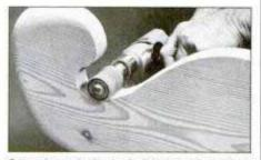
Smooth and shape inside curves with a sanding drum. Advance the drum against its rotation for the most aggressive cutting.
