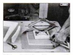
24 An auto jack is used to compress the seat cushion before stapling the fabric. The 2x4 is braced against a ceiling joist.
