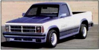
for appearance only. Remember that off road, wheels will get muddy. Pick a design that's easy to clean. If you're going for a larger wheel/tire combination, the wheel offset is critical. Taller tires require a negative offset to widen the track of the truck. Too much negative offset, however, puts additional stress and wear on the spindles and suspension.
