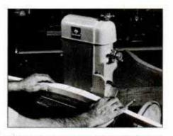
**11** Sand flat the area where the side rails join the legs. Be sure that the sander's table is perpendicular to the sanding belt.
