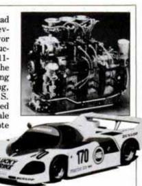
Mazda 757 LeMans entry has a unique 3-rotor Wankel engine (top) rated at 444 hp.
