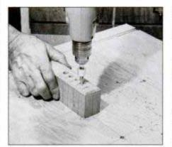
Make this simple guide to bore holes square to the work surface. Bore several holes in guide to accept different diameter bits.
