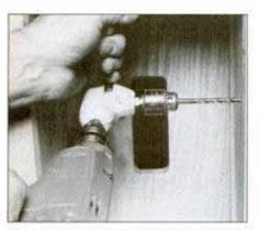
A right-angle drive head permits working in confined areas. The gear ratio is 1:1, so there is no change in the tool's rpm.
