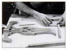
**15** Bore holes in the rung's ends and insert dowel centers. Transfer hole positions to the legs using a guide block.
