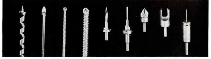
Here are some not-so-typical, but very useful, bits (left to right): screw-point hollow spiral, carbide-tipped glass bit, carbide-tipped
