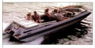
Heim station is farther forward on the Harris FlotDeck, which means a smaller bow rider area but correspondingly larger aft deck.
