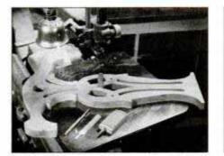
5 A file in lower blade clamp of scroll saw smooths away saw-blade marks. Tapered file tangs must be ground straight.
