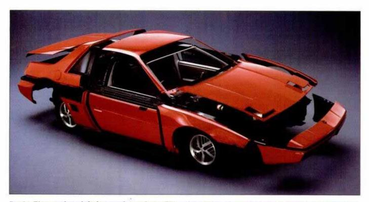
Pontiac Fiero panels are bolted to a steel space frame. This makes it cheaper to change styling and replace damaged panels.
