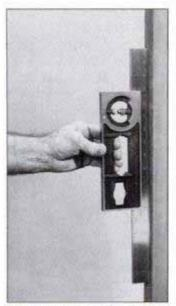
The 18-in.-long rule folds for easy storage and for use as a straightedge. Here, the level is used to determine plumb.
