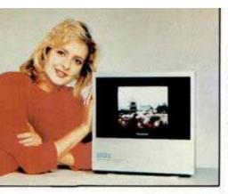
Flat, wall-mountable TV is still in development. Panasonic/Matsushita prototype (left and below) uses conventional cathode ray tube (CRT). Other experimental flat TVs use liquid-crystal displays to create image.
