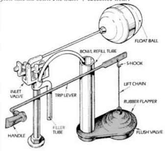
Excess slack in the lift chain, a worn flapper valve or a stretched Shook can cause poor flushing action in a tollet.
