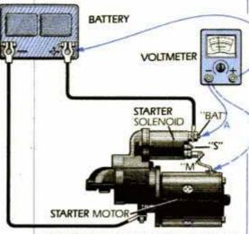
1 To check resistance on starters with external solenoids, connect meter as shown.
