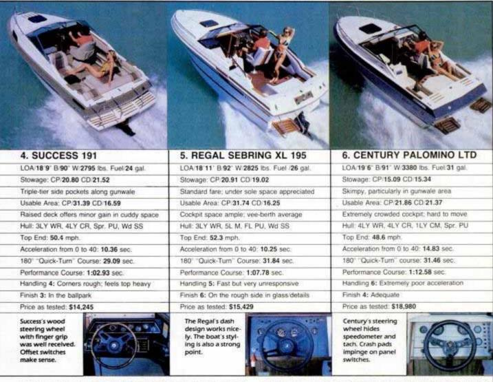
subjective ranking, plus comments, of steering ability and speed in a variety of wind and sea states. 8. Finish is a subjective ranking, plus comments, of glasswork and detailing in addition to an evaluation of how well components
