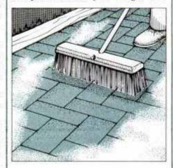
14 Once bricks are installed, spread sand over them and sweep to drive sand between cracks. Then, spray with water.
