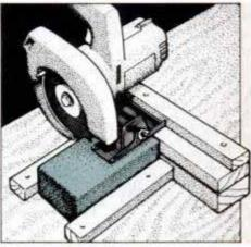
13 For cleanest cuts, use masonry blade in saw. Build jig from 2x4, 1x4 and 1x2 stock nailed to surface of plywood panel.
