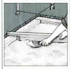
10 Rest screed on beams and move back and forth to smooth sand. Remove high areas with trowel, add sand to low areas.
