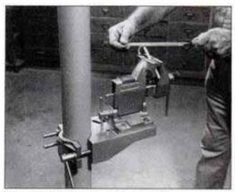
The holes in the tabletop make it easy to secure a vise or compact power tool. Table rotates 360°.
