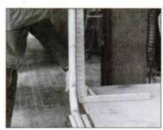
6 After bending top corner in back pole, clamp pole in vise so it's square to bench top. Then make sideways bend.
