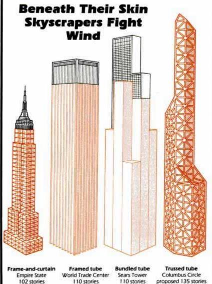
Ask an architect to define a skyscraper, and he will say it's any building with a height/width ratio greater than 7-to-1. But ask a structural engineer, and he'll tell you a skyscraper is any building whose major load is due to the wind. Architects work at drawing boards on dreams. But engineers have to deal with the real world, and their definition is perhaps more useful.
