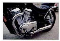
V-twin is a true 45°, uses 4-valve layout.
