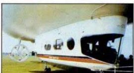
The Fuji airship (top) is a Britishmade vessel designed as a camera platform. Pan Am and others have used the Skyship 600 (above) with ducted-fan engines. It carries passengers on tours over European cities. Gondola (left) is of Keviar. Another artist's concept (below) shows an airship as a radar platform. Goodyear is working on an antisubmarine blimp.
