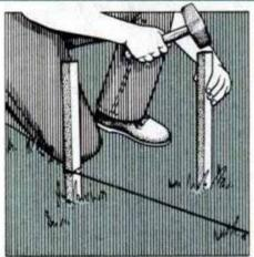
2 Drive stakes for adjacent sides at corners of patio. Hang string on stakes and, again, level it in place using line level.
