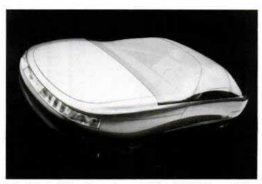
Ford Probe V has a lower drag coefficient (0.137) than an F-15.
