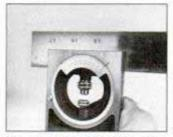
One side of the adjustable turret has double graduations from 0 to 90°. Adjust rule to desired angle, tighten knurled knob.
