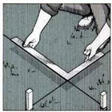
3 After all stakes and strings are in place, check each corner for square using framing square or by comparing diagonal measure.
