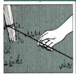
1 Lay out patio side nearest house first. Drive stake 1 ft. past both ends, then attach string and level it using line level.
