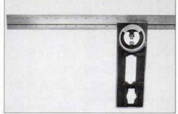
Versatile shop tool is seven tools in one. Features include adjustable, double-graduated turret, 1½ x 18-in.-long steel rule and four levels.
