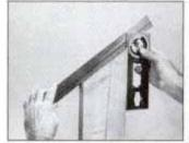
Adjustable turret makes it easy to determine, transfer and mark angles—a real timesaver when cutting hip and valley rafters.
