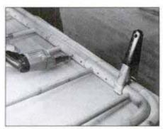
16 Clamp inner crest pole and back rail assembly to outer crest pole. Bore clearance holes and attach with screws.
