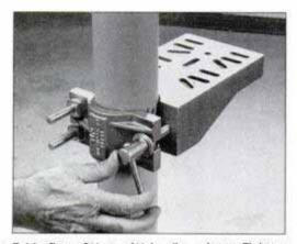
Table fits a 2½- to 4½-in.-dia. column. Tighten clamp handle to secure table at desired height.
