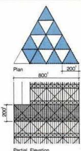
Roth's more than mile-high structure (top) consists of 16 steel frame tubes bundled into an 800-foot equilateral triangle (middle). The tubes are staggered, creating shafts of open space for atriums. Diagonal steel beams (bottom) combined with the triangular tubes are the most efficient structure for resisting wind loads on skyscrapers.
