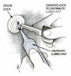
lubricant recommended for lock cylinders. A variety of these are sold in hardware and home supply stores. One mentioned by GM is sold under the brand name Lock-Ease.
