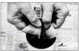
When cleaning a brush, free stubborn particles by working the solvent into the base of the bristles with your fingers.
