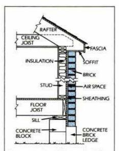
In a conventional house, insulation is hung on the frame within the outer and inner walls. Mason's foam serves as both wall and insulation.
