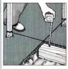
5 Lay timber within perimeter of excavation. Then measure to string to determine depth of trench required under beam.
