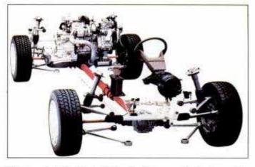
The chassis of the future (above) will have a 4-wheel-steering system that will improve high-speed handling and allow the driver to slip out of tight spaces. Computers (left) have replaced drafting boards in automobile design studios.
