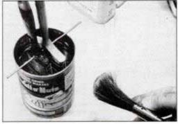
A soaking brush will be deformed if it rests on its bristles (right). Bore a hole through its handle and hang it from a rod.
