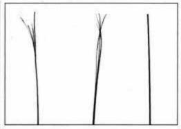
A closeup view of various bristles, left to right: naturally flagged hog hair, machine-flagged nylon and a low-grade blunt nylon.
