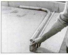
**5** Clamp board on edge of work surface, then butt bent pole against it. This gives accurate surface for measuring length.
