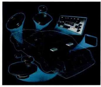
Phantom view shows placement of head unit, amp and speakers.
