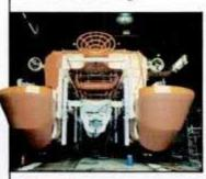
SUPRA, a German seagoing prototype is a robot, a minisubmarine, a diver's workshop and an underwater derrick. By remote control or with a crew of two, it can perform heavy underwater jobs, lifting up to 20 tons, that until now required surface ships. For pipeline laying and repair, SUPRA's claws (below) will make quicker, better work beneath troubled seas.
