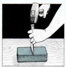
12 Cut brick to size using brick chisel and maul. Score cut line on all four sides of brick, then strike with maul to break.
