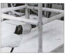
11 Test-fit butt joints then apply glue and attach parts with fh screws. Bore pilot holes and stagger screws.
