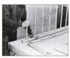
14 Apply glue to spindle holes in back rail, then slide spindles in place. Glue this assembly into holes in inner crest rail.
