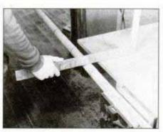
**2** Use workbench to check progress when straightening poles. Pole should align with surface and be parallel to edge.
