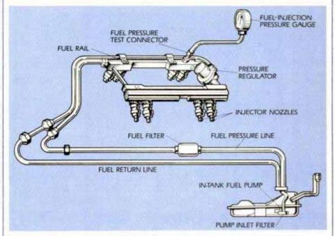
While excess fuel is a common cause of 7 To check for leaking fuel-injector nozzles, attach pressure gauge to Schrader valve.
