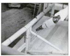
18 Scribe loveseat cross braces in place between front and rear center legs. Attach with screws driven at a slight angle.
