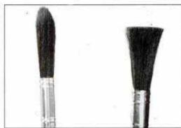
A quality brush, left, has a chisel tip that allows more bristles to contact the work than the economy, blunt-tip brush, right.
