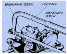
3 Remove carb from engine if necessary to cut slots in choke housing screws.
