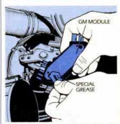
6 Dielectric grease on the back of GM ignition modules can prevent heat damage.
