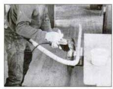
3 To bend pole, clamp in vise 2 in. from point of bend. Apply water and heat until pole softens, then bend to shape.
