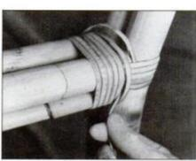
25 Tie off cane at armrest and leg by sliding end under whole row of cane strips and last turn of finish wrap. Cut end flush.
