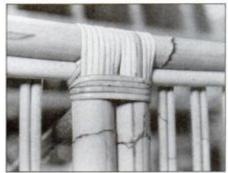
22 Apply glue to bottom edge of strips, then cover with continuous piece of cane. Wrap until all ends are hidden.
