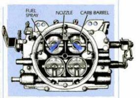
5 Fuel should spray from accelerator pump nozzles when throttle is opened manually.
