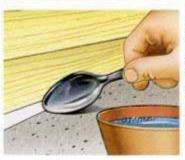
The trick to getting a smooth bead is to tool over the fresh sealant with an old spoon dipped in a soap solution.
