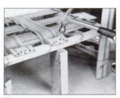
26 Attach ends of webbing to seat rails with tacks. Double-over end and support rail with block when hammering.
