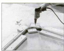
4 After first pole of given profile is bent, screw blocks around edges to create jig for testing other poles of same shape.
