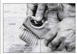
Use a brush comb during cleaning and before hanging it up to dry. It separates bristles for solvent access and aligns them for drying.
