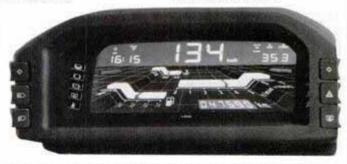
LCD dash combines graphic perspective and digital readouts.
