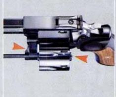
The Ruger cylinder locking system represents a successful mechanical engineering solution to the problem of positive cylinder locking. The Ruger cylinder is locked to the frame by a strong pilot bearing at the rear of the cylinder, and by a sturdy locking bolt at the front of the crane which engages a matching slot at the front of the frame.
