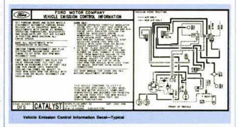
4 Decal in engine compartment shows vacuum hose routing and spark advance specs.
