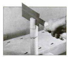
7 Cut 2-in.-deep splice joint in end of one pole using hacksaw or fine-toothed Japanese ryoba saw. Keep cut square to end.
