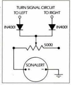
GM flasher (part Simple circuit features an adjustment for No. 10041073) fills volume level of turn-signal flashes.
