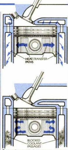
2 Heat flows easily from piston to coolant in normal cooling system (top). In clogged system, piston can expand enough to drag.
