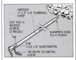
to one end of the wood to form an eve. and shape the other end to a point. To use the "needle," tie one end of the rope to the eye and push it under the pile of brush. Remove the needle, loop one rope end and pass the free end through the loop. Attach the free end of the rope to a garden tractor for towing.
