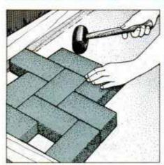
11 Begin laying brick in one corner. Work from plywood panel, and use rubber mallet to adjust brick alignment.
