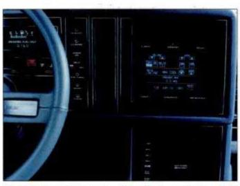
Touch-sensitive CRT tunes radio, adjusts a/c, monitors trip.
