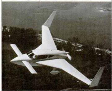
The Velocity cruises at over 200 mph with a 2000-mile range.
