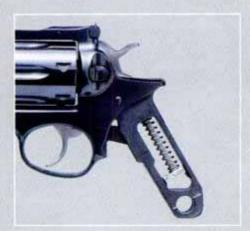
The grip portion of the Ruger GP-100 revolver unlike the conventional skeleton type grip frame has been designed to incorporate a variety of functions. It houses the mainspring seat, trigger guard latch, and grip panel locator. The design of this unique frame extension also permits the installation of customized wrap-around grip panels in a variety of shapes and sizes to suit the tastes of the individual owner.
