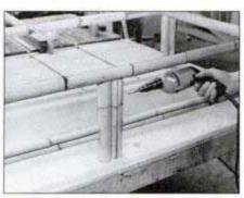
17 Center leg on loveseat is made of two assemblies. Stretchers must be attached to single legs before legs are joined.
