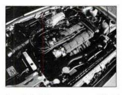
Integra's 4-cylinder engine uses traditional dual camshafts to work its 16 valves.
