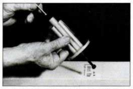
Hold the Molly upside down and then "load" it by sliding a drive pin into its barrel. The tool holds the pin upright as it's driven.
