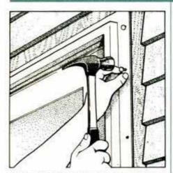
9 Check door frame for square, plumb and level. Attach by nalling through perimeter flange with galvanized roofing nails.
