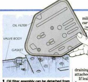
Oil filter assembly can be detached from valve body by removing two screws.
