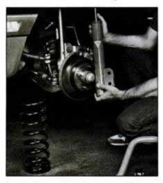
Gas shocks, special springs and stiffer sway bars are all part of Koni suspension kit developed specially for Thunderbirds.
