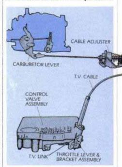
3 Pressing a tab on cable adjuster of some GM models will adjust the T.V. cable.
