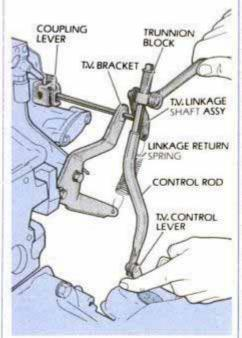
Front-drive Ford T.V. linkage is adjusted after loosening trunnion block bolt.
