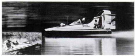
**Tri-Flyer** You grab the joystick, twist the throttle grip and suddenly you're flying at speeds over 75 mph on land or water. That's PM's latest high-tech hovercraft, propelled by a 65-hp snowmobile engine that powers a four-bladed fan. Lift comes from a 10-hp mower engine that carries you and two passengers over obstacles and up hills. Plans include six blueprint-size sheets and a 60-page instruction booklet with drawings, photos and building tips. (PL-1805—\$19.95)
