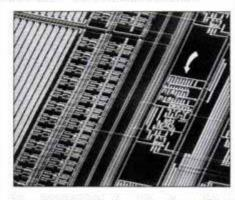
Magnified TV chip shows filter (arrow) that will improve signal from satellite dish.
