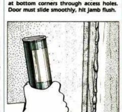
12 Working from inside, install insulation around perimeter of new door frame. We sprayed in aeresol foam insulation.
