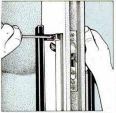
14 Inside and outside door pulls are attached with same two machine screws. Screws slide through prebored holes.
