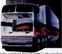
and a constant line of sight to the trailer sides when turning. The driver also rides on the trailer suspension, which may be more comfortable than that of the tractor.
