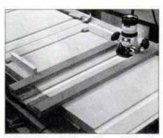
2 Rout the dadoes with a ¾-in,-dia. straight bit and a straightedge guide. Note that identical-length wood blocks keep guide parallel to previously routed dado.
