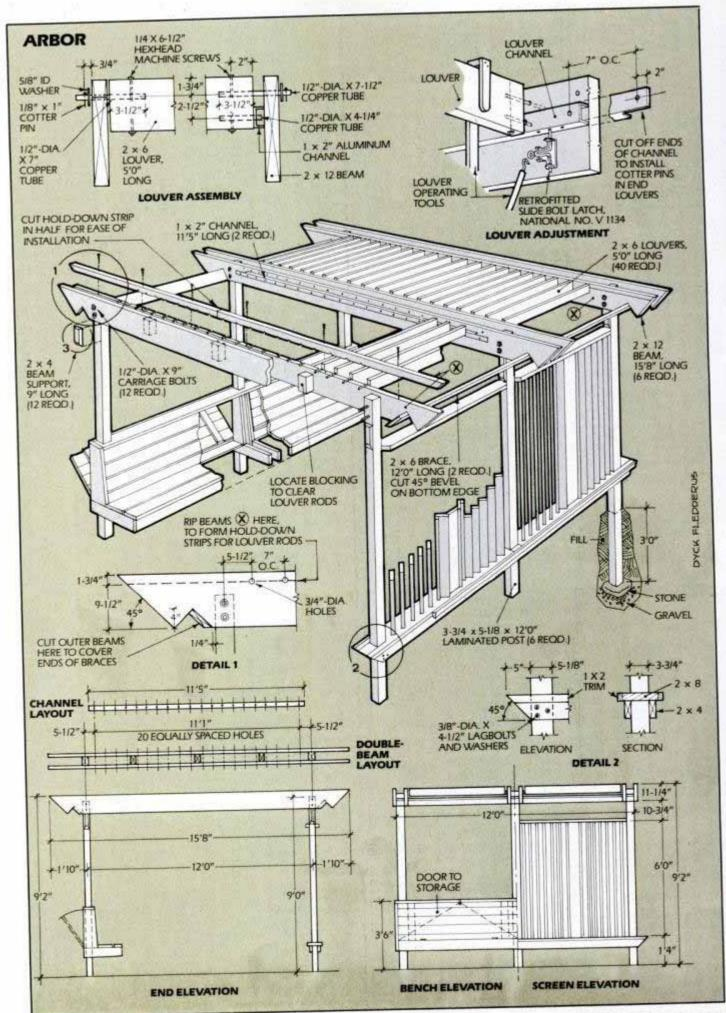
through. Add to this the built-in seating benches—which include storage for garden hose, small lawn care equipment and the tools to operate the louvers—and we hope you'll agree that this is something new that does work better. Following are directions for building this innovative structure.
