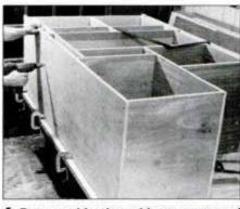
6 Dry-assemble the cabinets on top of their respective back panels. Then, bore screw holes. Before disassembly, outline the shelves and dividers onto back.
