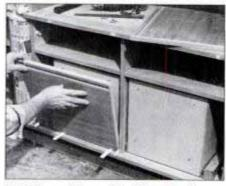
15 Drive 1-in. nails through drawer fronts so points protrude 1/8 in. Press drawer face against points to make marks. Apply glue, realign marks and drive nails.
