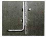
Close-up shows how driven fastener (upper) expands. Lower fastener is ready to be shot.
