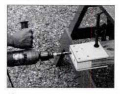
10 Construct hole-boring jig as shown on drawing then clamp over ends of louver boards and bore holes for copper tubing.
