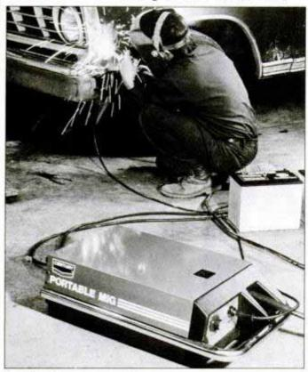
Portable MIG wire-feed welder runs on two 12-volt car batteries.
