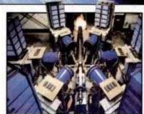
Checmate Railgun (above) zaps enemy spacecraft or can stop a missile as it is launched. Operating model (left) at Maxwell Laboratories in California tests this kinetic energy weapon. Concept (below) is to charge projectile with electrical power as it speeds out of railgun.
