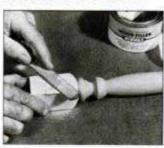
3 Use a file to remove most of the excess filler. Then, sand the filler flush with the wood.
