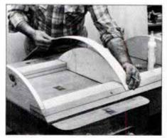
19 Use a 2-in. strip of 1/8-in. poplar plywood to determine correct width of the plywood needed to cover end columns. Attach plywood with glue and 1-in. nails.
