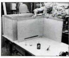
8 Assemble cabinets with slow-setting hide glue. Start with bottom and work toward top. Place wax paper under joints to shield against glue squeeze-out.
