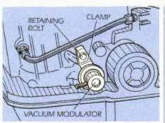
6 Vacuum modulator is located on the transmission case, above the pan flange.
