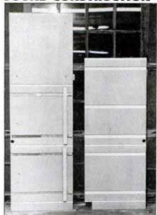
4 Cabinet side at left has door tracks and follower bars installed. Panel on right will receive five tracks. Wall unit's four large doors require three sliding tracks each.
