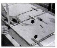
3 Install sliding door tracks flush with front edge of cabinets' sides. Then, screw a hardwood follower bar to the brackets (arrows) so tracks work in unison.
