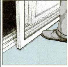
4 Grip fixed panel with both hands and lift up into top track until bottom clears lip on lower track. Pull out door bottom.
