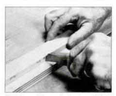
1 Make a story pole from a straight length of ½ × 1½-in.-wide pine. Mark the pole with various dimensions, then transfer marks to the workpiece using a knife.
