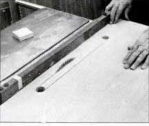
5 Airflow vents are necessary to prevent the electronic components from overheating. Bore two holes, then elevate the blade through shelf to cut out the waste.
