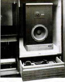
Foam below speaker centers it in cavity for cutout in baffle board (not shown).
