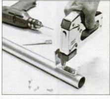
Snap-on accessory allows driving expanding fasteners quickly with a staple gun. Here, a bracket is secured to metal tubing.
