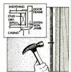
13 Nail extension jambs to door jambs so frame is flush with wall surface. Set and fill nail holes, then nail on casing boards.
