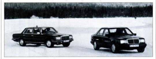
Car with 4MATIC (right) tracks safely around an icy turn while rear-drive car begins to spin out.
