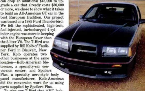
Spoilers Plus bodywork (above and at right) includes a deep chin spoller to direct air up to the turbo intercooler, Lexan headlight covers to improve aerodynamics at the racetrack, a distinctive grille and fascia assembly and a smart rear spoller. Together, the new parts give the PM Thunderbird a one-of-akind custom look.
