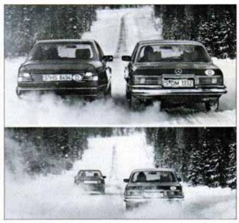
Car with traction control out-drags wheel-spinning competitor.
