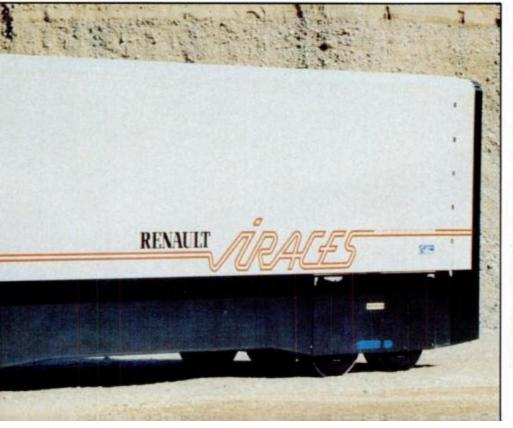
to sweep away air that could create turbulence under the cab and trailer.
