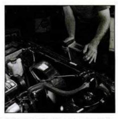
Aluminum heat exchanger portion of the intercooler kit bolts into grille opening, where cooling airflow is strongest.
