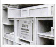
18 The completed cabinets are screwed together and ready for finishing. A cardboard carton, the same size as the TV, is used when cutting and fitting the grilles.
