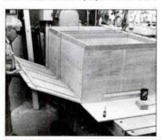
9 Install the cabinets' sides last. But first, be certain that all the sliding door tracks, follower bars and hinge-mounting blocks are attached and working properly.
