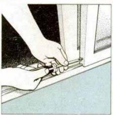
2 Loosen screw that holds plastic alignment bracket on bottom corner of fixed door. Slide bracket away from sill track.
