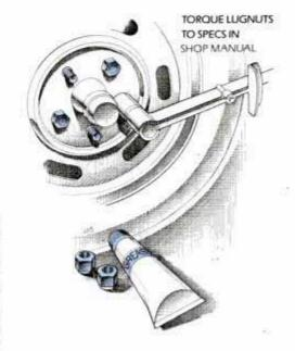
properly torqued, they do not need corrosion to hold them in place.
