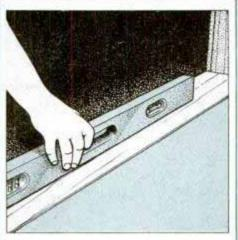
6 Remove old caulking or other sealant from sill, then check for level. If sill is not level, new door must be shimmed to level.
