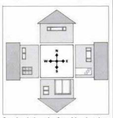
Sample window plan for cold and moderate climates calls for largest windows to face south with less glass on the west and east and the least facing the north.
