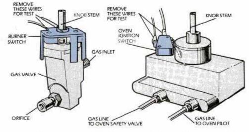
Remove the two wires on each burner switch and on the oven ignition switch to test continuity.
