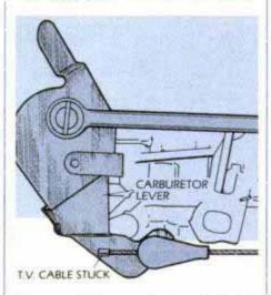
2 When pulled out and released, the T.V. cable should return to its original position.
