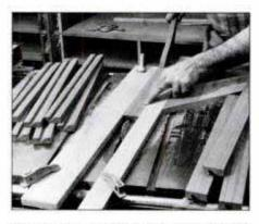
11 Mill door and drawer pulls on a table saw using tilted blade and angled guides. Raise blade  $\frac{1}{16}$  in. after cutting all the pieces. Continue until blade projects  $\frac{1}{2}$  in.
