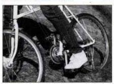
Stainless-steel cables replace frame tube in the Slingshot mountain bike chassis.
