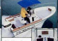
Robalo's excellent glass work and teak trim rated high. Handling could be improved by moving seats closer to console.
