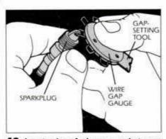
18 Insert wire of plug gauge between inner and outer electrodes to check gap.
