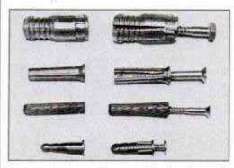
Screw-anchor types, from top: lead anchor with lagscrew, lead with wood screw, lead-lined jute with wood screw, plastic with sheetmetal screw.
