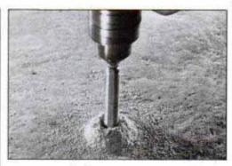
Operate masonry bits at low rpm, about 300 rpm for the ½-in.-dia. bit shown. Apply steady pressure and back out occasionally to clear hole.
