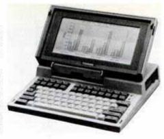
Toshiba's 9-pound IBM-compatible lap-top packs 512K-RAM and 31/2-in. disk drive.
