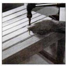
12 Nail seat slats to support frame using 3d finishing nails. Set nailheads and fill with red oak-colored wood putty.
