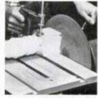
It's a 12" Disc Sander with 113 sq. in. of sanding surface to reduce stock up to 6" thick in a single pass.
