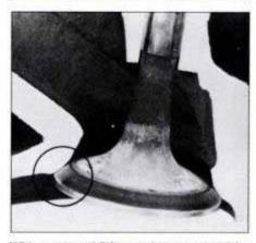
With proper additives, valve-seat area (circled) shows little evidence of wear.
