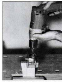
2 Cut seat-support members to shape then clamp in bench vise. Bore dowel holes in ends using doweling jig.
