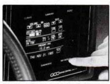
Touch-sensitive cathode ray tube (CRT) operates Buick radio and climate control.
