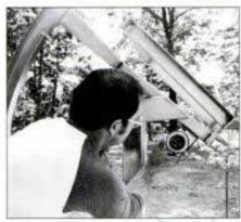
You'll need an inclinometer to get the right elevation angle when sighting dish on the satellites. Note handheld unit above.
