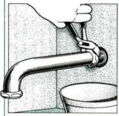
3 Next, loosen and remove the slip nut that joins the drain pipe to the plumbing stack within the wall. Keep all fittings and gaskets for later use.
