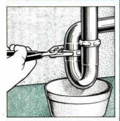
1 Begin by removing the existing waste line. Loosen the P-trap nuts with pilers or a pipe wrench and let the water drain from the trap into a bowl or pall.
