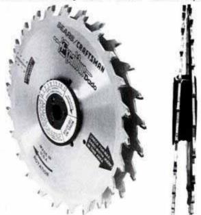
Dado has two 8-in.-dia. saw blades joined by an adjustable collar. The blades tilt on the hub to the desired width of cut (right).
