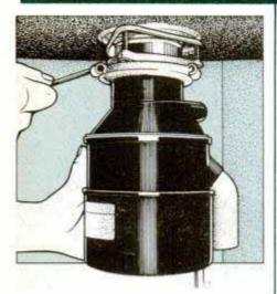
11 Lift the disposer into place, then turn the lug ring by hand until all lugs catch. Finish tightening the lugs with the angled wrench supplied with the unit.
