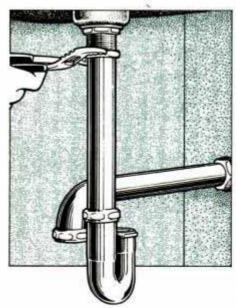
2 Loosen the slip nut that joins the tailplece to the threaded sink sleeve and pull the tailplece from the fitting. Empty the remaining water from the trap.
