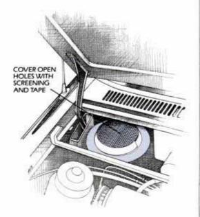
cover cowl openings with ordinary window screening. Use duct tape to hold screening to the cowl.
