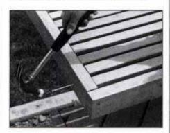
21 Nail seat boards to support frames, making sure that all ends align perfectly. Then cover by nailing end boards in place.
