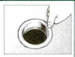
6 Thoroughly clean the sink opening to remove the old putty and then press the new sink sleeve into place. Wiggle the sleeve back and forth for uniform seal.
