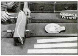
Once setup is complete and all mating surfaces are coated with glue, progressively tighten clamps and let stand until glue dries.
