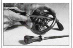
File handles are made from old stamp handles with holes bored in the ends to accept the file. Slip a ferrule cut from brass tubing over the end to prevent splitting the wood.
