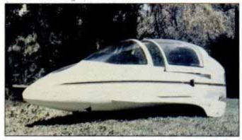
BD-200 autocycle, a motorcycle-based vehicle, is a 2-place tandem.
