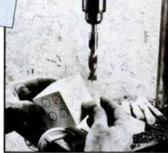
After boring a hole in the cube, insert the mating dowel. Be sure to brush-clean the hold-ing Jig recess so that the cube seats properly.
