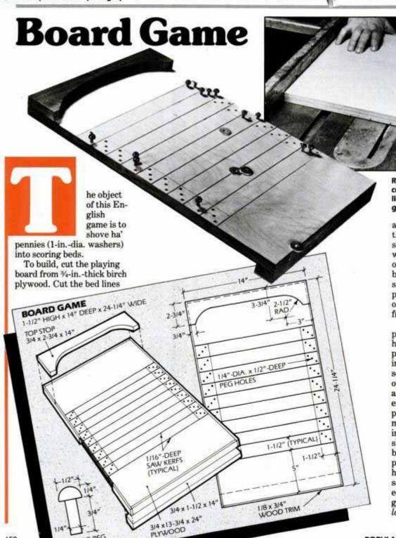
Rip the scoring bed to size and cut kerfs for the scoring bed lines. Then, sand the board and glue on edge band strips.
