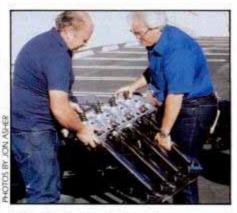
**5** Finally, the head stud nuts are removed and the cylinder heads are taken off with the exhaust headers still attached.
