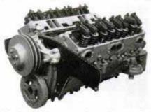
Aluminum plates replace side engine mounts, use block to bolster chassis stiffness.
