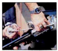
**7** Before reassembly, oil is applied to all bearing surfaces to prevent scuffing before the oil pump can pressurize the system.
