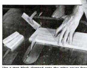
Use a stop block clamped onto the miter gauge fence to ensure that the staves are cut to a uniform size.
