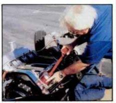
8 Pistons and rods are installed with one shove of rubber-handled hammer, thanks to tapered 1-piece piston ring compressor.
