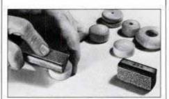
With the rubber lettering peeled off and abrasive paper glued in its place, the stamp block makes a handy sander for small jobs.
