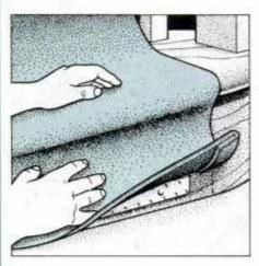
Secure bottom edge of runner to tackless strip on first riser, butted flush against the floor. Place three carpet tacks through each doubled-over edge, into riser.
