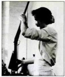
Each piece of Holland & Holland's traditional sidelock action (above left) is forged and assembled by hand. The sideplate then undergoes hand engraving by one of Holland's inhouse craftsmen. The length of pull on one customer's gun is double checked (right).
