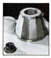
After gluing together the staves, clamp top and bottom.
