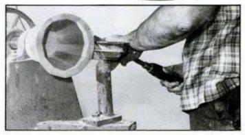
To shape the vase exterior, start with a deep-fluted gouge. Then, finish-shape the wood vase with a round-nose scraper.
