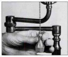
To use as a lamp pull, counterbore a hole in the top of the handle large enough to recess the chain end. Then, from the center of this hole, bore a 1/2-in.-dia. hole through the handle for chain clearance.
