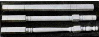
Legs in three stages are, from the top: initial blank has been squared and cut extra long with markings where turnings are needed. Middle leg is roughed out and the bottom leg is completed.
