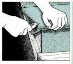
After riser is covered, secure tackless strip and padding to the tread below. Cut carpeting to size and attach it to the tackless strip. Make diagonal cuts at corners.
