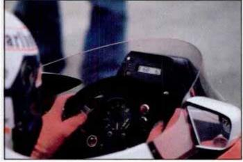
Digital display (above) tells World Champ Alain Prost how much boost he can use. McLaren's space-age carbon fiber and aluminum chassis (right) is made by Hercules Aerospace in Utah.
