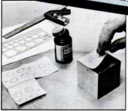
Cut out the pattern and adhere it to the cube with rubber cement. Be sure to position the pattern as shown in the drawing. Centerpunch each hole.
