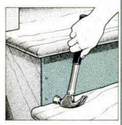
Cut carpet for riser to full riser height. Score carpet at end of riser, and fold against edge of padding. Staple at top and bottom of riser, and tack rolled-under edge.
