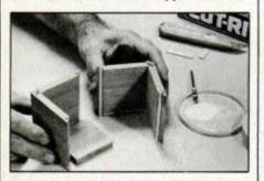
Glue two diagonal corners with splines. Glue bottom, join diagonals and clamp. Waxed paper keeps piece free from table.
