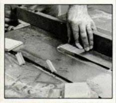
Cut pencil well sides with rip fence set exactly square. Miter one end of all sides, then reset fence to miter opposite ends.
