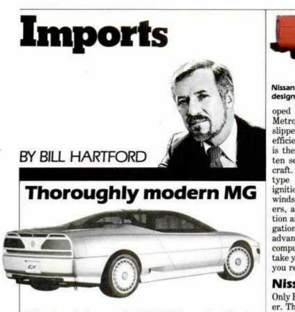
It's a tease to be sure, but this concept-car MG, put together by the Austin Rover Group in England, could become a production car in the 1990s. The EX-E couldn't be farther from the flapping side curtain MGs that came out of the Morris Garages. The MG could now stand for modular and glued up. Three main modules go together with the high-strength, aluminum-alloy frame: one car-
