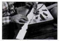
Cut the template shape on a scroll saw, following the paper outline. Mount template on the lathe brackets, as shown above.
