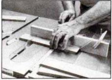
Cut each pair of sides with the same mitered stop block setting. This assures pairs of the same length and tight miter joints.
