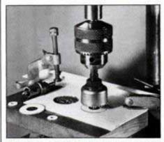
With the center hole cut, use a larger hole saw to cut the washer's outside diameter.
