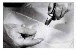
To cut narrow strips, first score the surface, then tap the underside of cut line with the end of cutter handle. Snap off glass with pliers.
