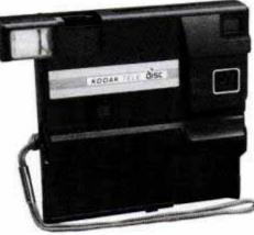
Kodak's TeleDisc camera has normal and telephoto lenses built in. Extending the flash engages the telephoto mode.
