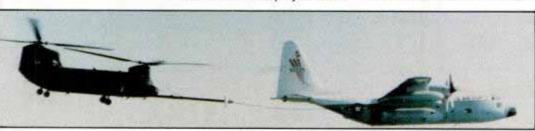
posite fuel probe into a 48inch-diameter drogue attached to the HC-130's 76-foot line. Fuel was transferred through the HC-130's fuel line into the fuel probe located along the CH-47D's side. The refueling took place at 5000 feet at 120 knots. At 150 gallons a minute, it took 6 minutes.
