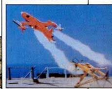
Northrop's Chukar II aerial target vehicle (above) rockets from a British vessel carrying two tow-bodies on its wingtips. Tows contain missdistance measuring devices and target simulators and are deployed 600 feet behind the drone to reduce the chance of damage.
