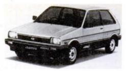
Three-cylinder Subaru Justy will offer 4wheel drive and CVT as options for 1988.
