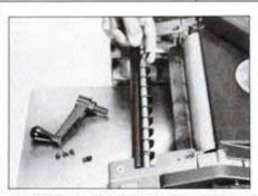
Antikickback fingers prevent stock from being thrown out of infeed opening. Knurled-steel infeed roller grips wood.
