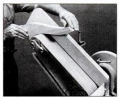
Keep work flat against extension fence to sand square, 90° edges on curved pieces. This isn't possible when sanding freehand.
