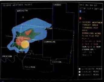
NEXRAD (Next Generation Weather Radar) will consist of a nationwide network of 160 S-band Doppler radar systems, which will warn airports, aircraft and civilians of hazardous weather. Competitive designs have been submitted by
