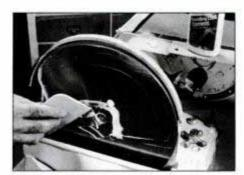
Liquid sanding disc cement provides an easy way to mount the sanding disc. First, apply a thin, even cement coat to the metal plate.
