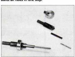
Adjustable length bit (left) has pilot, shank and countersink bits in one tool. Thin pilot bit does tend to break easily (right).
