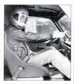
Driving position makes it hard to apply needed muscle to the tiny steering wheel.
