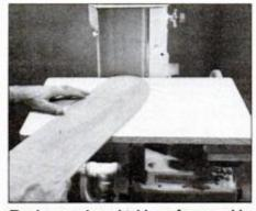
The increased worktable surface provides greater stability for manipulating workpleces and, therefore, increases accuracy.
