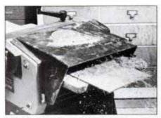
Maximum depth of cut for boards that are more than 8 in. wide is  $\frac{1}{32}$  in. per pass. Stock can be planed down to a mere  $\frac{3}{32}$  in.
