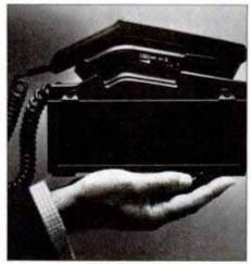
Transportables can be carried in hand, briefcase, or mounted in car. Seen here and in lead color photo is NEC's EZ-1401-A.
