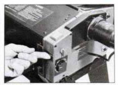
Safety power switch requires key to unlock it. Recess prevents unintentional turn-on. Button above switch is for fast turn-off.
