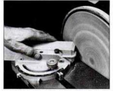
Form accurate, uniform chamfers easily by inserting a stop rod in the miter gauge. Adjust the rod to control the depth of cut.
