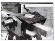
Maximum depth of cut for stock up to 4 in. wide is 1/6 in. using fast speed for softwood and medium speed for most hardwood.
