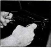
Saab 9000 instruments are lighted by fiber optics; radio can be removed and taken with you, operates only with secret code.
