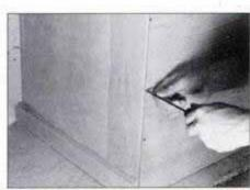
12 Mount the case back with %-in. No. 5 fh brass screws, set 6 in. apart. Counterbore screwholes to set heads flush.
