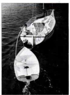
The towing whip keeps continuous tension on vessel being towed, avoiding transom damage on the mother ship.
