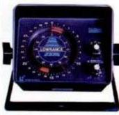
Obviously, the flasher was limited to intermittent flashes between zero and the indicated depth when fish passed between the bottom and the boat's transducer.
