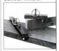
The Bulls Eye gauge quickly and accurately marks a center point.
