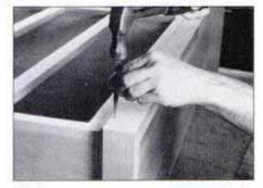
10 Apply base molding with 1-in. brads and glue. Fill nail holes with wood filler or cherry sawdust mixed with clear lacquer.
