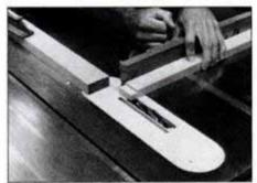
6 Cut ¼-in.-wide tenons with dado blade in a table saw. Clamp a stop block to the table to make identical repeat cuts.
