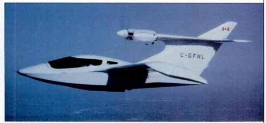
ogy is showing up on a grow- Canada's Seawind 4-place amphibian has smooth wing stall and goes 180 mph at 75 percent power.
