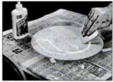
Then, spread a thin cement coat onto the back of the sanding disc. Wait for about 5 minutes before pressing disc to plate.
