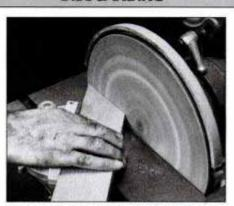
Use a miter gauge to sand precise miters. First, rough-cut the miters on a saw. Then, finish-sand the miters on the disc sander.
