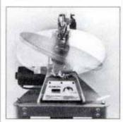
The saw's 16-in.-dia. cast-iron table tilts and locks 30° left, 45° right, 15° up and 30° down.
