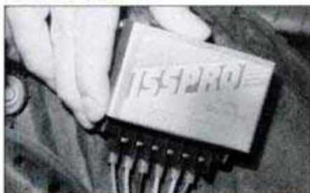
Electronic monitor protects turbocharger from damage by hot-engine shutdown.
