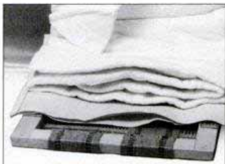
Muslin bag seams should be 1\frac{1}{4} in. wider than seat frame to allow for padding. Turn bag inside out before stuffing it with 3 or 4 double thicknesses of cotton batting.
