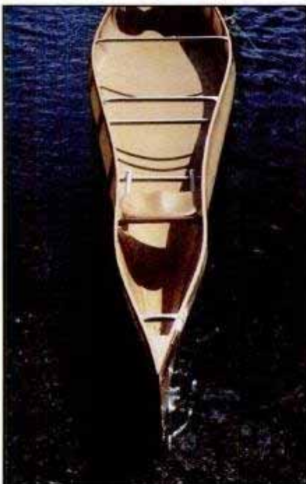
Many racers, like Wabash Valley Defeater, have exotic pinched gunwale shape aft.
