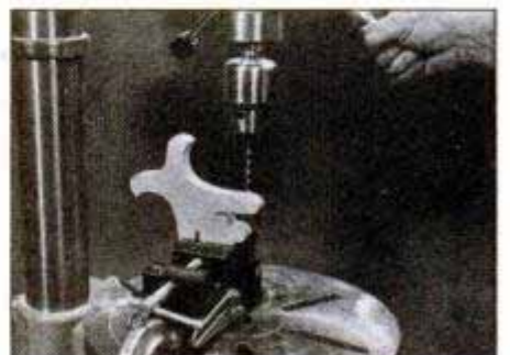
Bore string holes in the hands at right angles to the edges. The proper angle is necessary to make the bear climb.
