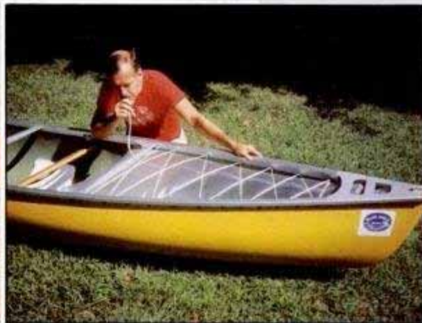
Blue Hole Sunburst, an ABS solo whitewater model with kneeling thwart, gets aft flotation airbag topped off.
