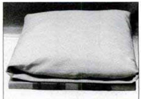
Stuffed bag should be about \frac{1}{2} in. larger than the seat frame. Fold the open end of the bag underneath and slap it to compress the batting and work it into the corners.
