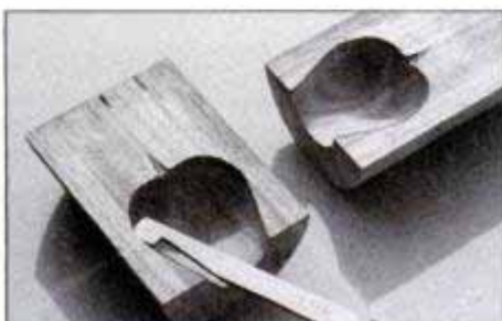
Cutaway sample shows how side scraper was used to hollow out blank. Tool comes with right- or left-hand cutting edge.
