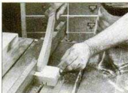
Cut grooves with saw blade set \frac{7}{16} in. high and tilted 11^\circ . Remove waste by making repeated cuts; clean out with chisel.
