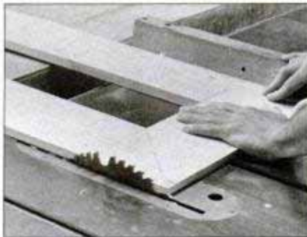
7 Glue, dowel and clamp base frame members together. Then, when dry, cut 18^\circ bevel on front and side edges using table saw.
