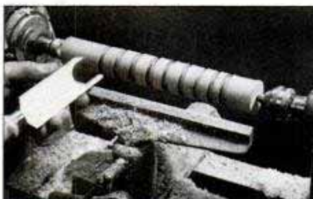
DiAccurate tools come in 10 sizes. Select the desired diameter and feed it slowly into the work. Tool stops cutting automatically.
