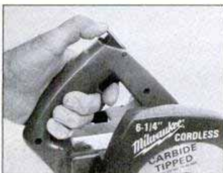
A spring-loaded safety latch prevents the saw from starting accidentally. First, lift the latch, then squeeze the trigger switch.
