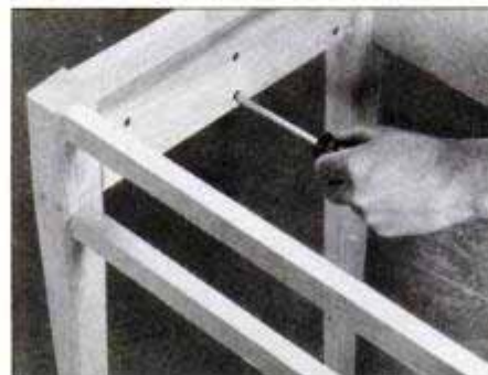
11 After desk base is assembled, screw filler strip to both side aprons to support drawer slides. Countersink screwheads.
