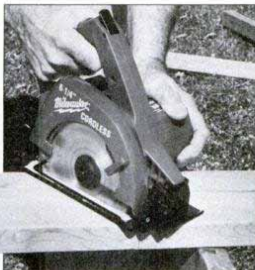
Cordless, battery-operated 6 1/4-in. circular saw has the power to cut through 2x6 stock easily.
