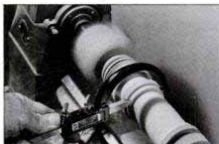
Diameter sizing tool fits on most parting chisels. It can cut up to a 2-in. dia. and is excellent for doing repetitive turnings.
