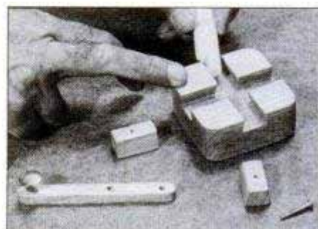
After applying the finish, wax the grooves for smooth movement. Then, assemble the crank and pistons using brass screws.
