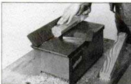
Compact jointer features a cast-aluminum worktable, four nonskid rubber feet and a fence that adjusts from zero to 45°.
