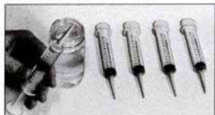
Test kit detects alcohol level in gasoline.
