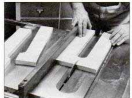
3 Cut each board in half to produce two leg members. As a safety measure, place two fingers over the saw fence, as shown.
