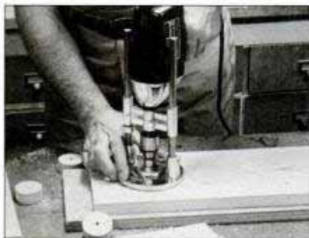
1 Form the inside leg corners using a drill and a 2\frac{1}{8} -in.-dia. hole saw. Drill guide attachment ensures accurate, true holes.
