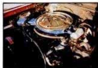
Ford Cobra Talladega 428-cu.-in. V8, 4-barrel carburetor, 335 hp
