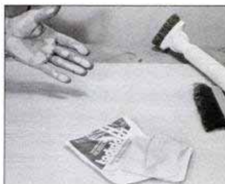
After sanding, wipe surface with a tack cloth. Note how much dust is picked up on hand after just brushing and vacuuming.
