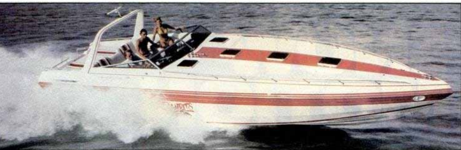
Deck gear on the 42 includes grab rails up forward and centerline vent hatches. Close-up of arch (below) shows radome mount.
