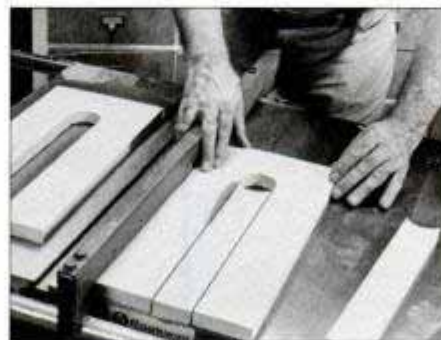
2 Drop out the waste area by making a tangent cut on both sides of the hole. High saw blade reduces length of undercut kerf.
