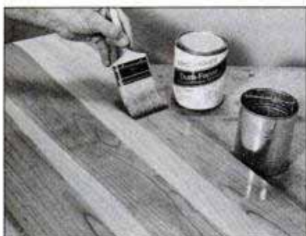
Brush on varnish in full, wet stripes spaced about a brush-width apart. Varnish can be applied heavier than shellac or lacquer.
