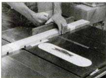
5 Tape vertical and horizontal grid parts together in separate groups. Then, lay out and cut cross lap joints using dado blades.
