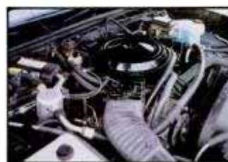
Chevy Monte Carlo SS 305-cu.-in. V8, 4-barrel carburetor, 190 hp
