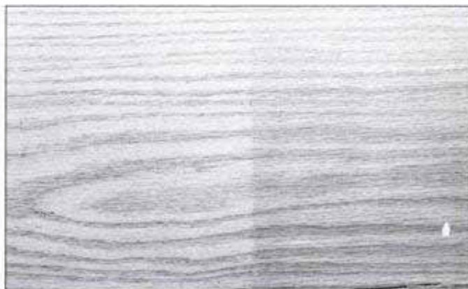
Here's a close-up view of an unfinished piece of red oak. The unfilled left side has a porous, rough texture. The right side has been filled to produce a smooth foundation for the clear topcoat finish.
