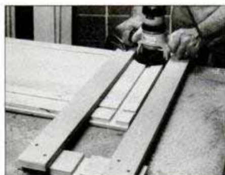
1 Cut lengthwise rabbets and grooves in case sides using dado blades in table saw. But cut cross rabbets and dados using router.
