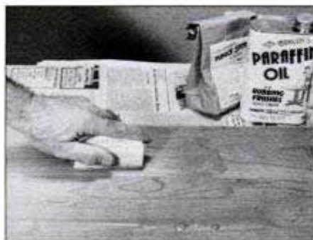
Using a felt pad, rub the final coat with pumice stone lubricated with paraffin oil or water. Stroke with the wood's grain.
