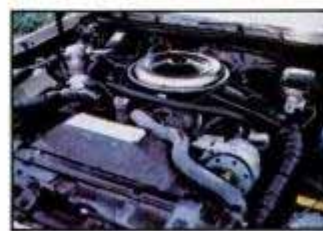
Olds 442 307-cu.-in. V8, 4-barrel carburetor, 190 hp
