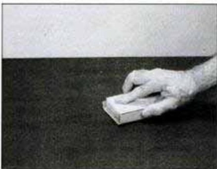
14 To acquire a smooth, level finish, sand each lacquer coat using a felt-padded wood block and 280-grit aluminum oxide paper.
