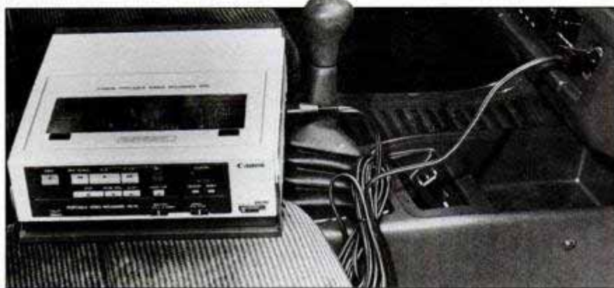
Adapter cord (left) plugs into lighter to tap car battery. Rechargeable Nicaid belt (above) gives 7 to 9 hours of power.
