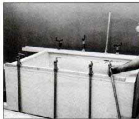
6 Glue frame to case using bar clamps spaced 2 ft. apart. Be sure to use glue blocks between clamp and face to avoid damage.
