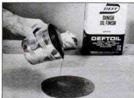
Easy-to-use penetrating oil contains tung oil and urethane to seal and protect the wood's surface. Apply the oil liberally.
