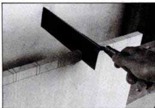
1 Lay out dovetail pins on the ends of the front and back panels. Then carefully cut the pin sides to depth using dovetail or backsaw.
