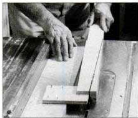
5 To cut taper, place end of leg in jig notch then feed both over blade. Width of notch matches finished width of leg bottom.
