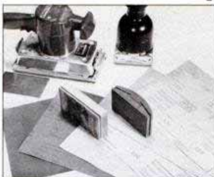
Surface preparation tools (clockwise from upper left): finishing and palm sanders, rubber and felt-backed sanding blocks, scraper.
