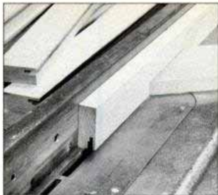
7 Rip grooves in door rails and stiles to accept glass panels. First cut is for spline. Second cut (shown) forms ledge for glass.
