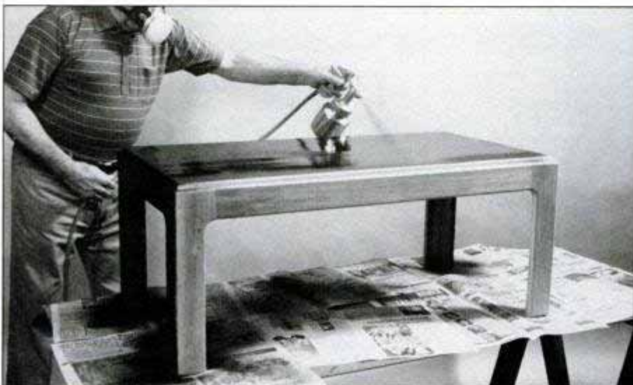
13 After applying two coats of sanding sealer, spray on three coats of gloss lacquer enamel. Move the spray gun parallel to the surface. Be sure that you wear a respirator.
