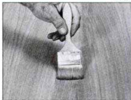
After applying a base coat of sanding sealer, brush on lacquer with long, quick strokes. Lacquer dries fast, hard and crystal clear.
