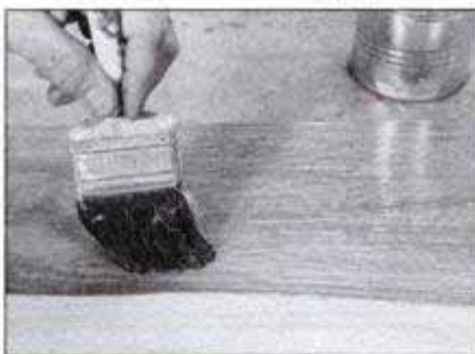
Brush with the wood's grain using a stiff bristle brush. Force the filler into the open pores. Then, brush across the wood's grain.
