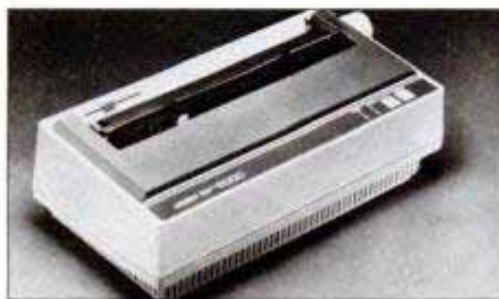
Daisywheel in Juki 6000 printer punches 10 characters a second in bidirectional mode. The printer weighs just 13 pounds.
