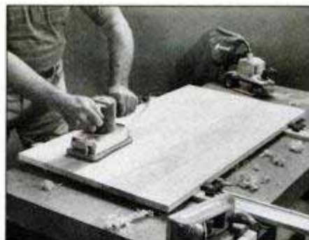
12 Trim the slab to the finished size. Then, plane and belt-sand the surfaces smooth. Finish-sand tabletop with orbital sander.
