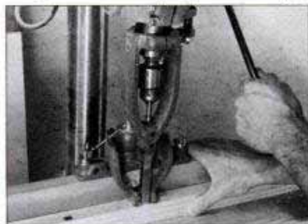
2 Cut grid mortises in rails and stiles using drill press mortising attachment (above) or doweling jig and handheld chisel.
