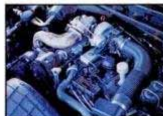
Buick Regal Grand National 305-cu.-in. V8, multiport fuel injection, turbo, 200 hp
