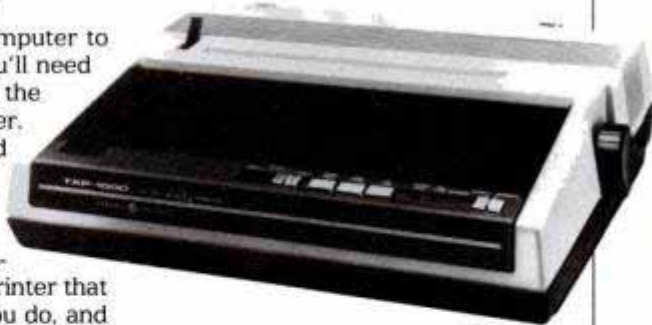
Dot-matrix print element gives graphics ability to General Electric's new printer.
