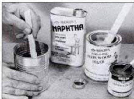
Thin the wood paste filler to the consistency of very thick paint with naphtha. Tint natural shade wood filler with Japan colors.
