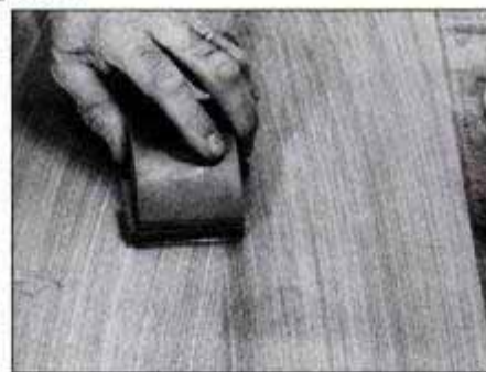
Once the lacquer has dried, sand the surface level using 280-grit wet/dry abrasive paper lubricated with paraffin oil.
