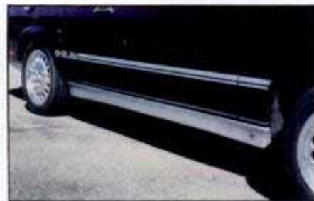
Ground effects panels reduce amount of air that can spill back under the sides of a car.
