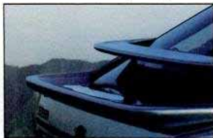
Dual rear wing on Merkur reduces turbulence behind car, allows room for wiper.
