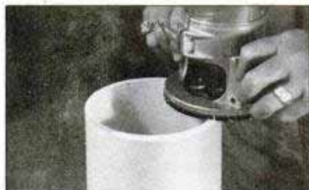
4 Rout the outside edge of each leg end with a 1/4-in. rounding-over bit. Hold the pipe securely upright in a vise and advance the router slowly for smooth, clean cuts.
