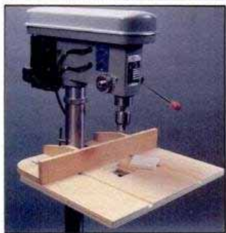
Auxiliary table provides a large, sturdy surface for handling oversized workpieces. Replaceable, 1/2-in. plywood table insert is removed for certain sanding operations.
