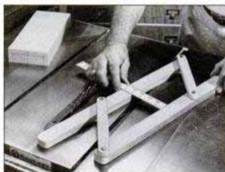
2 Build a parallel rule jig as explained in the text, then adjust it so the space between sides equals the desired cove width.
