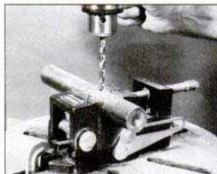
Drill press vise provides a safe, secure way to hold workpieces. Be sure to clamp the vise securely to the drill press table.
