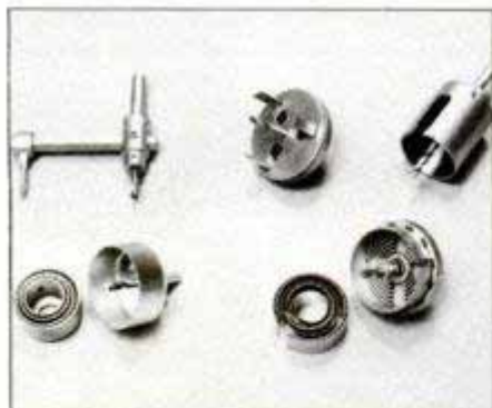
Fly cutter (upper left) is shown with hole saw models (clockwise from top center): adjustable, Enduro, bell type and 7-in-1.
