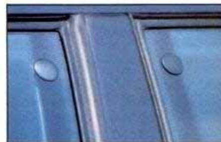
Pegs on Audi windows ride on internal tracks so side glass can be flush with frame.
