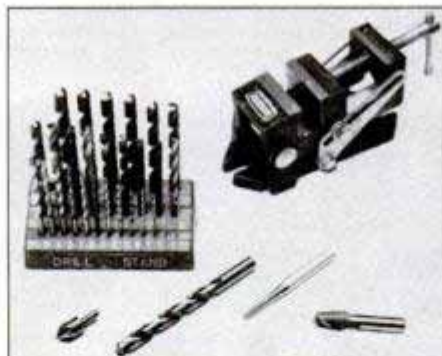
Metalworking accessories (clockwise from upper left): twist drill set, vise, end mill, centerpunch, twist drill and countersink.
