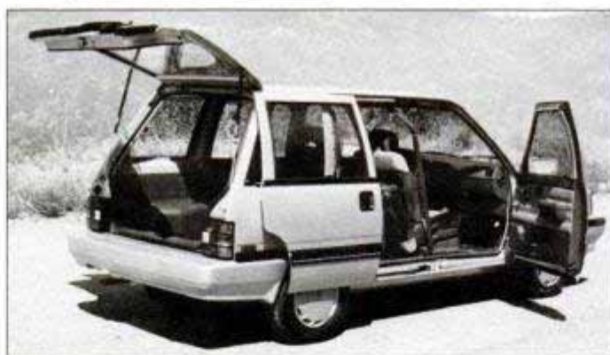
Square-rigged Stanza Wagon has hinged front doors, two sliding side doors and a hatchback/cargo door. There are no B pillars.
