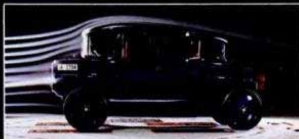
Most aerodynamic production car ever tested is this 1921 Rumberg Teardrop car. Its Cd: 0.28. It didn't sell and Rumberg folded in 1926.
