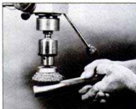
Cup-type wire brush removes rust, tarnish, paint and grime from metal surfaces easily. Grip the work firmly with two hands.
