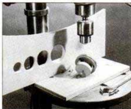
Adjustable hole saw can be changed to cut any size hole within its capacity. This model cuts holes from 1 1/2 to 2 1/2 in. dia.
