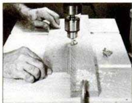
When using a low-speed shaper bit, clamp a fence to the drill press table to guide the work and control the depth of cut.
