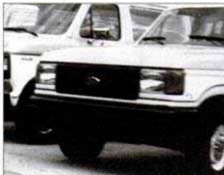
Full-size F-350 pickup prototype sports flush aero headlights, just like on a Mark VII.
