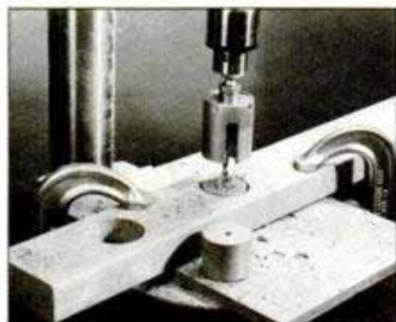
The Enduro hole saw features a single carbide-tipped tooth and the capacity to cut through 1 1/2-in.-thick stock in one pass.
