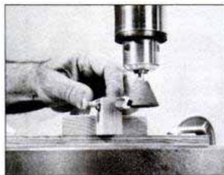
Sharpen router bits with a cone-shaped grinding stone. Short bolt in threaded insert holds the bit securely in a homemade jig.
