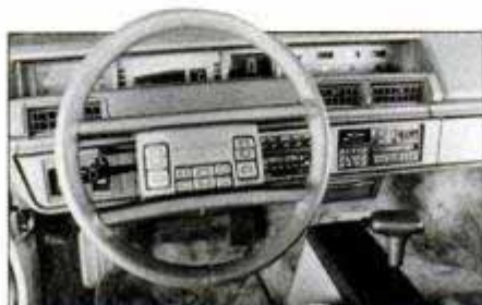
Pontiac Advanced Radio Concept adds full radio control to the steering wheel hub.
