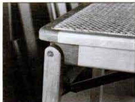
11 After hardware is attached, join seat to support frame by driving screws up through support frame into underside of seat panel.
