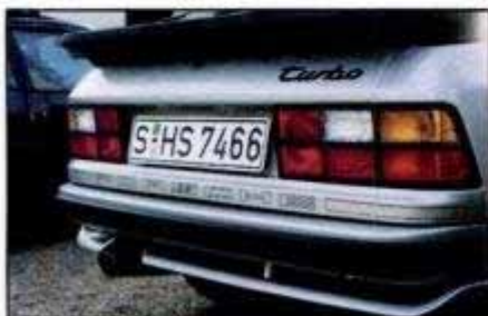
Rear lip on Porsche 944 Turbo controls air exiting from under car to reduce turbulence.
