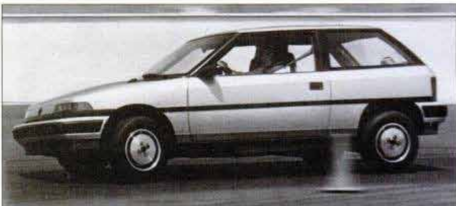
GM's Saturn prototype has the "formal" roofline typical of so many GM models. The Cavalier-size car has a 1.9-liter aluminum Four with fuel injection and fwd.
