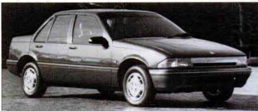
Chrysler's Liberty I prototype is a Colt-sized hatchback with a plastic body and a 1.6-liter, 3-cylinder version of the Mopar 2.2-liter Four. Styling has Honda overtones.
