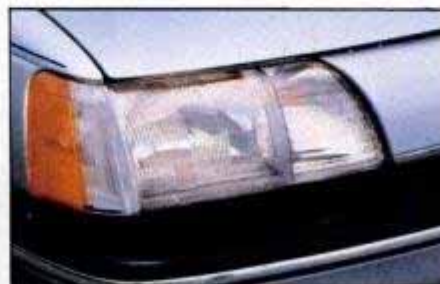
Flush headlights smooth airflow around nose of car. Most have replaceable bulbs.
