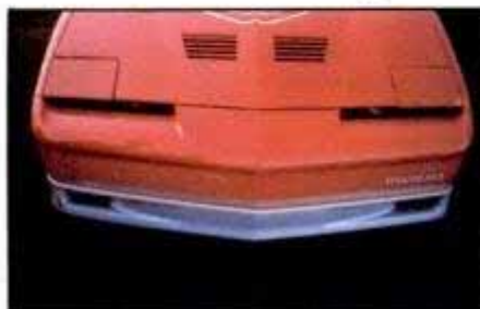
Trans Am has no grille. Cooling air is taken in from high-pressure area under the nose.
