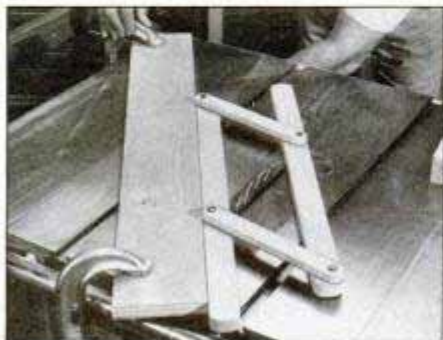
4 Temporarily clamp an auxiliary fence to the saw table in line with the jig. Be careful not to knock jig out of alignment.
