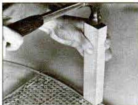
7 Stretch cane over frame and hold temporarily with 1-in.-long dowels. Drive full spline into groove with hammer and block.
