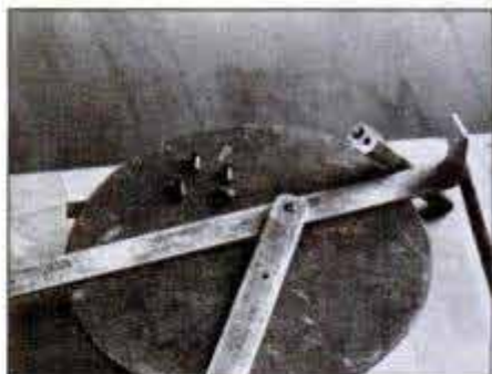
9 Slide solid rivet through mating holes in folding hardware, then round over straight end by striking riveting tool with hammer.
