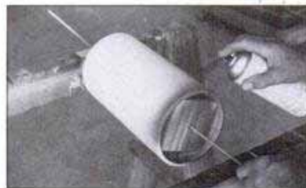
6 Suspend the legs between sawhorses to make painting easier. Apply two coats of sandable enamel primer followed by a coat of gloss enamel in the color of your choice.
