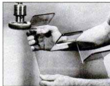
Polish plastics and metals against a buffing wheel coated with rouge. Keep the workpiece in motion to prevent scorching.
