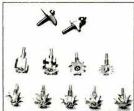
Perform shaping operations using standard router bits (top row) or specially designed low-speed shaper bits (bottom rows).
