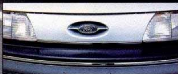
Aerodynamic touches on upscale Taurus nose include flush-fitting headlights, blocked-off grille with floating Ford logo.
