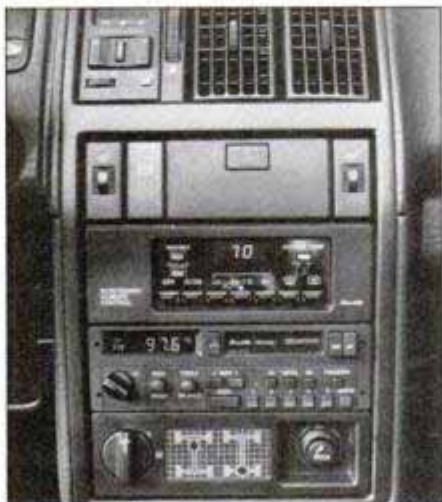
Center dash panel carries controls and display for differential lock functions.
