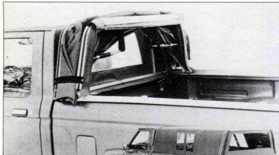
Collapsible cap slides on aluminum rails to allow tall loads (top) or lockable storage space (inset).
