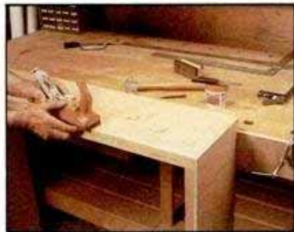
6 Glue and nail hardwood stiles in place with edges overhanging slightly. Then, plane stiles flush to cabinet.
