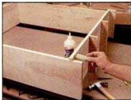
5 Glue and nail \frac{3}{4} -in. blocks to the front edge of the sides. The blocks bring the sides out flush with the cabinet bottom.
