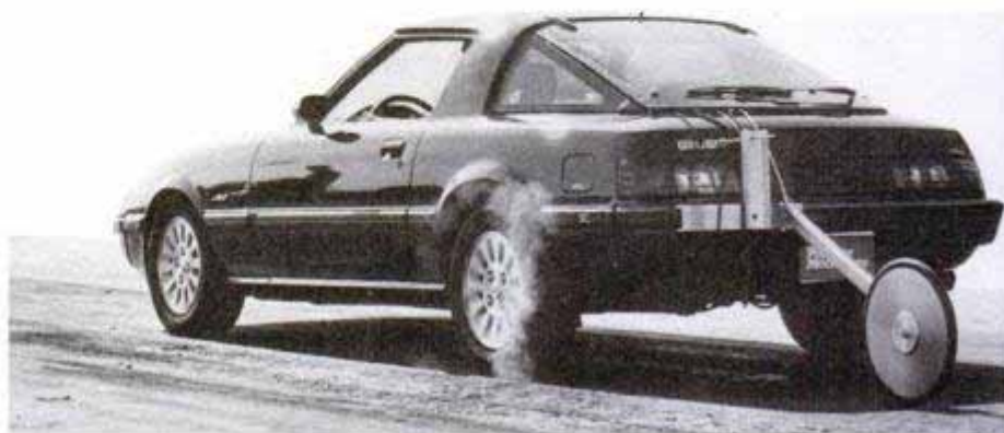
The computer gets its raw data from the fifth wheel—a high-tech sandwich of aluminum and balsa wood that trails along behind the car on acceleration and braking runs.
