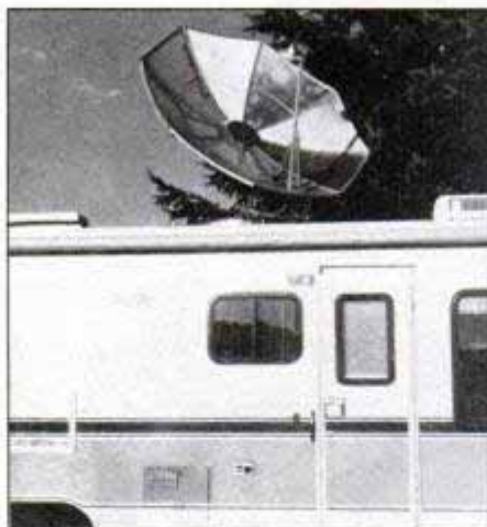
Typical roof-mount antenna—this one is a TravelSat dish—is deployed for reception.
