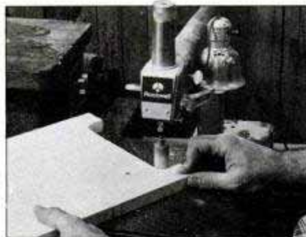
Cut the curves on the sides and the front rail with a jigsaw. Then smooth with sanding drum, or a rounded sanding block.
