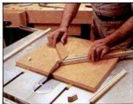
10 Miter the ends of the trim pieces after routing the decorative edge. A homemade mitering jig ensures safe, accurate cuts.
