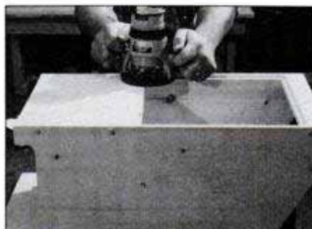
Cut a 5/16-in.-deep x 3/8-in.-wide rabbet around the back opening for wire mesh and cleats. Square corners with a sharp chisel.
