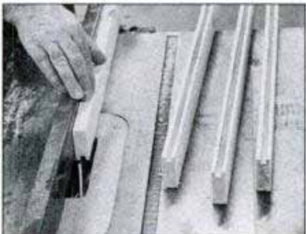
2 Cut \frac{1}{4} -in. grooves in web frame pieces for dust panels and splines. Adjust groove width for under-thickness plywood.
