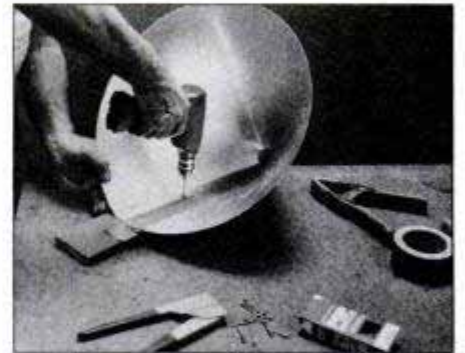
To make baffle, cut shape using pattern, then bend aluminum into cone shape. Tape ends together and drill rivet holes.
