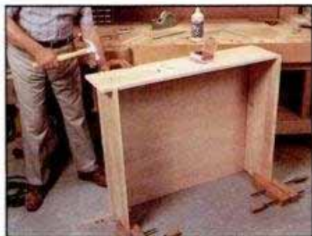
4 Assemble the bookcase with glue and 4d finishing nails. Tape the back panel in place temporarily to hold the cabinet square.
