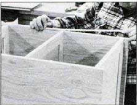
6 Rip edging strips a hair wider than \frac{1}{4} in. Glue to side, then frame edges, and clamp with strips of masking tape until dry.
