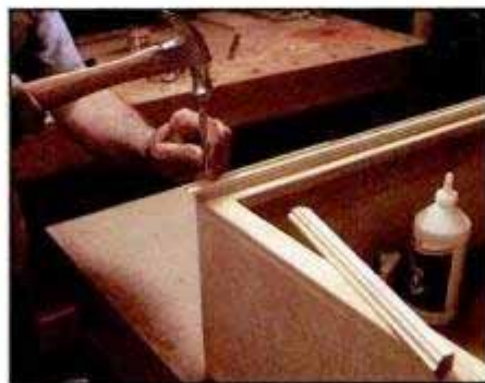
11 Glue and nail the trim to the cabinet. Be sure to bore pilot holes first. Then, set the nails and fill the holes with wood putty.
