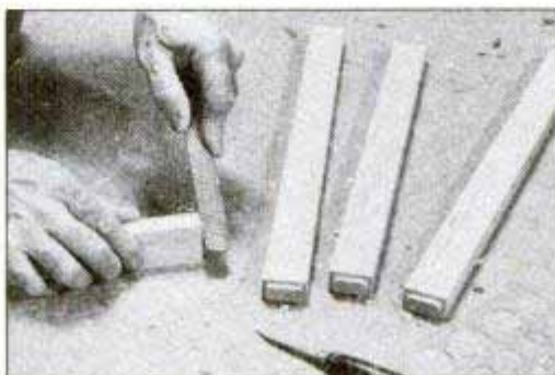
Cut crosspiece tenons on a table or radial-arm saw. Then, trim tenon corners with a knife and file to match round ends of mortises.
