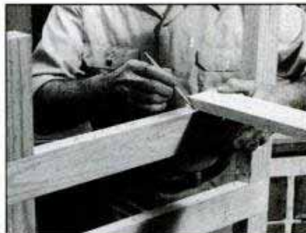
3 Assemble frame temporarily and position stretchers on vertical parts to permit marking the notch locations accurately.
