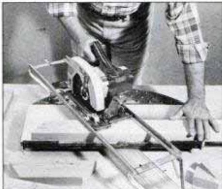
Adjustable guide allows you to cut accurate miters with circular saw. Track assembly swings to the left and right 45°.
