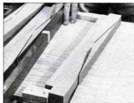
11 Before making second cut, reposition rear guide block. Tape markers on fence and jig base indicate when to stop cutting.
