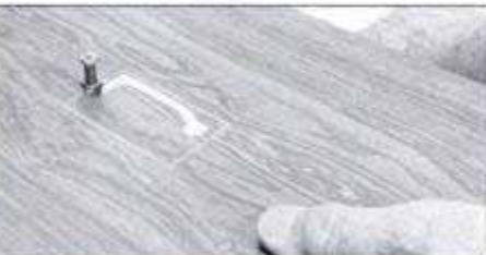
Use the Nibbler to make neat cutouts in plastic laminates. Bore a 1/16-in.-dia. hole in the waste area to start the cut.
