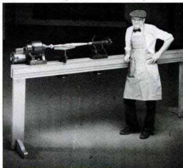
Wood lathe features unlimited center-to-center capacity for turning extra-long pieces such as porch posts and columns. Custom-make the lathe bed from two 2x6s.
