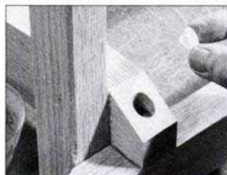
15 Cut an angled plug to conceal the bolt at seat supports' front end and to provide a solid nailing surface for the seat slat.
