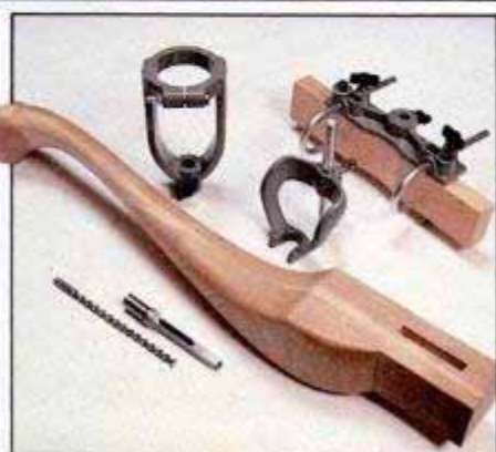
The mortised cabriole leg is shown with a five-piece mortising attachment. Note the drill bit and hollow chisel (front, left).
