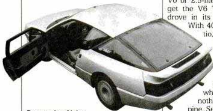
Rear-engine Alpine has its V6 longitudinally mounted under the hatch with enough room left for two small, rear bucket seats.
