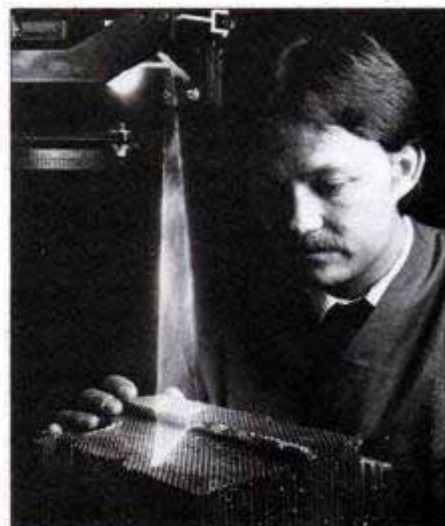
A Northrop researcher follows 3-D laser light as it measures part of an aircraft.
