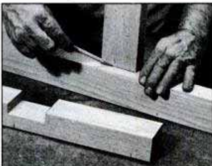
2 Insert vertical frame part into horizontal member's notch. Then mark the vertical part to indicate the end rabbet length.
