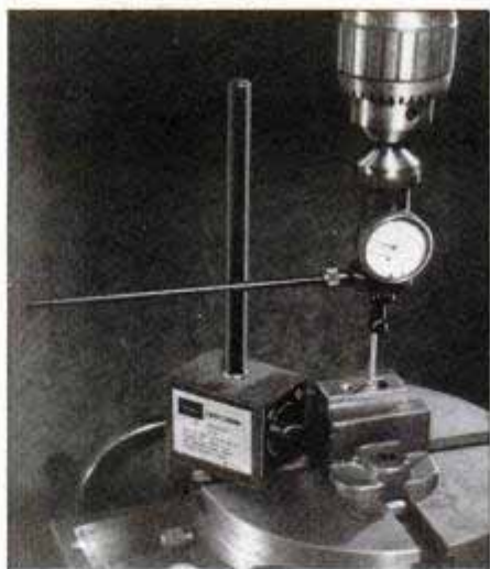
Co-Ax Indicator speeds setup of machining by simplifying the centering operation.
