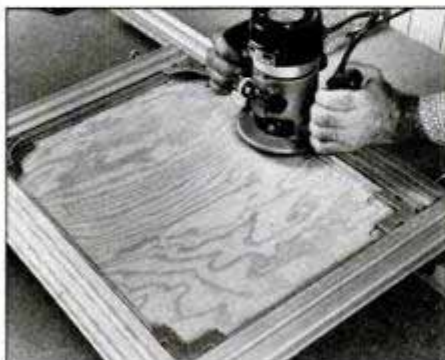
Grip router with both hands, and set and lock depth adjustment. Then run the router around workpiece periphery with the bushing riding on rails and templates.
