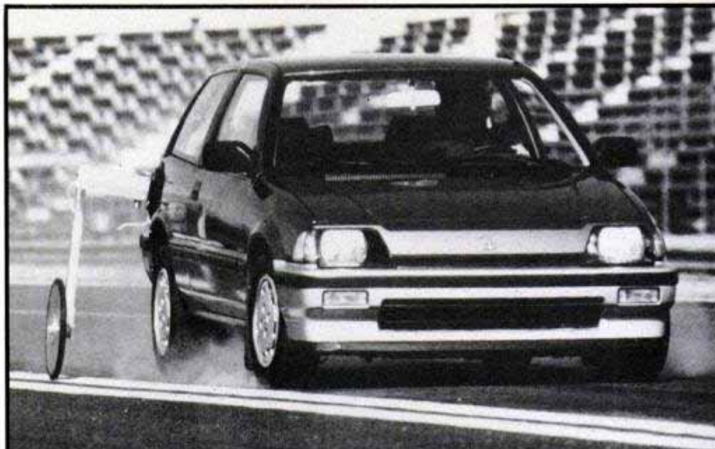
The Honda Civic S had one of the shortest stopping distances we've ever recorded from 60 mph—120 ft. The VW and Dodge were close behind it, both stopping in 124 ft.
