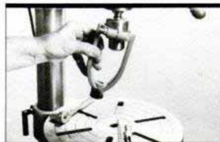
Slip the chisel holder over the chuck and onto the base of the quill. Then, tighten the locking bolt to hold it securely in place.
