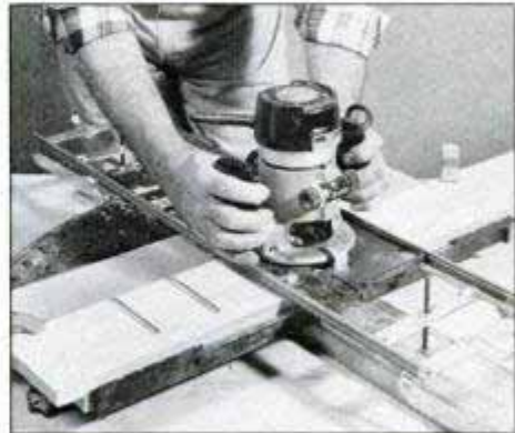
The guide's sliding base plate also accepts a router. Adjust the track assembly to secure the router at the desired cutting height.
