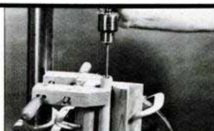
To bore into the end of round stock, adjust the worktable into a vertical position with the V-block device clamped in place.
