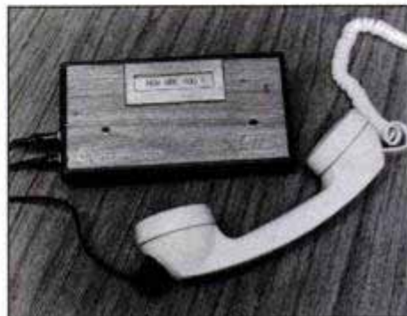
Echo 2000 converts tones to words on a scrolling display for the hearing impaired.
