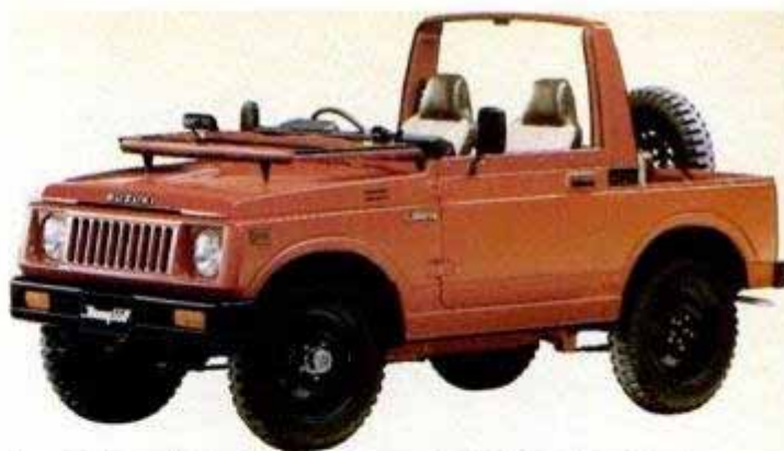
Suzuki Jimmy SJ is a miniature Jeep only 10 1/2 feet long. Its three-cylinder, 539-cc engine belts out a rompin', stompin' 28 hp.
