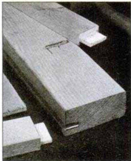
Cut the leg grooves for the side and back deeper where the rails intersect so they will accommodate the longer tenons.
