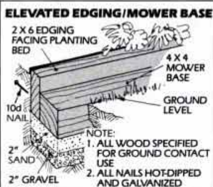
An L-shaped wooden structure sunk in the ground is used as a raised, flower-bed border and as a lawnmower base.
