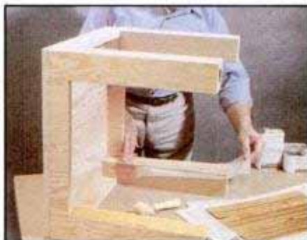
6 Use wax paper to separate the glued surfaces to allow positioning veneer. Then, remove paper and press veneer down.
