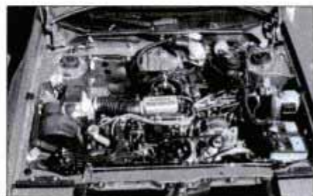
Subaru's new overhead-cam flat-four has excellent service access without a/c or turbo.
