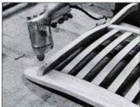
Attach the seat-back upper rail to the sides with 1\frac{1}{2} -in. No. 8 fh brass screws. Bore pilot holes and countersink the screwheads.
