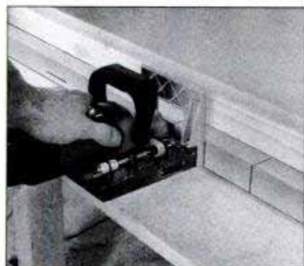
A good way to join top boards is with plate jointer tool. It registers off workbench to cut concave grooves for premade splines.
