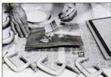
We applied the wavy overlay veneer with woodworking glue. Apply glue to both surfaces and clamp quickly before it sets.
