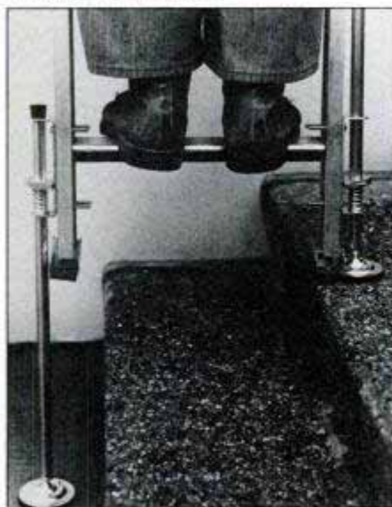
Ladder levelers are essential for working safely on stairs and uneven ground. Nonskid swivel feet maintain full ground contact.
