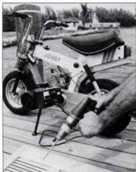
The generator mounts on power take-off.
