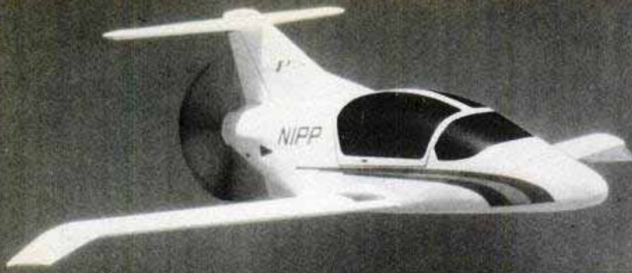
Futuristic Prescott Pusher, shown as mockup above, is 180-hp, retract-gear, metal-and-composite four-seater capable of cruising at nearly 200 mph. Rear-engine layout permits slim bullet nose with superb visibility, low cabin noise. Kit is $15,350, less engine.
