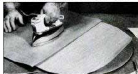
Apply iron-on veneer with a hot clothes iron. Place a sheet of paper between the iron and the veneer to prevent scorching.
