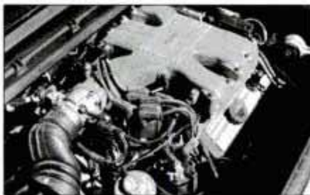
Chevy's 2.8-liter V6 is a tight squeeze in Fiero's engine bay. Note flat intake manifold.
