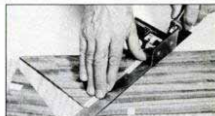
Cut the four 90° segments simultaneously from a stack of matching veneer strips using a veneer saw and combination square.
