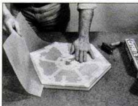
Separate glued surfaces with wax paper to permit positioning veneer exactly. Remove the paper and press down the veneer.
