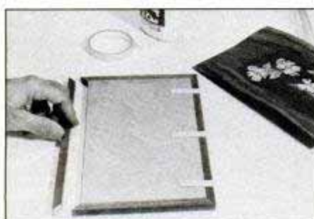
Make the box top from ½-in. birch plywood edged with ½ × ½-in. walnut. Glue and tape the edging to the plywood top.
