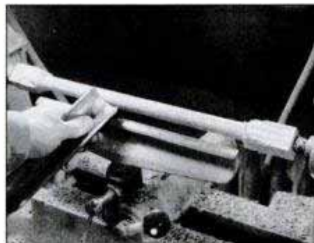
Turn towel bar to 1\frac{1}{4} -in. dia. on lathe using red oak stock to match rest of cart. Sand smooth, then cut to length on table saw.
