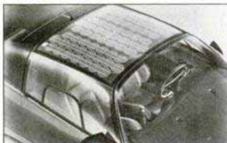
Solar cells power a fan that ventilates the interior when car is parked in the hot sun.
