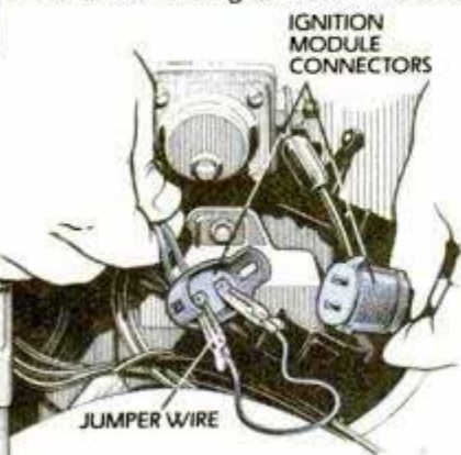
2 Ford-type electronic ignition modules must be jumped to set timing correctly.
