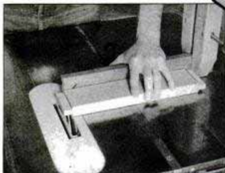
Cut apron tenons on table saw using dado blades. Clamp, on miter gauge, acts as stop block for making repeated cuts accurately.
