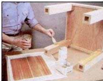
5 Apply glue to the veneer strips and to the inside leg surfaces with a brush. Tape down the strips to prevent curling.
