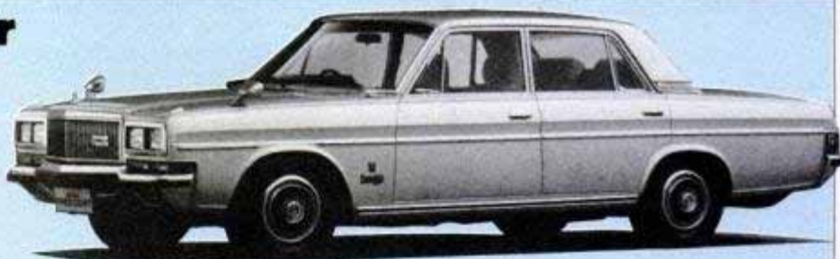
Nissan President is powered by a 200-hp, 4.4-liter V8 that delivers 13 mpg in city driving.
