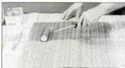
14 Book-matched veneers are taped together to form the tabletop veneer. Apply veneer glue with a short-nap paint roller.
