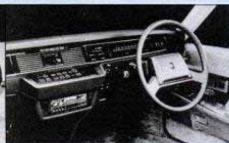
Toyota Century limo has a 190-hp V8 and rear-wheel drive. Interior includes rear seats with a built-in massage function. Although right-hand-drive dashboard looks like a '60s Chevy, it masks an ultramodern, fiber-optic electrical system.
