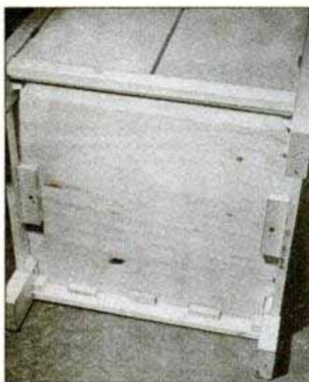
Bottom rests on edge of back and side rails, and a support cleat at front. Glue blocks around bottom give cabinet rigidity.
