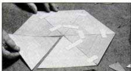
Assemble the pieces into a hexagon shape using gummed veneer tape. If cut accurately, the last piece will fit without trimming.
