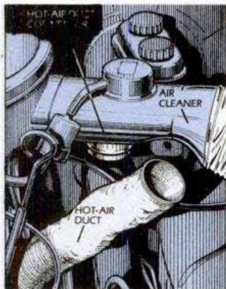
5 A disconnected carburetor hot-air duct will cause cold hesitation and stalling.
