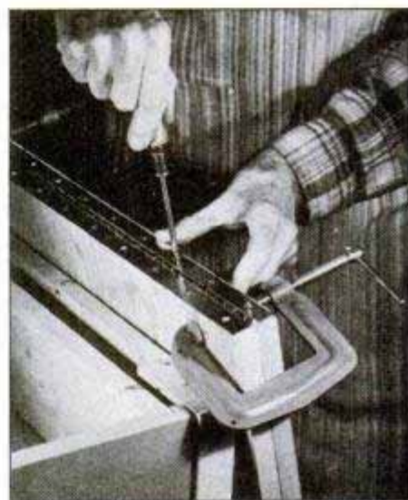
Join the fixed top to the swing-over top with a continuous hinge. Then, attach the fixed top to the legs with screws.
