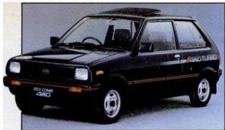
Subaru Rex Combi features four-wheel drive and a two-cylinder engine good for 65 mpg. Normal engine has 31 hp, turbo 41 hp.
