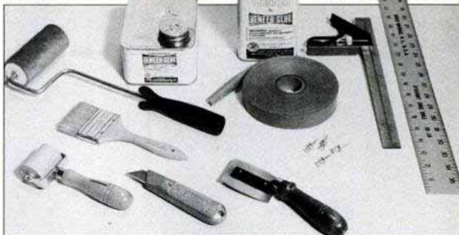
Veneering tools (clockwise from lower right): saw, knife, veneer roller, brush, paint roller, glue, thinner, veneer tape, pins, combination square and straightedge rule.
