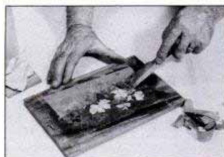
Remove protective paper from the veneer by moistening it slightly and then scraping it with a wide chisel or cabinet scraper.
