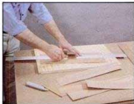
4 Use a veneer saw and straightedge to cut the inside leg veneer. Cut the strips slightly wider and longer than needed.
