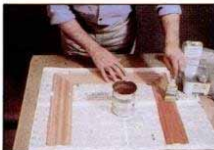
11 Apply veneer glue to the leg/apron veneer assembly. The parts are taped together to ensure tight-fitting miter joints.
