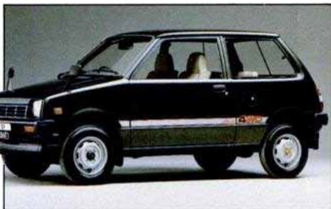
Daihatsu Mira hatch has a two-cylinder engine and four-wheel drive with 30 hp. Turbo model with 41 hp has front-drive only.
