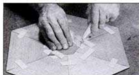
Tape the diamond-shaped inlay motif to the veneer assembly for use as a template when cutting out the center area with a knife.
