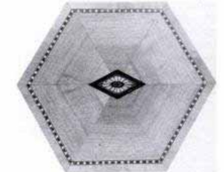
The completed table top after trimming, tape removal and finish-sanding. Allow about 48 hours before applying a finish.
