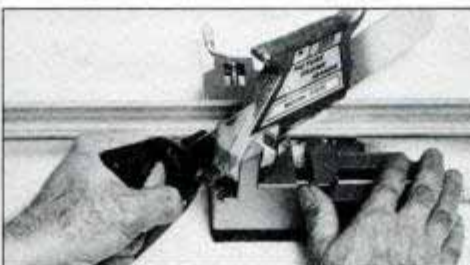
Move saw guide and backsaw to right end clamping fixture and make the second miter cut. Repeat for matching frame member.
