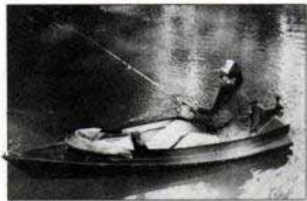
The Sidekick one-man sport boat weighs only 48 lb. but has a 350-lb. carrying capacity.
