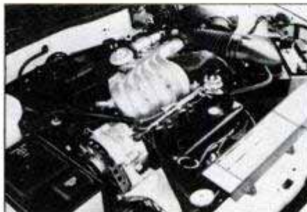
All-new 3-liter V6 has 60° angle between cylinder banks for smooth operation. Distinctive fuel-injection manifold is aluminum.
