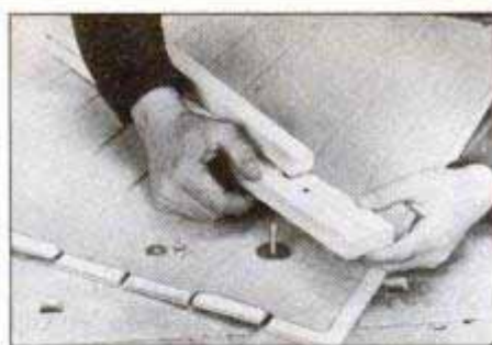
Attach leg supports to tabletop with carriage bolts and wingnuts. Washers between supports and top allow supports to swivel.
