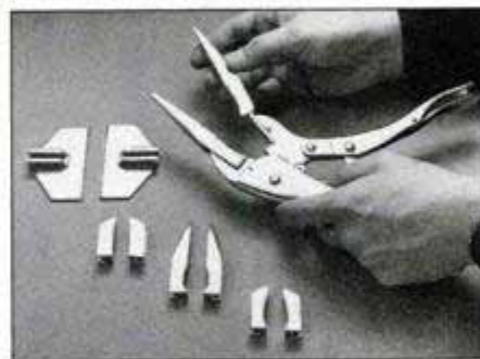
Locking pliers accept five jaw styles.
