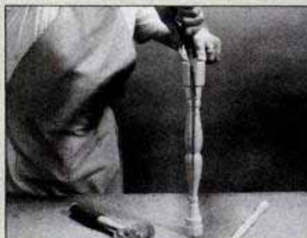
Use a chisel to separate the spindle halves. Slight chamfers on the ends of the parts make it easy to insert the chisel.
