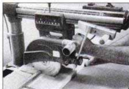
To cut precise stopped dados across the surface of board, firmly attach clamp to saw arm to limit outward travel of the carriage.
