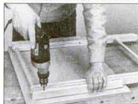
Join the two pairs of legs, then the leg assembly to the brackets, with pivot screws. Glue and screw brackets to table bottom.
