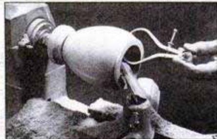
Check the wall thickness frequently with calipers while hollowing out. Toolrest is positioned for maximum support.
