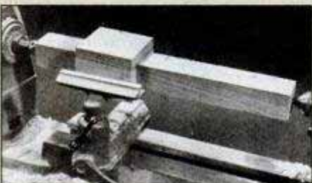
Mount the blank between centers after building up the mid-section with glued-on blocks. Be sure the glue dries thoroughly.
