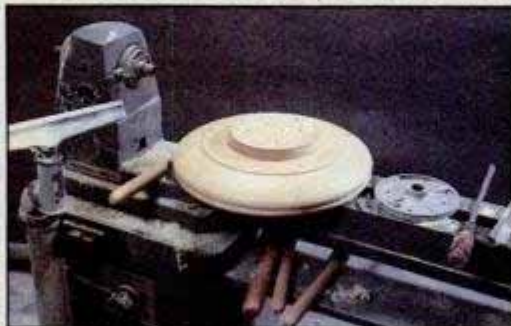
A large tray is being turned on the outboard end of the spindle (top). Note the use of a floor-standing toolrest holder. Tray bottom has a glued-on base for mounting the face plate (above).
