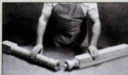
Use this mortise-and-tenon technique to produce columns and spindles of virtually any length. Join the parts with glue only.
