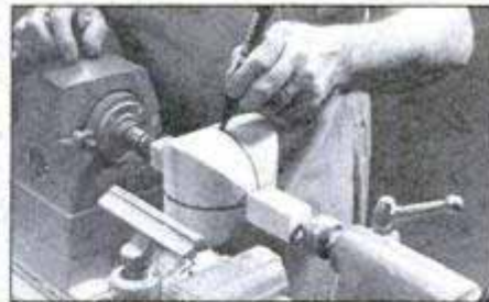
Mark centerlines on the blank so that when the piece spins, the ball's outline will become visible and help guide the cutting.
