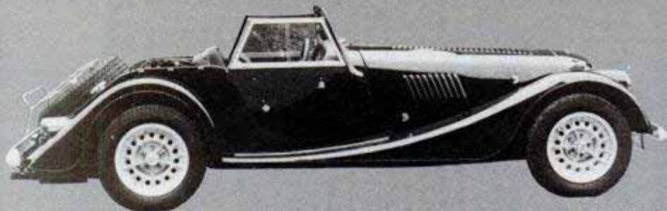
The Morgan roadster has been available, wood frame and all, since the mid '30s. You can buy one with a propane-powered four-cylinder engine or an aluminum Rover V8.
