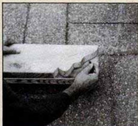
After sculpturing the ends of one crossarm with a sabre saw, use it as a template to lay out and mark the other crossarm.
