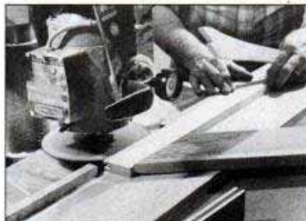
To groove an edge, align blade, lock yoke, feed work against blade rotation. Feather-board keeps work against fence.
