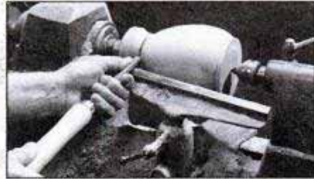
Tailstock center stabilizes blank while exterior is shaped. Keep parting cut at base shallow until turning is completed.
