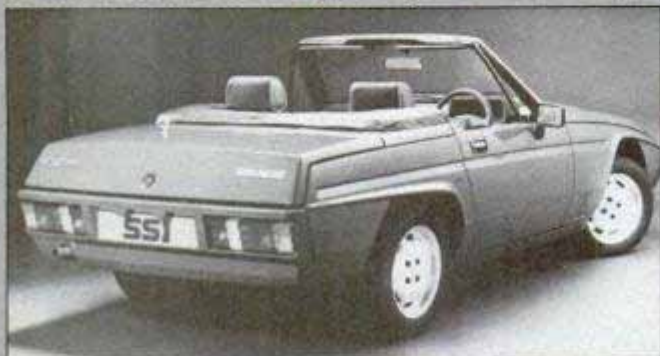
Reliant Scimitar SS1 convertible, with Ford Escort engine and rear-wheel drive, is a modern-day MG Midget/Triumph Spitfire.
