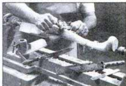
Engage the indexing pin in the headstock pulley to keep the leg from rotating. Then, finish-shape with assorted hand tools.
