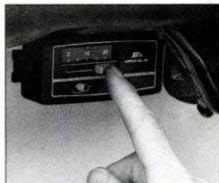
Control adds intermittent wiper action.
