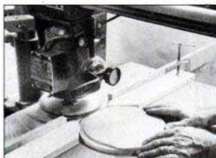
To cut rabbet on round stock, clamp mitered guide boards against fence and lock saw yoke in place. Rotate stock against blades.
