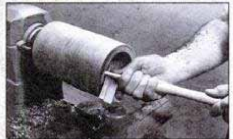
After squaring the log ends, mount it back on the lathe using a face plate to permit hollowing out the vase interior.
