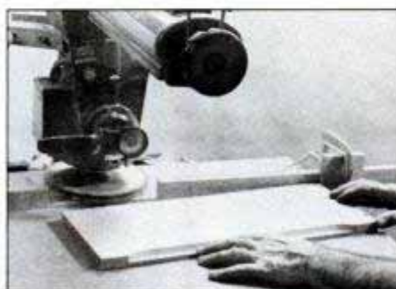
To cut stopped dados or blind grooves, clamp stop blocks to fence. Butt stock to rear block, then swing into rotating blades.
