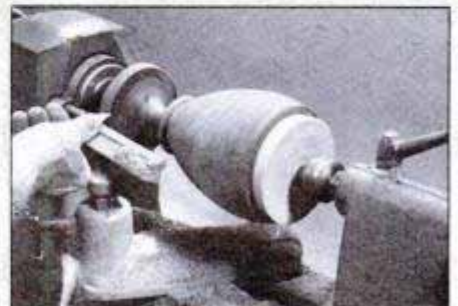
Increase the lathe speed as the vase nears completion. Faster rotation and light finishing cuts produce a smooth surface.
