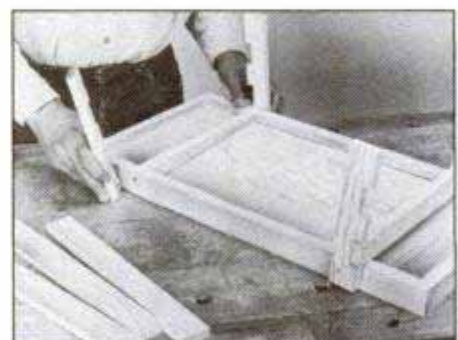
Glue hinge dowels into leg holes. When dry insert dowels into sides; then nail and glue leg crosspieces into notches.
