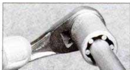
Gripping a totally stripped bolt head is no problem for the cam-action grip socket.
