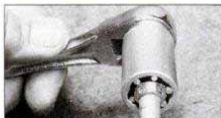
Gripping a totally stripped bolt head is no problem for the cam-action grip socket.
