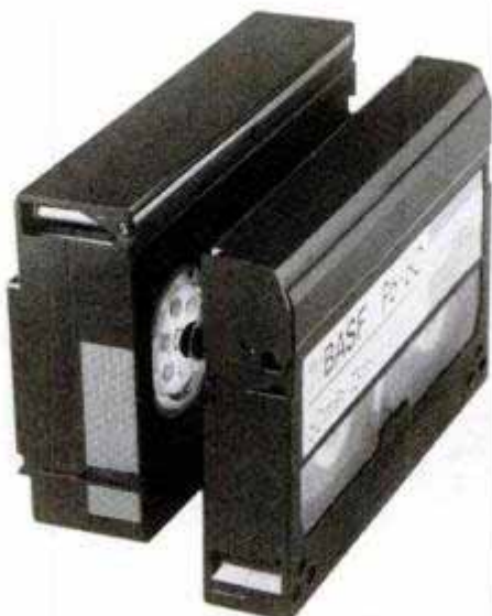
Two-hour 8-mm tape (right) is about the same size as 20-minute mini VHS-C tape.
