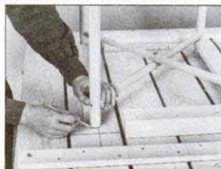
Place leg assembly in position and mark locations of the ¼-in.-deep leg holes. Keep tabletop overhang equal in both directions.
