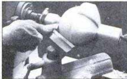
Turn the blank until the inked centerlines are barely visible. Then, finish-shape the piece using skew and spear-point chisel.
