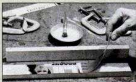
Glue up the turning blank separated by a strip of slick magazine paper. When the glue dries, turn the spindle on the lathe.
