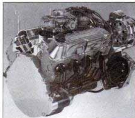
The 302 c.i. V8 has been pumped up to 210 hp with a roller tappet cam, dual exhausts.
