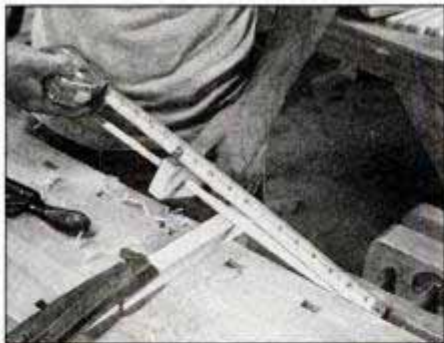
When carving spindles, check progress with tape measure and diameter gauges. All spindles must be exactly the same.
