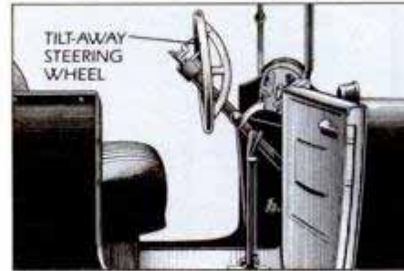
The 1914 Cadillac had a tilt-away steering wheel. The idea goes back at least to 1903.
