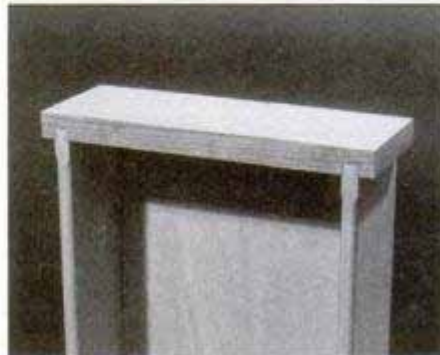
Although it's assembled with glue only, the dovetail dado joint is one of the strongest joints used in drawer construction.
