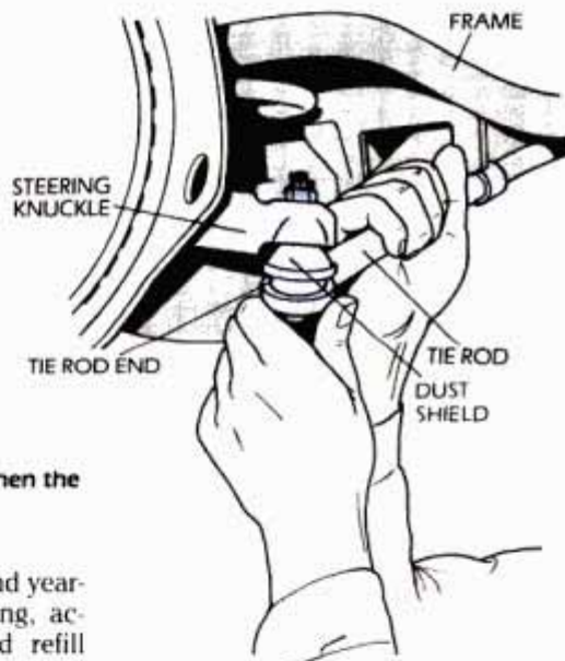
23 Tie rod ends should move some when wiggled, but not have excess freeplay.
