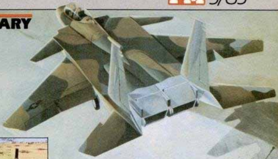
Modified F-15 will land and take off in 1,000 feet, a fraction of the mile or more normally required. Head-up display (left) tells pilot if he has room to land on bomb-cratered runway.
