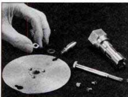
Hand crank components are shown above. Disk was made from a round electrical junction box cover plate. Drill disk center to accept drawbolt and mounting screws.
