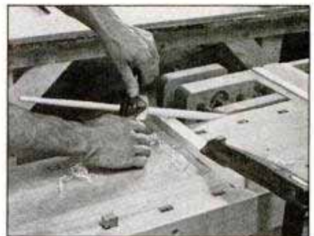
Clamp spindle blank in vise. Then, carve to shape using spokeshave or block plane. Turn work frequently for round shape.
