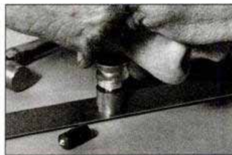
The optical center punch by Skidmore offers pinpoint accuracy for neater metalworking.
