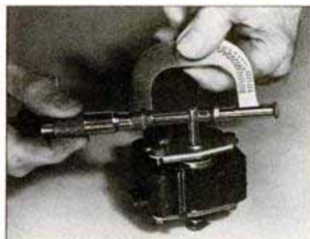
With the range doubler attached to the micrometer frame, you increase the measuring capabilities of a 1- to 2-in. micrometer to allow measuring from 0 to 1 in.
