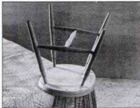
Glue stretchers to legs and legs to seat. Using a mallet, progressively tap bottom of legs until tenon shoulders hit seat.
