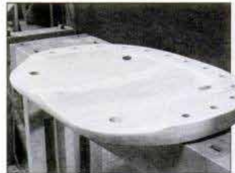
Finished seat ready for assembly has flat spindle rail, concave top with center rise, and rounded edges on perimeter of bottom.
