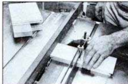
Use a standard table saw blade to trim the back of the drawer front dados. Use the miter gauge to ensure safe, accurate cuts.
