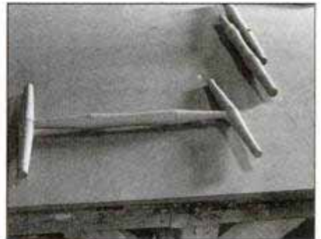
Glue center stretcher to side stretchers on flat surface so all parts align in one plane. Then, use single bar clamp at joints.
