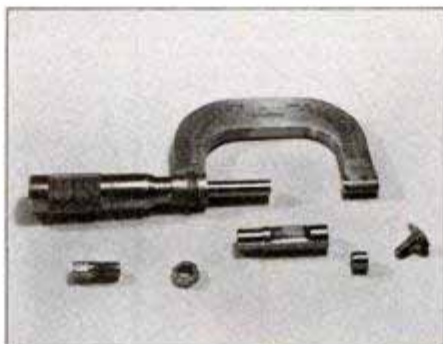
Disassembled range doubler is shown with a 2-in. micrometer. Parts are (left to right): anvil extension, hexnut, body, threaded plug and knurled locking screw.
