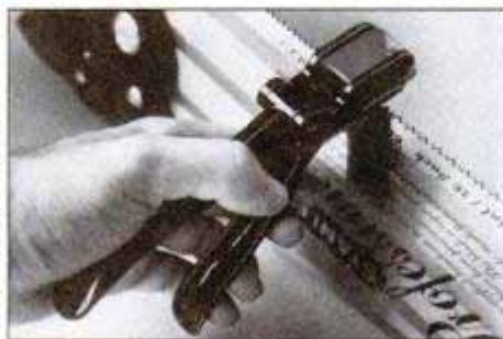
Pistol-grip saw set features a built-in magnifying lens that offers a clear view of the saw teeth alignment and condition. Use it on saws with from four to 12 teeth per inch.
