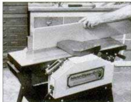
Jointer infeed and outfeed tables create a stable 36-in.-long surface for long stock. Fence tilts over to 45° for beveling jobs.
