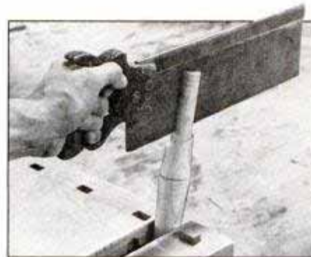
Use a backsaw to cut a kerf in each leg tenon perpendicular to direction of wood grain in seat. Kerf will receive wedge later.
