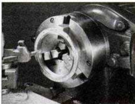
After machining the outside diameter of the blank, remove the ring from the plate and mount it in a jawed lathe chuck. Take shallow cuts to remove any residue solder.
