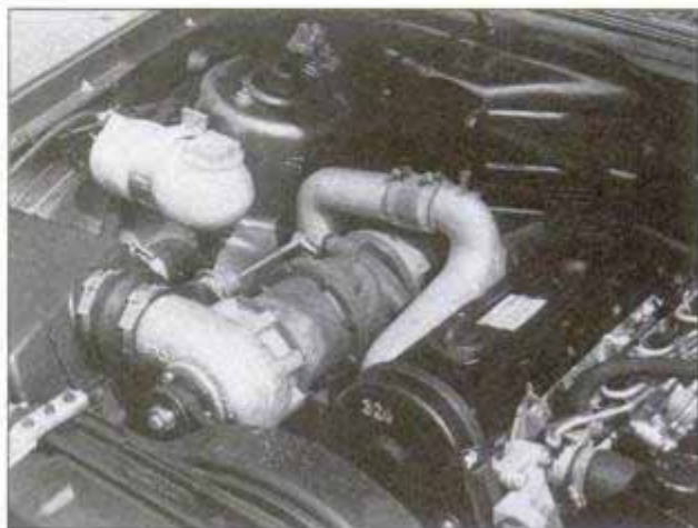
Installation of Comprex system is bulky, requiring a drive belt, intercooler and hookups to intake and exhaust manifolds.
