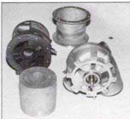
Channels in rotor (front) align with ports in exhaust and fresh-air housings (rear).
