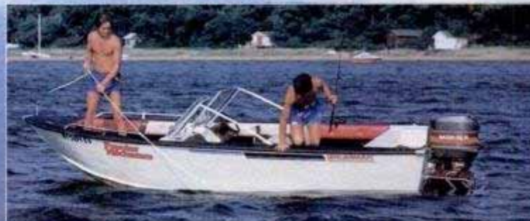
PM's Water Sportster project boat is based on a 16-foot aluminum hull Grumman Skidaddle. Power is by a 75-hp Mariner.
