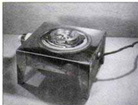
Use an electric hotplate to solder the blank to the support plate. Place flux and solder pieces around the blank. As the solder melts, it will be drawn between the parts.
