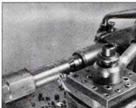
The body was machined from a 1 1/8-in.-dia. hexagonal bar, but a round bar could be used, too. Note that the tailstock center is used to steady the end of the bar.
