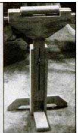
This roller support stand will improve the finish and the accuracy of thickness planing.
