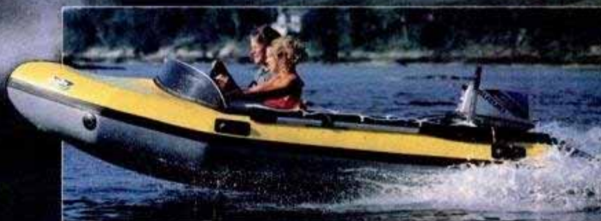
Achilles SR-140 is an inflatable with a rigid hull for a more comfortable ride. Boat moves out even with a small outboard.
