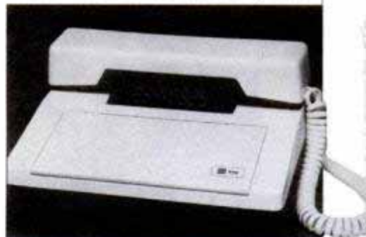
This dial-less telephone from TTC is made possible by voice recognition technology.
