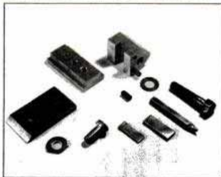
Disassembled setback toolholder is shown with two shims and a 1/4 × 1/4-in. bit. Long bolt fastens toolpost to setback plate; short bolt mounts plate to clamping bar.
