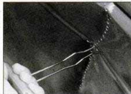
Drill holes 1/4 in. apart in the deepest part of the dent. Insert two or more rods into the center of the dent and pull gently.
