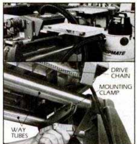
Wear mask (left) when planing lumber to keep dust out of your lungs. Some hardwood species produce toxic sawdust. A shop vacuum attachment (top, right) catches dust to avoid this problem. Mounting clamps (above, right) secure the planer on the way tubes of the Shopsmith Mark V. Spin clamp handles snug, then tighten a quarter of a turn.
