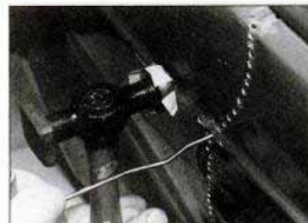
Use a hammer with a taped face to tap the surface near a crease while pulling at a right angle to the bodywork. Don't pry.
