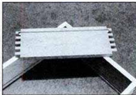
Note how the blind groove is contained within the piece to prevent it from being visible when the drawer is assembled.
