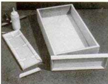
Create your own custom drawers by adding wood molding to the add-on faces. Attach the molding with glue and masking tape.
