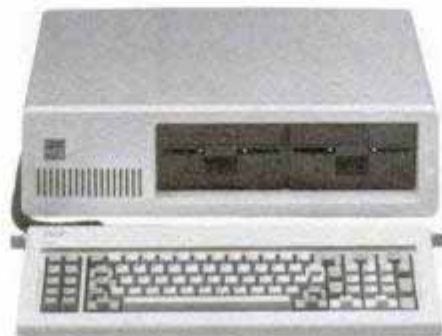
IBM's Personal Computer comes with 64K or 128K of memory, but has room for 256K.
