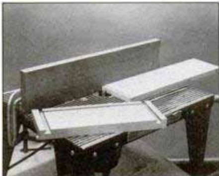
Cut the grooves for the drawer bottom with a 1/4-in. straight bit. Note that drawer front groove is contained between dados.
