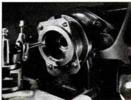
When the soldered joint cools, bolt the support plate to the faceplate separated by the spacer. Use a boring tool to cut the centerhole to the desired inside diameter.
