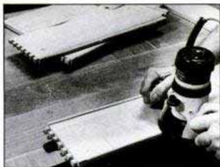
Shape top edges of the drawer sides with a 1/4-in. rounding-over bit. Stop cut 1 in. from end so it doesn't interfere with the joint.
