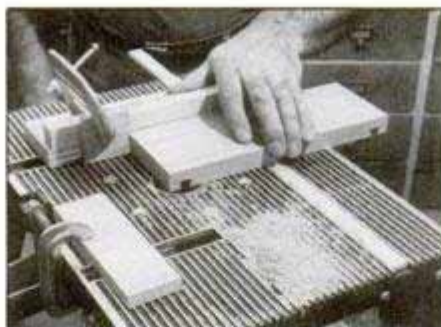
Cut the dovetail dados in the drawer front using a router table and a dovetail bit. Guide the work with the miter gauge.
