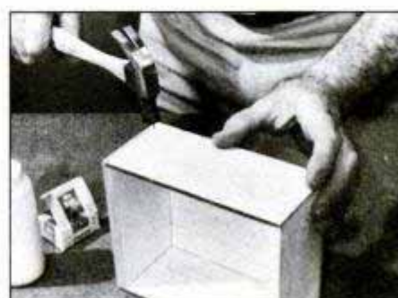
Assemble the drawers with glue and 5/8-in. brads. Fronts and backs are 1/2-in. pine; sides and bottom are 1/4-in. plywood.
