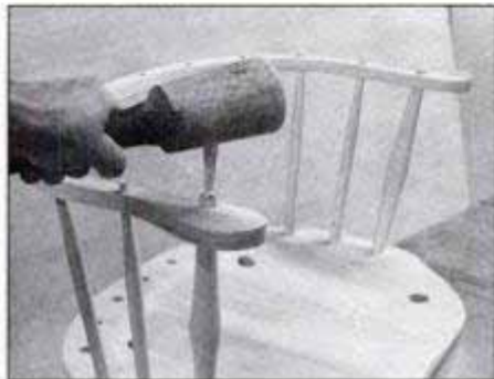
Glue and wedge arm posts and short spindles to seat from below; to arm rail from above. Cut ends flush with dovetail saw.
