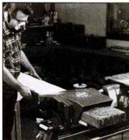
Wear mask (left) when planing lumber to keep dust out of your lungs. Some hardwood species produce toxic sawdust. A shop vacuum attachment (top, right) catches dust to avoid this problem. Mounting clamps (above, right) secure the planer on the way tubes of the Shopsmith Mark V. Spin clamp handles snug, then tighten a quarter of a turn.
