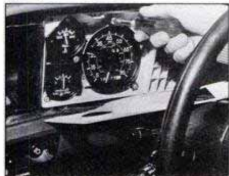
Late-model dashboards are going "front-service," for repairs from the driver's seat.
