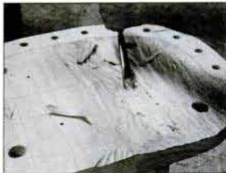
Transfer seat profile from drawing onto front edge of blank. Then, carve rough shape using mallet and 3/4-in. or 1-in. gouge.
