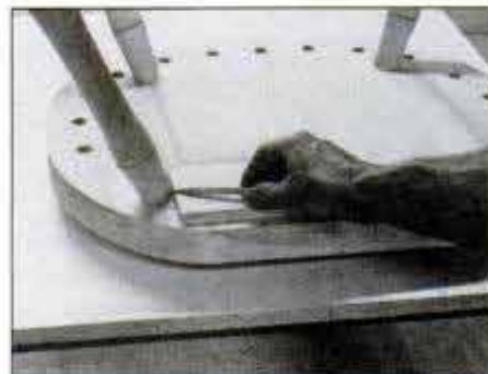
Mark position of angled shoulder for each leg tenon by scribing circumference of leg with pencil resting on 1/2-in.-thick block.
