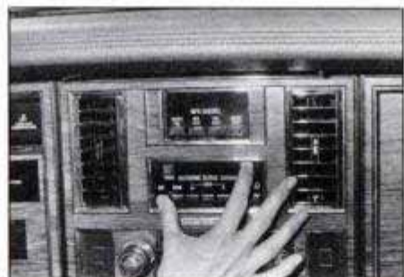
Cadillac self-diagnostic system is triggered through a/c controls, displays trouble codes.
