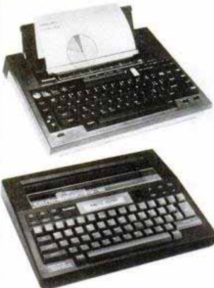
Lightweight, portable electronic typewriters from Panasonic (top) and Casio also function as computer printers.
