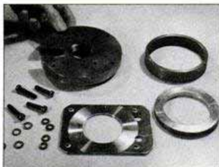
Here are the components needed to turn distortion-free rings (clockwise from upper left): faceplate, spacer ring, turning blank and support plate with mounting bolts.
