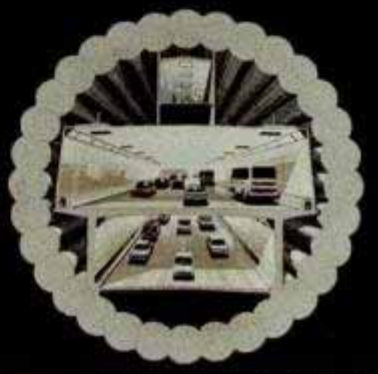
Cross section above shows how ring of concrete "logs" encases three-level tunnel. At left, a 55-ton boring machine digs perimeter tunnels.
