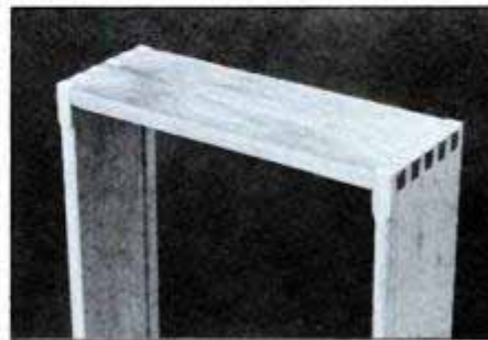
Assemble box joints with glue only. These joints often are used to join both the drawer front and back to the sides.
