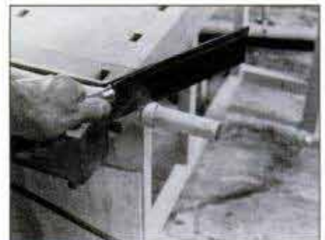
Clamp leg in vise. Then, carefully cut angled shoulder using dovetail or backsaw. Pare waste from tenon using sharp chisel.
