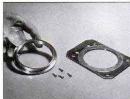
Here's the completed ring (left) and the support plate. Before reusing the support plate, bolt it to the faceplate and take very shallow cuts to clean the soldered surface.
