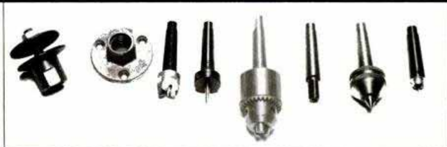
Lathe accessories (left to right): screw on arbor for mounting grinding and buffing wheels; face plate; spur center; screw center for small, delicate work; geared chuck for boring operations; adapter; ball-bearing center; and cup (dead) center.
