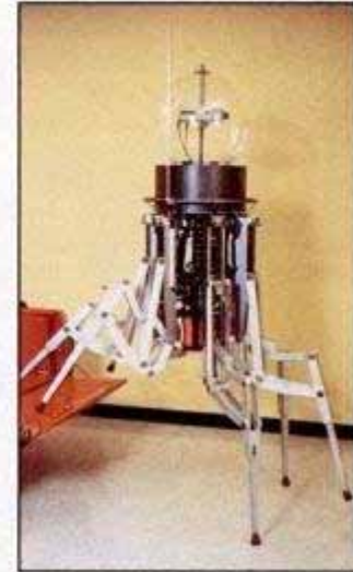
The Odex from Odetics is the first commercial walking robot.
