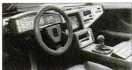
Quasar dash is cantilevered off of the center tunnel; electronics system is from Clarion.
