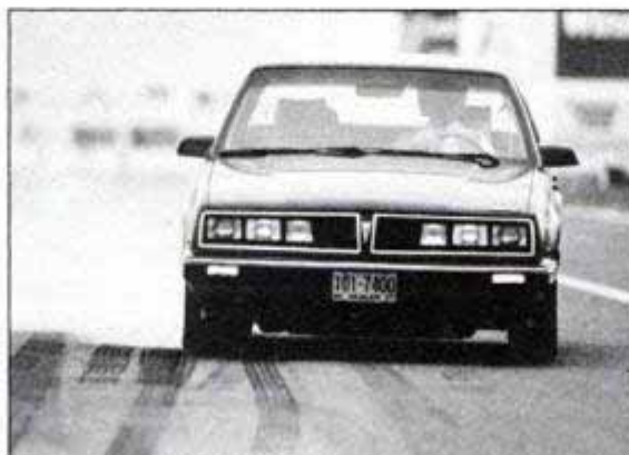
Four-wheel disc-equipped Pontiac 6000 STE outbraked the disc/drum Eurosport, but was bested by Ciera and Century A-bodies with heavier 3.8-liter engines up front.
