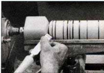
Round the top of the shoulder with a skew. Hold the blade flat on the toolrest and swing the handle slowly to the right.
