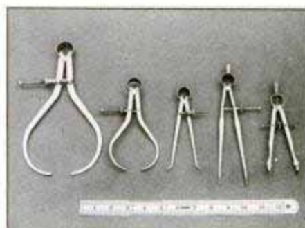
Essential measuring tools include (left to right): two sizes of outside calipers, an inside caliper, dividers, compass and rule.
