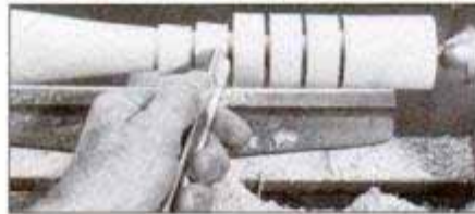
Make a long taper by first cutting diameter-sizing grooves with a parting tool. Then, remove the waste, as shown, with a gouge.
