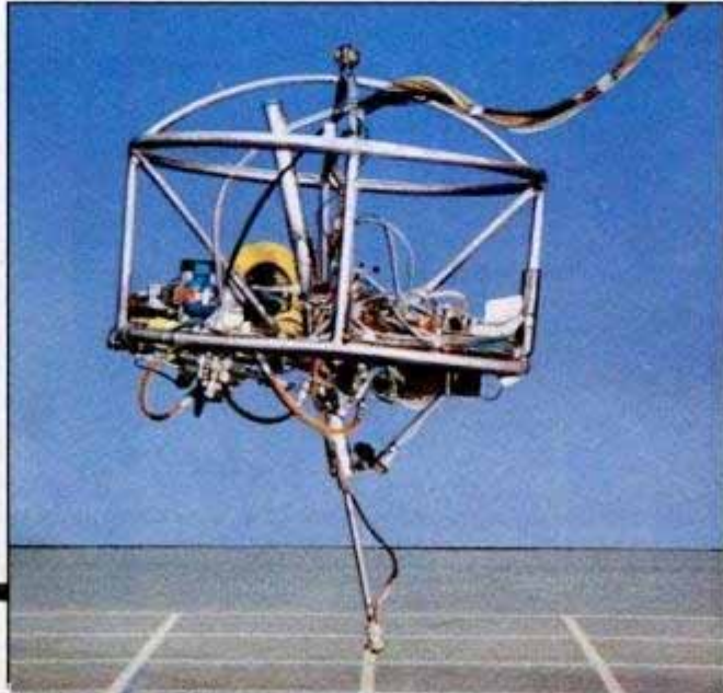
Marc Ralbert's one-legged hopping machine carries a balance rig that moves up and down by compressed air on spring leg.
