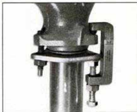
Clamp will replace broken manifold studs.
