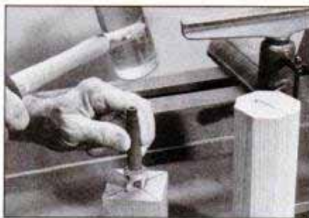
Drive in the spur center with a mallet. Reference mark on blank end corresponds to mark on spur center to permit recentering.
