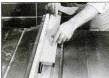
Cut duplicate rabbets against fence because one fence adjustment yields same cut even if boards vary slightly in width.
