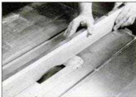
To make cuts against fence with wobbler blade, attach board to fence, then slide over rotating blade to cut recess in wood.
