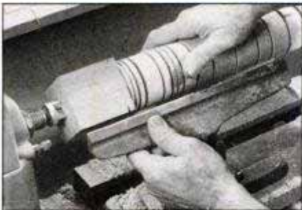
When repositioning the toolrest opposite the square shoulder, rotate the blank by hand to make certain there's clearance.
