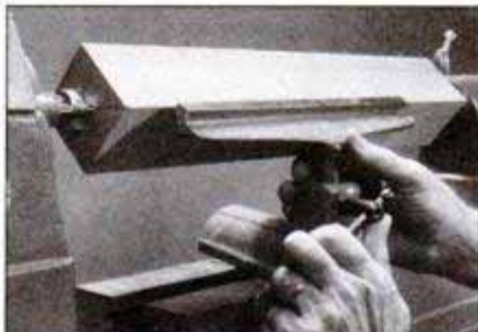
Adjust the toolrest so it's no more than 1/8 in. away from the blank and approximately 1/8 in. above the spindle centerline.
