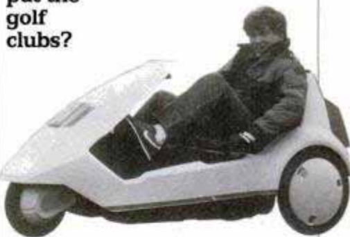
Sinclair C5 electric is steered by the front wheel; handlebars are under your knees.
