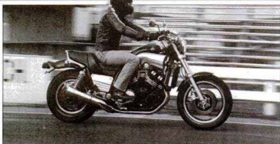
Yamaha V-Max is quick off the line with its 145-hp V4. The 1,200-cc liquid-cooled engine uses four valves per cylinder.
