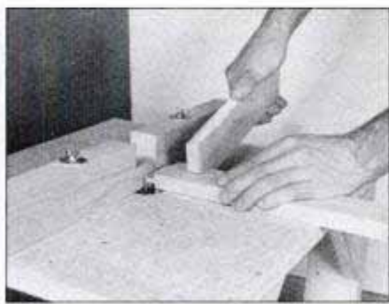
Cut tenons on rail ends with same cutter used for door panel groove. Tenons require at least two cuts per side to remove waste.
