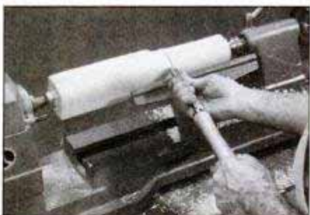
Using a gouge, start cutting a few inches from the end. Cut toward and off the end. Repeat this procedure on opposite side.
