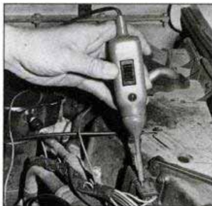
Versatile tester can also apply 12-v. power.
