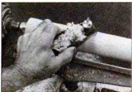
Cylinder can also be finish-cut to size using a block plane. Set plane for a very shallow cut and slide it along the toolrest.
