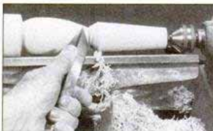
Shaping convex curves with a skew is similar to cutting long tapers. Always work downhill from the high point of the curve.
