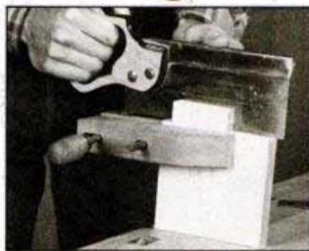
Clamp a blade guide block to sides and cut tenons with backsaw. Or make cuts using radial-arm or table saw, with blade set to remove 1/8 in. of waste from each surface.
