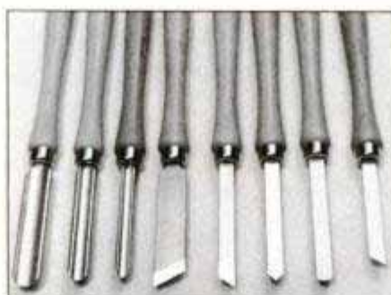
Complete set of basic turning tools includes (left to right): three gouges, two skews, a spear-point, round-nose and parting tool.
