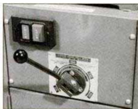
The variable-speed drive mechanism, shown on a Delta lathe, allows quick selection of any speed between 340 and 3,600 rpm.
