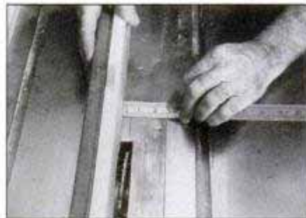
Adjust fence for rabbet by measuring from pencil lines. If table won't take marks, apply a piece of masking tape and mark it.
