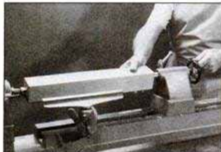
With the tailstock clamped in position, turn the hand wheel to advance the tailstock ram which drives the cup center into blank.
