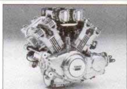
Yamaha V-Max is quick off the line with its 145-hp V4. The 1,200-cc liquid-cooled engine uses four valves per cylinder.
