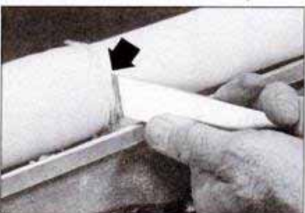
Use a skew to finish-cut the cylinder to size. Cut with the blade's center section only. Toe (arrow) must not make contact.
