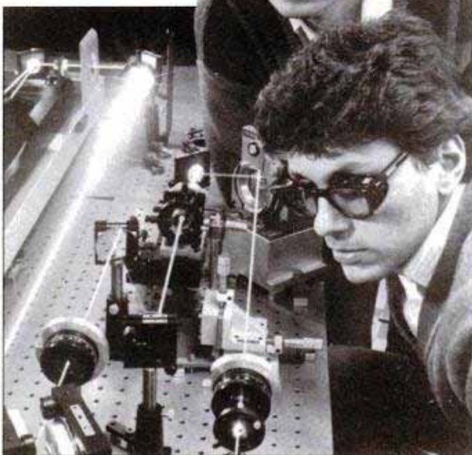
Ford researchers aim laser at experimental cylinder to measure engine heat loss.
