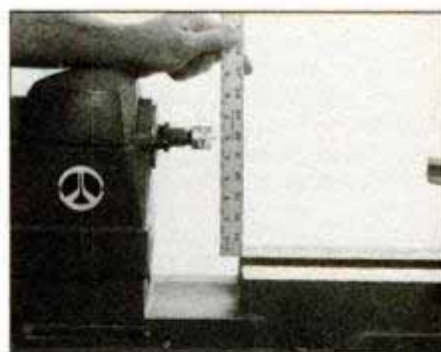
Determine the swing of a lathe by doubling the distance from the spindle center to the bed. This lathe has a 12-in. swing.
