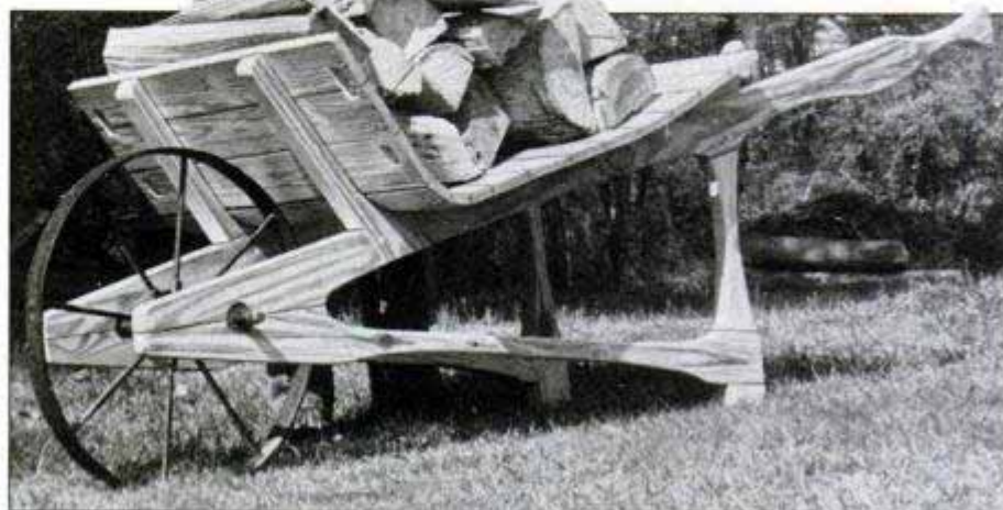
Removable sides allow easy loading. To unload soil or cut grass, remove one side and tilt the wheelbarrow.
