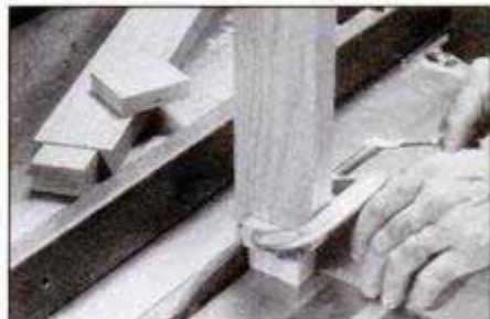
Clamp the rail to the miter gauge to cut edge cheeks. Wood block in background is used to position the rail before clamping.
