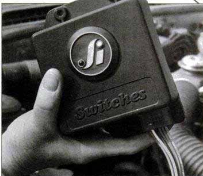
Replacement ignition module uses LEDs to report on its own status.
