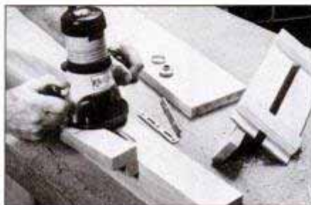
Make two short, deep plunge cuts in the post mortises to accept the rail plate hooks. L-shaped guide on router controls cuts.
