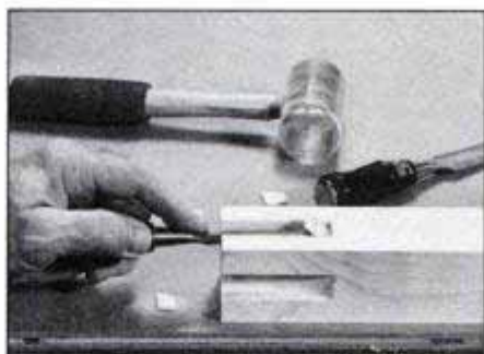
Cut the open mortises in the square leg blank using a dado blade in a table saw. Square the mortises with a sharp chisel.
