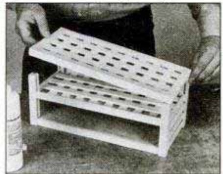
Glue lower grid in place, then glue and nail top to corner posts. If you plan to stain, apply before the top is mounted.
