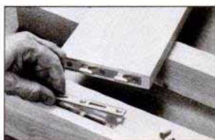
After routing the mortises, attach the fasteners to their respective parts. Completed bed rail is shown in the background.
