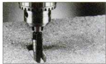
The high-speed steel bit can also be used to cut through particleboard and plasterboard. Move the drill with a sawing motion.
