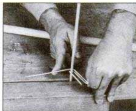
Bend \frac{1}{8} -in. brass rod around a 1-in. dowel to form the large curve, and around a \frac{1}{4} -in. dowel to form the small curve on pot hook.
