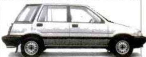
Honda Civic wagon with four-wheel drive is 1.1 in. taller than its fwd counterpart.
