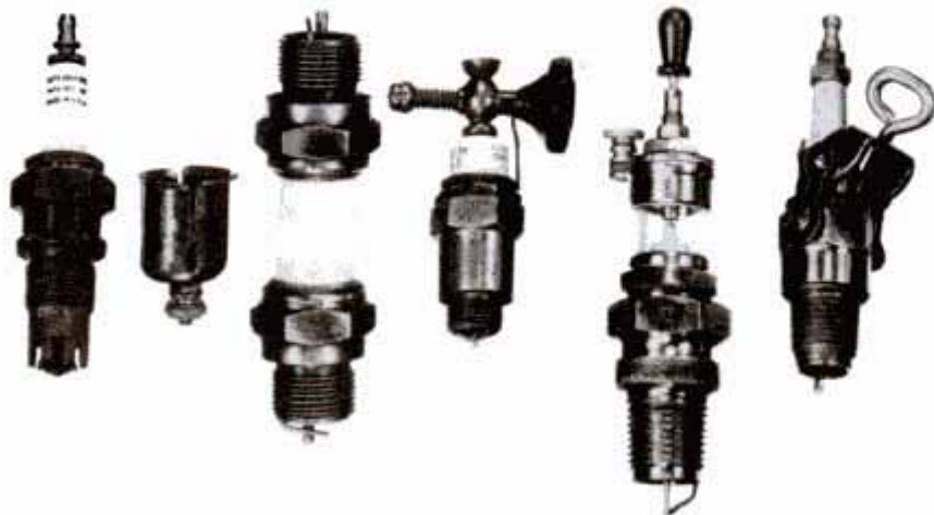
Antifoul plugs (left to right): Fan Flame model with rotating electrode; terminal/cap and double plug could be reversed when fouled; priming plug lets you pour gas into cylinders for starting; adjustable gap blasted deposits; removable core allowed quick cleaning.
