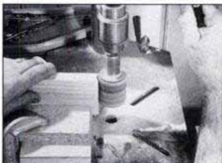
Use a sanding drum chucked in a drill press to smooth the rail ends. Be sure drum size matches the desired leg diameter.
