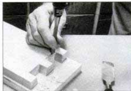
Cut pins like tails were cut using dovetail and coping saws. Then, trim sides of pins square with chisel before cleaning crosscut.
