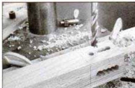
Form blind mortises by boring a series of overlapping holes. Brad-point bit keeps the bit from sliding into the adjacent hole.
