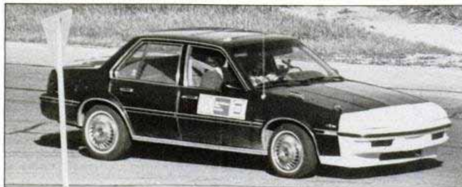
Bolt-on aerodynamic nose cap with pop-up headlights could transform Cavalier/Sunbird.
