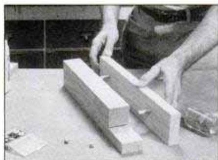
Now attach a third board to the leg using glue and dowel pins. This will form a notched seat for mounting the rails.
