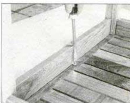
Turn tabletop and base upside down and center base on top. Bore screw pilot holes into rails using fasteners as guides. Attach top by screwing fasteners in place.
