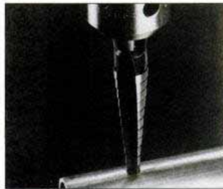
The nonskid tip starts on curved surfaces such as pipe and conduit. Stop boring when the desired hole diameter is reached.
