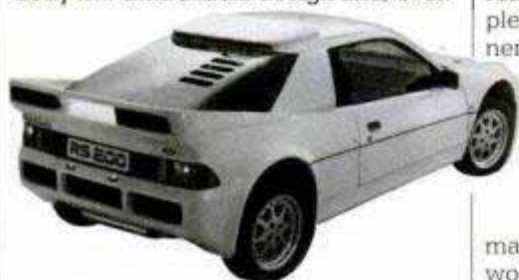
Turbo intercooler of the mid-engine RS 200 is aerodynamically integrated in the roof.
