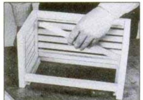
Glue floor supports in place, then notch the rear floor slat to fit around the corner posts. Glue remaining floor slats in place.
