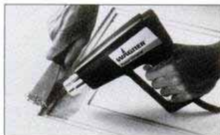
Apply heat until the paint starts to blister, then remove it with a putty knife or scraper. It works on both latex and oil paints.
