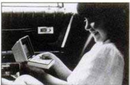
The color liquid crystal display screen of the SuperMicro game console closes up like a clamshell for portability.
