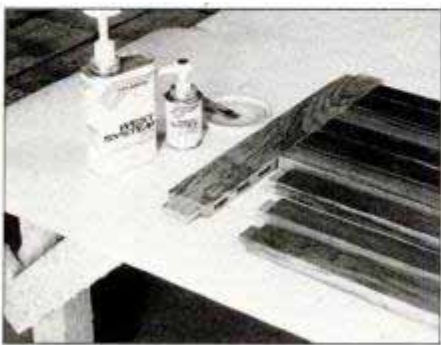
Begin assembly of tabletop by gluing top slats into one end rail. Then glue opposite end rail in place, followed by both side rails. Check assembly for square; let dry.
