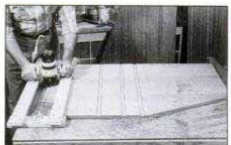
Cut the rabbets and dados in the sides using a router and straight bit. Be sure the interior surface is facing up. Build a guide, as shown, to keep router on course.
