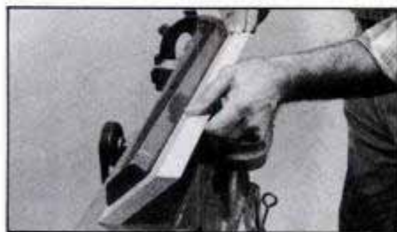
The safest way to cut bevels is with the fence tilted in to form a closed angle. This makes it easier to keep the workpiece in close contact with the fence and table.
