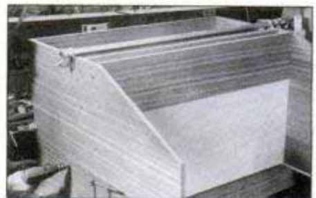
Assemble the desk with shelves and bottom in place. Then, bore screw pilot-holes. Place shims under the shelves to hold their front edges flush with the side pieces.
