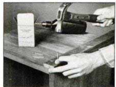
Assemble chest with glue and 5d cut nails; attach trim with glue and 4d cut nails. Bore 1/32-in. nail holes to avoid splitting wood.
