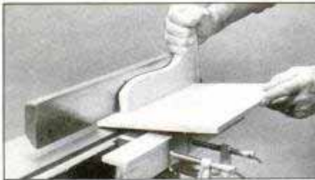
Cut raised panels for cabinet doors on the jointer with the aid of a push stick. Clamp a wood block to the rabbeting ledge to support the workpiece at the desired angle.
