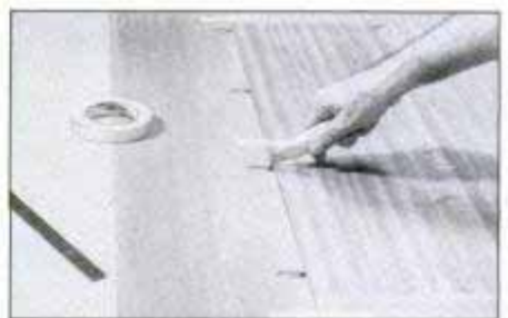
Transfer hinge mortise positions from main shelf to the lid using a utility knife. Tape parts to prevent shifting. Rout lid mortises using the knife marks as guides.
