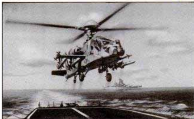
Proposed Navy version of Hughes Apache carries antiship Harpoon missiles and has a target-spotting radome above rotor.
