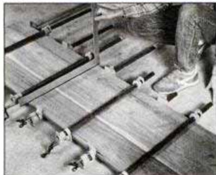
Straighten board edges with a jointer, then match for pleasing grain. Glue and clamp, alternating clamps top and bottom.
