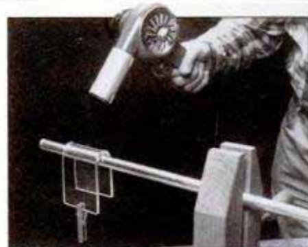
Acrylic plastic up to 1/4 in. thick can be bent using a heat gun. Choose metal tubing of proper diameter and direct heat at bend.
