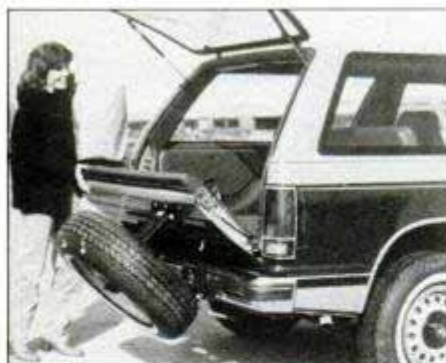
Spare rack leaves tailgate operation normal.
