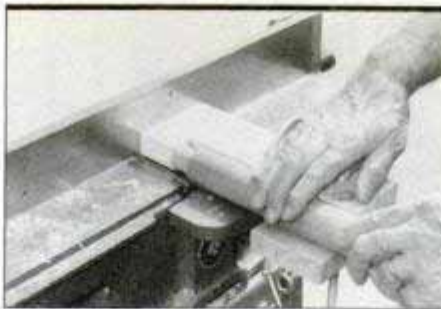
Cutting round tenons is handled easily with the aid of an L-shaped jig. Clamp the jig to rabbeting ledge. Push the work into the spinning knives and rotate clockwise.
