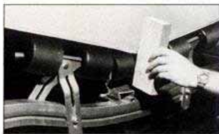
Cox trailer is galvanized and has 1,600-lb. capacity. Check the boat's position on trailer with a straight-edge (above, left). Recheck adjustment bolt tightness after the first few hours of trailering (above, right).
