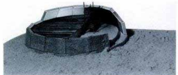
As courses of brick are laid, bottoms are cut at increasingly steeper angles, causing the walls to bend toward the middle. Wood placed atop platforms made of snow provides sleeping area.
