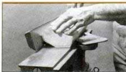
Contouring workpieces into irregular, free-form shapes is possible on the jointer. First, make a series of shallow chamfer cuts to form the basic shape of the piece.
