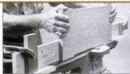
Advance the workpiece slowly past the cutterhead to the stop block. Install an auxiliary fence with extension tables, as shown, to support oversized workpieces.
