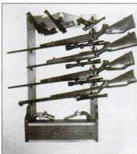
PM's "upside-down" gun rack built by reader Johnson. It keeps wood stocks oil-free.
