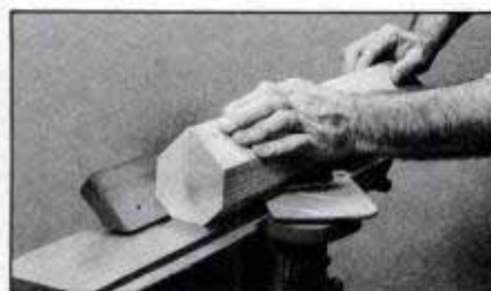
Here's a quick and easy way to make an octagon: Set the fence to 45^\circ . Then, chamfer the corners of a square workpiece. Make the same number of passes for each corner.
