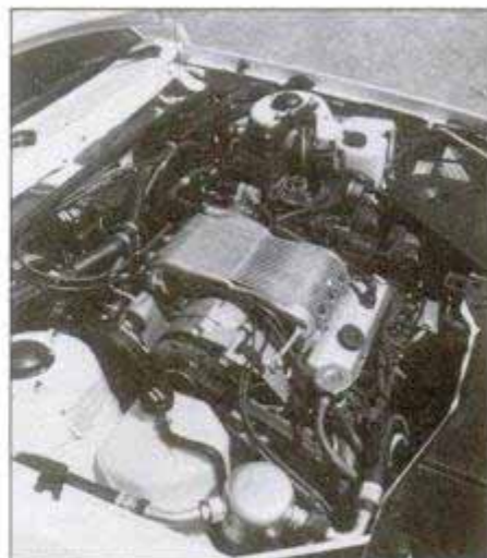
Transverse 2.8-liter V6 has a ribbed fuel-injection plenum that looks like a finned oil pan, leading to upside-down motor jokes.
