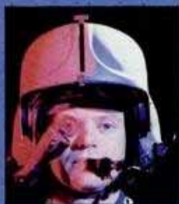
Target-spotting sight attaches to pilot's helmet so that it looks wherever he looks.
