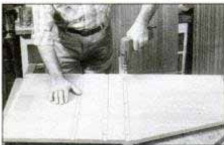
Bore screw pilot holes in the center of the dados and bottom rabbet. Position a scrap board under the desk side to prevent splintering caused by exiting bit.
