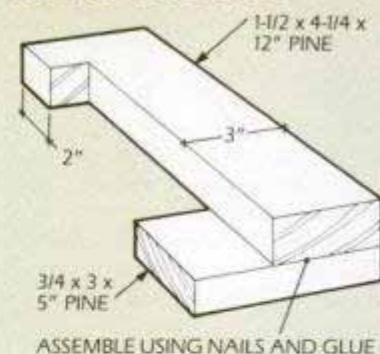
Cutting round tenons is handled easily with the aid of an L-shaped jig. Clamp the jig to rabbeting ledge. Push the work into the spinning knives and rotate clockwise.
