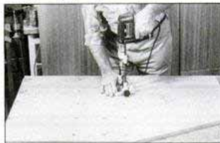
Turn the desk side over so that the dados face down. Now counterbore each screw location for 1/2-in.-dia. mahogany plugs. Use a drill guide to keep the bit perpendicular.
