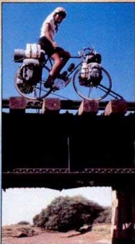
The single bicycle rode the tracks with its fork extension on one rail and an outrigger for balance attached to the other rail.
