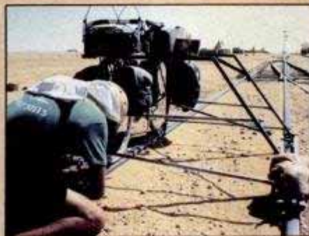
Guide bars were built to run along inside of the railroad track up to the bike's axles.
