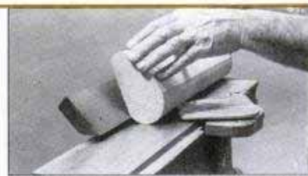
Finally, finish-shape the workpiece with the jointer adjusted for very shallow cuts. Use the fence to guide the piece straight. Hand-sanding completes the project.
