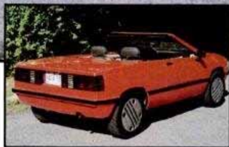
Clever two-piece rigid top uses stock Honda rear window, including defroster. Flush wheel covers snap over Honda wheels.
