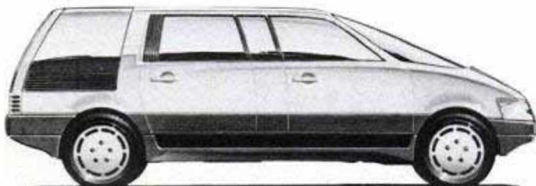
Precedent will use steel doors and a fiberglass-sandwich body to provide custom-van luxury without trucklike ride or styling.
