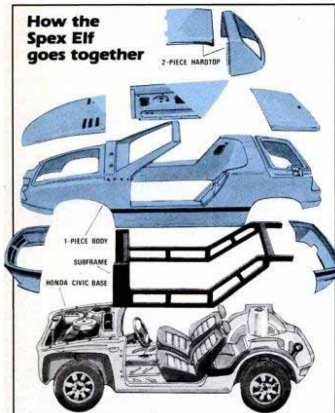
Honda Civic chassis, minus bodywork, retains all of its modern features—transverse-engine, front-wheel drive, MacPherson strut suspension. Unibody platform is reinforced with steel subframe.
