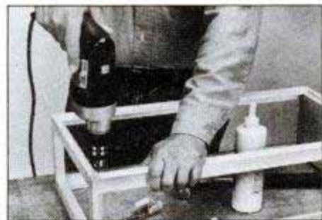
Bore pilot holes for all nails before gluing. Glue and nail together the four corner posts, then glue and nail these assemblies to the top and bottom pieces.
