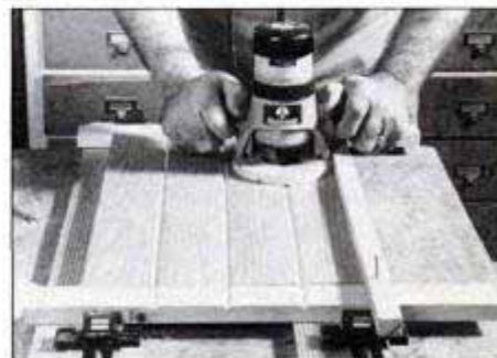
Cut grooves along the glue-joint lines using a router and a V-groove cutter. Set the depth-of-cut to \frac{3}{16} in. Use a straightedge guide to control the router.
