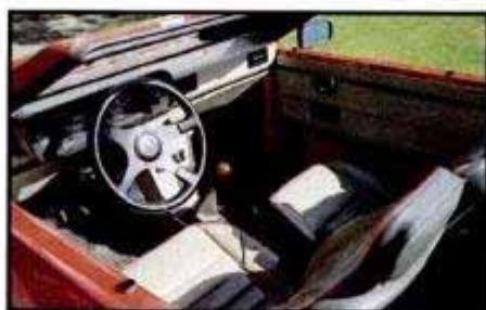
Lovely design looks like it was done by GM or in Italy. Stock Honda seats and instruments bolt into the modern Spex interior. You can use the Honda steering wheel, too, although the sport wheel is shown here.
