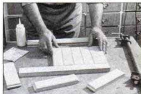
Assemble the door on a flat surface. Apply glue sparingly to all contact areas. Then, clamp door square using three bar clamps.
