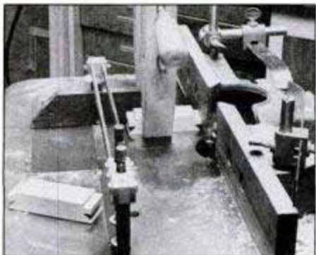
Clamp the short cross-rail pieces to the miter gauge when making the coping cuts. Never try to hold the rails by hand. Position the front fence to act as a stop block.
