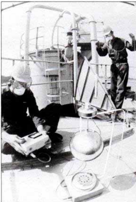
British scientists use metallic sphere to collect electrons to help explain "spontaneous" silo and pipe explosions.
