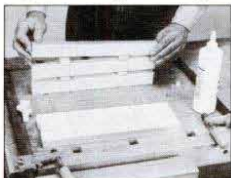
Draw layout lines on the tabletop and shelf slats to position spacers accurately. Then glue and clamp the parts, making sure that spacers remain properly aligned.
