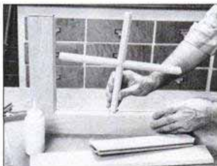
Glue the two-piece muntin to either side of the mullion. Once the glue dries, glue this cross-shaped assembly to one stile and rail. Then add the other stile and rail.
