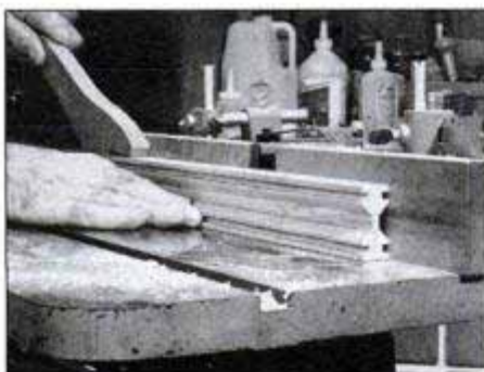
Make the mullion and muntin from a single board. Mill the sticking, as shown, on the shaper. Note the use of a push stick. Saw the board in half to obtain two parts.
