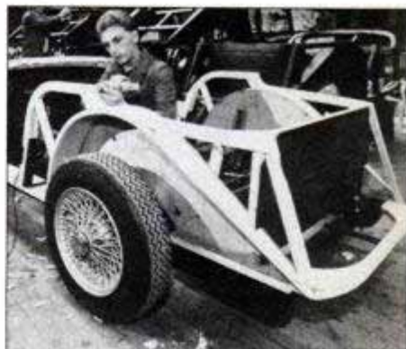
The framework for the Morgan hand-beaten steel and alloy body is white ash.
