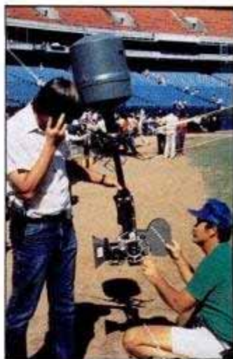
Skycam (above) runs on cables to move over its subject, as shown in drawing (below).
