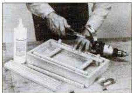
Attach outer slats of cutting board with supports in the crumb box to maintain proper spacing. Then remove cutting board and attach remaining slats.
