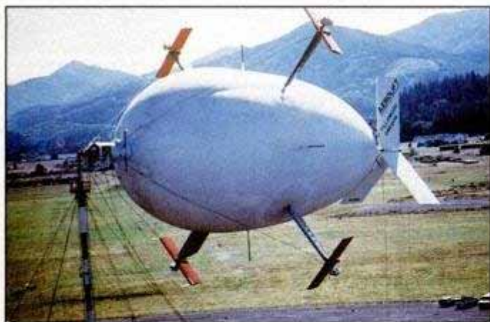
Small test model lifts 2 tons. Larger versions will haul 16 tons.
