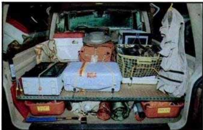
The Bronco II is ready to accept the full complement of gear we've assembled behind it (top). The double-decker setup (above) is provided by the 4x4-foot Peg-Board.
