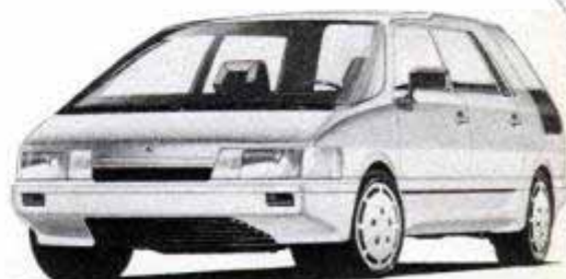
Precedent will use steel doors and a fiberglass-sandwich body to provide custom-van luxury without trucklike ride or styling.
