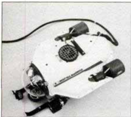
The Mini-Rover is a tethered and remotely operated deep-sea sensing machine.
