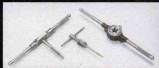
Two-handed tap and die wrenches provide leverage for cutting large diameter threads. The one-handed T-handle wrench (center) uses small taps.
