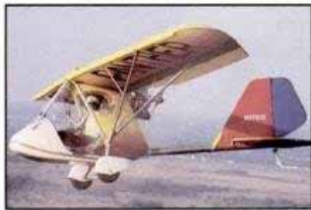
A 12-cubic-foot baggage compartment makes the Panther ideal for cross-country cruising and camping. Kit-priced at $5,800, it has full-span ailerons, removable wings, steerable tail wheel and a 28-hp engine.
