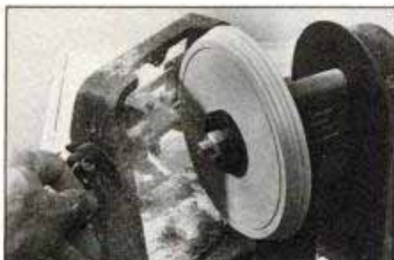
Feed the cutters first through the front surface, then into the back. The cutters are controlled by turning the advance handle.
