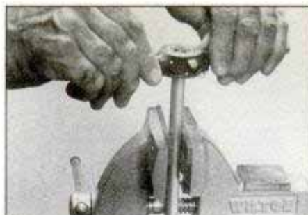
With the guide adjusted, insert the die with the tapered side down. To start die squarely, hold stock with both hands near the center, bear down and rotate clockwise.
