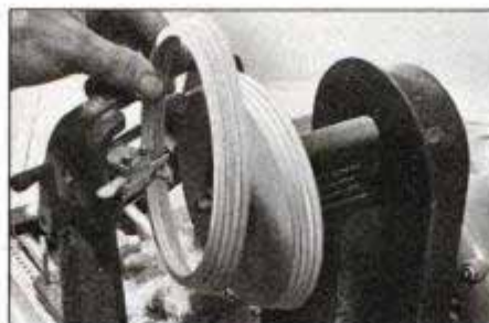
A severed ring with beveled, splinter-free edges drops neatly away from the blank. Advance the carriage for progressive cuts.
