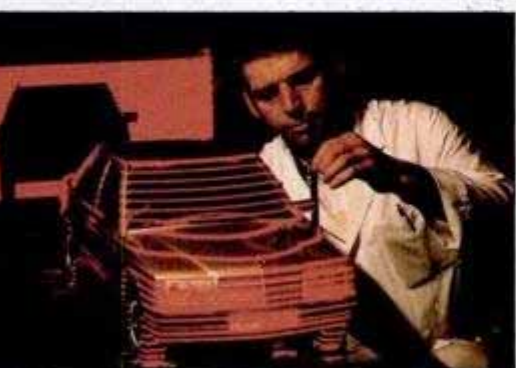
Daimler-Benz engineer uses laser beams to measure the contour of a model car body (above). A laser-equipped truck (right) passes through a train tunnel, its pencil-thin lights bouncing off the wall to measure the tunnel before completion.
