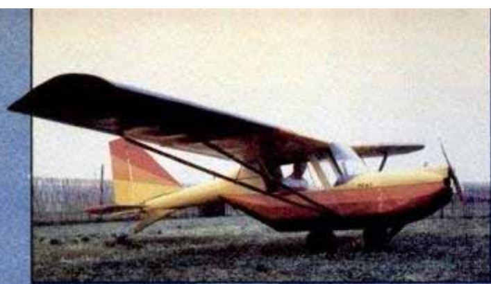
A big, fully enclosed cabin offers all-weather comfort in this high-wing Pony monoplane. The craft does 60 mph on only 25 hp, burns less than 2 gallons an hour, will sell for under $10,000.
