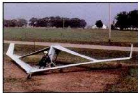
Trident T3 has a 32-foot wingspan and power-off glide ratio of 15 to 1, giving it near-sailplane performance. Its high-lift, twin-wing design is said to be inherently stable, easy to fly and difficult to stall.
