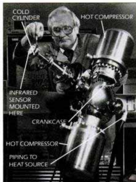
Space-based infrared sensors are kept cool for years with Hughes refrigeration system.
