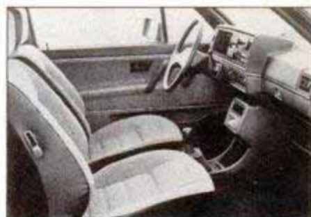
Golf/Jetta dashboard switches are placed high for an almost "heads-up" type display.
