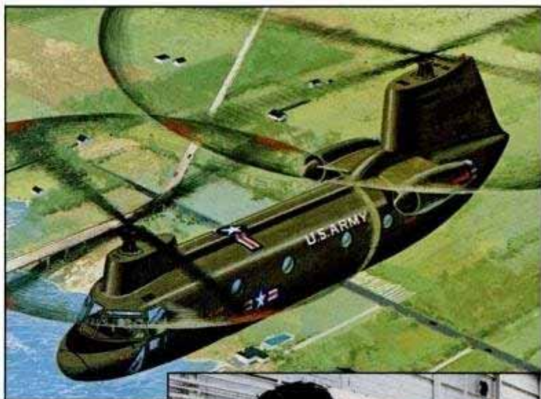
Artist's conception of a new all-composite tandem-rotor helicopter now under construction. Most fuselage parts are bonded with high-strength adhesives, eliminating even metal fasteners.
