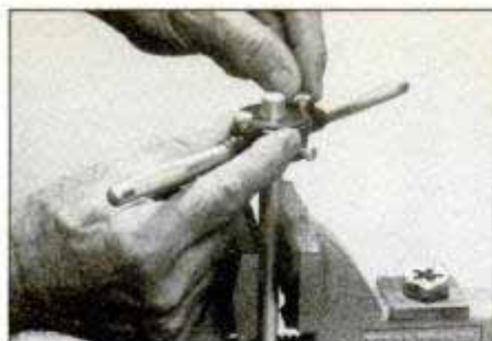
Before inserting the die, position die stock with adjustable guide facing up. Align guide to ensure straight threading, then tighten the guide's holding screws.
