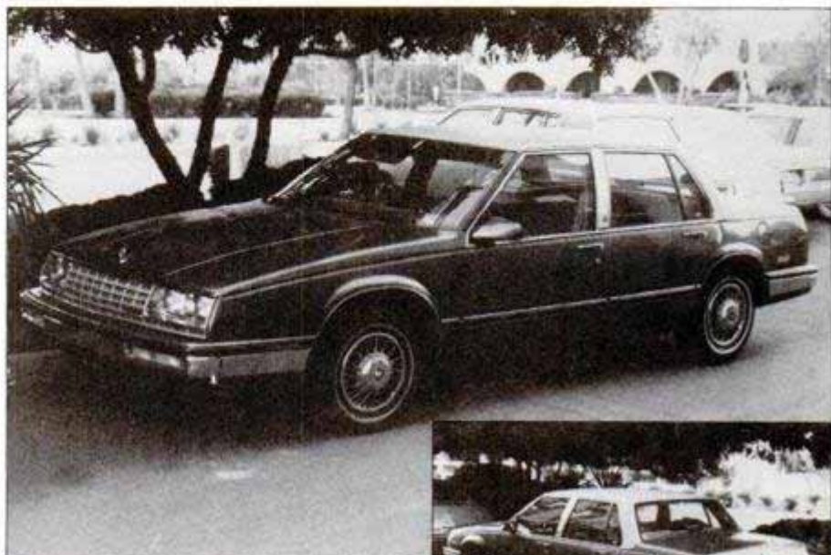
Our spy photographer caught the downsized Buick B-car near its desert test site. The '86 LeSabre will be 610 pounds lighter and 20 in. shorter than its rear-drive namesake.
