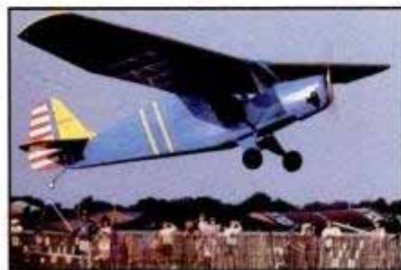
Survivability is a key design feature of this 28-hp Wren. Pilot is surrounded by an energy-absorbing "crash tub" for impact protection. Craft can be built from a kit for about $6,000 or from plans for $100.
