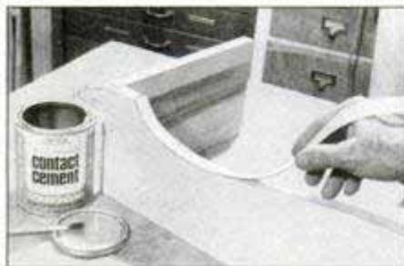
For curved edges, where using an iron to apply adhesive backed veneer tape is impractical, use plain hardwood veneer tape instead. It is attached with contact cement.
