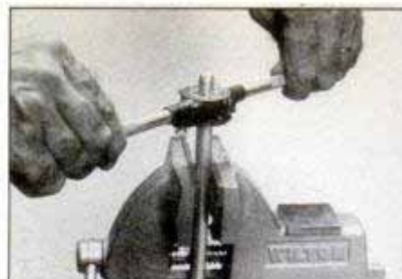
After the first few threads are started, move hands to handle end. Downward pressure can be relieved, since die self-feeds as it's rotated due to screwing action.
