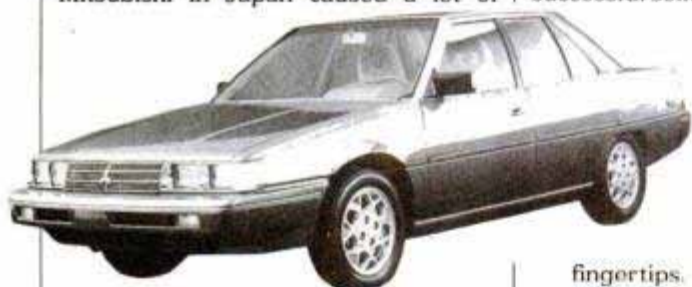
Galant's got electronic o.d., suspension, steering; radio controls on steering wheel.
