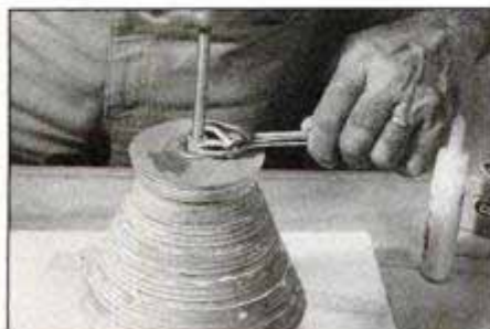
The accessory clamping jig is available for gluing up rings into the rough project shape.
