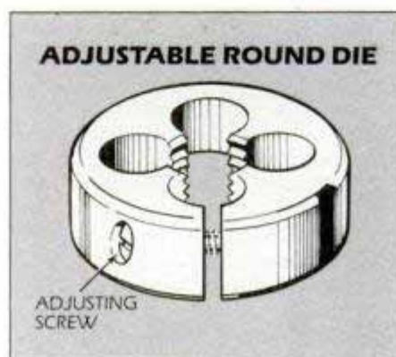
Adjustable round die cuts standard-size threads on bolts and rods, but slot allows minute adjustments for cutting oversized or undersized threads. The adjustment is made by turning setscrew on edge of die.
