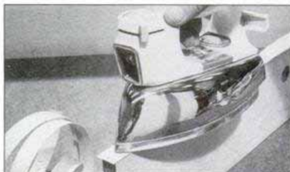
Adhesive-backed hardwood veneer tape is applied directly to edge with a few passes of hot clothing iron.
