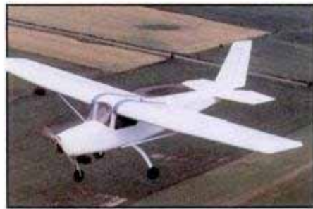
You can't get much closer to a real-plane look than this 27-hp, enclosed-cabin Solo, said to be the first all-composite ultralight. Priced at $15,000, it comes with instruments, wheel brakes, steerable nose wheel.
