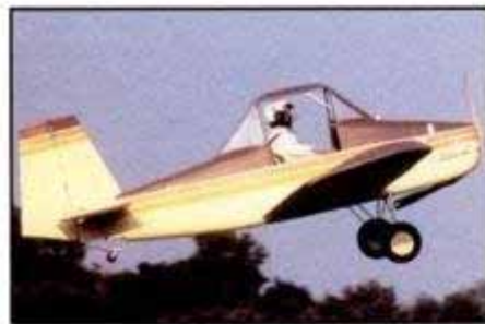
A rare low-wing design, the Bobcat has the high cockpit and good visibility of a crop duster. Features include removable wings and a 25-hp mill with electric start. Plans are $100; construction cost, about $3,000.
