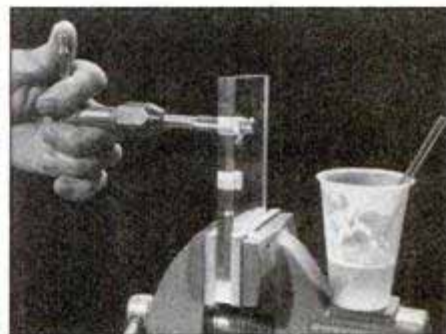
Acrylic plastic accepts threading well. Use the same tap drill sizes as for metal and lubricate the tap with soapy water.
