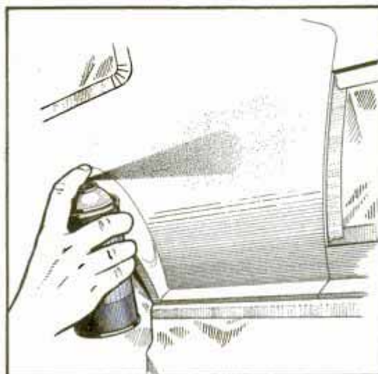
6 Once the surface has been sanded to a shiny smoothness, apply a finishing primer that will be compatible with the final color coat.
