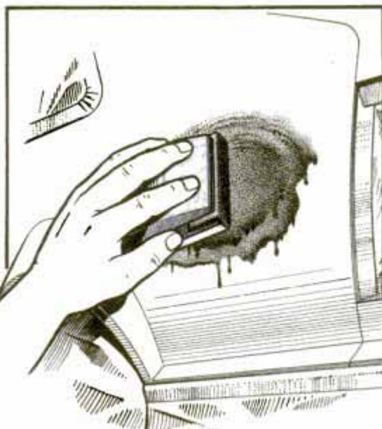
5 When the glazing putty has dried, wet-sand with 400-grit paper. Splash water on the area as you sand to flush away sludge and keep the paper fresh.
