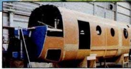
Artist's conception of a new all-composite tandem-rotor helicopter now under construction. Most fuselage parts are bonded with high-strength adhesives, eliminating even metal fasteners.
