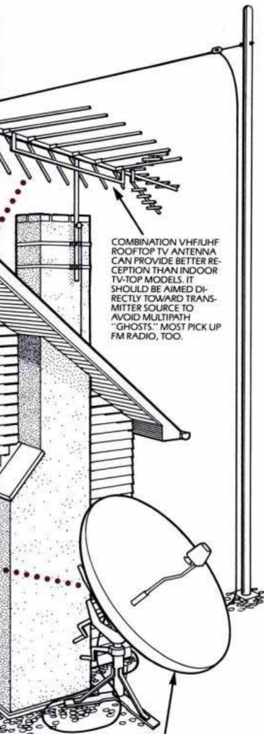
Most rooftop TV antennas combine VHF (long elements) and UHF (short elements).
