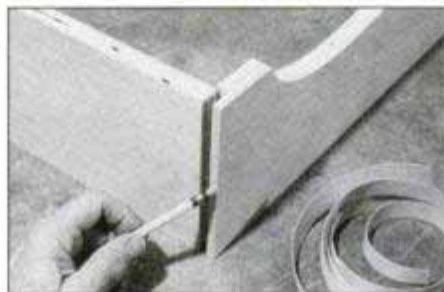
If you want to cover the edge of a plywood piece that must be rabbeted, be sure to apply veneer tape before rabbeting. Otherwise, overall length dimension will be off.
