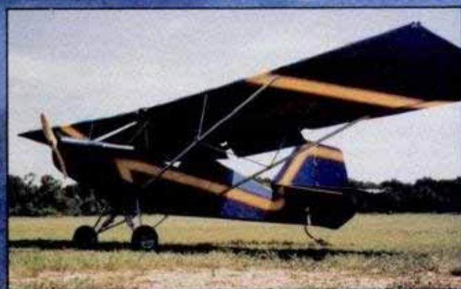
Speed-reducing flaps on this 40-hp Clipper are an indication of just how far ultralights have come. Kit offers choice of either tri-gear or taildragger [above] configuration, sells for $6,595.
