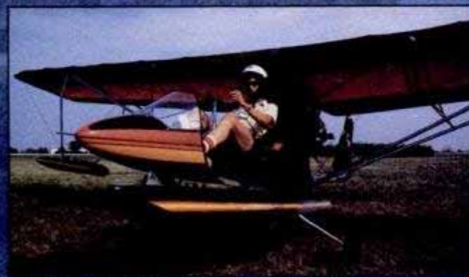
New centerline float provides amphibious operation with less drag and better control than twin floats. Shown on a Quicksilver GT. It fits most center-spar ultralights, costs about $2,200.
