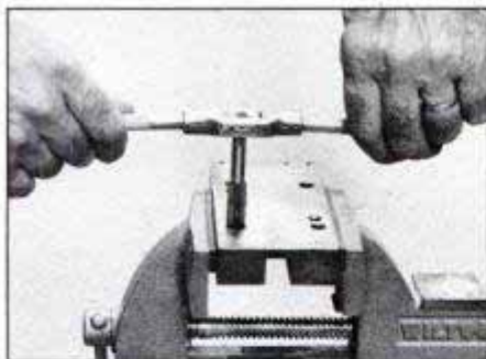
When the tap starts biting, use both hands and hold the handle at the ends. Back off a quarter-turn after each forward half-turn.
