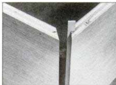
To conceal edges without adding anything to them, use a splined miter joint and glue. A good spline for 3/4-in.-thick stock is a 1/2-in.-wide piece of 1/8-in.-thick plywood.
