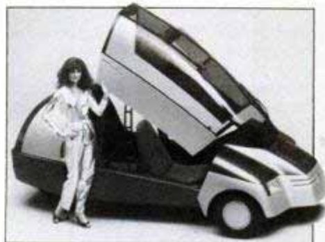
Ford's Cockpit show car features a motor scooter engine and tandem seats for two.
