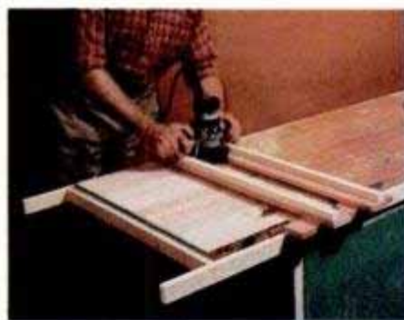
8. Router —Use a router with the jig shown to flatten deeply worn or gouged surfaces. The cut is made to a uniform depth from above using a \frac{1}{8} -in.-dia. straight cutter.
