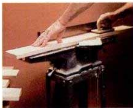
6. Jointer —A properly adjusted and sharpened jointer flattens and smooths narrow boards in one operation. You should remove only \frac{1}{16} in. of stock—or less—per pass.
