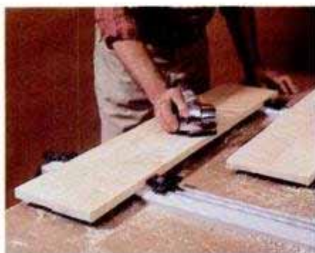
5. Power plane —This tool is used most often for planing door edges, but it works well for rough surfacing, too. Direct it diagonally across the stock to remove high spots.
