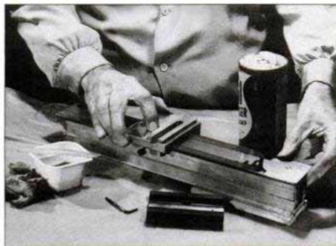
Lap lathe ways before assembly (above) with compound of scouring powder and oil. Stock parts at right are: head stock (A), cross slide (B), allen wrench (C), carriage stop (D), tool post (E),
