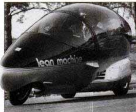
GM's experimental Lean Machine is a single-seater with a cab that leans into corners.
