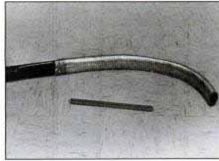
Vacuum accessory for cleaning soot from flue heat exchanger can be made from aluminum hose hammered to oval shape.
