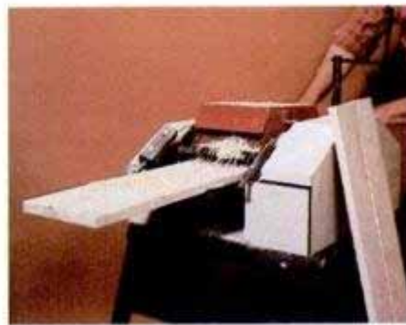
7. Planer —A planer quickly removes stock from wide boards and creates a uniform thickness. It's nearly indispensable if you want to work with rough-sawn hardwood.
