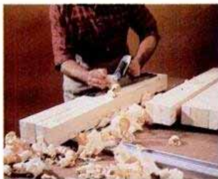
3. Jointer plane —If individual boards—or components of a larger assembly—are particularly warped, smooth with a long jointer plane before parts are glued together.
