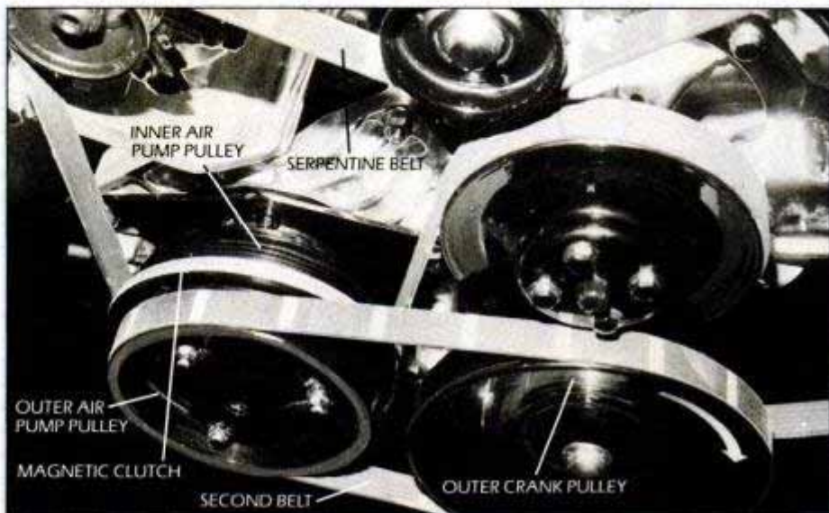
Mustang's two-speed belt drive turns all accessories (except the air pump) half speed.
