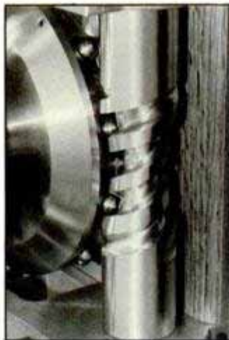
Squirm Drive's ball bearings replace the bronze teeth used in traditional worm drive rigs.
