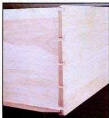
Drawer back and side (right) are joined by dovetails. Note side is tapered from top to bottom.
