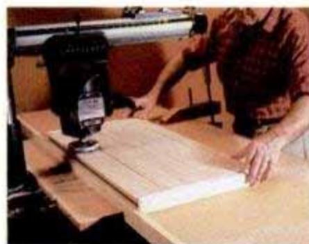
10. Radial-arm saw —A rotary planer attachment for a radial-arm saw has a cut depth capacity of \frac{1}{8} in. The cutter unit is fixed and stock passes underneath.
