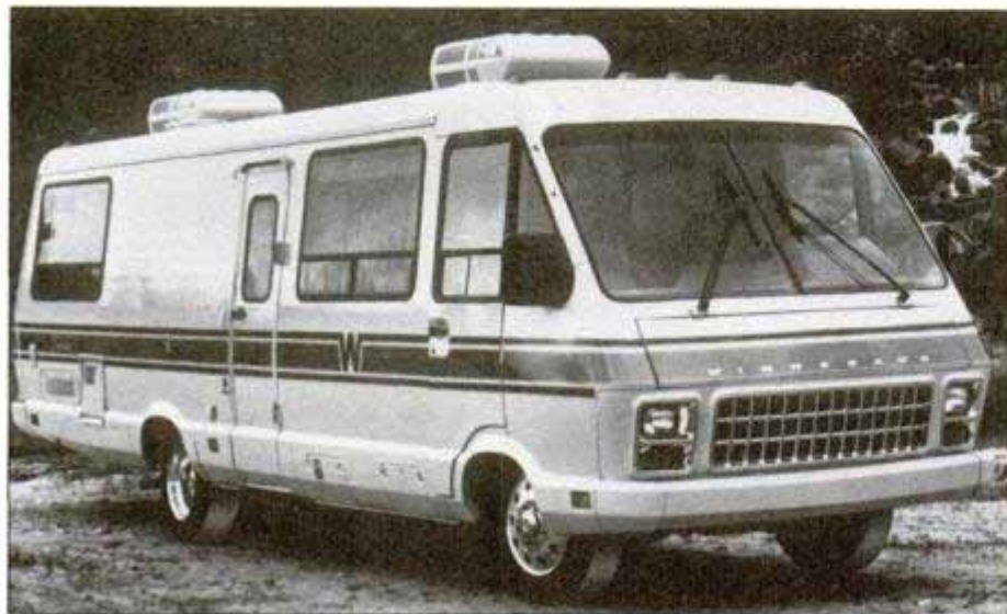
Rounded aerodynamic look is in, even in motor homes. Note the steeply raked windshield.
