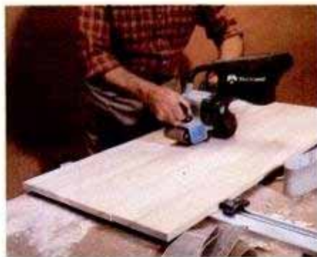
4. Belt sander —When the grain direction varies across a wide panel, use a belt sander for surfacing. It works by abrasion instead of cutting, so it won't chip the surface.
