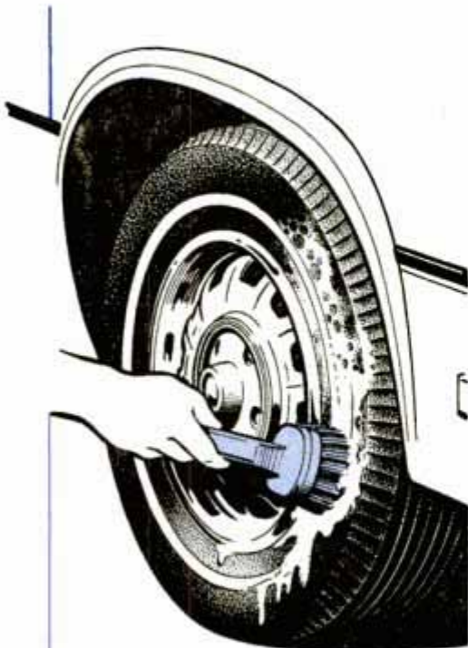
Special cleaners are available for tires and for cast aluminum wheels. Use a stiff brush to remove brake dust and grime.
