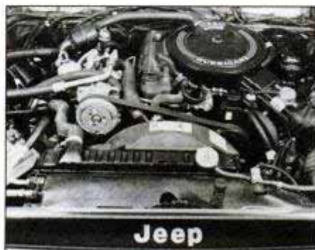
Most buyers chose AMC's first home-grown Four, a short stroke, 2.5-liter model.
