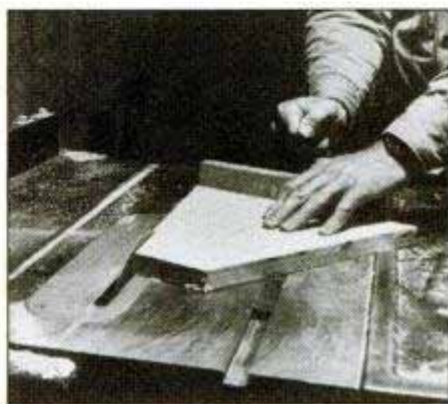
Trim the edges of each end piece with the blade angled 4^\circ and miter gauge set at 21^\circ . Orient the 4^\circ bevels so that the inside surface is wider than the outside face.
