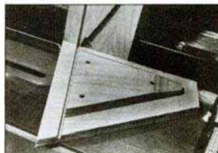
When cutting the \frac{1}{4} -in.-wide dados for the toolbox bottom, be certain that dados align in the corners of the box (arrow).
