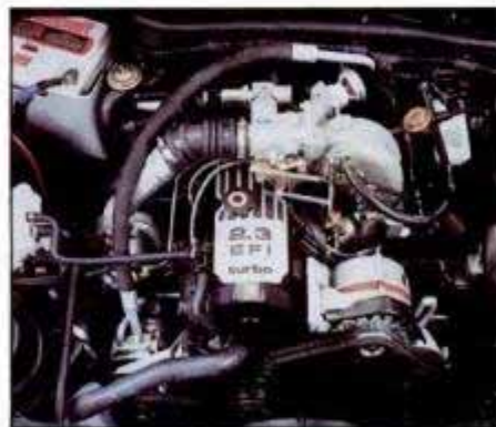
Merkur's turbo Four is set at 15-psi boost, and puts out 170 hp (160 hp with automatic).
