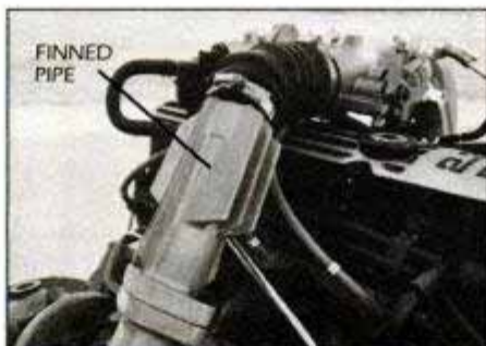
Merkur's turbo Four isn't intercooled, but part of the air delivery plumbing sports cooling fins. This might allow future racers to install intercoolers and still meet "factory trim" rules.
