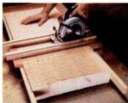
9. Circular saw —Make repeated kerf cuts with saw and sliding jig to remove stock from rough assemblies and to act as depth guide marks for hand planing later.
