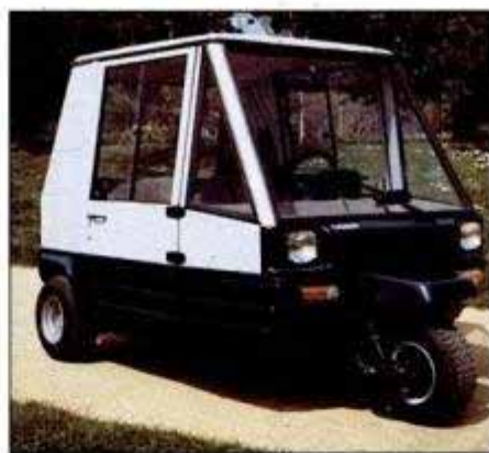
Ligler's 125-cc delivery van delivers up to 100 miles per gallon at a $3,500 price.
