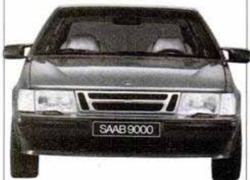
The 9000 head-on shows wide stance, familiar grille; drag coefficient is a low 0.34.
