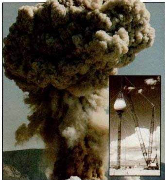
Defense Department tower (inset) uses 1 million tons of ammonium nitrate to set off a blast that simulates an atom bomb.
