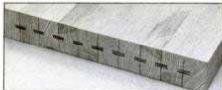
Splines are visible on end grain (above). Cut the spline grooves on a table saw (right). Feather-board applies side pressure.
