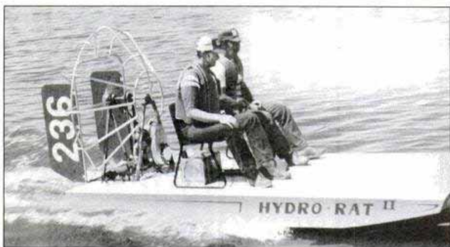
Hydro-Rat II airboat can carry two and is powered by a 20 hp, two-cycle engine.
