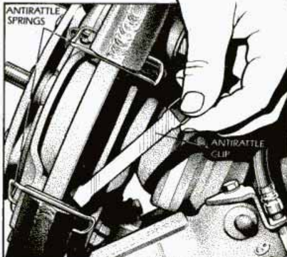
4 Clips that hold antirattle springs may require replacement. If so, they'll be supplied in the pad kit.
