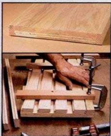
5. Glue-joint —Use a glue-joint bit to cut mating edges on all parts. Then glue the parts to a plywood base. Cross section (top) shows tight-fitting joints.
