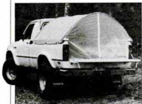
The total weight of the whole Mini-Dome assembly is just five pounds.
