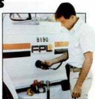
Pump attendant hooks up computer line. No fuel flows unless computer gives the okay.
