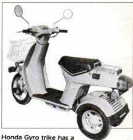
Honda Gyro trike has a frame jointed so front end leans in turns.
