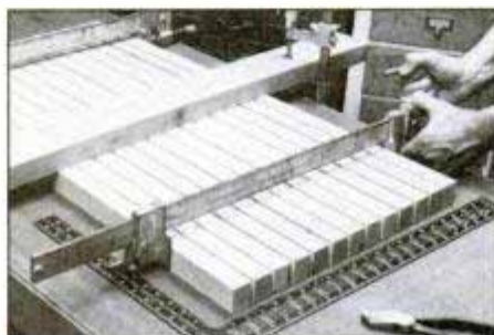
Use bar clamps to drive nail pins into adjacent pieces. Note board clamped across the top to keep butcher block flat.
