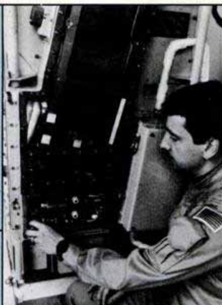
McDonnell Douglas/NASA Shuttle payload specialist Charles Walker starts electrophoresis unit (above). The machinery (top, left) makes pure protein. Under strict temperature control, the unit can make insulin. The diagram (left) shows an unrefined protein as it enters a carrier fluid. This will flow up and separate under an electric field.
