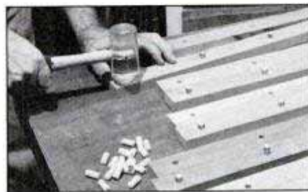
Apply glue to the walls of the holes and then tap in the pins using a wooden or plastic mallet to avoid damaging the ends.
