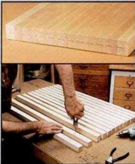
4. Nail pins —Cut pins from finishing nails using a pair of end-cut nippers. The pins strengthen the glued joint and prevent the wood from slipping when clamped.
