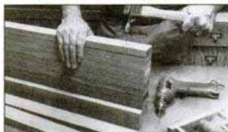
Direct-nailing technique is a quick and easy way to make a butcher block. Be certain to bore nail pilot holes first.
