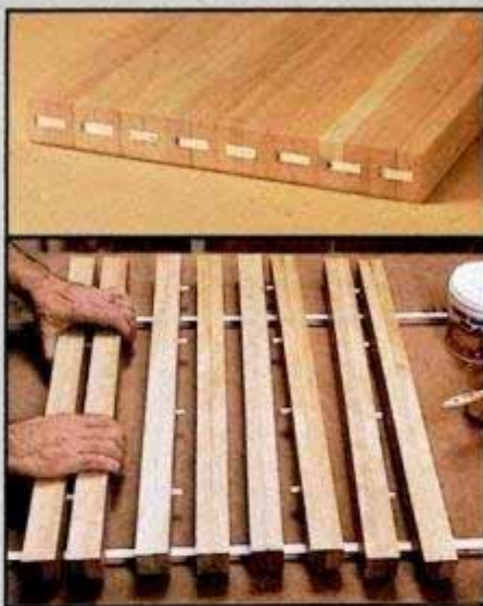
1. Dowel pins —Fluted dowel pins are used to join lengths of \frac{3}{4} × 2-in. cherry. Note that they're joined in pairs first. Cross section (top) reveals dowel locations.
