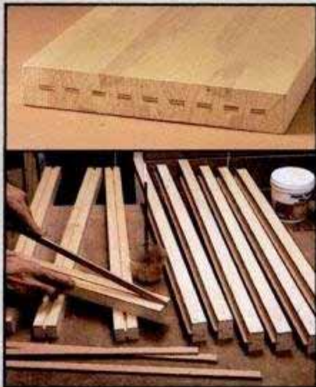
3. Spline-joint —Assemble spline joints using mahogany plywood splines. Groove each member on both sides, except the end pieces (top), to accept the splines.
