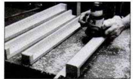
After nailing together the four L-shaped leg assemblies, round all outside corners with a router and a \frac{1}{2} -in. rounding-over bit.
