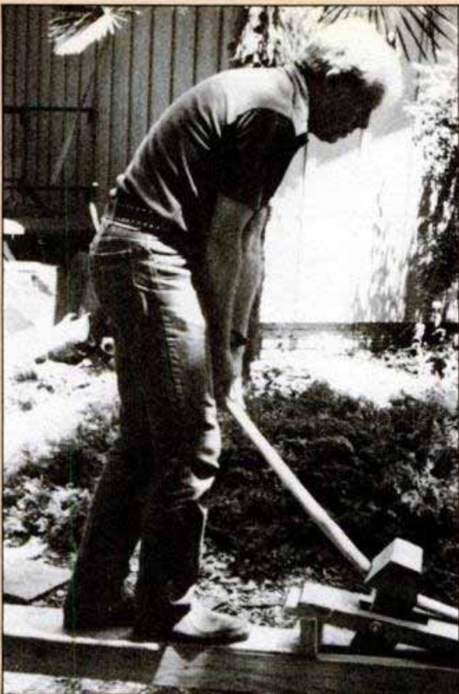
Carter bends a back leg for one of the chairs. The legs and slats are bent by hand after wood is steamed soft.
