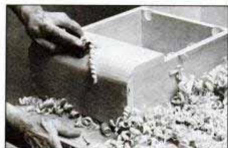
Round the top of the cabinet using first a bench plane and then a smaller block plane. Finish the shaping with a belt sander.
