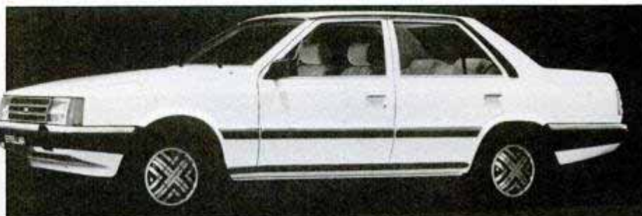
Hyundai's big car is the Stellar. It has a 102-in. wheelbase and a 100-hp, 1.6-liter Four.
