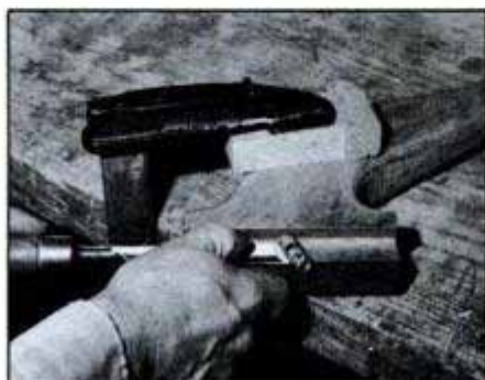
If the legs won't fit into the pedestal column, pare down the dovetail using a sharp chisel. Don't remove too much wood.
