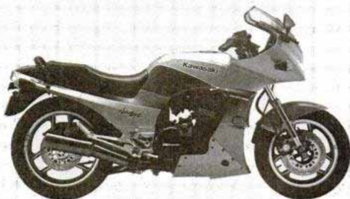
Kawasaki Ninja [translates to assassin] has new water-cooled Four, equals others' performance with just 900-cc displacement.
