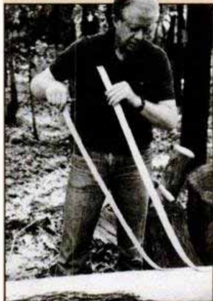
White bark strips off after scribing. It's saved for use in weaving the seats.
