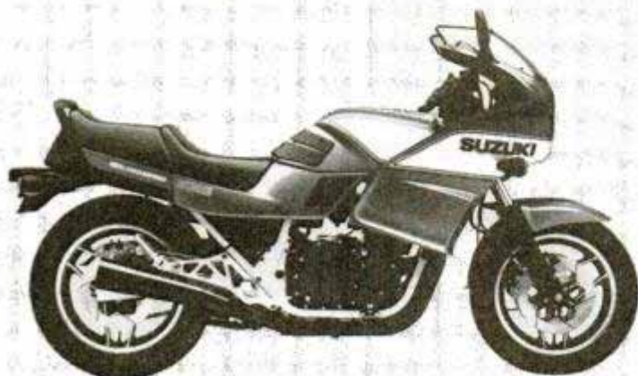
Suzuki GS1150ESE is the dean of the superbike school, with conventional transverse Four and multiaadjustable suspension.
