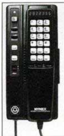
Portable phones for in-car use, like this Nynex Mobile Telephone, are mounted between front seats. The power output of mobile units can be as high as 25 watts.
