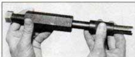
Slide hammer oil seal puller as ideal tool for recessed valve stems of ohc heads.
