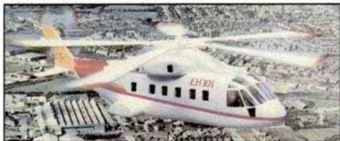
New European helicopter uses three engines to run its rotor.
