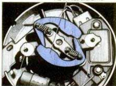
1. Check distributor advance weights for sticking caused by corrosion, lack of lubrication, or weak return springs.
