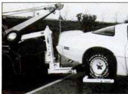
Wheel-lift supports car by its suspension, instead of axle, bumper, undercarriage.
