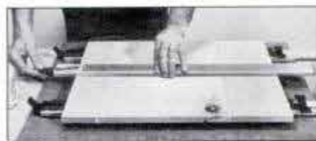
Once jaws are positioned, clamp is tightened with lever and cam mechanism. Design eliminates bowing in edge-gluing jobs.
