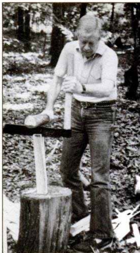
With a froe, the tree trunk is cut into sections. Sizes can be varied to any length desired.
