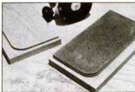
Rout the tambour door tracks using a template and a router fitted with a \frac{7}{16} -in.-dia. guide bushing and a straight bit.
