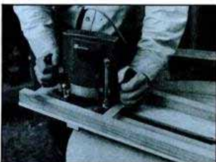
Trim the tabletop to its finished diameter using the router and jig combination. Note that a stop is nailed inside of the router.
