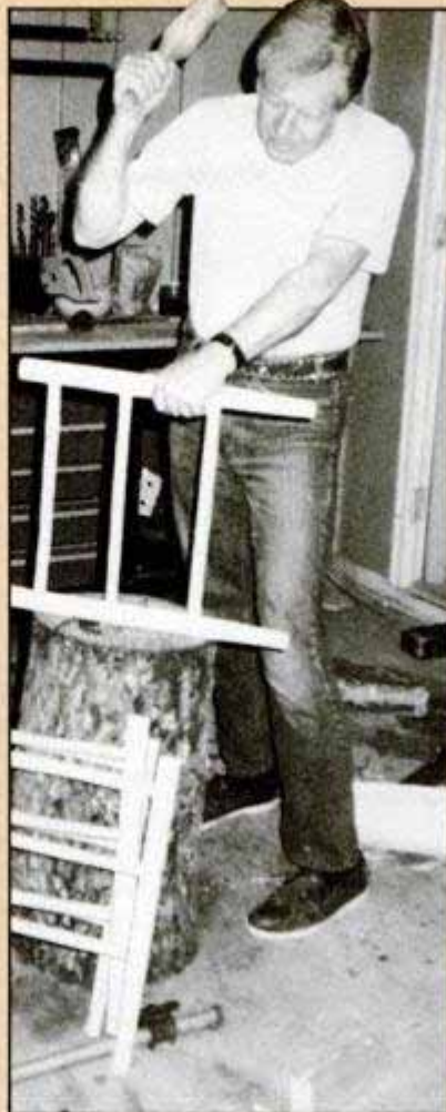
Rungs are hammered in after the ends are trimmed to give them a tight fit.
