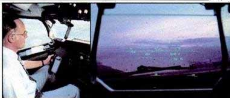
HUD (left) displays flight data on a transparent screen (right).
