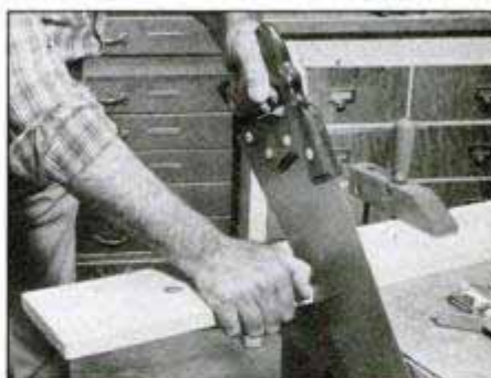
Use thumb knuckle as guide to start crosscut saw precisely on waste side of cut line. Draw blade back a few times to gain entry, then push blade forward at 45° angle.
