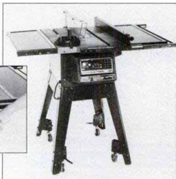
Electronic table saw has a touch-control panel (above) for programming blade height.
