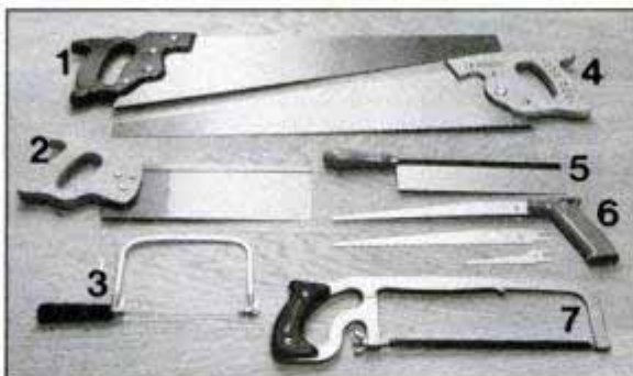
The most common handsaws for shopwork are (1) crosscut saw, (2) backsaw, (3) coping saw with removable blade, (4) rip saw, (5) dovetail saw, (6) compass saw with interchangeable blades, (7) hacksaw for metalwork.
