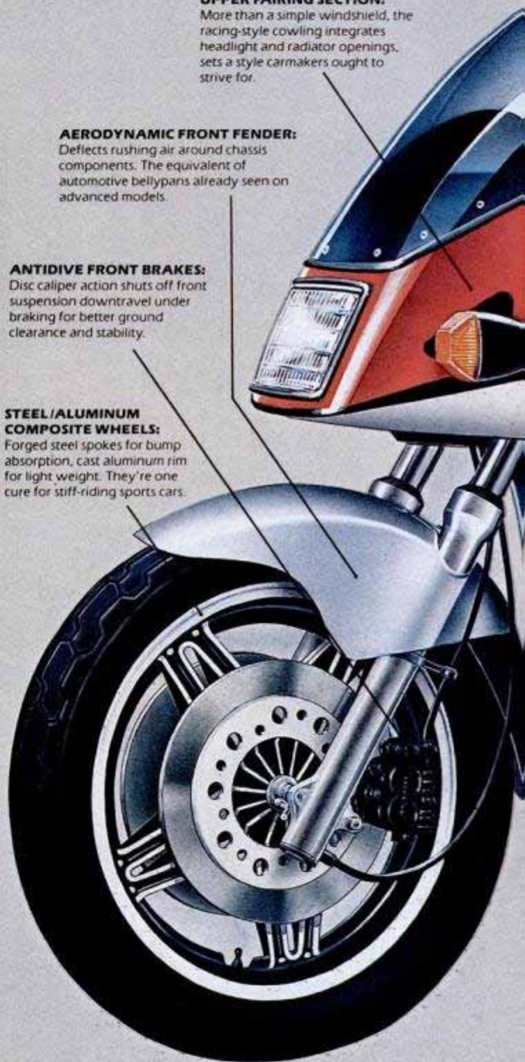
Superbike defined: High G-force cornering and 100+ horsepower.
