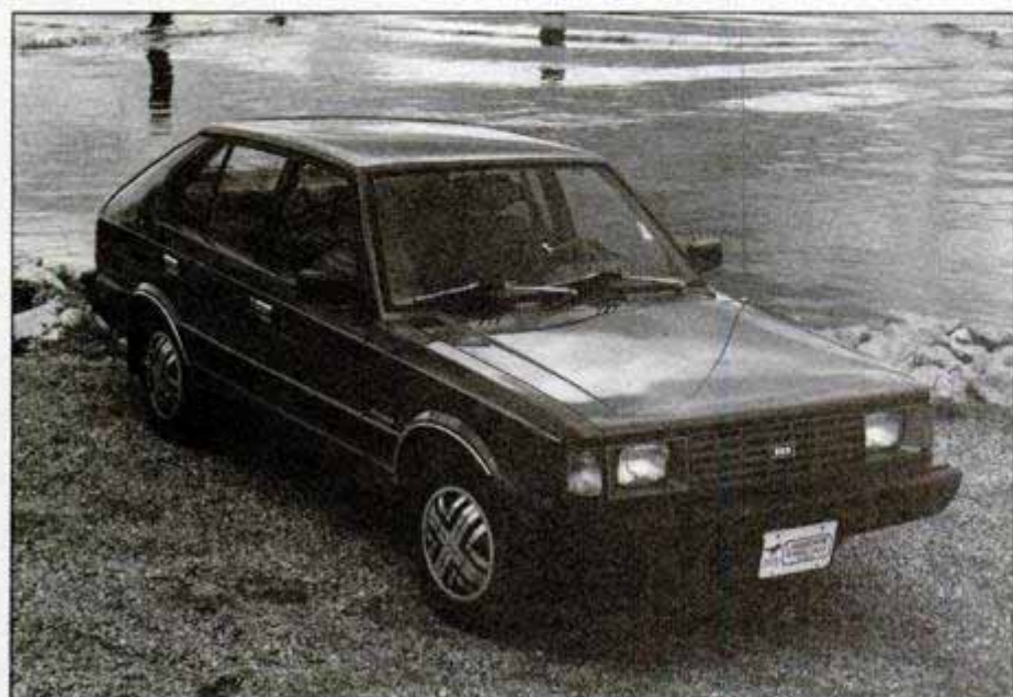
Hyundai Pony (left) is a basic front-engine/rear-drive four-door hatchback that sells for $4,530 in Canada. Top-of-the-line model costs only $5,233. Contemporary styling, inside and out, is by Ital Design. The 1.4-liter, overhead-cam, four-cylinder engine (right) is built under license from Mitsubishi.
