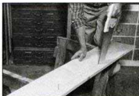
Start rip saw like crosscut saw, but use a 60° cutting angle. On long cuts, kerf may close and bind blade. To prevent this, insert nail or wedge to spread kerf open.
