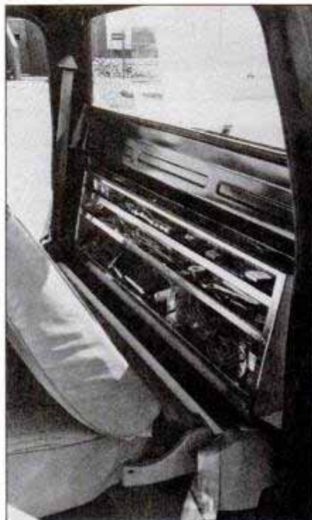
A four-shelf storage bin from Crafcro screws in behind the seat of your pickup to stow tools or hardware neatly. The shelves are carpeted to quiet rattles.
