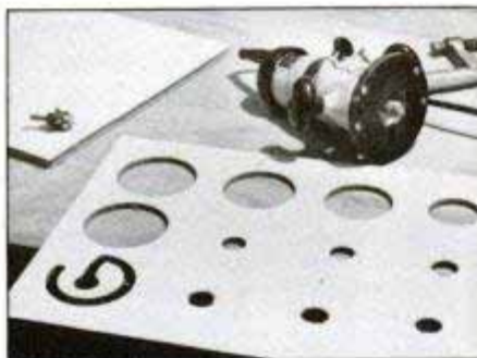
Apply plastic laminate to hole panel with contact cement. Then bore cutter entry holes through middle of each panel hole. Flush trimming bit in router removes waste.
