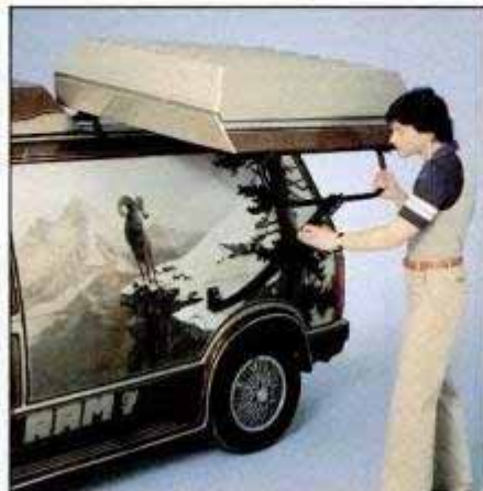
Clever linkage swings the bin down to waist level for loading or unloading of luggage.
