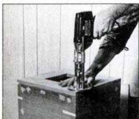
Glue and nail top trim boards in place, then fill nail holes with wood filler. Tape or clamp front panel to box and bore pin holes using a drill guide for accuracy.
