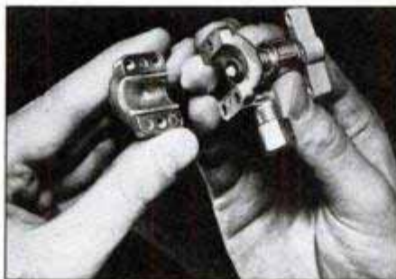
7 Select the proper tap valve insert— \frac{1}{8} -, \frac{1}{2} -, or \frac{3}{8} -in. O.D., depending on the size of the cold-water risers under your sink—and fit to riser. The inserts come with the company's separate faucet kit.
