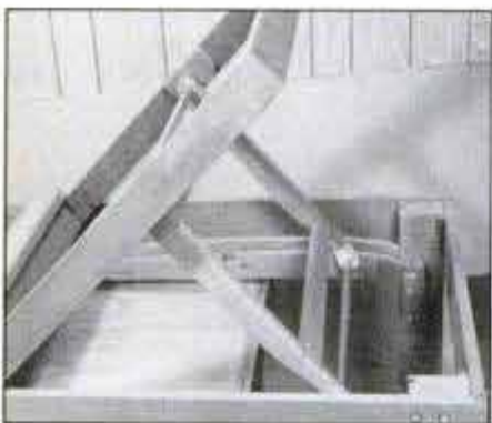
Support arm should move freely over notched guides and lock at 15°, 30°, 45° and 60° intervals. When flat, back rails should be 3/8 in. below top of side rails.
