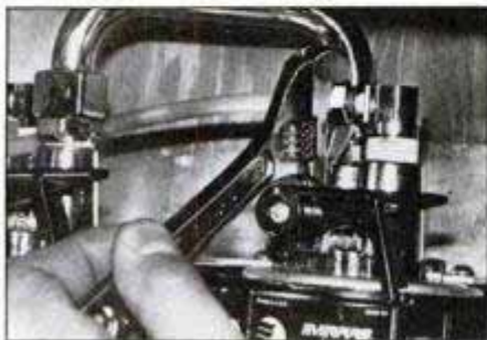
9 To connect compression fitting, remove nut and brass ferrule. Slip nut, then plastic ferrule over tubing. Place tube insert in tubing end; then insert tubing end into the fitting and tighten nut.
