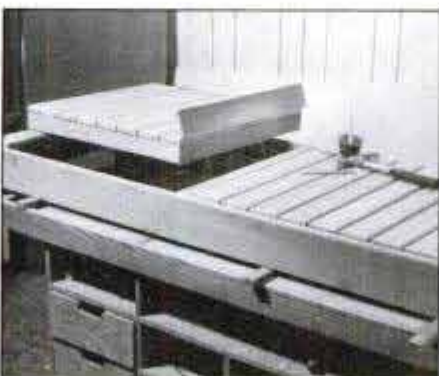
When all slats are attached to seat and back, complete the assembly by gluing and nailing the final seat slat—already attached to the back as shown—into place.
