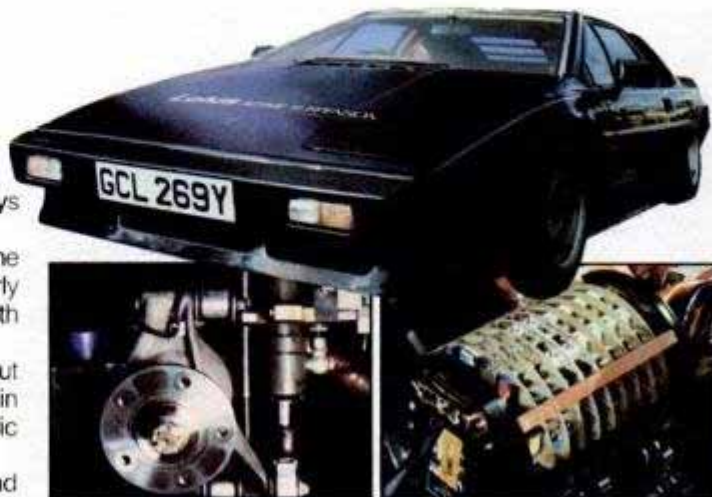
Lotus suspension jack (left) is regulated by a computer (right).
