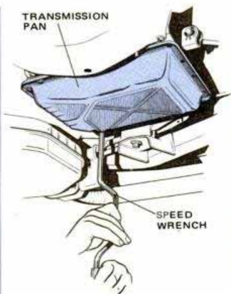
1. To drain transmission pan, loosen bolts that hold the pan to the transmission body and lower one corner of the pan.
