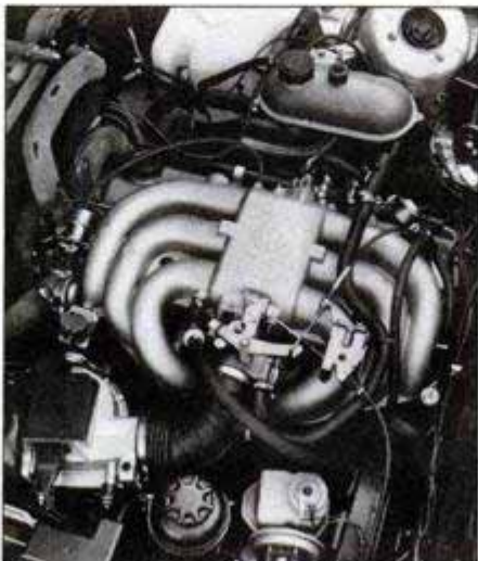
High-torque, low-rpm "eta" engine gives the 325e a 20-hp advantage over the 318i.
