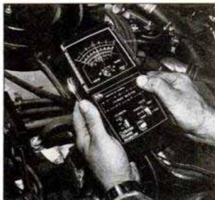
Cylinder Power Analyzer from Kal-Equip makes quick work of power balance checks. Just push a button to short out each cylinder and note the rpm dropoff.
