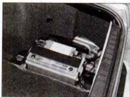
Battery is now mounted in trunk to help offset the extra weight of Six up front.
