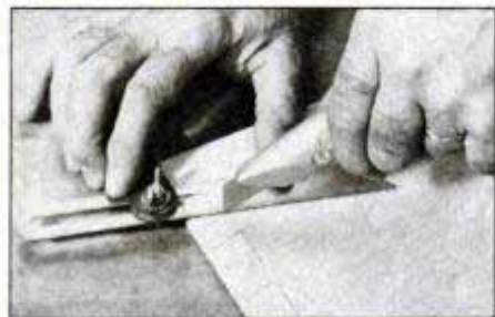
Marking dovetails with a utility knife gives you greater accuracy than a pencil. Score also aids in beginning cutting work.
