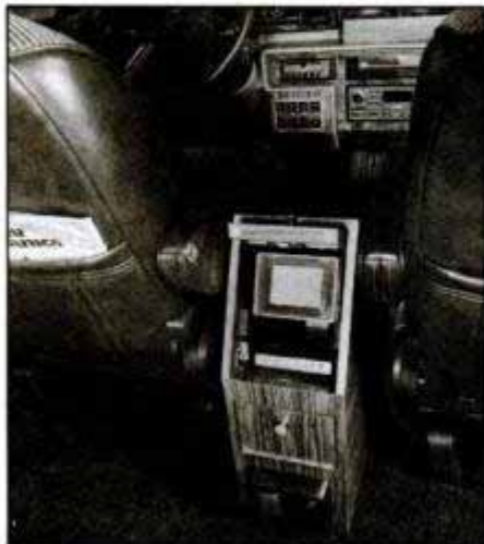
Tiny Sony color TV is mounted in custom center console. Locking door hides TV when not in use. Console ducts heat to rear seats.
