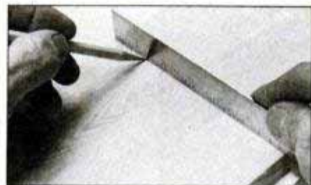
Hold a thick rule on edge to strike off a measurement for greatest accuracy. Distortion from viewing angle is minimized.
