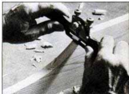
Use the convex-bottom spokeshave to trim a small radius concave curve. Always pull or push with the grain for all strokes.
