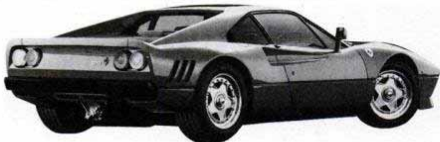
Ferrari 308GTO V8, for World Endurance Cup and IMSA racing, gets 600 hp from 2,855 cc.
