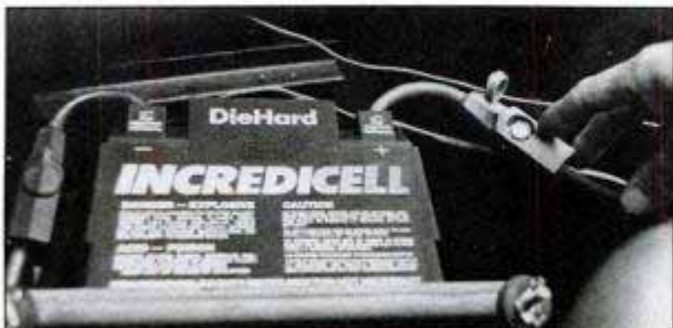
The Incredicell System, installed at a Sears Auto Center, includes connectors that are covered to resist corrosion.
