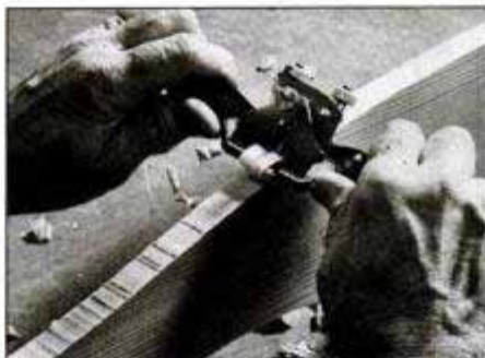
Trim saw ripples from a curved edge with a flat-bottom spokeshave. In this position, the spokeshave is pulled toward you.
