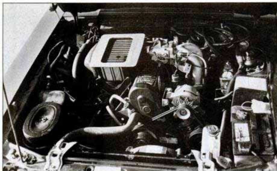
Engine bay is businesslike, if not pretty. Engine is set far back for better weight distribution. You must remove the intercooler in order to reach the sparkplugs!
