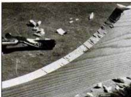
Stroking against grain produces rough, gouged area as shown here. It's time to change stroke direction when blade skips.
