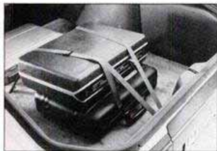
Luggage tiedowns keep cargo secure in the hatchback when the roads get twisty.
