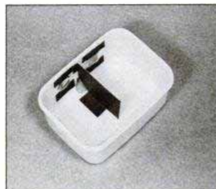
Tape the lenses to the eye openings and mount a black cardboard divider that reaches two-thirds of the way into box.
