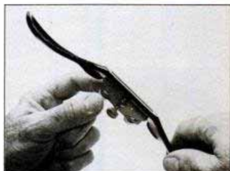
Turn spokeshave upside down and sight along bottom to adjust blade position. Then tighten the lever cap thumbscrew.
