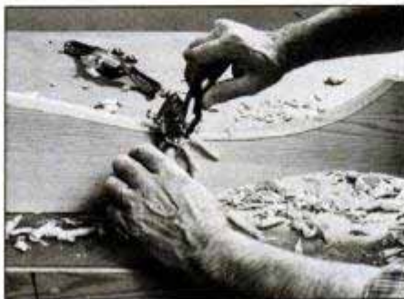
Use pencil guidelines to cut a chamfer. Position a lamp directly over this kind of work to make it easier to see results.
