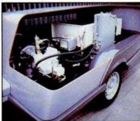
Production car (top) pulls rolling-resistance rig (above), which simulates terrain.
