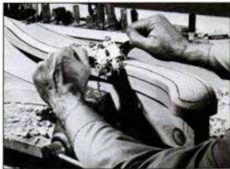
Contour an arm for a chair by first chamfering, then adding guidelines as shaping progresses. Use long strokes.
