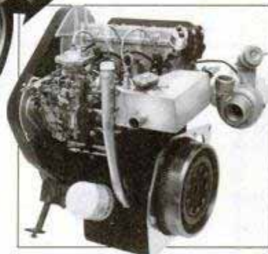
The three-cylinder diesel engine has a magnesium block that weighs only 26½ pounds. A second, counter-rotating flywheel helps absorb low-speed vibrations. The thermally insulated engine can run on different fuels.
