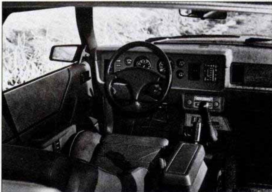
The controls are simple and clear, but a bit awkward to use. Heavily padded leather wheel has the horn button in its center, a position the new Fords are changing back to.
