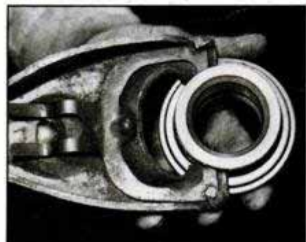
13 The throwout bearing installs with the fork springs under the collar and the smaller end toward the transmission.
