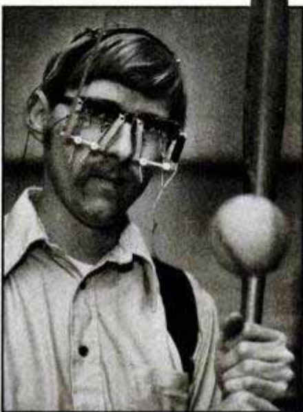
Engineer Terry Bahill demonstrates glasses that measure a batter's eye movements.
