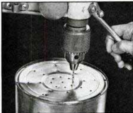
Drill holes in the bottom of a paint can for use in dispensing garden insecticide.
