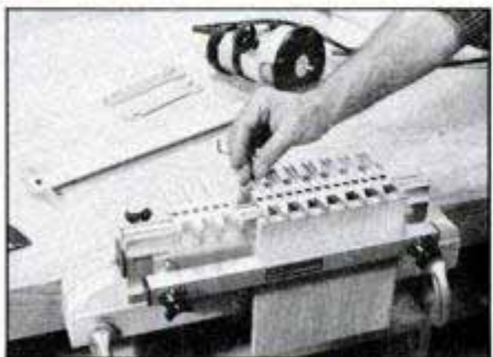
Remove top slide bar to position guide fingers; tighten using a hex-key wrench. Note 2x3 support bar clamped to workbench.
