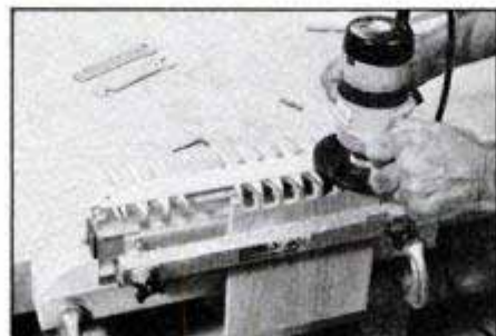
Use a router fitted with a guide bushing to cut the joint. Here, pins are cut using a straight cutter. Make the tails on opposite side using a dovetail cutter.
