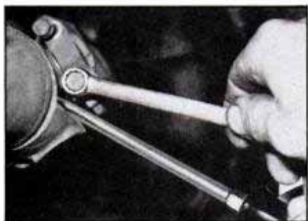
1 Use a screwdriver to hold the driveshaft still while unbolting the U-joint straps, then pry the shaft forward.
