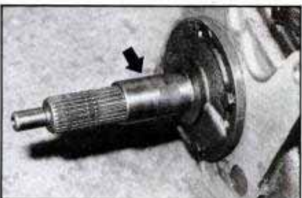
12 Throwout bearing rides on the transmission's front bearing retainer; it must be in good shape for smooth operation.
