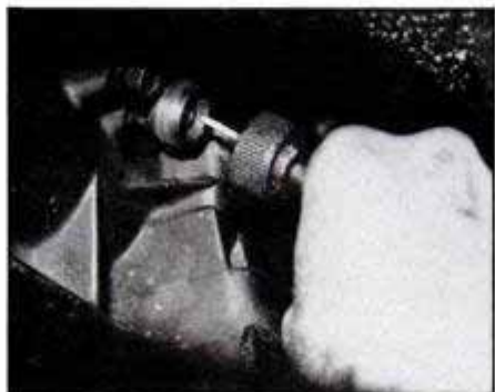
3 Speedometer cable unthreads from the transmission's tailhousing. Now, lower the engine for better access to shifter.
