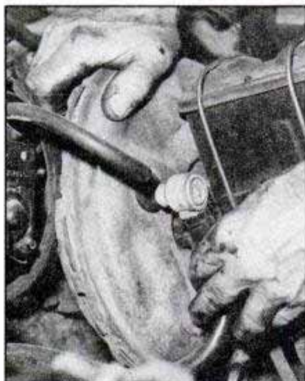
4 Vacuum line to the power brake booster—and all others coming from engine—must be tagged and disconnected.
