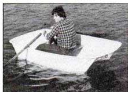
Cricket with cat bow has a 4-foot beam and 7-foot length. It carries 375 pounds.
