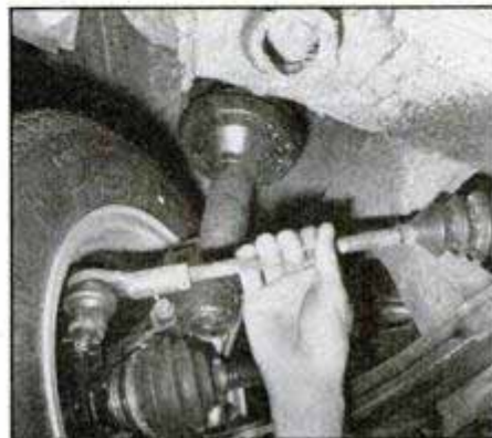
6 Steering linkage rods should be tight, with no free play in them.
