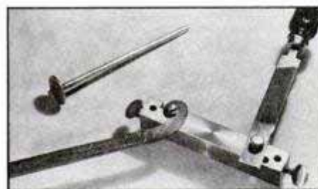
With cutter removed from vise, both blades are shown in place. It isn't necessary to remove a blade when using the other one.
