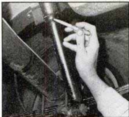
1 Shocks usually fail by spouting a leak and losing hydraulic fluid.
