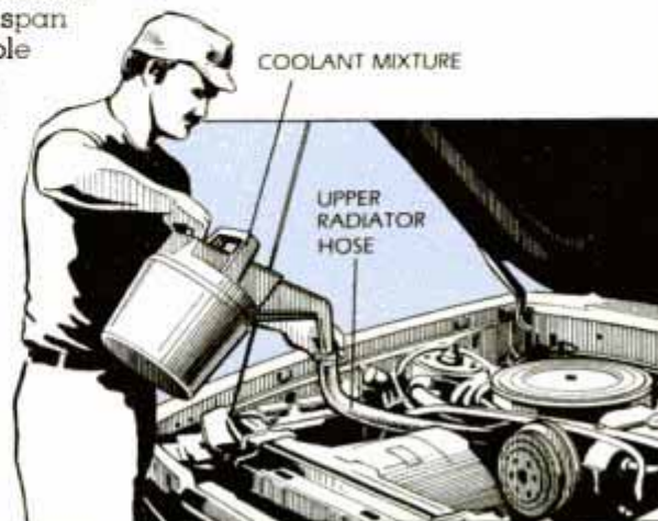
14 Cooling systems of 2.8-liter V6 Fords must be filled through upper radiator hose to prevent air locks.
