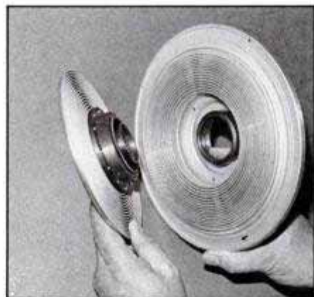
A silicon-filled clutch in the Cadillac transmission masks torque converter lockup.
