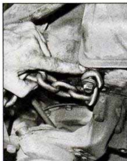
10 Hoisting chain should be attached diagonally across the engine to an existing hole in the block or head.
