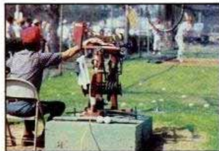
A coach feeds a baseball into a catapult-type pitching machine at Phillies spring training camp. The "Iron Mike" sees limited duty because it only throws fastballs.
