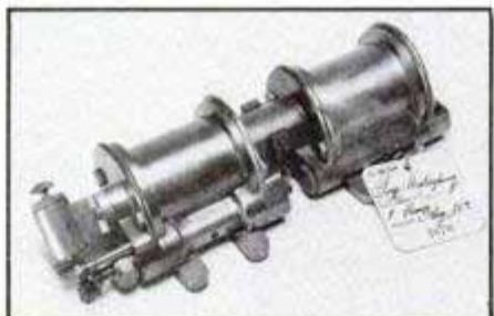
The Westinghouse pump, patented in 1870, looked ahead to efficient cylindrical valves.
