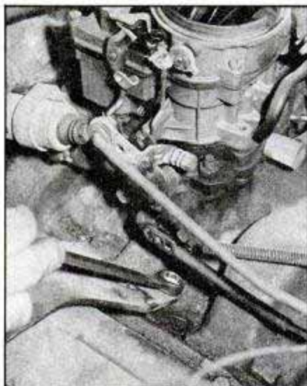
3 Position of the transmission kickdown linkage must be marked to ensure correct adjustment on reassembly.
