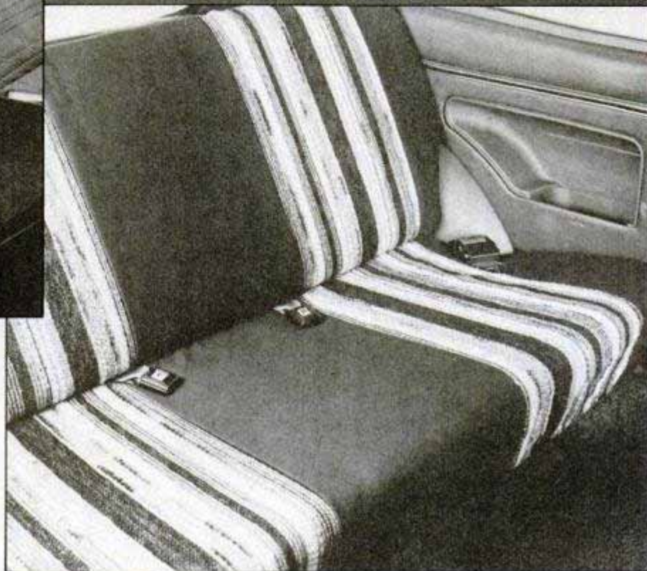
Upholstery in this Accord shows what can happen if kids use a car seat as a trampoline. You must remove rear seat cushion to install the cover.
