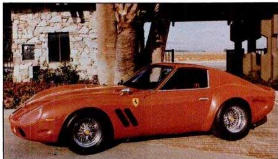
Only 39 Ferrari GTOs were ever built, and this is not one of them. It's Joe Alphabet's 72,000-mile 1974 Datsun 260Z, with Alpha 1 fiberglass panels bonded over the old body.
