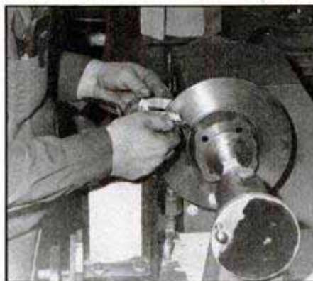
5 Auto machine shops can turn rotors or drums for a nominal charge.
