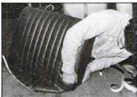
4 Upholstery panels are stitched together and secured to seat with hog rings. If original padding is sound, new upholstery can slip on over old.
