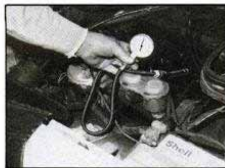
A compression test will tell you if the valves and piston rings are okay.
