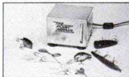
Fishhook sharpener uses a narrow fine-grit wheel to fit the gap on tiny bream hooks.
