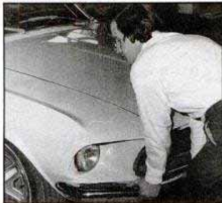
2 Rocking test is easy and may reveal bad shocks, depending on wear.
