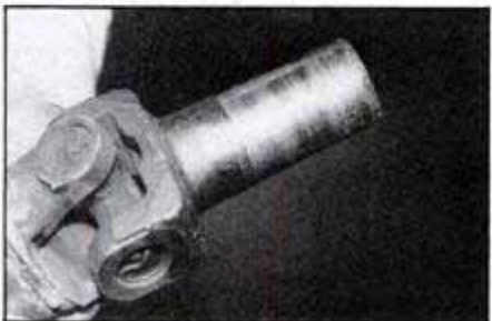
11 If the driveshaft yoke looks grooved or scored it must be replaced, along with the rear transmission seal.
