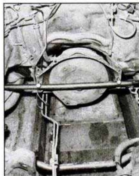
12 A bar laid between the frame rails will support the automatic transmission and allow the car to be rolled around.
