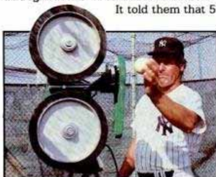
Former Yankee batting coach Charley Lau feeds a baseball into a twin-wheel pitcher. The machine throws all the major league pitches with extreme accuracy.
