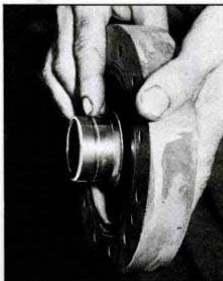
14 Severe wear on the hub of the harmonic balancer could allow oil to leak past the front cover seal.
