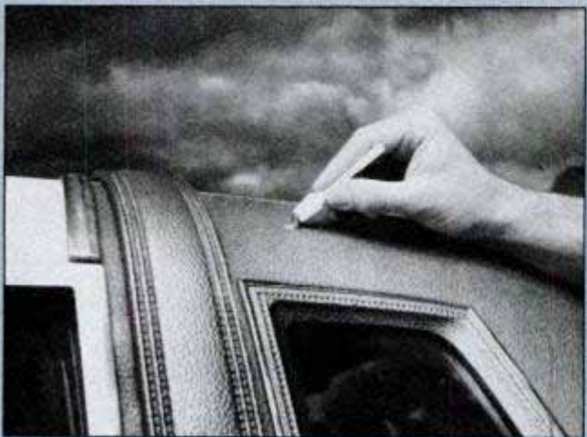
Loose vinyl tops and deep cracks in dashboards can be fixed with Duro's Perfect Match repair kit. The repair material ($10.25) is designed for tops and dashes, not seats.
