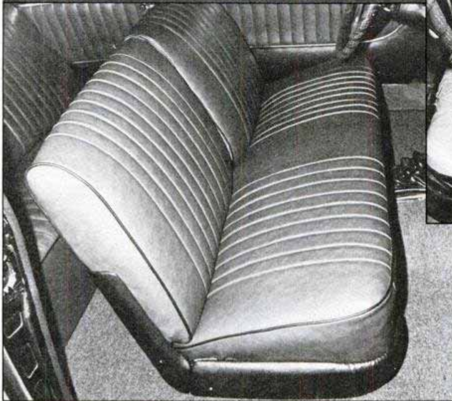
The front seat of this 1957 Chevrolet looked like a battle zone. Remove seat and peel off upholstery and padding down to the bare frame and springs.
