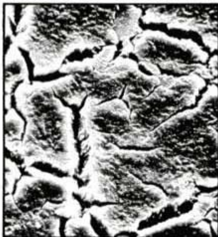
Electron microscope photos show a new metallic paint job (top) and same paint after accelerated weathering (bottom) equivalent to 2-3 years in Florida. Magnification is 2000x. Wax can slow damage.
