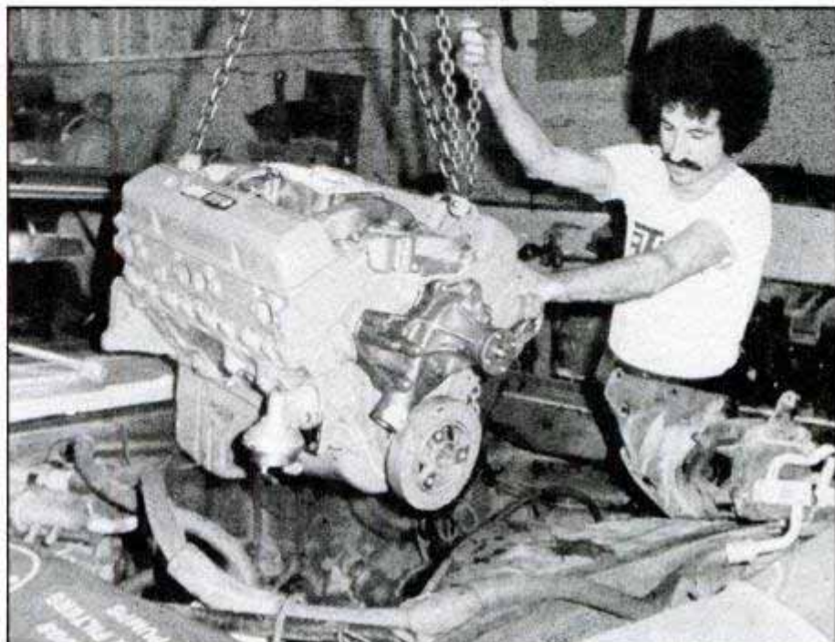
Older cars suffering from nothing worse than a lot of miles on the engine get a new lease on life when the worn unit is swapped for a new or rebuilt replacement.
