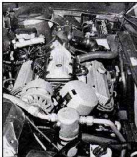
Engine compartment on 3.8-liter Buick V6 is so uncluttered you can easily remove the valve covers—a modern rarity.
