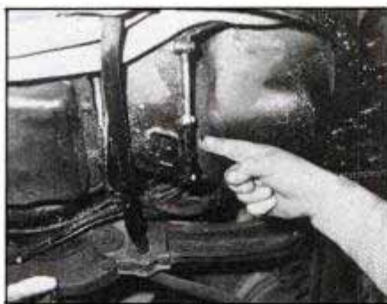
Oil leaks from the engine rear main seal are difficult and expensive to repair.
