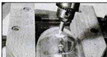
Start boring the hole at an angle. Then rotate the drill in a circular motion until the bit cuts through the glass.
