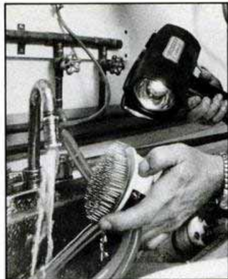
Using a timing light with a strobe range from one pulse per minute to 30,000 pulses per second, Tip can stop action on a tiny water-powered motor so that he can tell what angle will be the best for a scrubber that has to cover wide surfaces.
