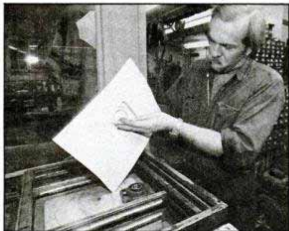
At his Thermoform plastic press, Tip can throw together a plastic model in a very short time. A boiler in the back of the press softens a sheet of plastic. Then a handmade pattern is pneumatically pushed against the softened plastic to create the final plastic model.
