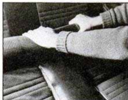
2 Rear seat cushions can be held down with bolts or a wire loop. Some release by pushing in at the lower front edge and pulling straight up.
