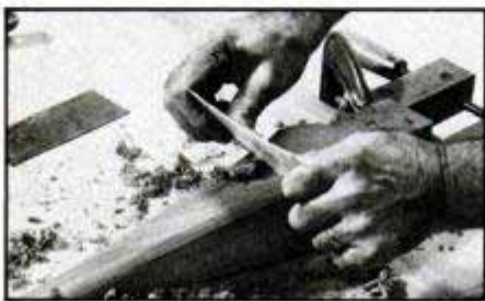
To use cabinet scraper, hold it firmly in both hands, bow blade slightly with thumbs. Tilt blade in cut direction and push.
