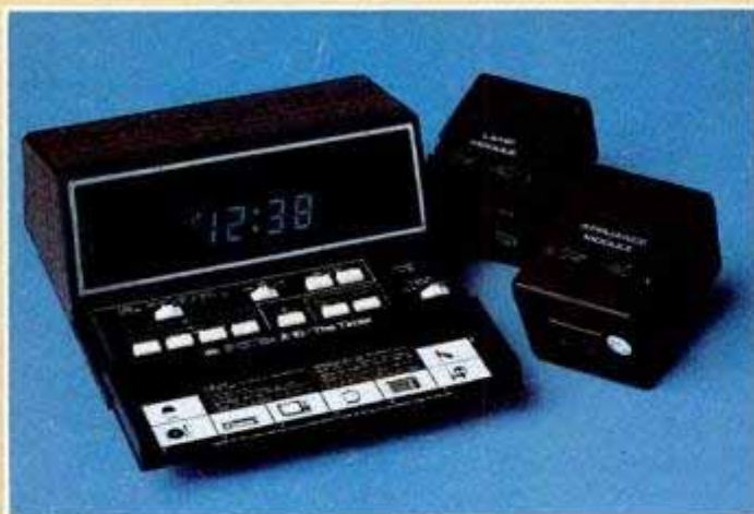
BSR's system X-10 features an optional timer/programming unit (left) for controlling home appliances. Modules (right) plug into the house wiring. The appliances plug into the modules.
