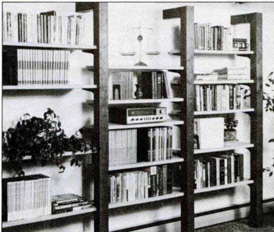
There's no need for you to fasten this bookshelf to the wall. Simply assemble the units and lean the 4x4 uprights against the wall. All of the shelf hardware faces toward the rear.
