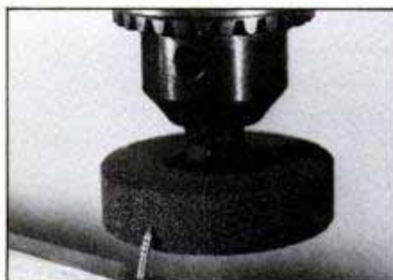
Grind the nails to a sharp point. A file can be used to sharpen the nails as well.
