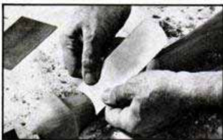
Use straight blade with concave and convex ends, or gooseneck scraper, to smooth curved surfaces like those on cabriole leg.
