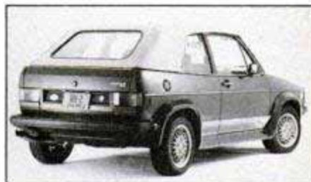
Fender flares and rocker panel skirts are part of Kamei's fuel-saving X1 package.
