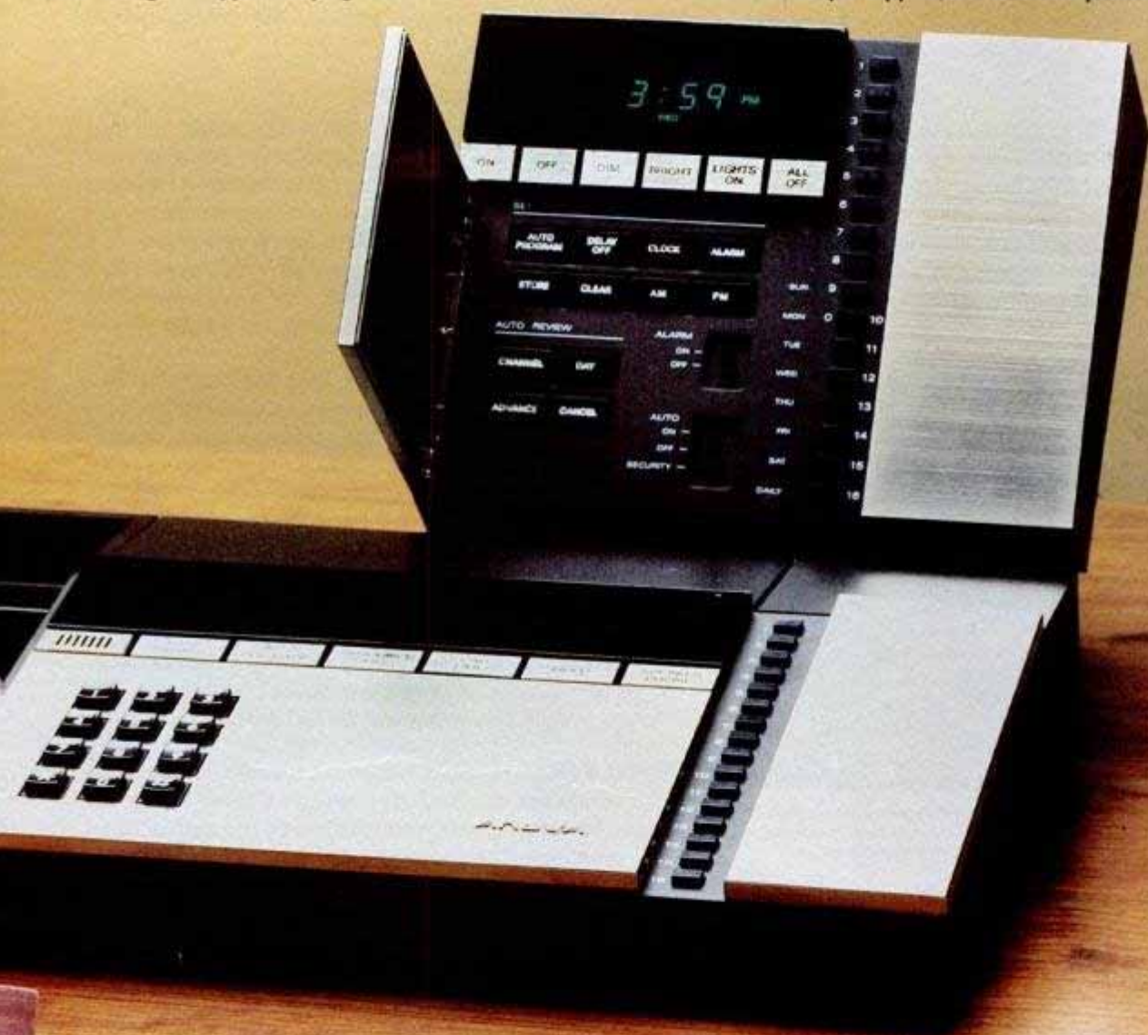
HomeBrain (above) must be programmed by the dealer's computer, but then it operates on its own to control the house. The system 1200 from CSI (on top) needs a dedicated personal computer.
