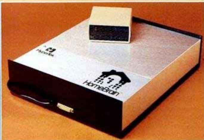
HomeBrain (above) must be programmed by the dealer's computer, but then it operates on its own to control the house. The system 1200 from CSI (on top) needs a dedicated personal computer.
