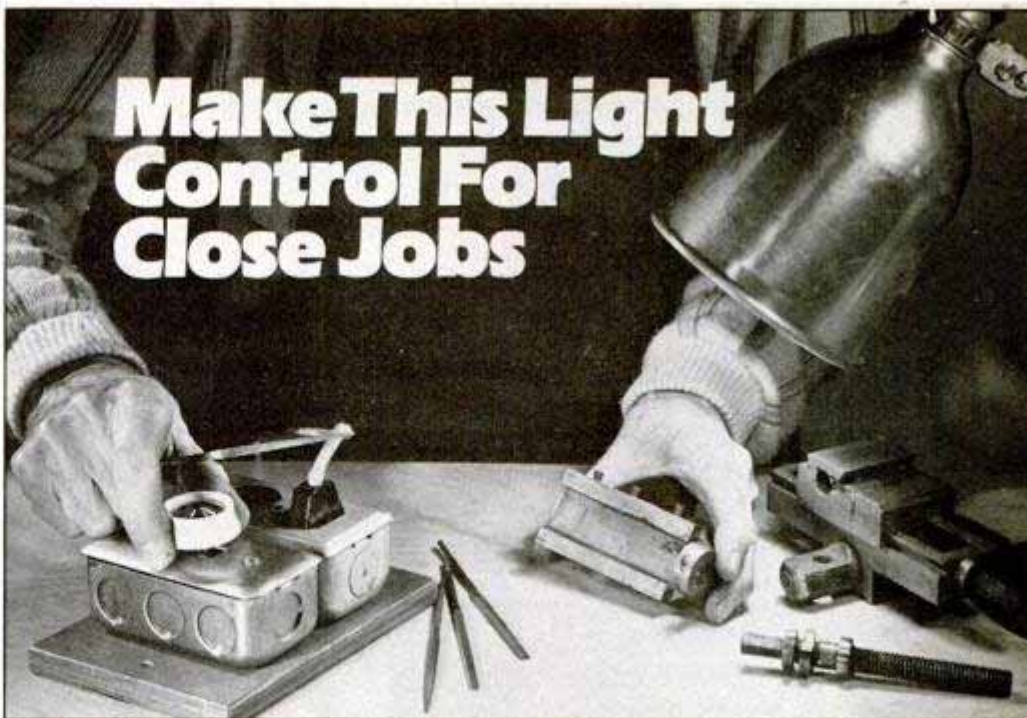
The light control shown is tested for use with a No. 1 photoflood lamp on a workbench.
