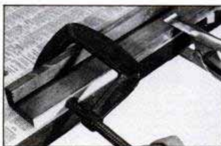
Tighten the C-clamps gradually to draw the two pieces together. Place newspaper down to absorb messy glue squeeze-out.
