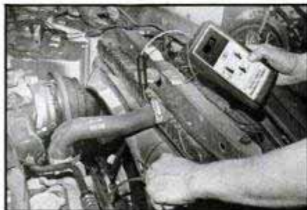
Magnetic timing tester can be used with ease on Ford, GM, AMC and Chrysler motors.
