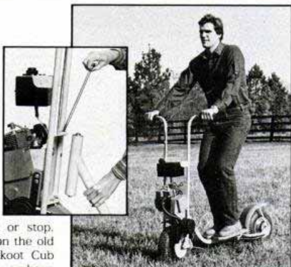
Skoot Cub rides trails that are too tight for a bigger bike. It can be tucked in a car trunk by just pulling the pin (inset) to separate the front power section from the rear.
