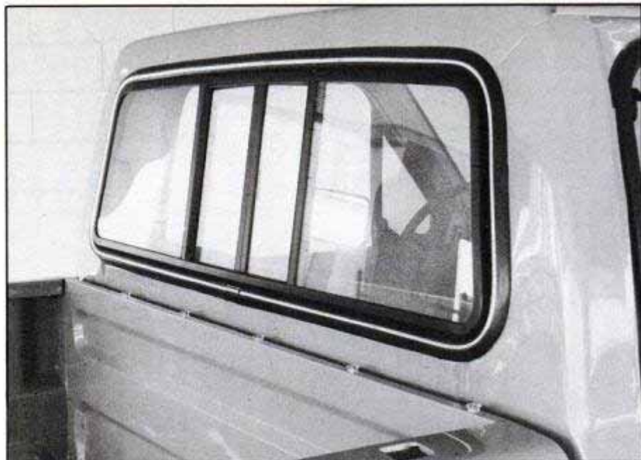
Pass-through window has sliding panes that allow access between pickup bed and cab.
