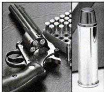
New .32 Magnum round stands 1.35 in. tall, almost ¼ in. longer than the .32 S&W Long.
