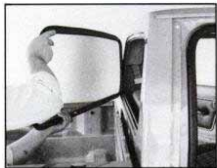
Pass-through window has sliding panes that allow access between pickup bed and cab.
