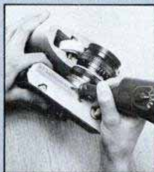
Go over the identification markings with an engraving tool, such as the Dremel electric engraver shown.
