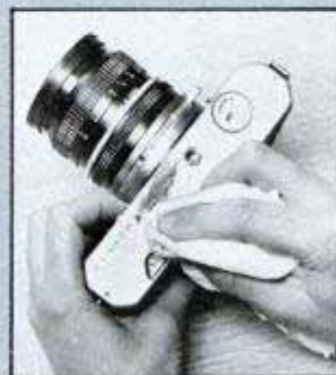
Rub the engraving with a colored lacquer stick to fill the indentations with color. Take time to wipe off the excess.
