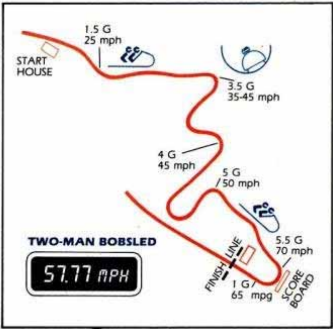
Sempliner's bobsled (top) has a rounded belly and attenuated body so it can take advantage of the G-forces. The chart above details the speeds and gravitational forces on the bobsled run at '84 Winter Games. Readout shows average course speed.
