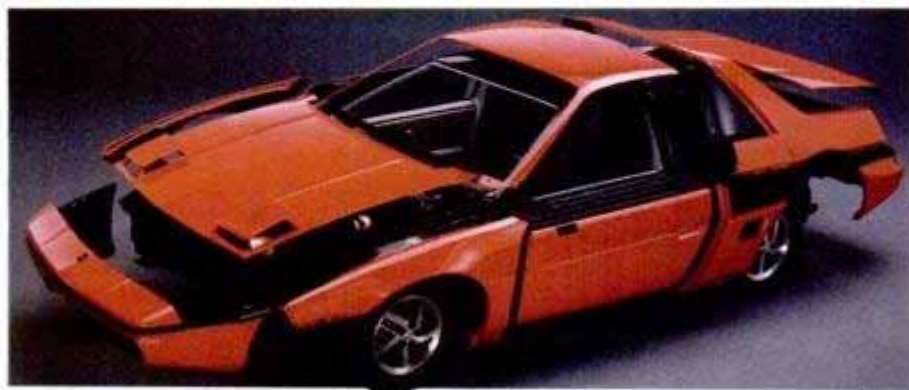
Underneath the Fiero's plastic body shell is a drivable skeleton called a "space frame." The body panels are attached to this frame with 39 bolts and other screw-type fasteners. Replacing all the body panels would take a beginner about five hours. Firms that now sell add-on spoilers could make completely new fenders, decks, nose sections and tail sections for the Fiero. And Pontiac is wholeheartedly encouraging such customizing.
