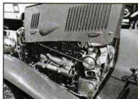
MG hot rod is powered by a "flathead" Ford V8 with double overhead cam Ardun heads—designed by Zora Arkus Duntov.
