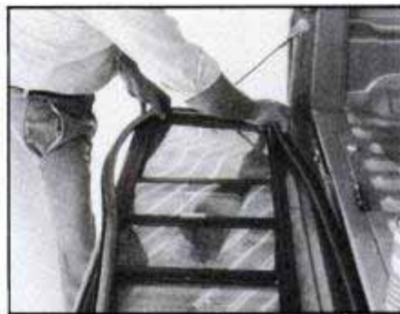
Pass-through window has sliding panes that allow access between pickup bed and cab.
