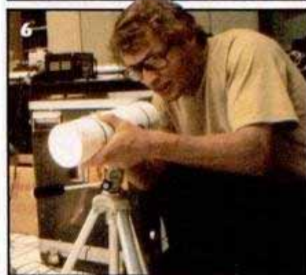
Equipment also includes advanced weight-training devices (5) and high-speed cameras and other visual detecting equipment. Light-beam guns (6) are used to determine timing improvements to split seconds.
