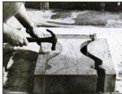
Remove endpieces from base form, then lightly tap curved pieces with a hammer for a clean separation. Pull curved form straight back away from base.
