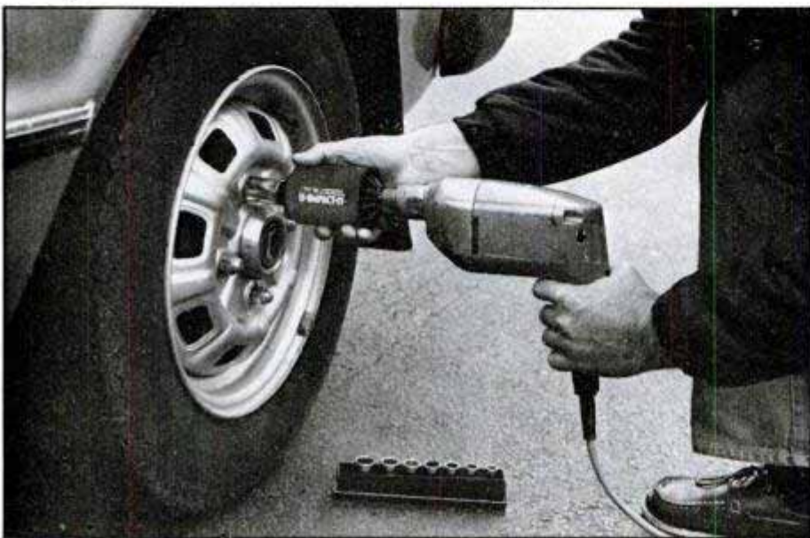
New mini impact wrench operates with ordinary 1/2-in. sockets and reversible drill.
