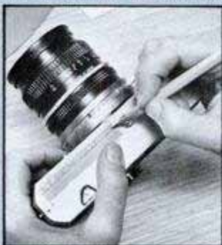
Position Scotch transparent tape on area of proposed engraving. Draw guidelines; pencil in the engraving.
