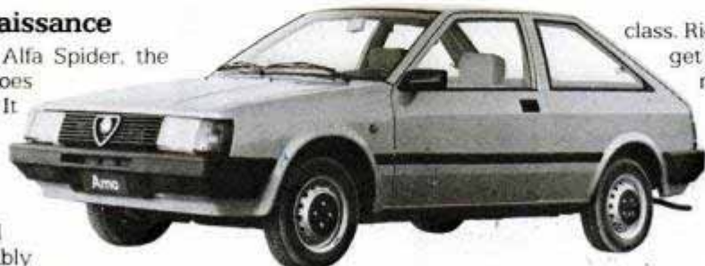
Arna (for Alfa Romeo Nissan Automobiles) has Alfa engine and Nissan sheet metal.
