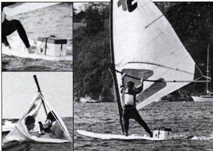
Sailboarders can take it with them on the Ten Cate Cruiser. Board has removable watertight box. Sail design allows the craft to be used as a tent for camping out.
