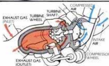
Honda's prototype of the turbo-supercharger uses a system that pipes exhaust gas over a turbine shaft that runs a compressor for increased power. Recycled exhaust gas makes engine more efficient.
