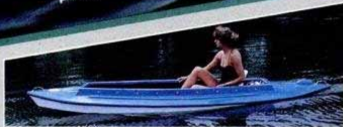
Built-in Shakespeare trolling motor gives Electric Feather almost 14-knot top speed. At only 78 pounds, this 12-foot pirogue runs silently on 12-v. marine battery you recharge at home.
