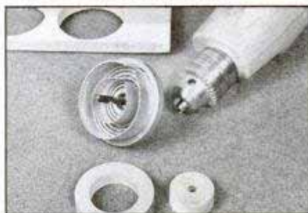
Cut rings by using two saw blades at once.
