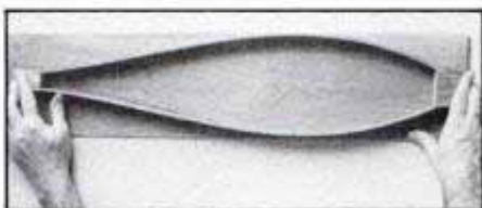
End-piece jigs force the teardrop dulcimer into its standard shape. You can make small adjustments by hand to help the symmetry when you glue the sides to the bottom.
