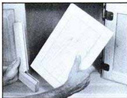
Cabinet door scrap shows assembly of raised panel, rail and stile (see drawing).
