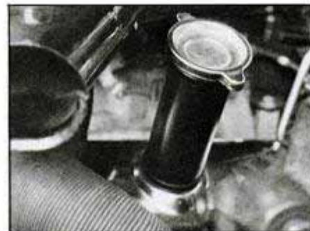
Extendo-Tube lifts oil filler hole up to where you can reach it on many engines.
