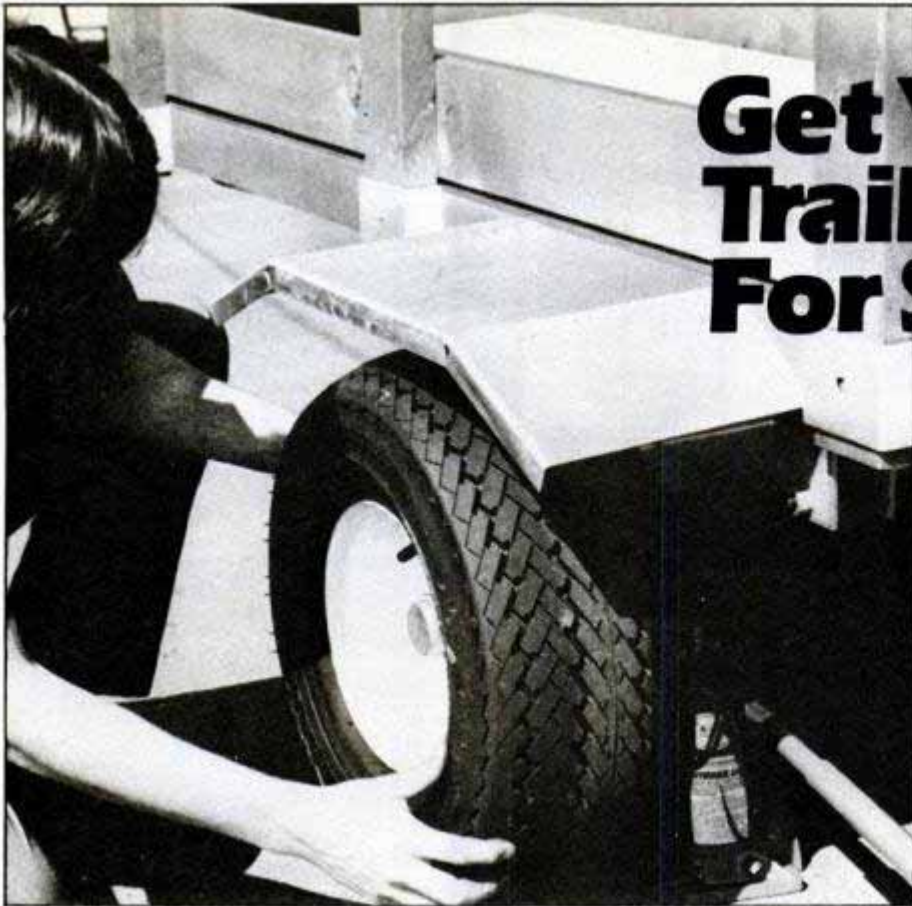
Rock wheel from top and bottom to check for play in bearing with trailer jacked up.
