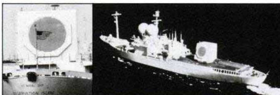
Cobra Judy is the code name given to a special secret vessel equipped with phased-array radar (above, right). The radar (above, left) sends out pencil-thin signals that pick up targets at various angles for complex pictures. Cobra Dane, a 10-story, phased-array radar (right), stands on an island off the Alaskan coast. The unit is made up of individual sensing plates. Each plate is a self-contained radar station. Supercomputers analyze the data received by Cobra Dane.
