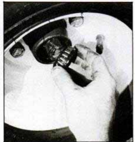
Rollers in their cage pop out in your hand after removing hub cap, cotter pin and nut.
