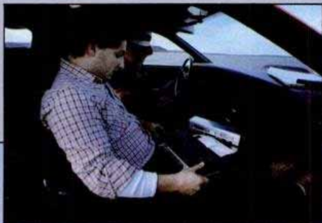
PM crew checks the readout on computerized road-test equipment, which is fed by a "fifth wheel" clamped to car.
