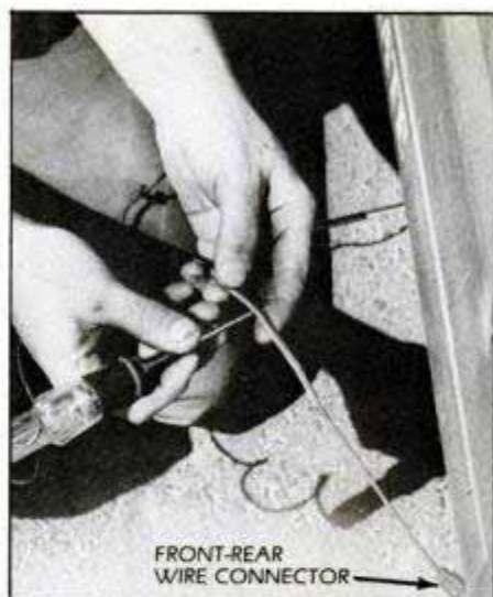
Professional electric circuit tester has a sharp probe to piece insulation on wires.
