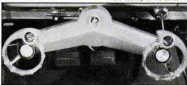
Mercury's experimental Wrist-Twist Steering employed two palm-sized wheels with thumb grips. The press loved it.
