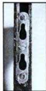
Flair Fold wood shelf and brackets (left) attach directly to the wall. A metal fitting, set into the back of each bracket (right), can slide easily over the two wall-mounted screws.
