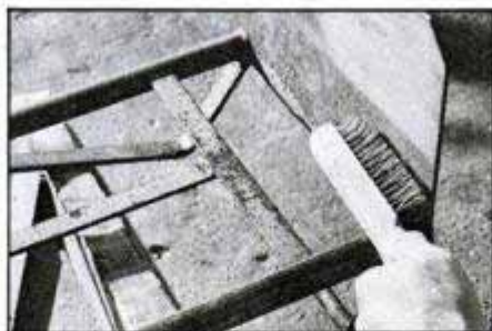
On extremely rusty projects, like the hand truck above, complete rust removal is too difficult. Instead, brush off the loose rust with a wire brush, then apply rusty-metal primer. Its fish-oil base penetrates through rust and drives out all of the air and moisture.
