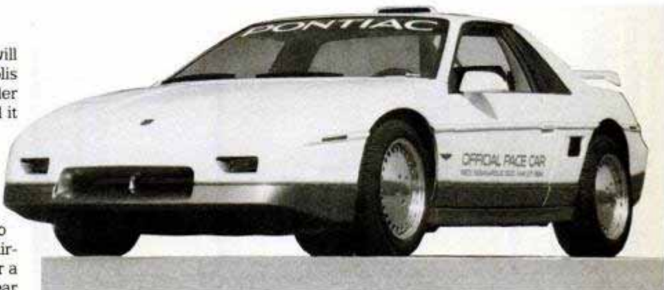
Pace car's low, aerodynamic nose was a simple swap due to bolt-on Fiero bodywork.
