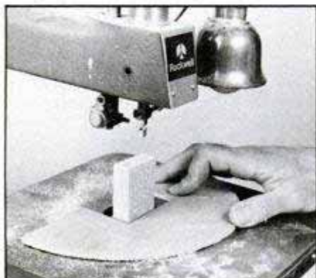
Mount the sanding block in saw's lower chuck. Remove blade guide for easy access.
