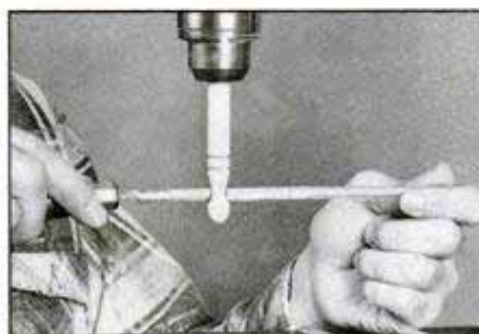
Place dowel in drill and contour with file.
