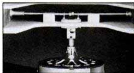
Hanger bracket, once it's expanded, bites into joists to hold ceiling fan securely.
