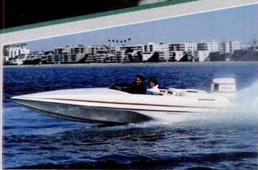
Sponson-hulled Starcraft CPS 200 features a small, flat pad just ahead of the stern to reduce wetted area and drag while planing at top speed. Designed for all-out performance by Art Carlson, the sponsons stabilize the hull at any speed.
