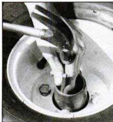
To remove outer race or cup to replace bearing assembly, drive it out with a brass drift.
