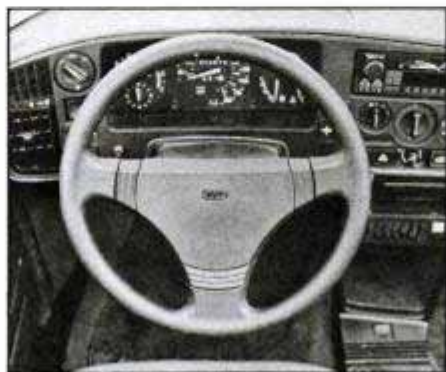
Great design of Saab Turbo steering wheel is nullified by location of horn buttons.
