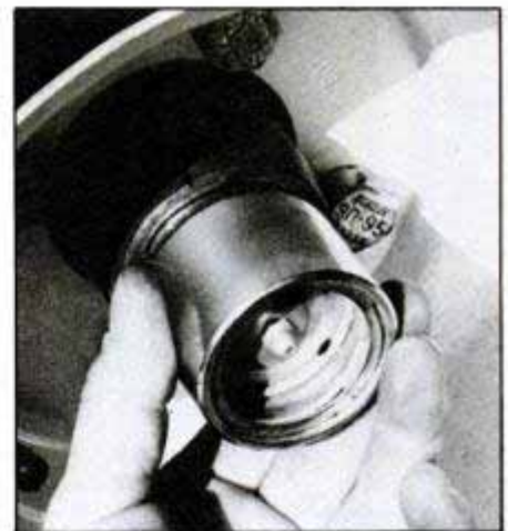
Special hub cap with grease fitting, called Bearing Buddy, speeds lubrication service.
