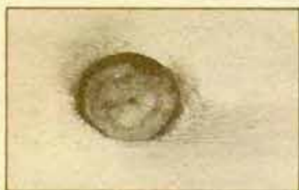
Encased knot is not firmly fixed. It's formed by an embedded branch stub.
