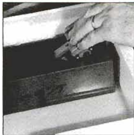
Honing guide promotes uniform sharpening whether you use a water or oil stone. With both hands, push full strokes across the stone face. Be sure to vary grinding path slightly as you go so stone wears evenly.
