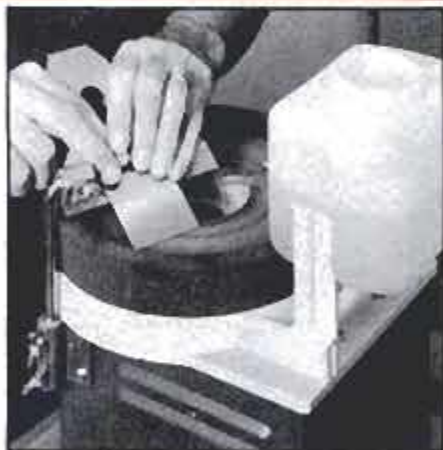
Water grinders like the Rakuda model shown can easily accommodate entire width of standard plane irons. Slow motor rpm and constant water lubrication reduce heat buildup, protecting temper of blade.
