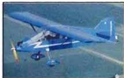
A real airplane for only $4,000? That's the projected construction cost for 28-hp, 110-mph Zippy Sport. Plans are $100.
