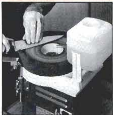
The curved profile and extreme length of a kitchen knife are problems for vertical wheels; the blade pivots during grinding. More blade contact—which yields a more uniform arc—is possible with type shown.
