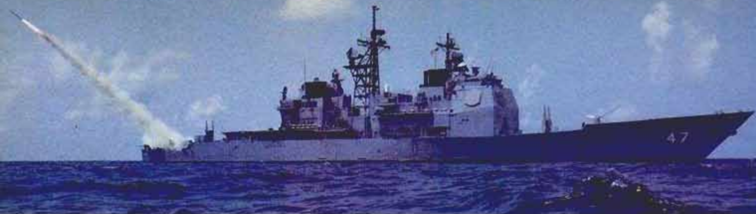
The Ticonderoga , the prototype Aegis -class destroyer, fires sophisticated Standard guided missile. Work is being done to trim some of weight from the fast ship's topside.
