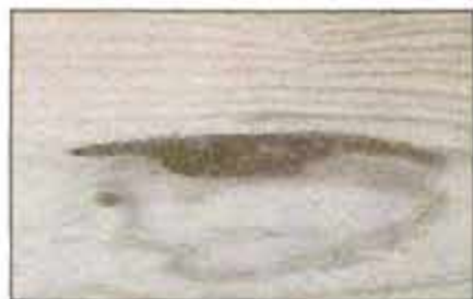
Pitch pocket is a seam or streak that holds or once held solid or liquid resin.
