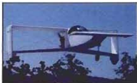
One of most radical new ARVs is Acro-X, a box-wing, canard biplane said to be super-easy to fly. About $8,000 with 50-hp mill.
