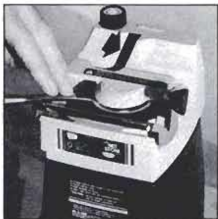
Not all water grinders are Japanese-made. Some American makers offer their own versions, like Wen unit above. It features an adjustable toolrest and an innovative guide slot (arrow) to sharpen twist drill bits.
