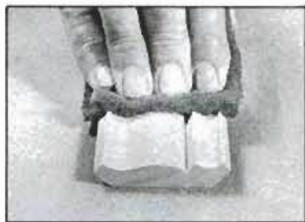
For final sanding on irregular shapes such as the molding shown, use a nonwoven nylon fiber pad in medium or fine grit. These are often sold for cleaning kitchen pots.
