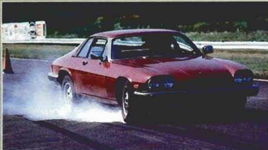
Braking test involves stopping in the shortest possible distance from 60 mph. Here, the big Jag locks up one front wheel and the driver turns wheels to correct skid.
