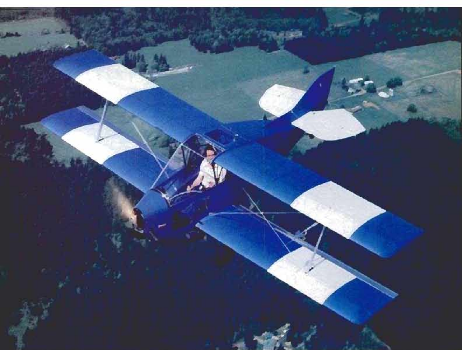
You can't get much closer to a real airplane and still be an unlicensed ultralight than this striking Sorrell Hiperlight, a negative-stagger biplane reminiscent of the famous Staggerwing Beech. It's $8,500 prefabricated or $6,500 as a kit, both with 28-hp engine.
