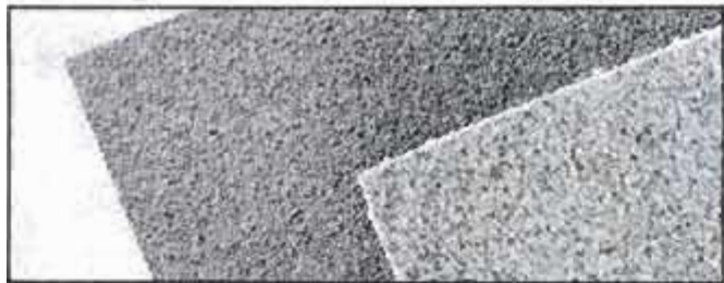
Closed-coat paper (left) has abrasive over entire surface for fast cutting. Open coat (right) has less coverage, won't clog as fast.
