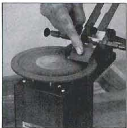
The advantages of horizontal wheel alignment are not limited to water grinders. Hone-Rite unit above has a ground-glass wheel on which you spread abrasive compounds, suspended in light oil.
