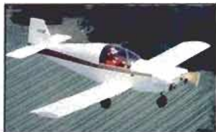
Tri-gear Questor weighs only 270 pounds, cruises at 120 mph on 37 hp and burns less than 2 gal. per hour. Kit is about $7,500.
