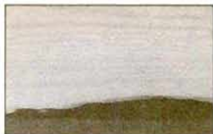
Wane is bark or missing wood along the edge of a board cut too near log surface.
