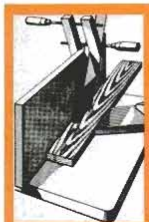
Use this setup for ripping long, thin stock.
