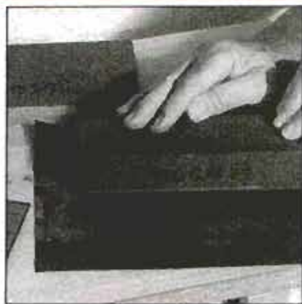
Japanese water stones wear faster than Western oil stones, so they must be flattened regularly. To do this, soak stone in water, then rub it over fine waterproof sandpaper until it is flat.
