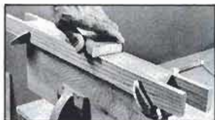
Sandpaper can also be used to achieve a true flat edge with the aid of two straight-edged boards clamped to the workpiece as shown. Use an unpadded sanding block.
