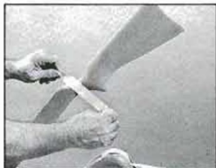
To sand sculptural shapes, cut cloth-backed abrasive into narrow strips and use like a shoeshine rag. Paper-backed abrasive will work if you apply masking tape to back.
