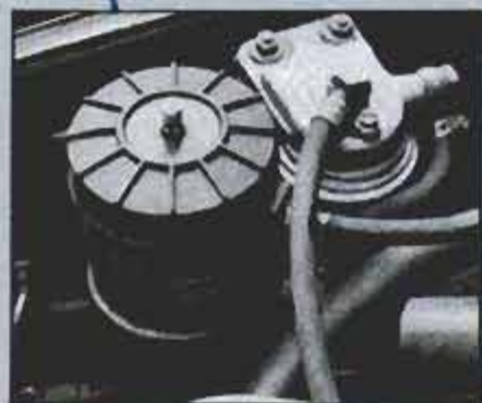
Fuel filter/water separator fits next to stock filter. In schematic above, the add-on parts are shaded, the VW parts are in white.
