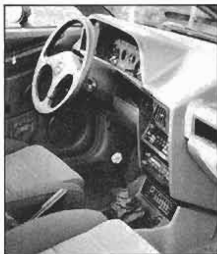
EXP interior benefits from a new dash, seats and door panels in '84. Turbocharged version gets sports seats and SVO wheel.
