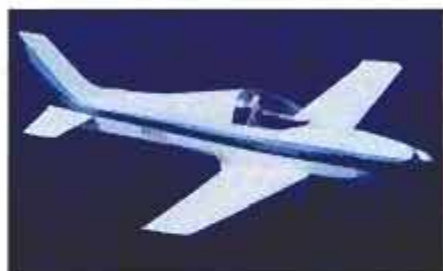
At 195 pounds, tiny Star-Lite could be an ultralight if it weren't so fast. It does 110 mph on only 20 hp, costs about $6,000.
