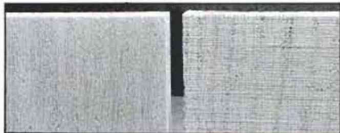
When sanding wood, work with grain (left), not against it (right). Latter yields deep scratches. Same grit was used on both boards.
