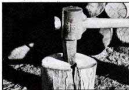
Use a maul to drive a steel wedge into the widest crack in the log end. This will split the wood where nature intended.
