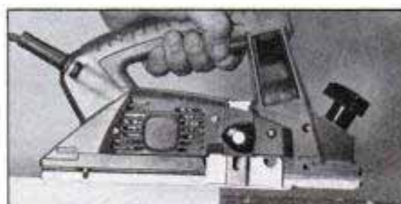
Maintaining the same flat tool alignment is equally important at the other end of a planing pass. Make certain that the tool remains level until the cutter has moved completely clear of the board's edge.
