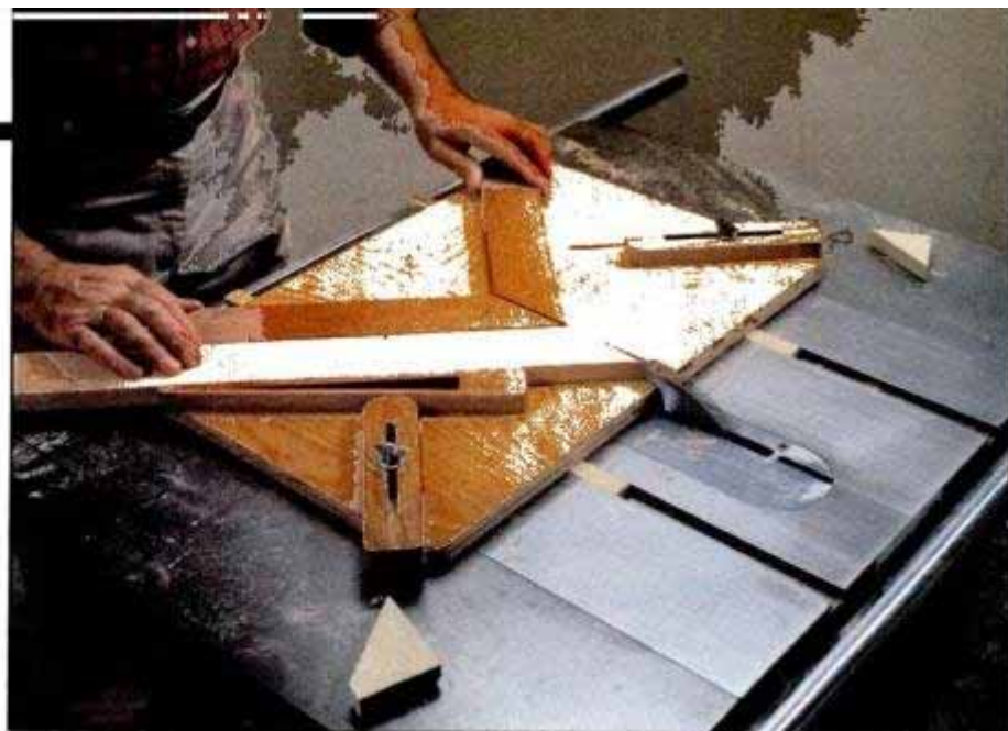
The table saw mitering gauge makes easy work of cutting precise 45° miter joints. Attach hardwood strips to the underside of the jig to fit into the saw table miter grooves which lock the jig accurately on course. The workpiece is held in place by the flexible wedge.
