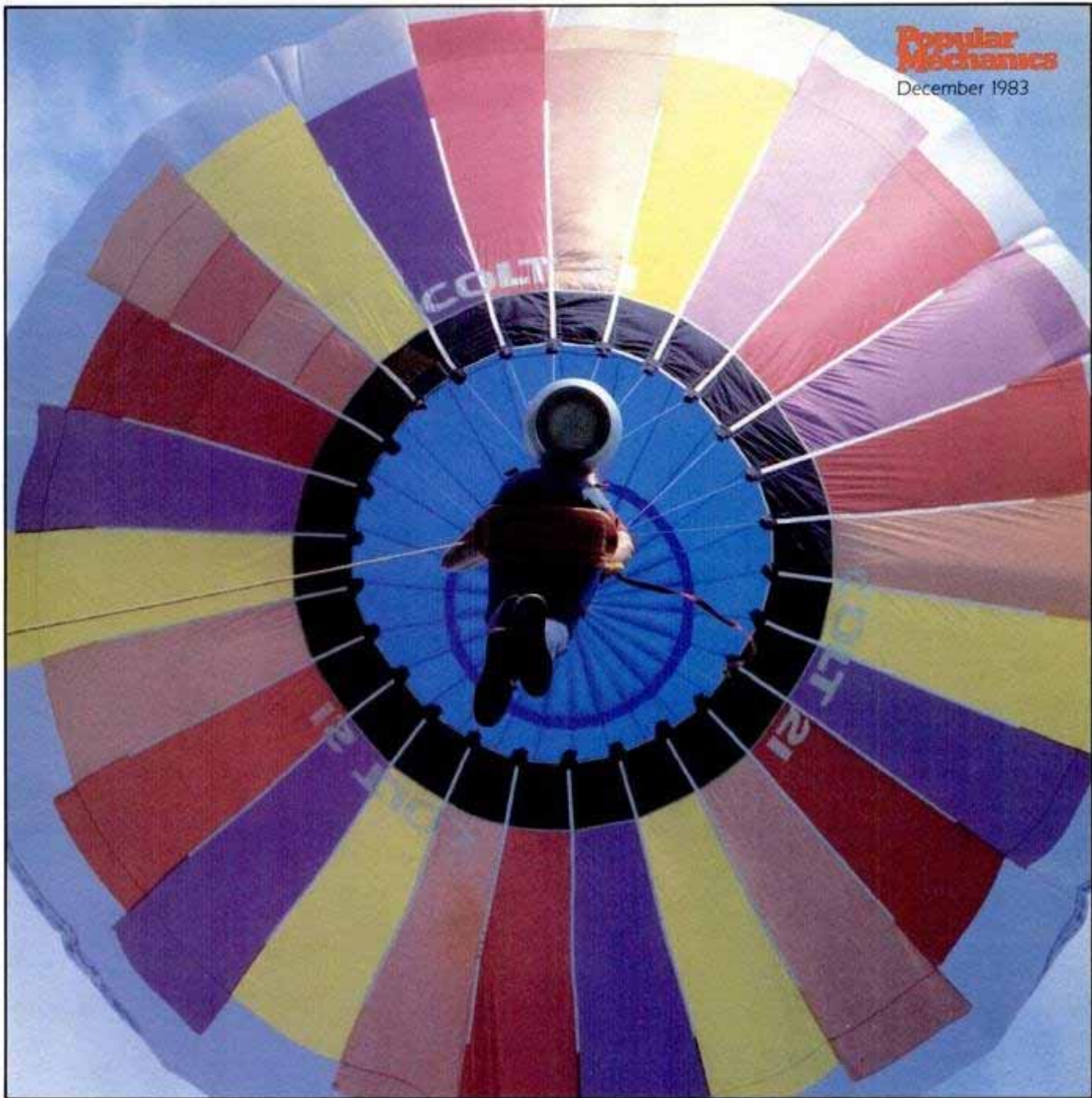
PM's Outdoors Editor hangs from the one-man Cloudhopper, supported by a plastic seat. A propane fuel tank is strapped to his back.
