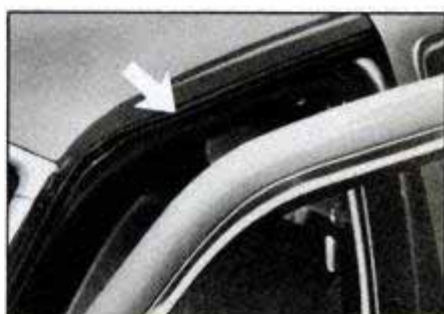
Elimination of rear-drive hardware means that the Tempo and Topaz can have a big, deep trunk (top). The transversely mounted, 2.3-liter, pushrod engine (left) impressed many owners with its pep. Doors curve into roof (right)—just like a T-Bird or Mercedes—but internal rubber rain gutter (arrow) gave some owners problems.
