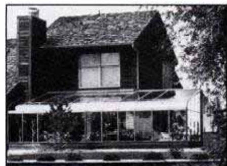
Flores II from English Greenhouse has a bronze-finish aluminum frame and double glazing, with acrylic glazing on curved parts. The 10-ft.-wide unit comes with sliding doors and operable windows.
