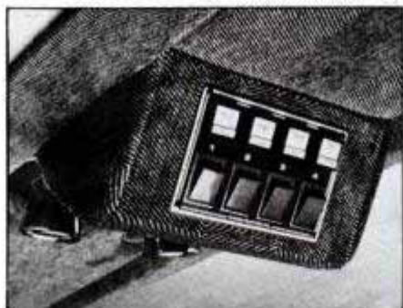
Circuit breakers and aircraft-style swivel lights are mounted in the ceiling console.
