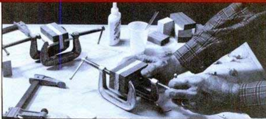
Assemble wood scraps into blocks with carpenter's or white glue, then secure blocks with C-clamps. Two-stage, walnut-ash glue-up at rear will be trimmed before it is turned.
