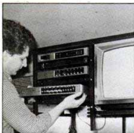
All of the components were installed in framework of 1-in.-sq. mild-steel tubing.
