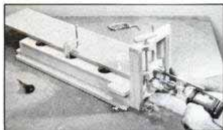
Attach a Portalign drill guide to the jig for boring holes in workpiece edges. Use the crankscrew mechanism to raise or lower the drill for exact, repetitive boring.
