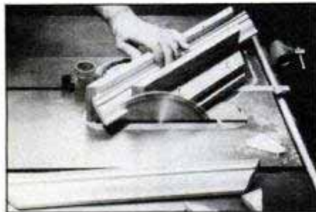
Screw the table saw jig to the miter gauge for cutting accurate compound angles on the table saw. Tack-nail the support wall to the base to hold molding securely.
