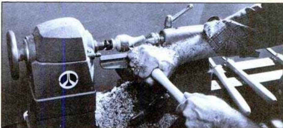
The new tool handles are spindle-turned using conventional turning techniques. Remove the end waste after the tang hole is bored (with the workpiece still on the lathe).
