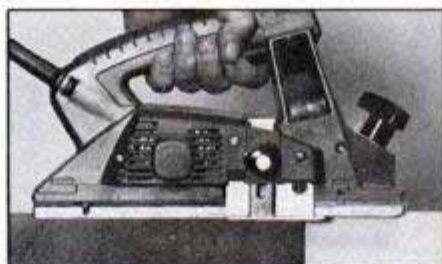
It's crucial that the plane be positioned properly before starting. It should rest flat on the board edge, as shown here, with the cutter not yet touching the wood.
