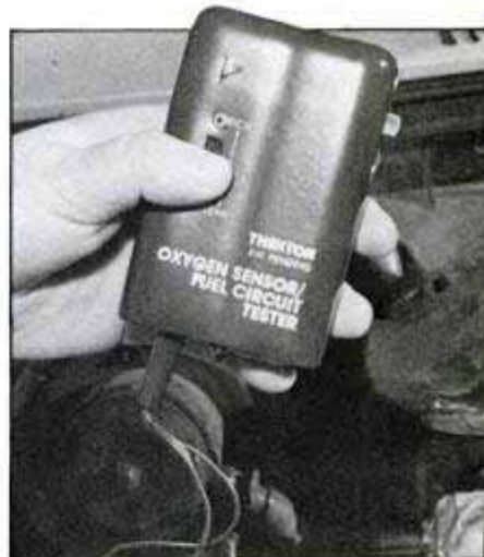
You may need an oxygen sensor tester to track down any rough running problems.
