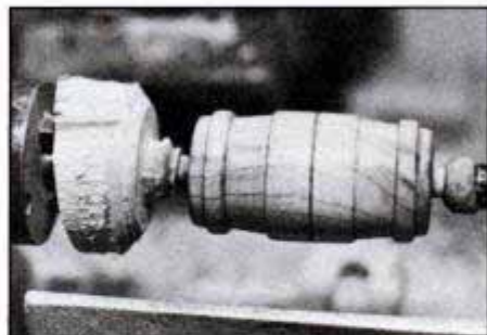
A little lathe work will turn a piece of cherry firewood into a gavel head. French polish finish brings out the grain.
