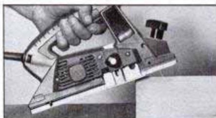
This exaggerated pose shows the wrong way to start a planing pass. But even if the back of the tool is just slightly lower than the leading edge, you will get a pronounced dip at the beginning of the cut.
