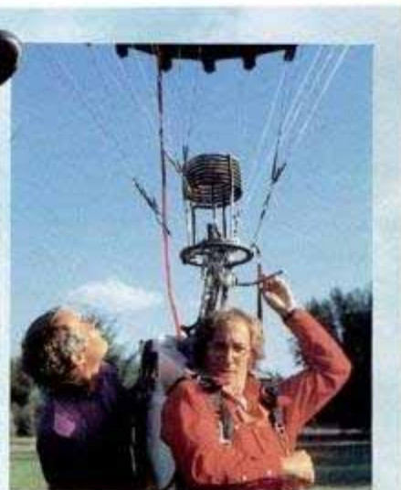
Balloon pilot Tony Chace gives Hill instruction on operating burner. Pulling lever with left hand ignites burner. Pilot light burns all the time, but burner is used only intermittently. At left, Hill practices balloon walking. He flies the Cloudhopper high enough so he can walk on a conventional-size balloon.
