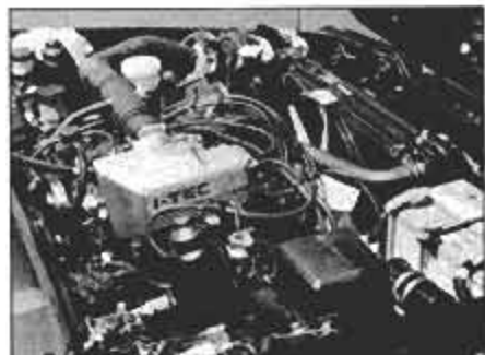
Fuel-injected, overhead cam, 90-hp engine delivers good, but not great, performance.
