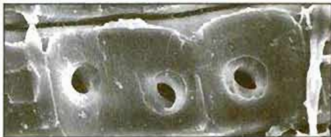
An electron micrograph reveals closed pores in modern violin wood (top). A new treatment can prevent them from shutting.
