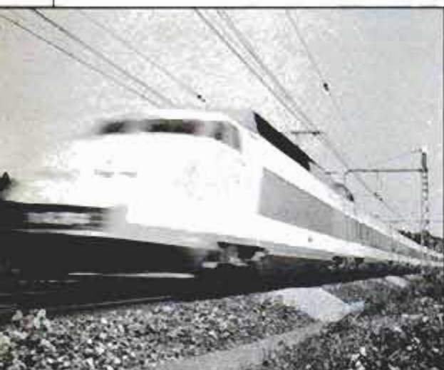
France's TGV bullet reaches speeds of up to 165 mph. The motorman goes along for the ride since the train is controlled by microprocessors in the tracks.
