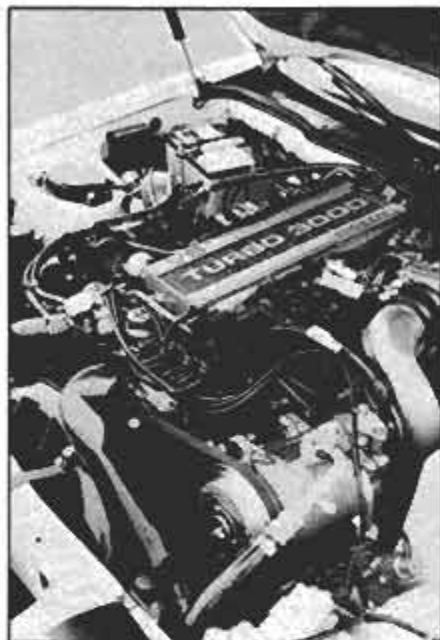
Unique 60° overhead-cam V6 engine produces 160 hp, 200 hp with turbocharger.
