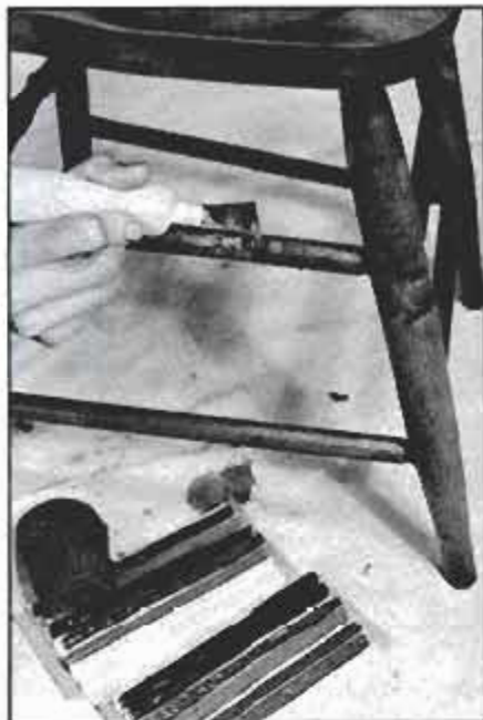
To fill gouges and cracks, melt stick shellac on the blade of an electric burr-in knife, then flow molten shellac into the hole.
