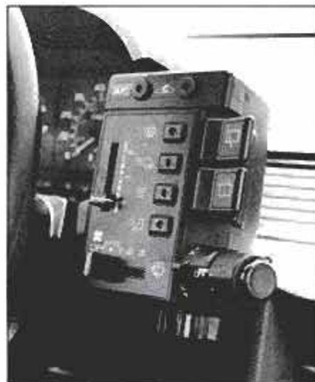
Pods on each side of the wheel give fingertip control of lights, wipers, A/C, vents.
