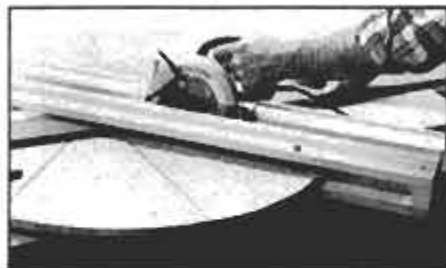
Here, a 45° miter is cut. Notice that guide rail is locked in place by the positioning pin.
