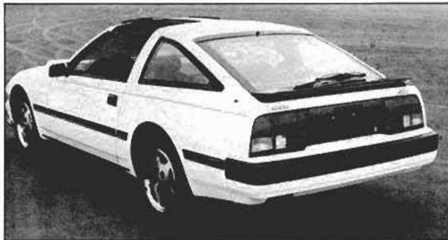
Z-car family resemblance is strongest from behind. The T-roof is standard on the 300.
