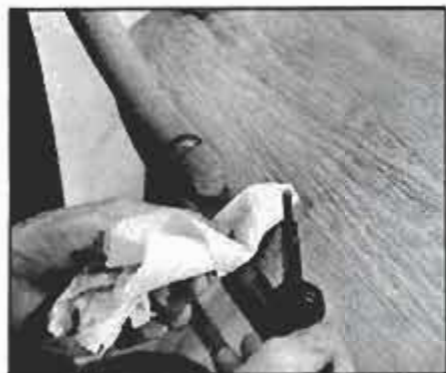
Raise dents by placing a moist paper towel into the depression with a hot soldering iron. The steam produced will swell pores.
