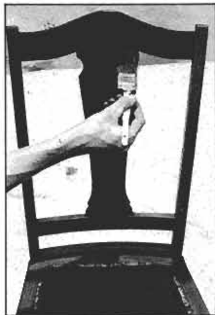
Allow stained wood to dry for at least 24 hours, then apply a sealer coat of 2-lb. cut shellac. Use a natural bristle brush.
