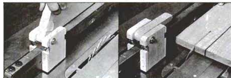
With the lever raised, position the jig at the desired distance from the blade (left). Then, push the handle down to lock the jig so that you can make exact, repetitive stopped cuts.
