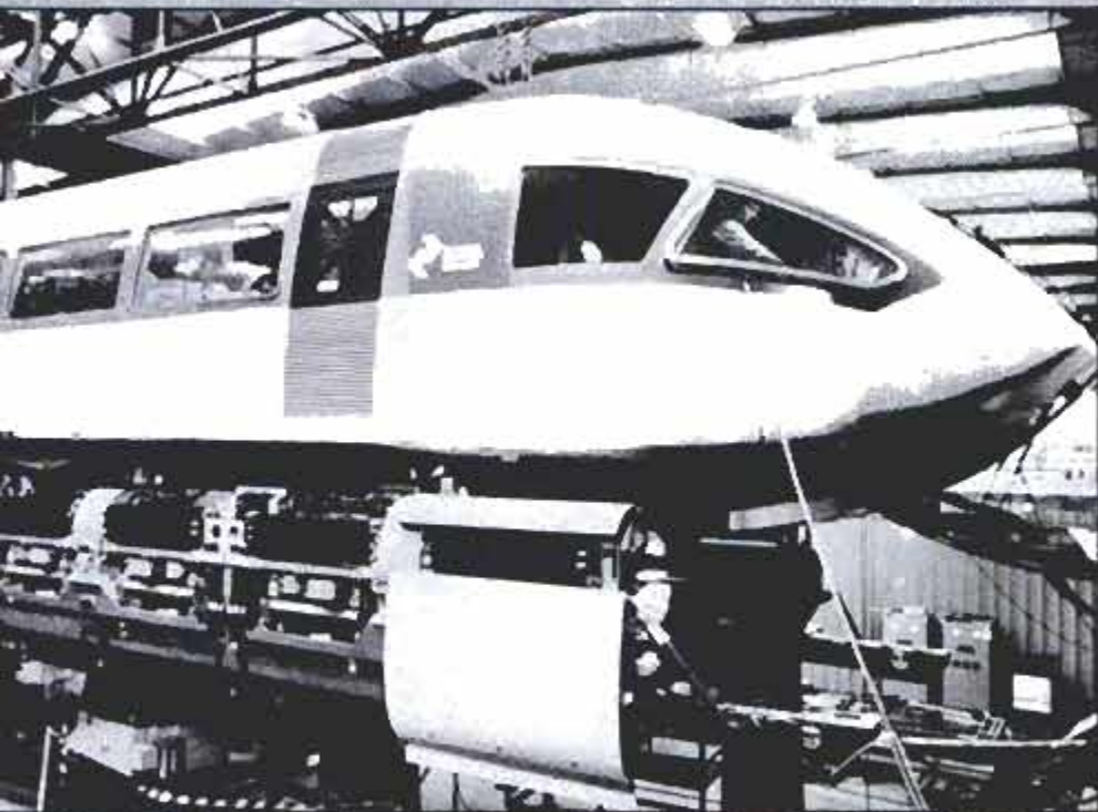
Side view of Transrapid shows guiding magnets that keep the 178-foot-long train on its forward run. Each car has a total of 60 magnets. Power is from a 110-kilovolt line.
