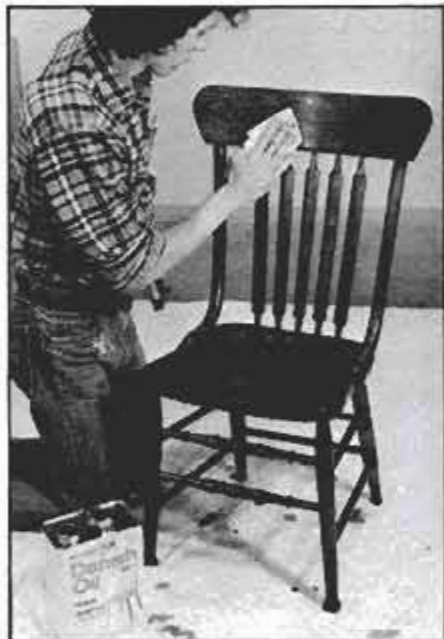
Allow one-step finishes like Danish oil to penetrate for about one hour. Then wipe away excess with a clean, dry cloth.
