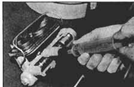
Inexpensive syringe bleeds master cylinders faster and easier than the high-priced kits.
