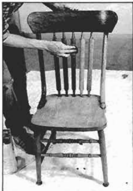
When stripping and repairs are complete, apply finish. The product here, a Danish oil finish, stains and finishes in one coat.
