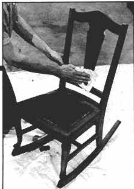
When applying a pigmented oil stain, brush it on straight from can, allow it to stand for about 10 minutes, then wipe off excess.
